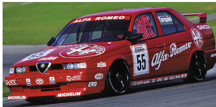
Alfa contributed to spiralling development costs with adjustable front splitter and elevated rear wing
