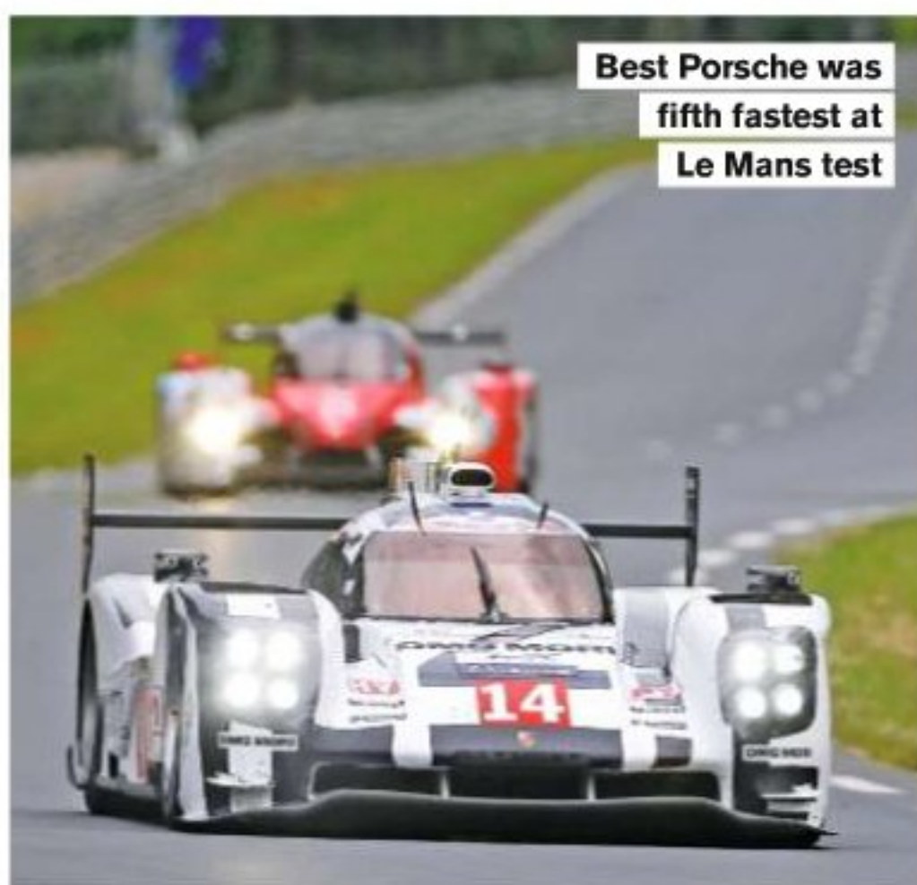
Hybrid power gives 919 temporary four-wheel drive
