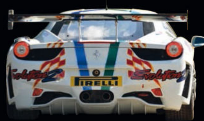
Aero Rear Bumper / Apron & Deep Double Diffuser
