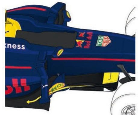
THE AREA UNDER THE RAISED FRONT OF THE chassis is ripe for development. Turning vanes and aero details work with the front wing to create the Y250 vortex, a strong airflow that spirals between the front wheel and chassis to keep the wheel's turbulence from upsetting the car's central bodywork.
