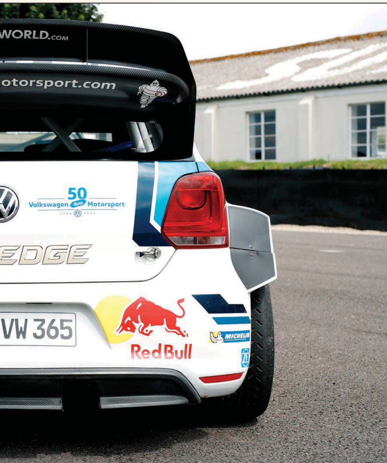
Everything in VW's latest Polo R WRC has been engineered to sit low down for the lowest possible centre of gravity.
