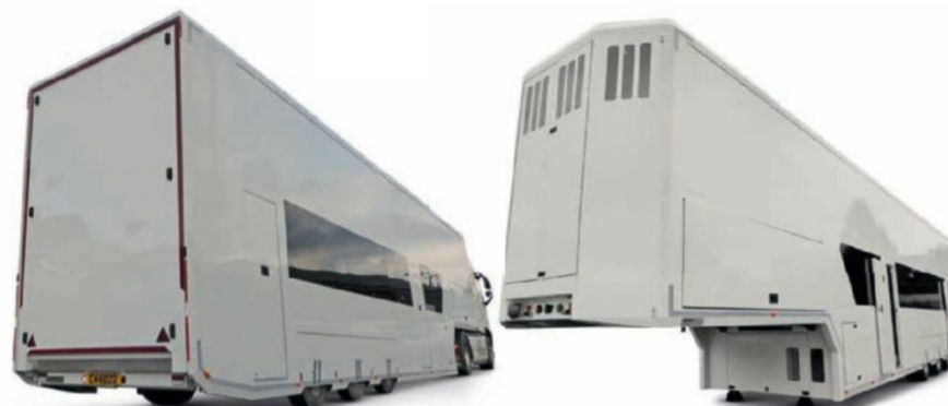
Lower deck as bulk storage/ car carrier
