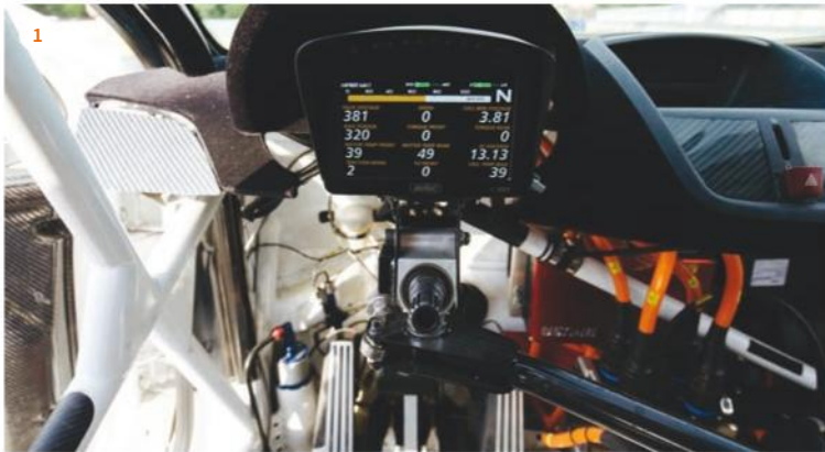
1 No gear lever, so handbrake takes its place
