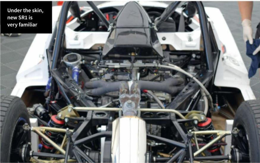
despite retaining almost all its inner workings and capability. Under the bodywork you'll find the same 175bhp RPE (Radical Performance Engines) tuned 1340cc Suzuki Hayabusa motorcycle engine and rear-wheel chain drive as the old car.
