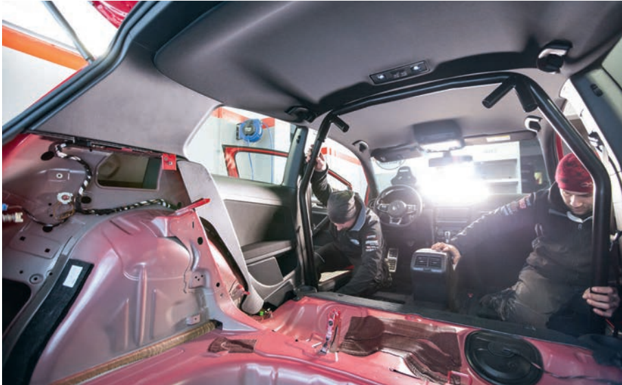
Clockwise from top: saving weight and adding a rollcage are first steps to improved performance; Wenzel marks out enlarged wheelarches; company works with top partners
