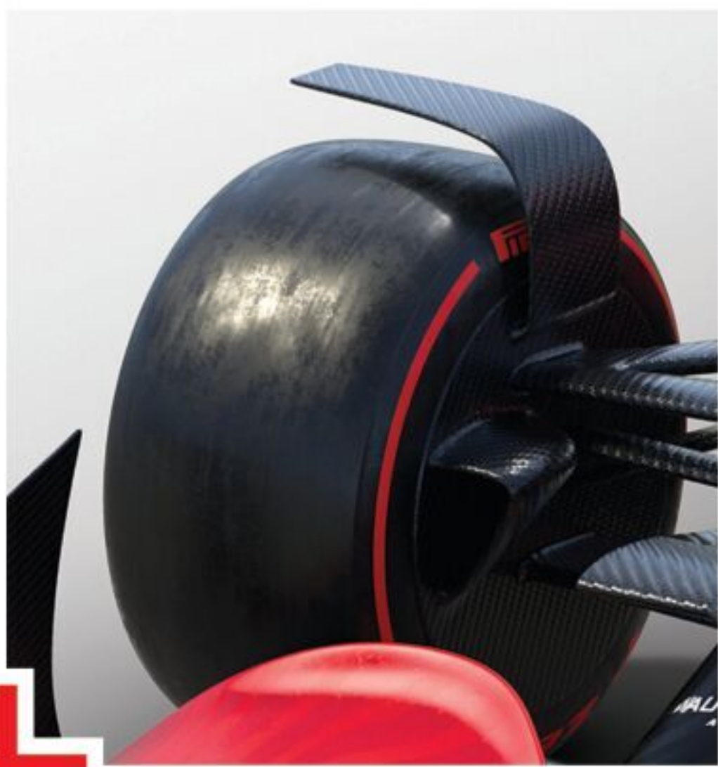
Deflector above the front wheels introduced to control turbulence
