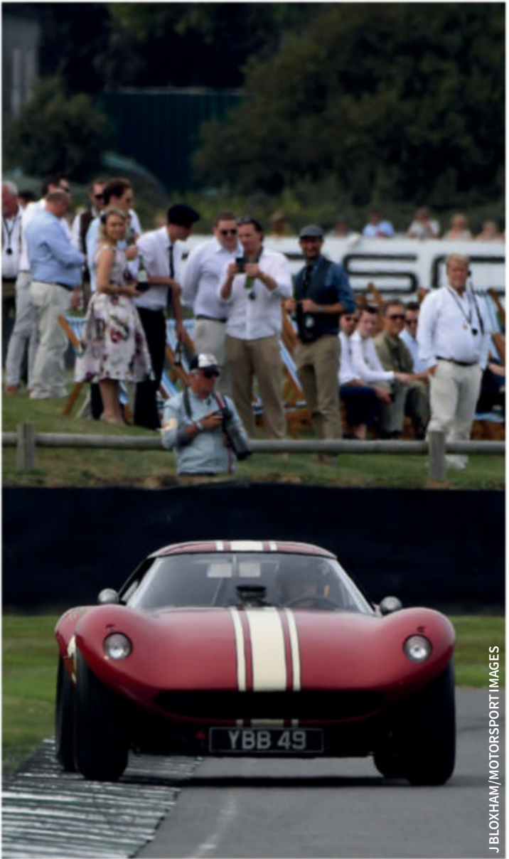
CHEETAH-CHEVROLET With short wheelbase, wide track, poor aero and 5.4-litre Chevrolet V8 engine, Bill Thomas's Cheetahs earned a reputation for being wild. Owner Duncan Pittaway and wide-eyed Stuart Graham didn't disagree.
