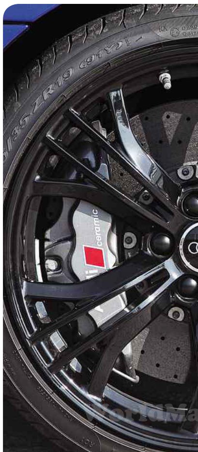
Above: new optional twin-clutch S-tronic transmission suits the character of the Plus. Left: carbon-ceramic brakes are standard
