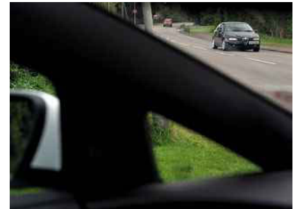
Above: view left at junctions is obscured by A-pillar. Below left: dials glow red in VXR mode. Below right: Competitive Mode relaxes ESP
