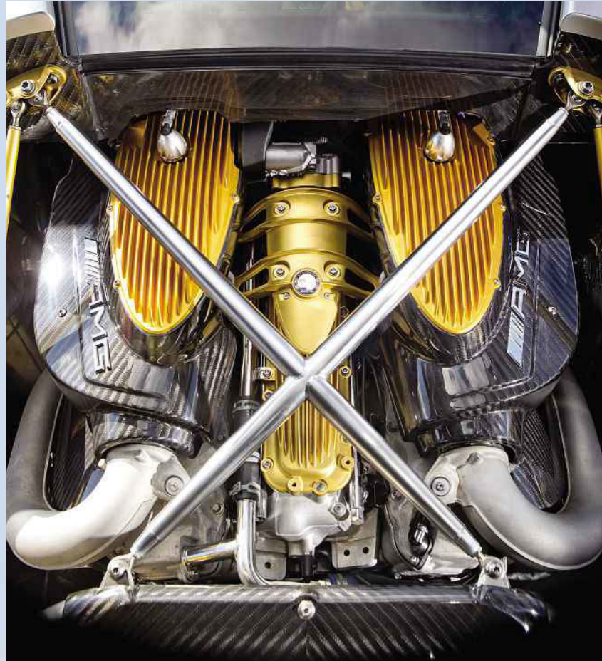
Left: Huayra's 6-litre, twin-turbo AMG V12 is every bit as gltzy as the rest of the car. Below: GT86 is playful at Blyton, if not that quick
