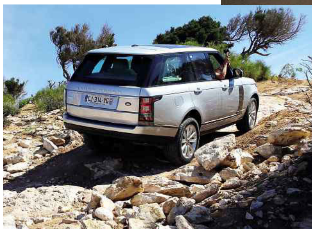
Above: 20in wheels were used in Morocco to reduce risk of punctures while off-road; standard wheels are 21s, while 22s can be specified
