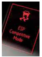
Above: view left at junctions is obscured by A-pillar. Below left: dials glow red in VXR mode. Below right: Competitive Mode relaxes ESP
