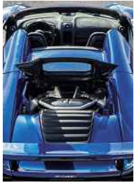
Above: 3.8-litre twin-turbo V8 produces 616bhp. Right: driver aids benefit the Spider's agility
