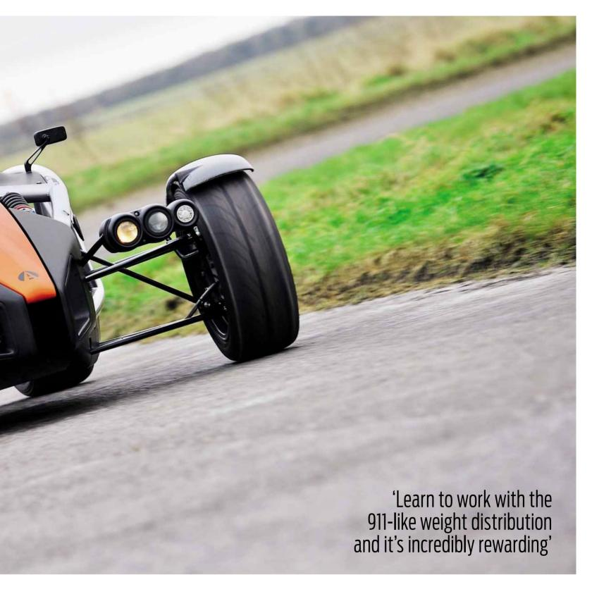
couldn't call it Atom 4 because a whole new integer only appears when the engine changes, but nevertheless there has been a raft of small upgrades. Most of the chassis changes are things that Ariel learnt while building the wild V8 model, with new suspension pick-up points and bracing around the engine all helping to make the chassis stiffer. The 3.5 also gets the carbon-surrounded digital dash from the V8, which looks very smart, and the nose panel has
