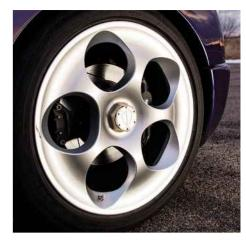
**Above left:** interior is the biggest clue to the age of the CC8S. **Above middle:** supercharged 4.7-litre V8 puts out 655bhp – an impressive figure today, but even more impressive back in 2002. **Above right:** wheels have centre-locking nuts and are 18in in diameter at the front, 20in at the rear; rears are 12.5 inches wide
