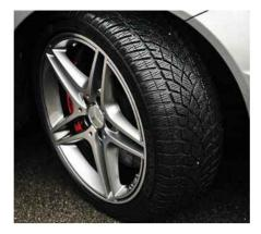
driven a car on winter tyres before, the first thing you notice on dry or damp roads is an odd feeling of looseness. The softer compound and, in this case, the taller profile necessitated by the inch-smaller wheels contributes to this. The 20mm narrower rear tyres mean that the rear footprint is also considerably smaller now, resulting in urgent and frequent flashes of the TC light.
