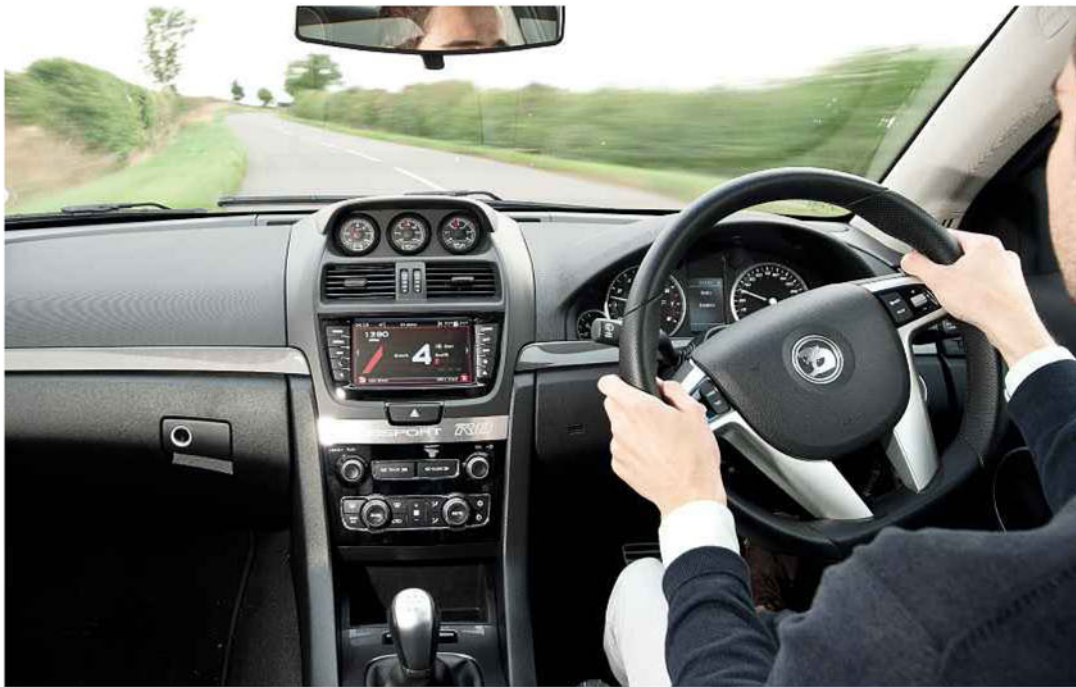
Above: interior is utilitarian, but central display (below left) boasts G and yaw meters, and a lap timer. Below left: 425bhp 6.2 V8
