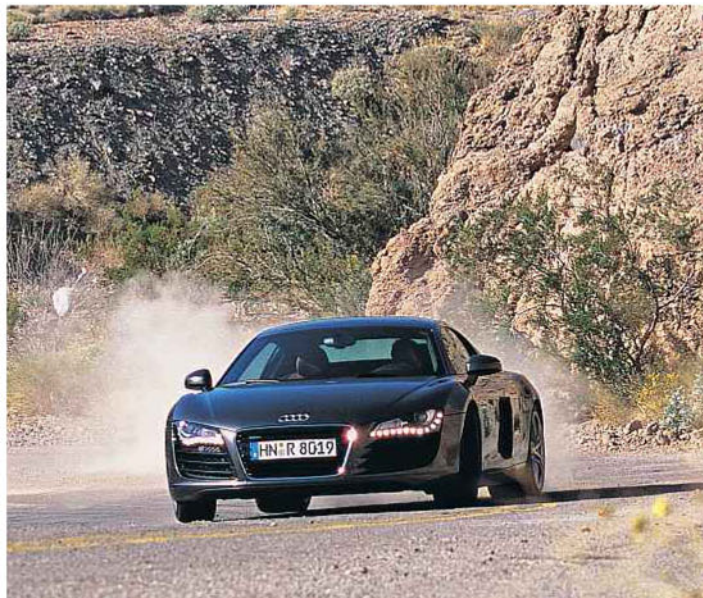
Above: R8 has quattro four-wheel drive, but a rear bias means oversteer is possible
