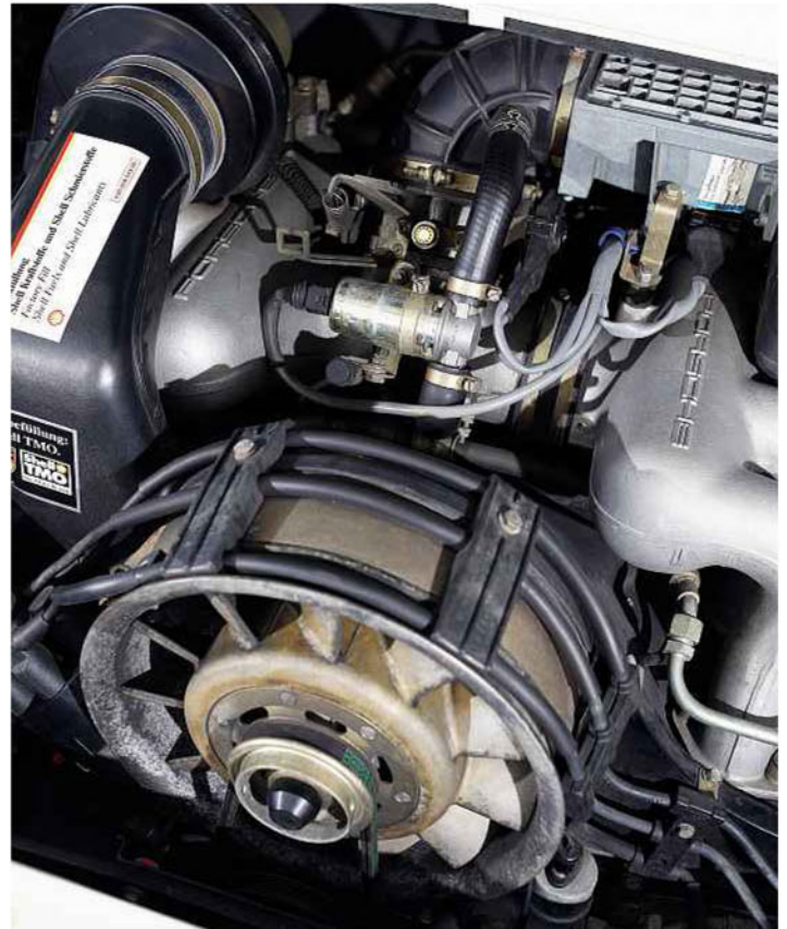
Above: weight-saving drive meant CS's windows had to be operated manually; 3.2-litre flat-six likely put out more than the 228bhp of standard Carrera, although Porsche claimed it didn't
