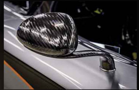
Above: body panels are made from a carbonfibre/kevlar mix. Right: sculpted door mirrors clean up side airflow
