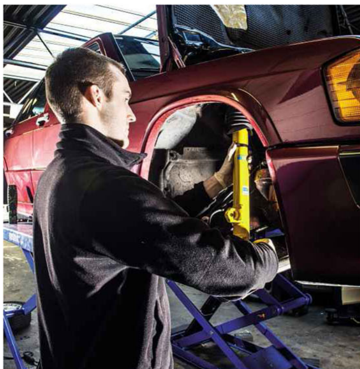
Above: new Eibach/Bilstein suspension was fitted by Autoclass in MK. Right: self-levelling hydraulics have been made redundant
