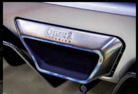
Above: air passing through the front cooling system is released via bonnet ducts with minimal drag. Above right: Alcantara and carbonfibre dominate interior. Right: titanium exhaust outlet is 3D-printed
