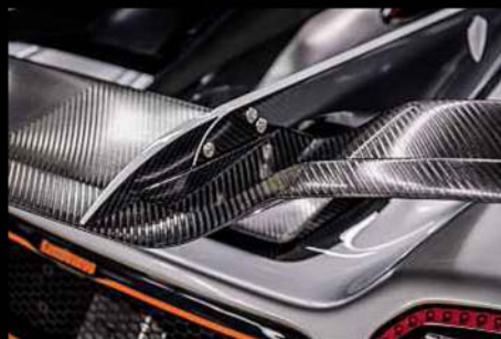
Far left: our man Bovington (left) with von Koenigsegg. Left: rear wing acts as an airbrake as well as generating downforce. Below left: wheels are carbonfibre. Below: the first One:1 in build at the Ängelholm factory
