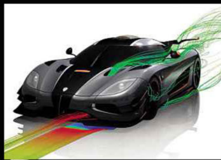
Above: air passing through the front cooling system is released via bonnet ducts with minimal drag. Above right: Alcantara and carbonfibre dominate interior. Right: titanium exhaust outlet is 3D-printed
