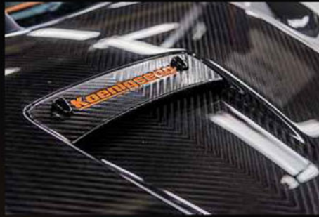
Above: body panels are made from a carbonfibre/kevlar mix. Right: sculpted door mirrors clean up side airflow
