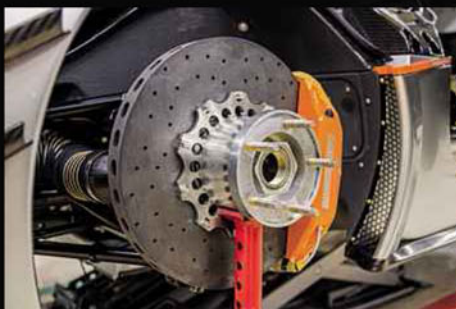
Above left: winglets form part of the One:1's new aero. Above: rear of the mid-mounted engine bears a '1M' graphic. Left: ceramic brakes help One:1 stop from 248mph in a claimed 10sec
