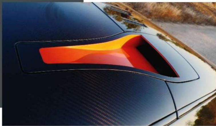
Above: Super Sport badge can be found in the engine bay on the newly enlarged chargecoolers. Left: don't kerb this. Each wheel takes BBS 30 hours of machining and costs the thick end of ten grand. Below: ducts are new for the Super Sport. The tub, including roof, is made of a new type of carbonfibre
