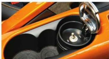
Above: door mirrors and rear diffuser are amongst the new carbonfibre exterior components. Below: interior battery cut-out switch (part of the 'Race' package) is hidden inside a pot in the centre-console cup holder
