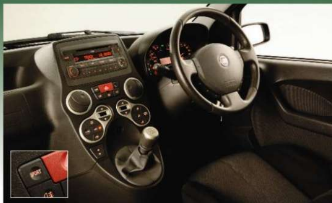
Above: engine is generally strong. Left: electrics can be troublesome; Sport button (inset) adds weight to steering
