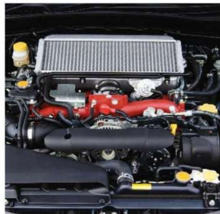
Above: turbocharged 2.5-litre flat-four still has 296bhp. Below: four-door body looks dull without big rear wing
