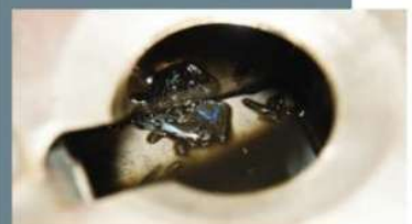
Above: traces of silicone inside the V8's sump were not a welcome find
