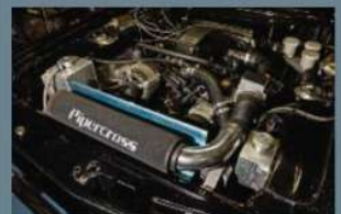
New Pipercross filter will keep the 5.2-litre V8 motor fed with cool air
