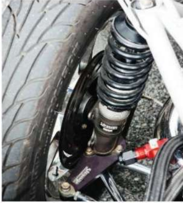
Above: front suspension uses 'Strange' MacPherson struts. Below: show-car finish extends to the door hinges
