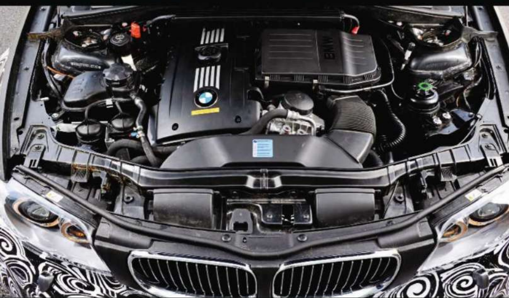
This is a development car, hence the camouflage paint and blanked badges. Interior (right) isn't finished either. However, the mechanical package, including an updated version of the twin-turbo straight-six (left) good for around 340bhp, the manual gearbox and rear suspension and M-diff from the current M3, feels great. A spiritual successor to the E30 M3 (far right)? Perhaps
