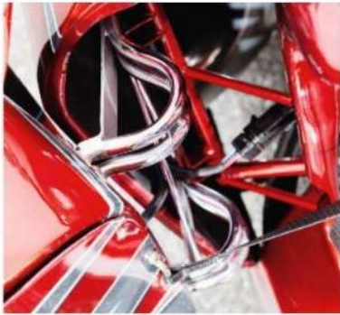
Above: front suspension uses 'Strange' MacPherson struts. Below: show-car finish extends to the door hinges
