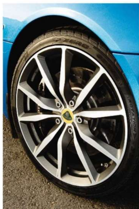
Above: neat supercharger installation lifts power of Toyota-sourced V6 from 276bhp to 345bhp. Above left: power slides now an option, despite lack of slippery diff. Below: optional diamond-turned forged alloys with sticky P Zero Corsas. Above right: diffuser is standard
