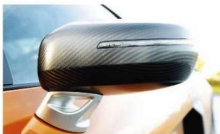
Above: door mirrors and rear diffuser are amongst the new carbonfibre exterior components. Below: interior battery cut-out switch (part of the 'Race' package) is hidden inside a pot in the centre-console cup holder
