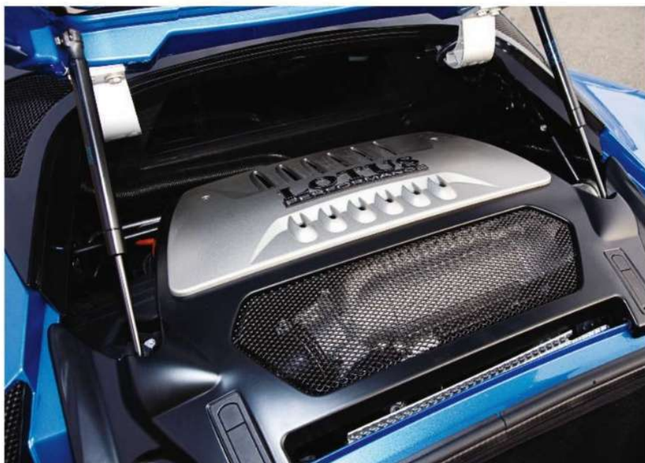
Above: neat supercharger installation lifts power of Toyota-sourced V6 from 276bhp to 345bhp. Above left: power slides now an option, despite lack of slippery diff. Below: optional diamond-turned forged alloys with sticky P Zero Corsas. Above right: diffuser is standard
