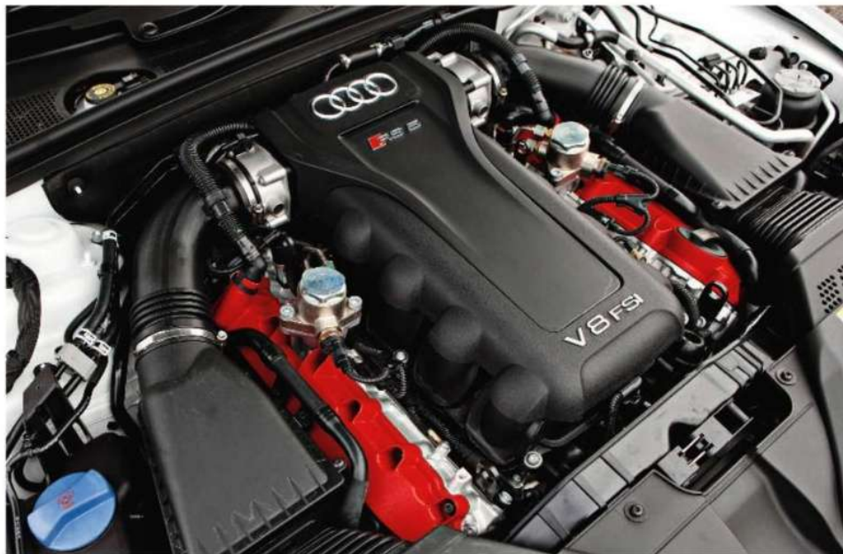
All four V8s are normally aspirated (enjoy them while you can). 4.2-litre Audi (left) and 4-litre BMW (below) both rev to well over 8000rpm. 6.2-litre Merc (above left) and 5-litre Lexus (above right) major on torque
