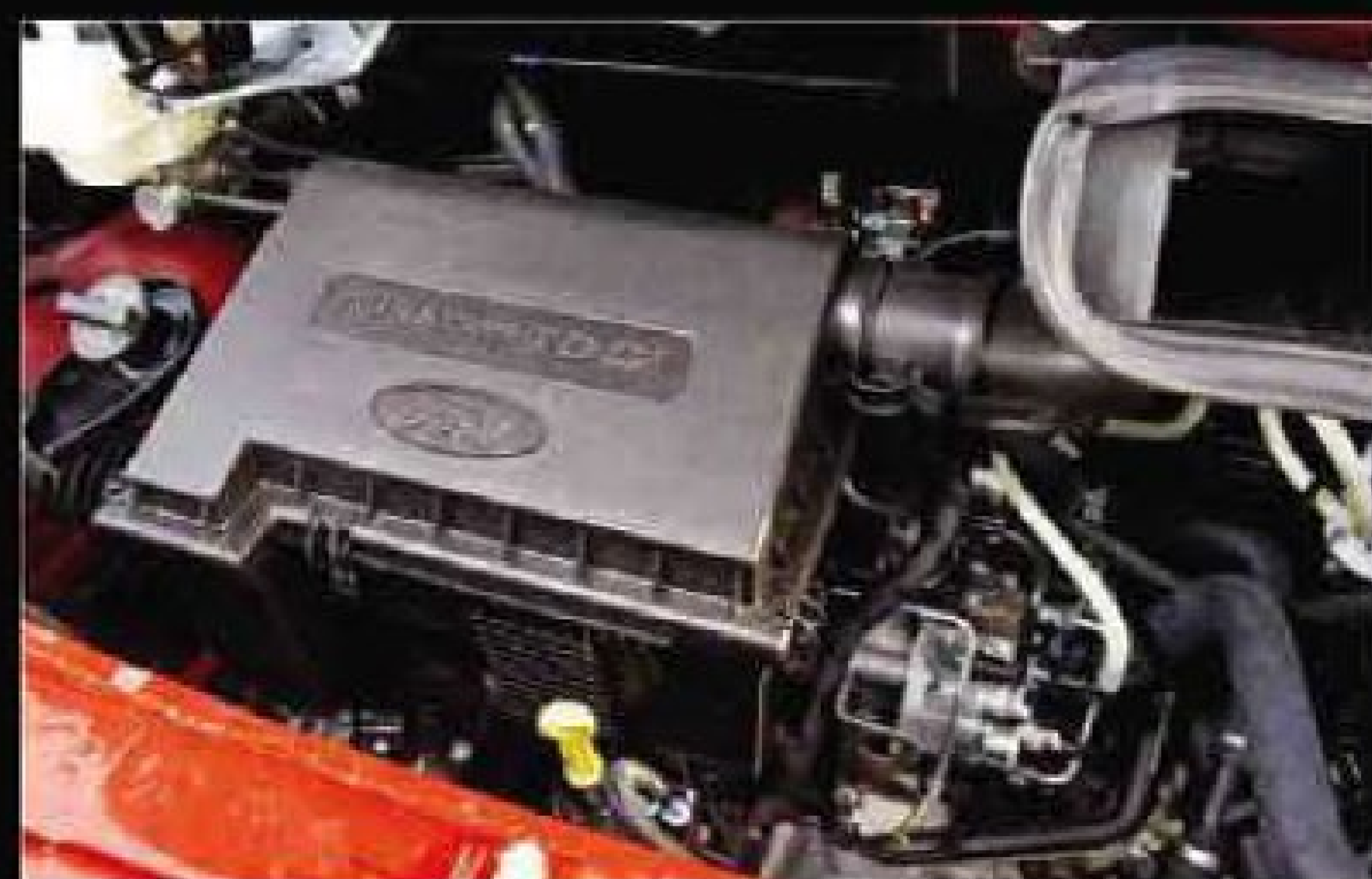
2.2-litre diesel is unchanged, but pumps out 258lb ft of torque
