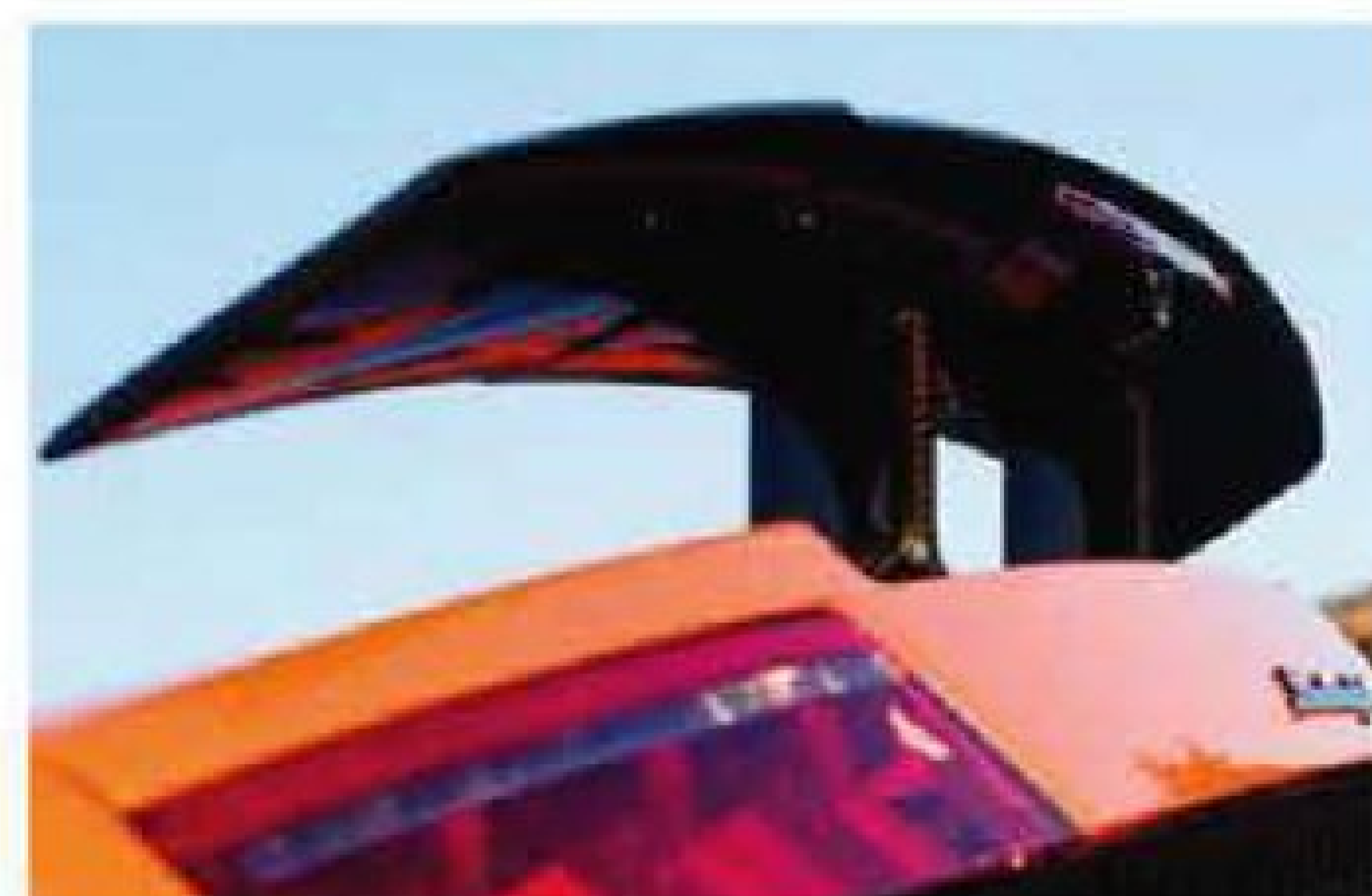
Above: large carbonfibre wing is standard; a smaller version is an option. Left: seats feature carbon shells
