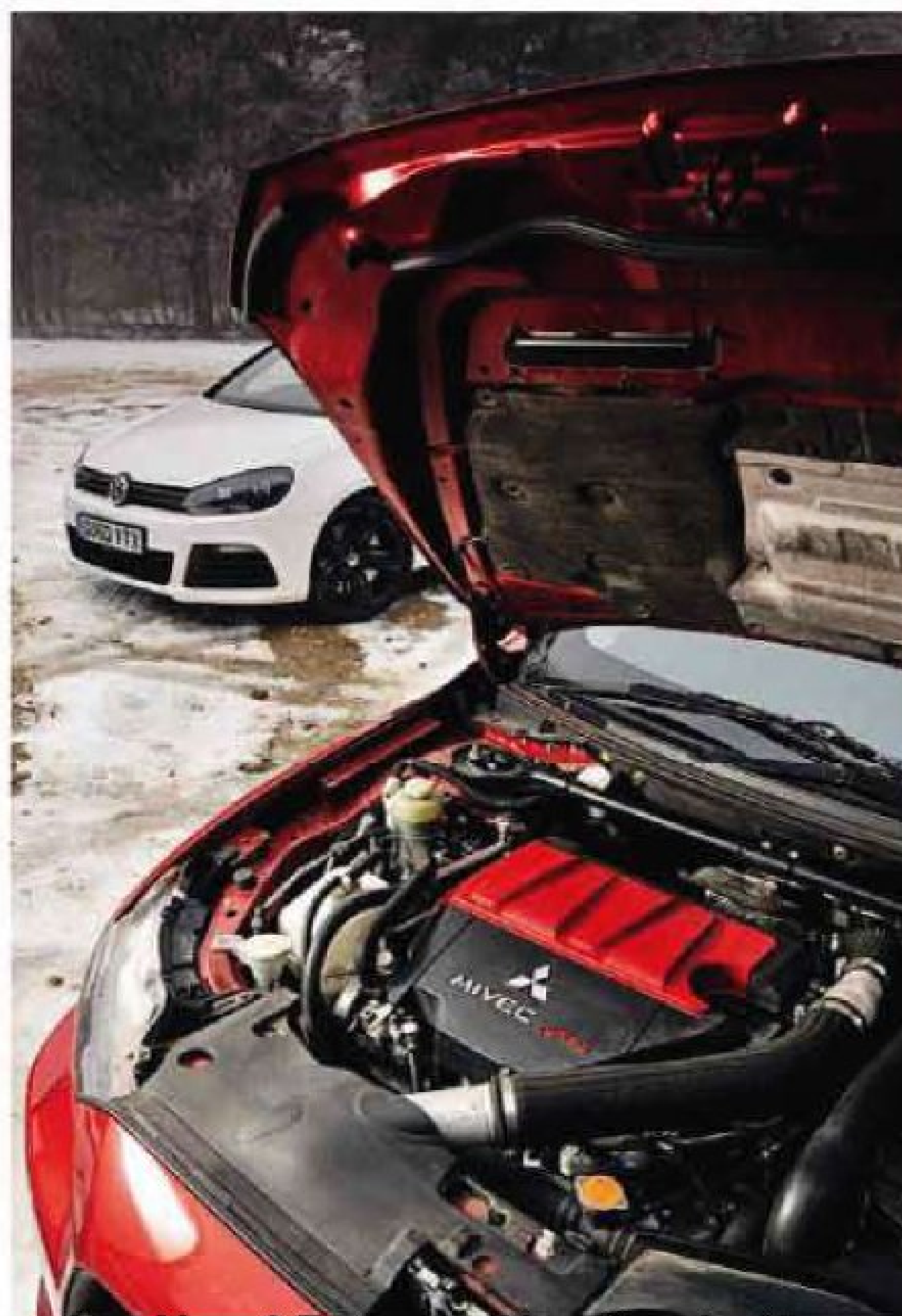
Above: STI's 296bhp turbo 2.5-litre flat-four. Evo (right) and Golf (below) have turbo 2-litre in-line fours with 290 and 266bhp respectively
