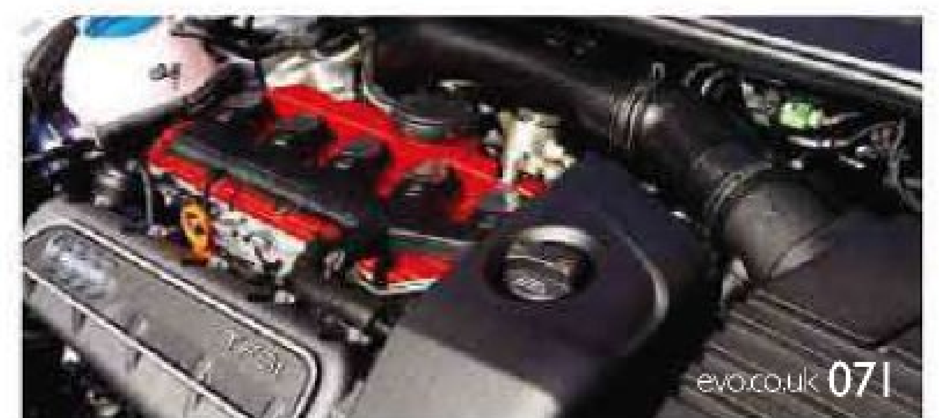
Single bonnet-vent is another nod to the Sport Quattro. Below: turbocharged 'five' from the RS TT sits longitudinally in the Quattro concept
