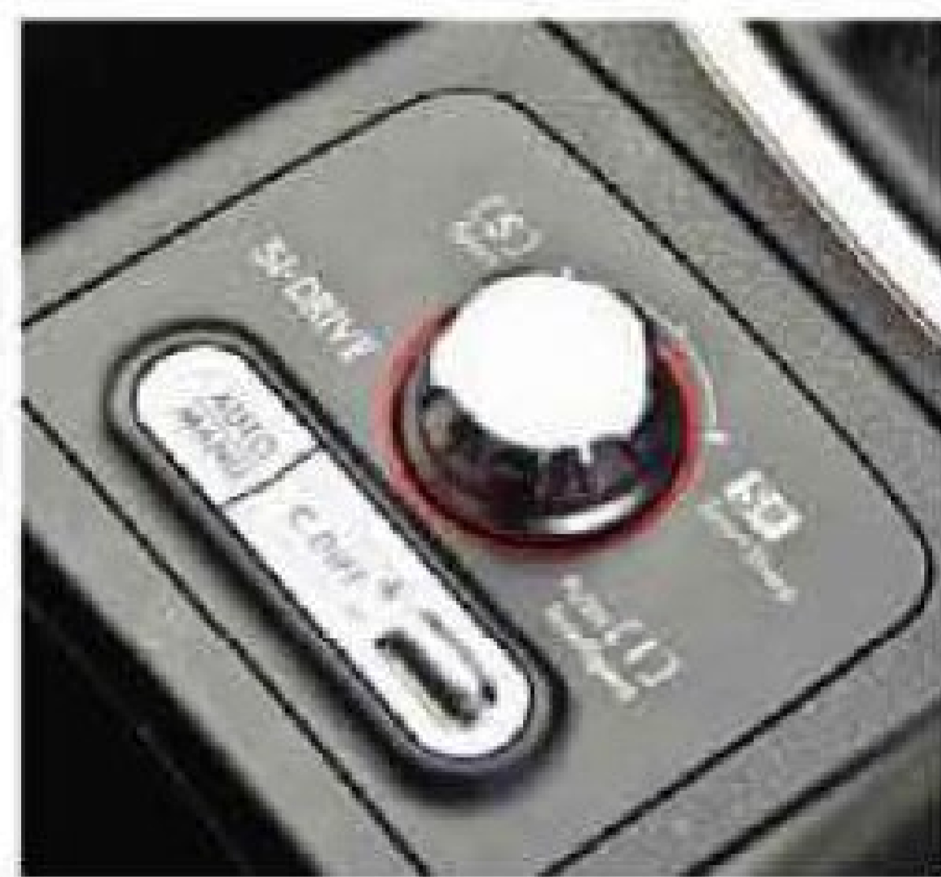
Left: Subaru's SI-Drive dial allows the driver to fine-tune the throttle response; C.Diff control alters the front:rear bias of the centre limited-slip differential. Below: toggle by the Mitsubishi's gearlever adjusts the shift speed of its dual-clutch gearbox
