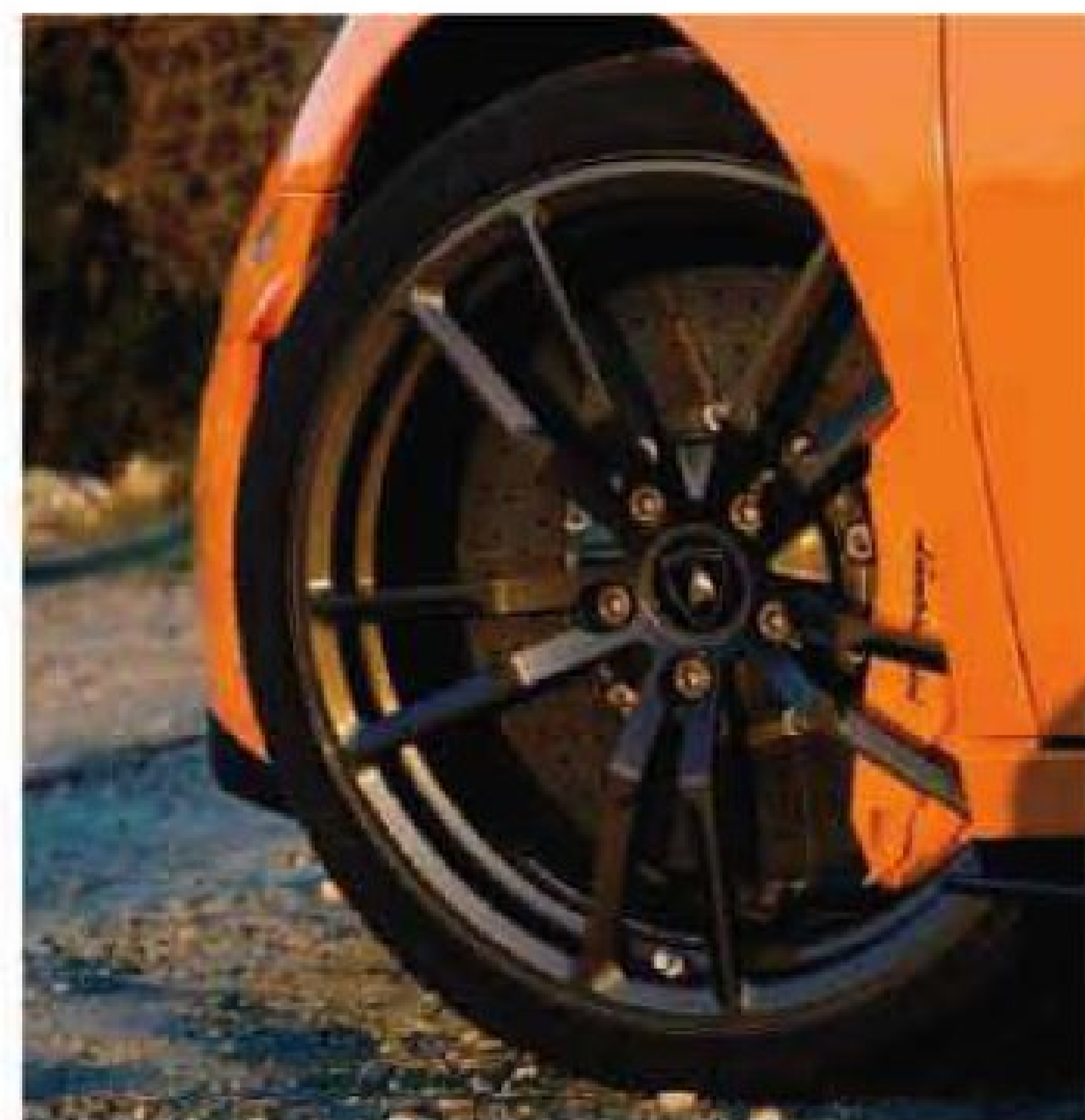
Above: engine cover, diffuser, sills and mirror casings are all carbonfibre; the material is responsible for 40 per cent of the weight savings. Below left: front spoiler is painted version of Superleggera item. Below right: 19in wheels are from Superleggera too; optional carbon-ceramic discs (clamped by eight-piston calipers) work best when used hard
