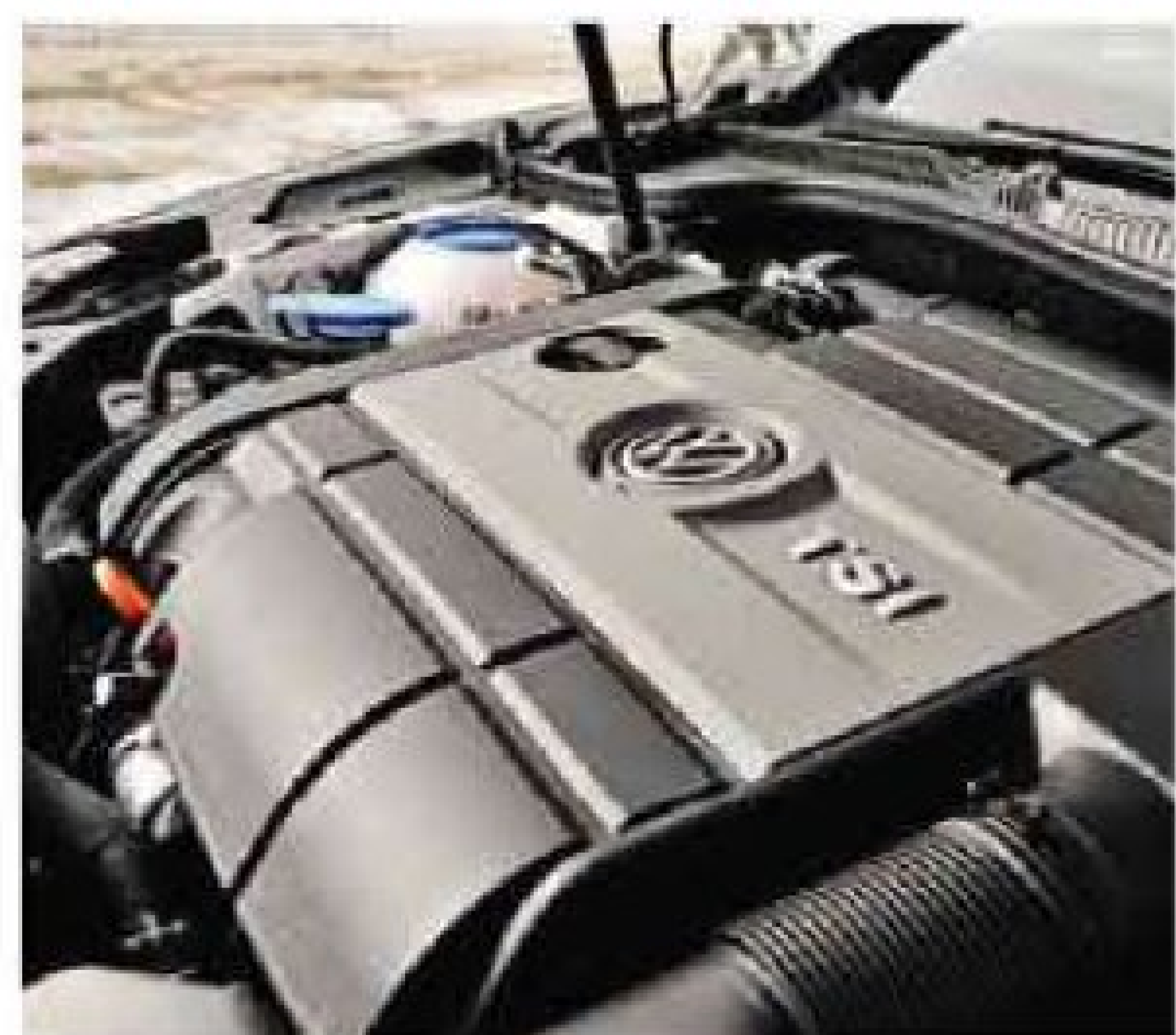
Above: STI's 296bhp turbo 2.5-litre flat-four. Evo (right) and Golf (below) have turbo 2-litre in-line fours with 290 and 266bhp respectively
