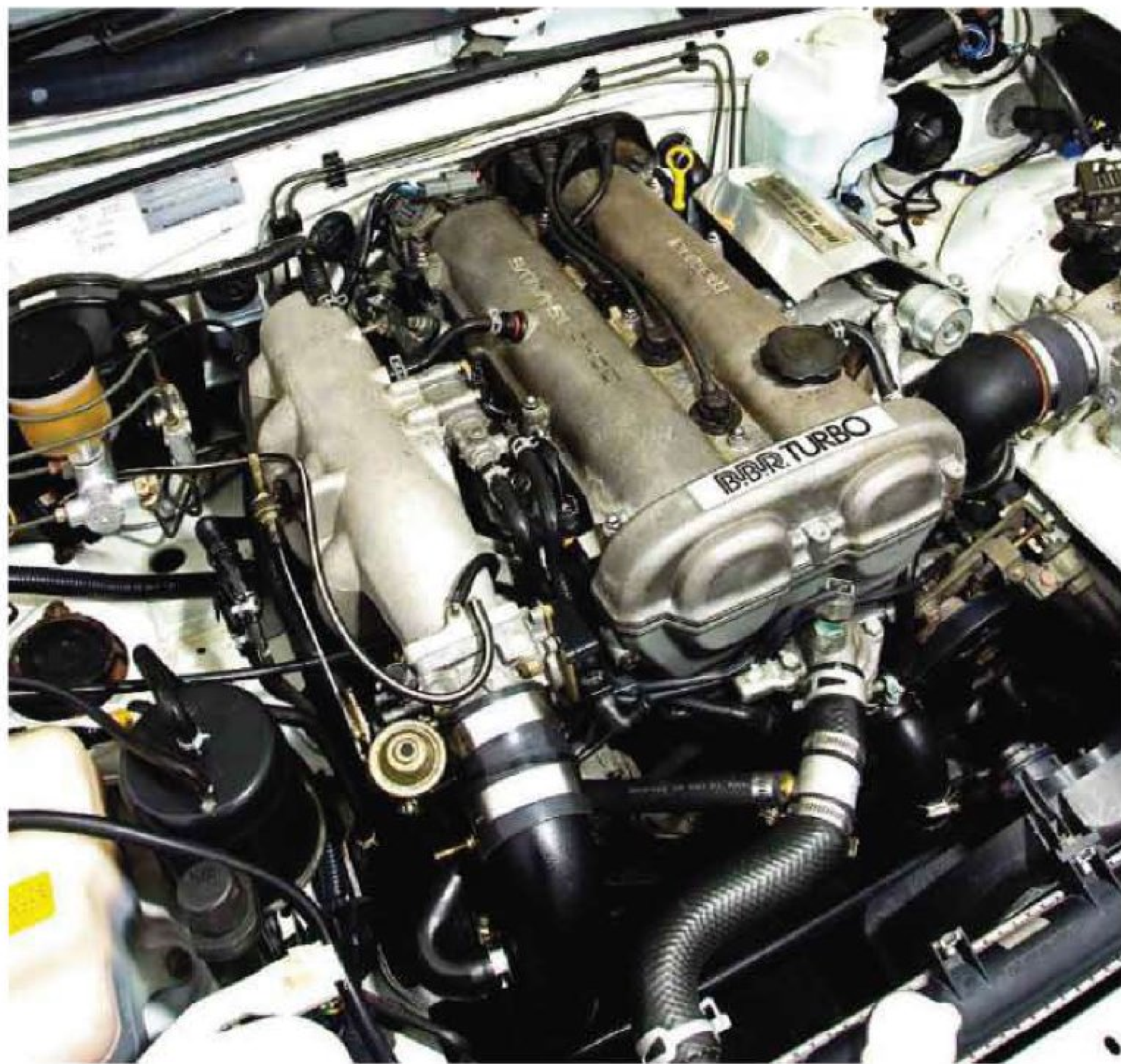
Above: turbo upgrade raises the outputs of the 1.6-litre motor by 105bhp and 75lb ft. Left: 16in alloy wheels, up from the standard 14s, are available from BBR as an option
