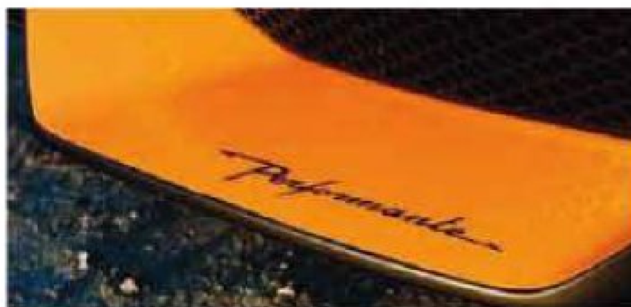
Above: engine cover, diffuser, sills and mirror casings are all carbonfibre; the material is responsible for 40 per cent of the weight savings. Below left: front spoiler is painted version of Superleggera item. Below right: 19in wheels are from Superleggera too; optional carbon-ceramic discs (clamped by eight-piston calipers) work best when used hard
