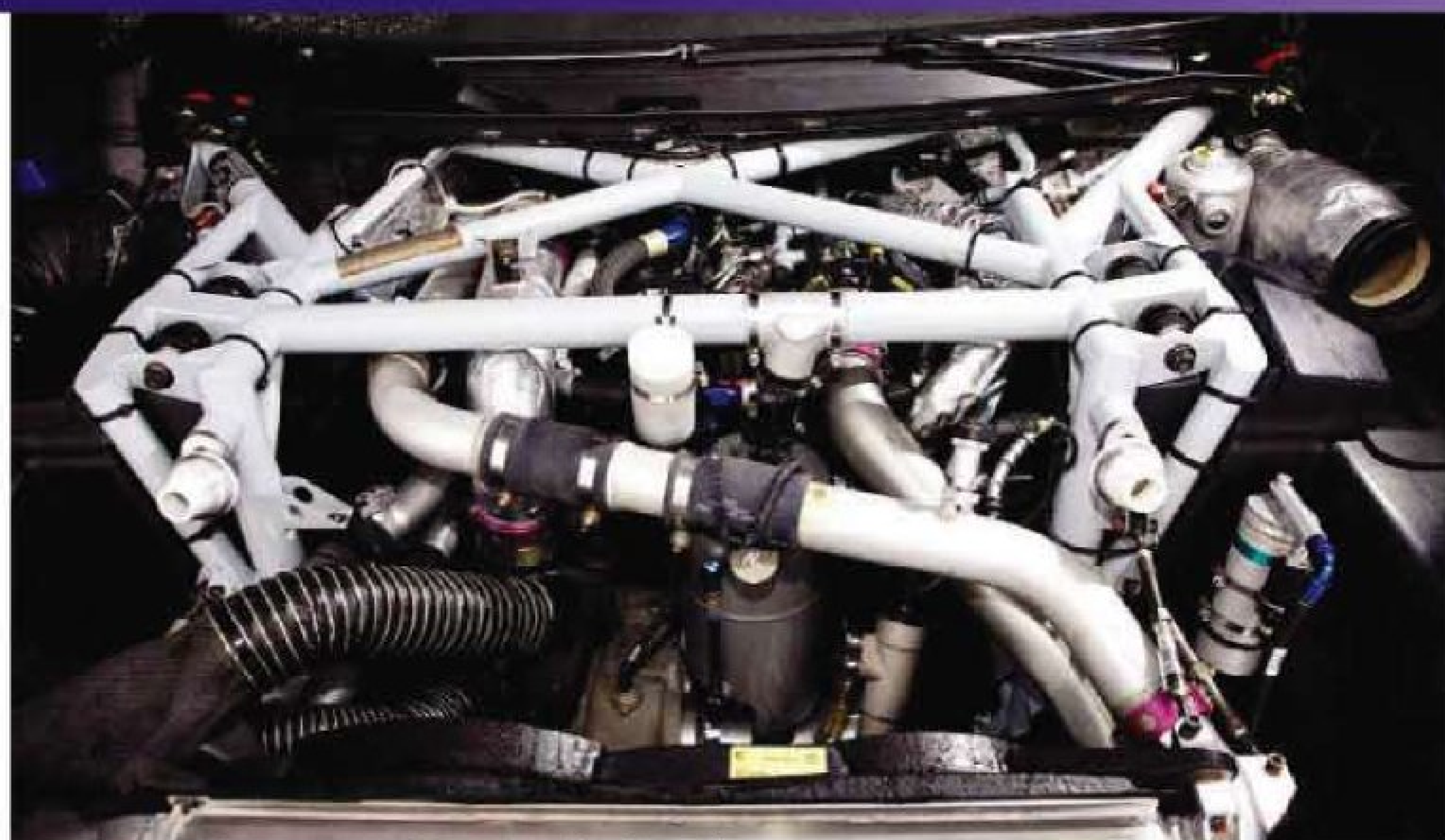
Above: 2.5-litre turbodiesel engine sits in the nose of the car beneath the high-strength steel spaceframe chassis. Below: exhausts exit from the Touareg's sills. Left: tyres have been specially developed by BF Goodrich
