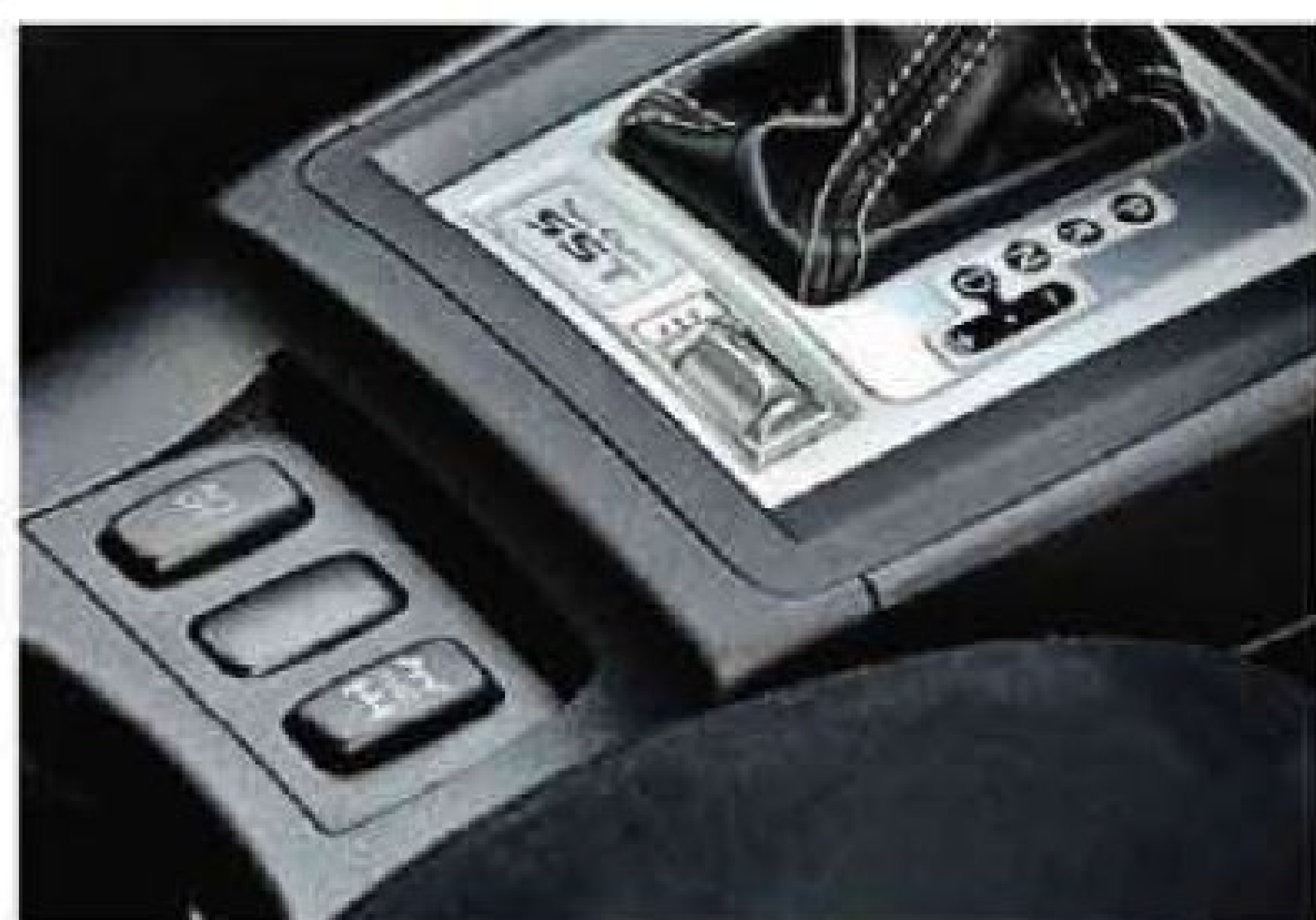
Left: Subaru's SI-Drive dial allows the driver to fine-tune the throttle response; C.Diff control alters the front:rear bias of the centre limited-slip differential. Below: toggle by the Mitsubishi's gearlever adjusts the shift speed of its dual-clutch gearbox
