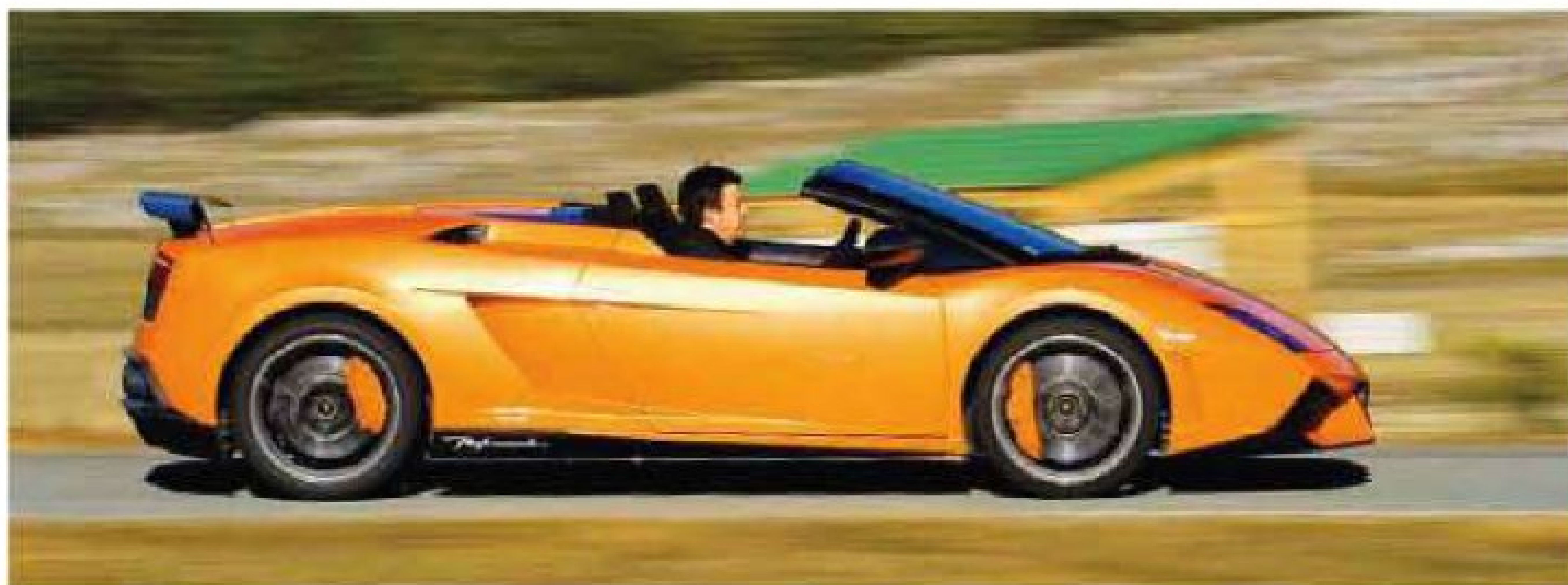
Above: engine cover, diffuser, sills and mirror casings are all carbonfibre; the material is responsible for 40 per cent of the weight savings. Below left: front spoiler is painted version of Superleggera item. Below right: 19in wheels are from Superleggera too; optional carbon-ceramic discs (clamped by eight-piston calipers) work best when used hard
