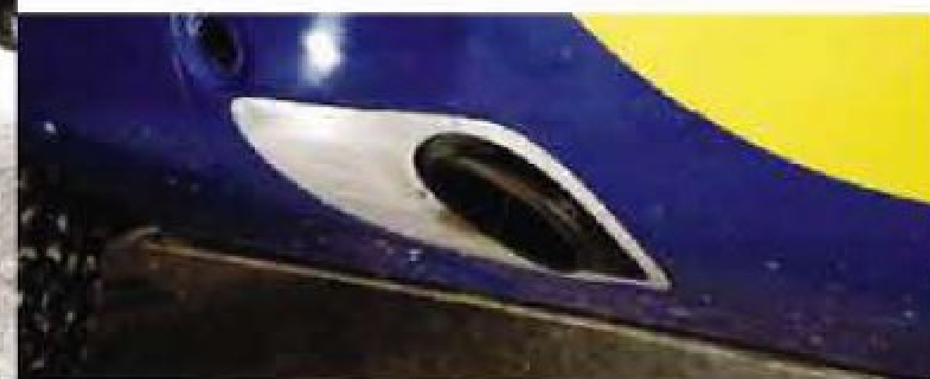
Above: 2.5-litre turbodiesel engine sits in the nose of the car beneath the high-strength steel spaceframe chassis. Below: exhausts exit from the Touareg's sills. Left: tyres have been specially developed by BF Goodrich
