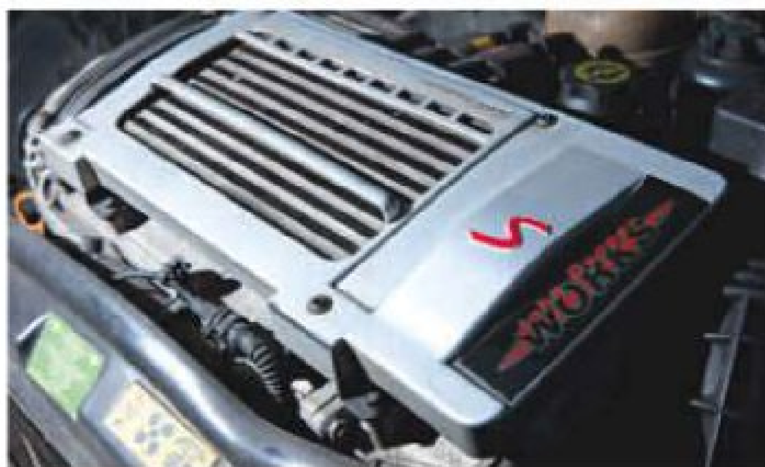
Above: supercharged 1.6-litre engine in Cooper S Works packs a beefy 210bhp. Mini puts it to good use
