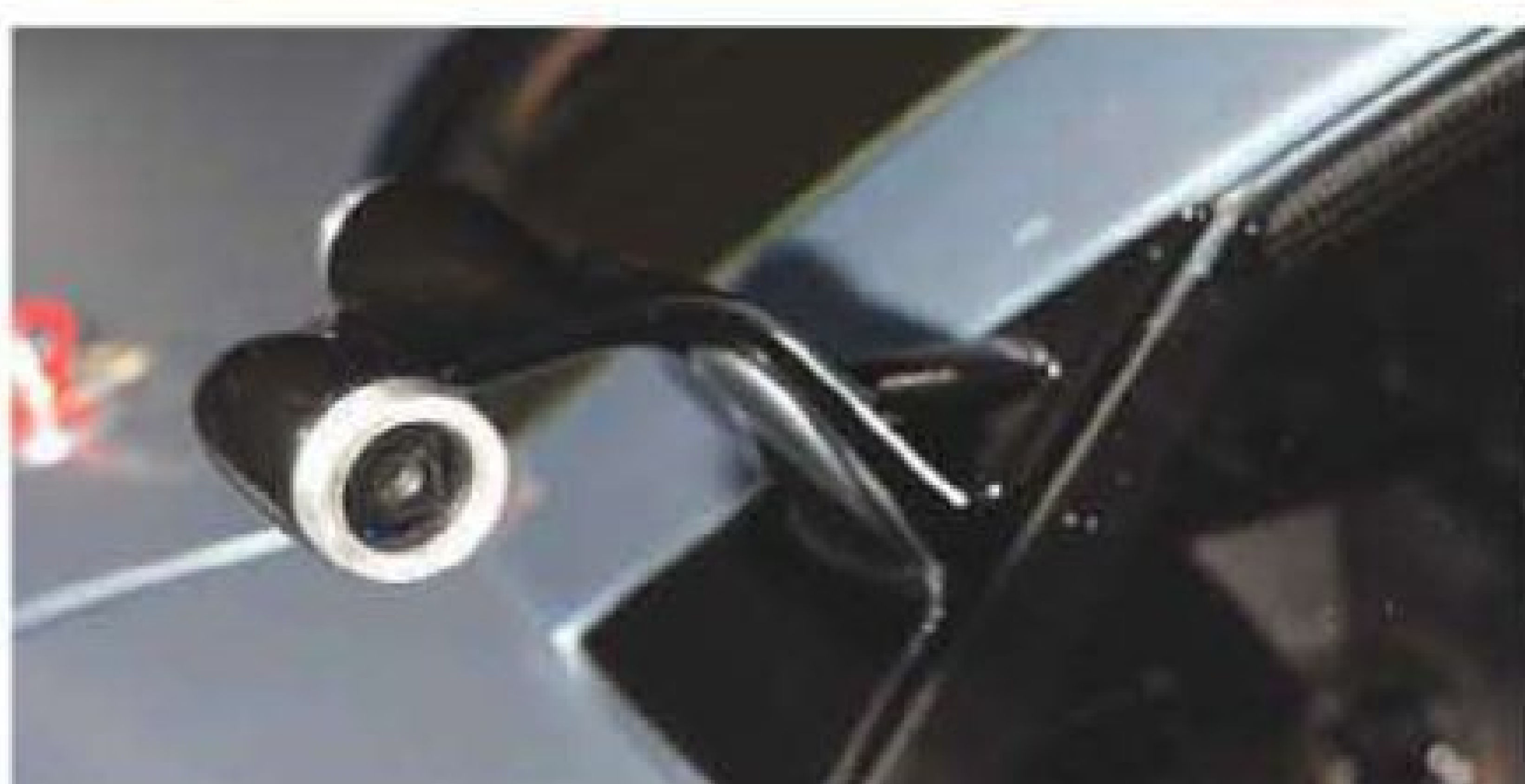
Right: flywheel resides in the cabin. Left: cameras act as mirrors. Below right: car bears names of regular Porsche racers Walter Röhrl and Marc Lieb
