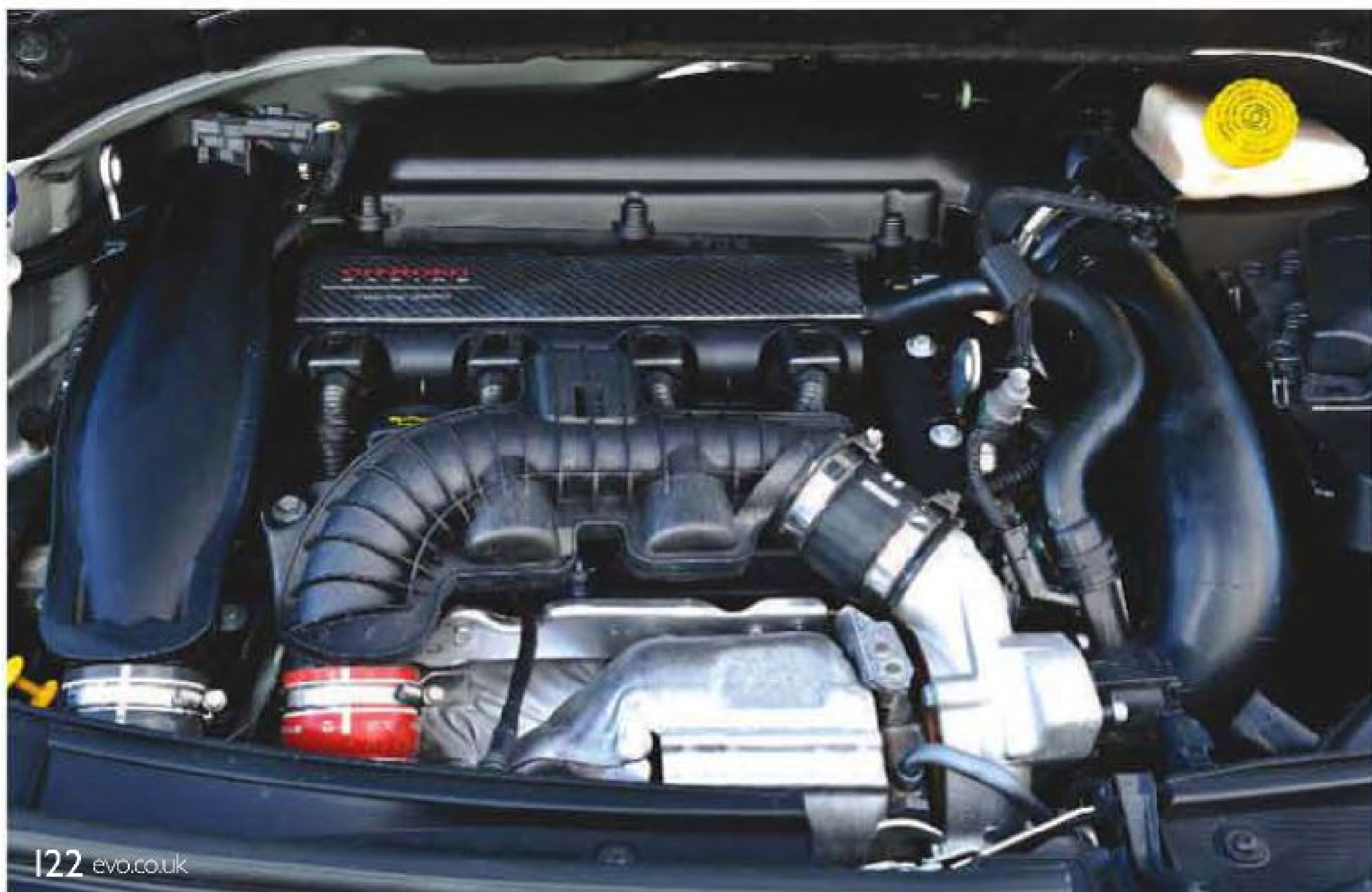
Engines, clockwise from left: DS3, VXR and Mini all have turbocharged 1.6-litre units, the VW has a twin-charged 1.4 and the Clio a naturally aspirated 2-litre
