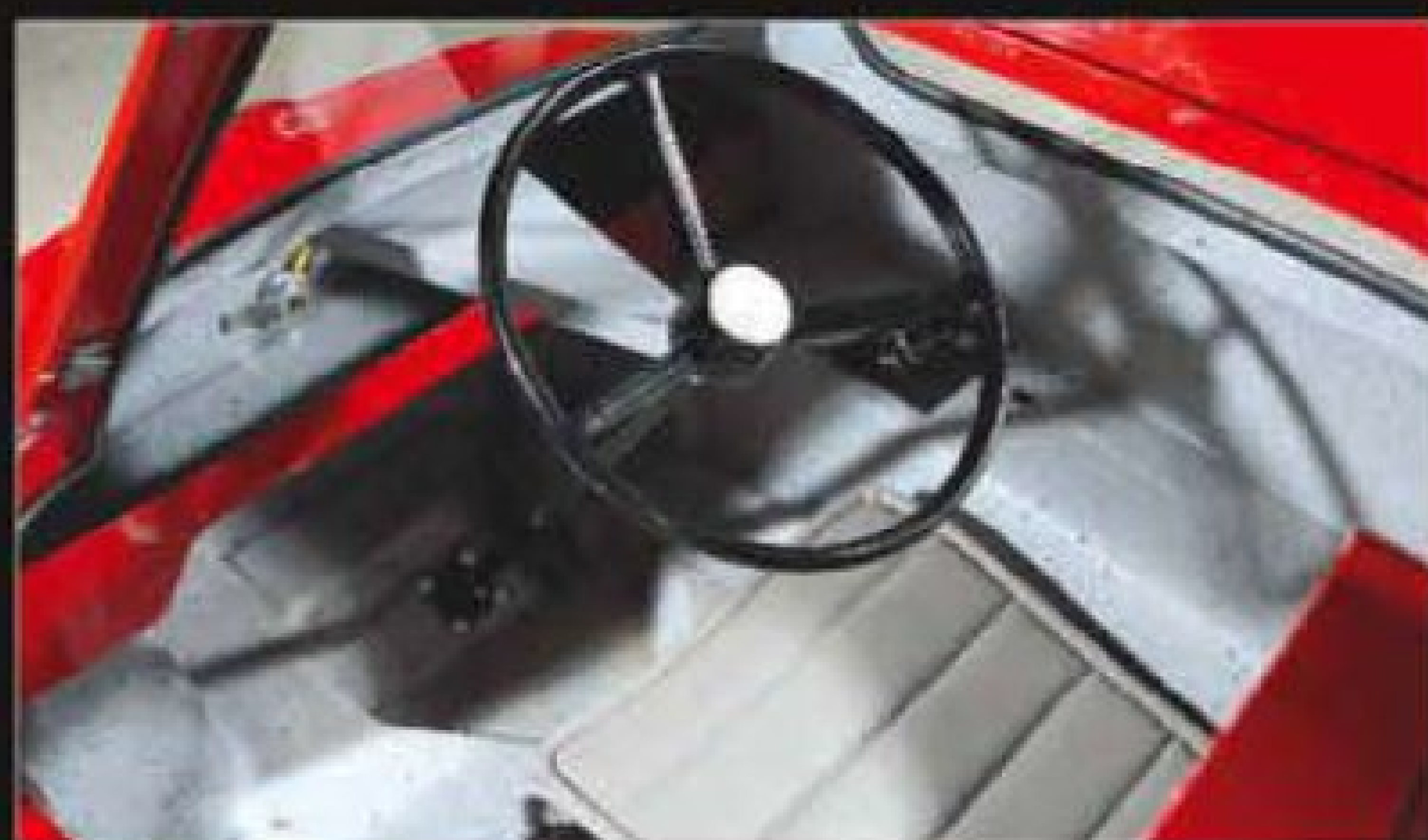
Cabin is as basic as they come, with bare glassfibre on show
