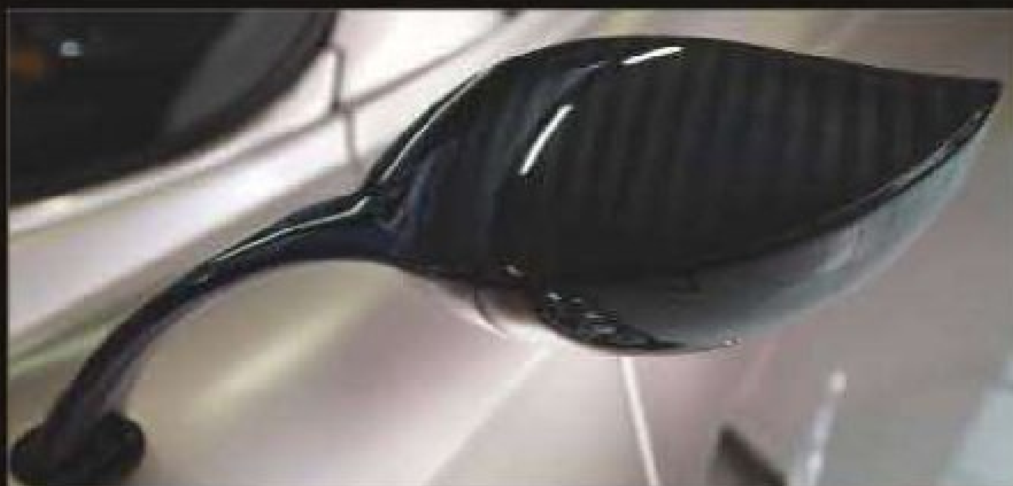
Above: new seats offer better support than Zonda's. Below: mirrors look delicate, but carbon construction makes them strong. Right: front flaps in raised position. Below right: wheels have a single central nut
