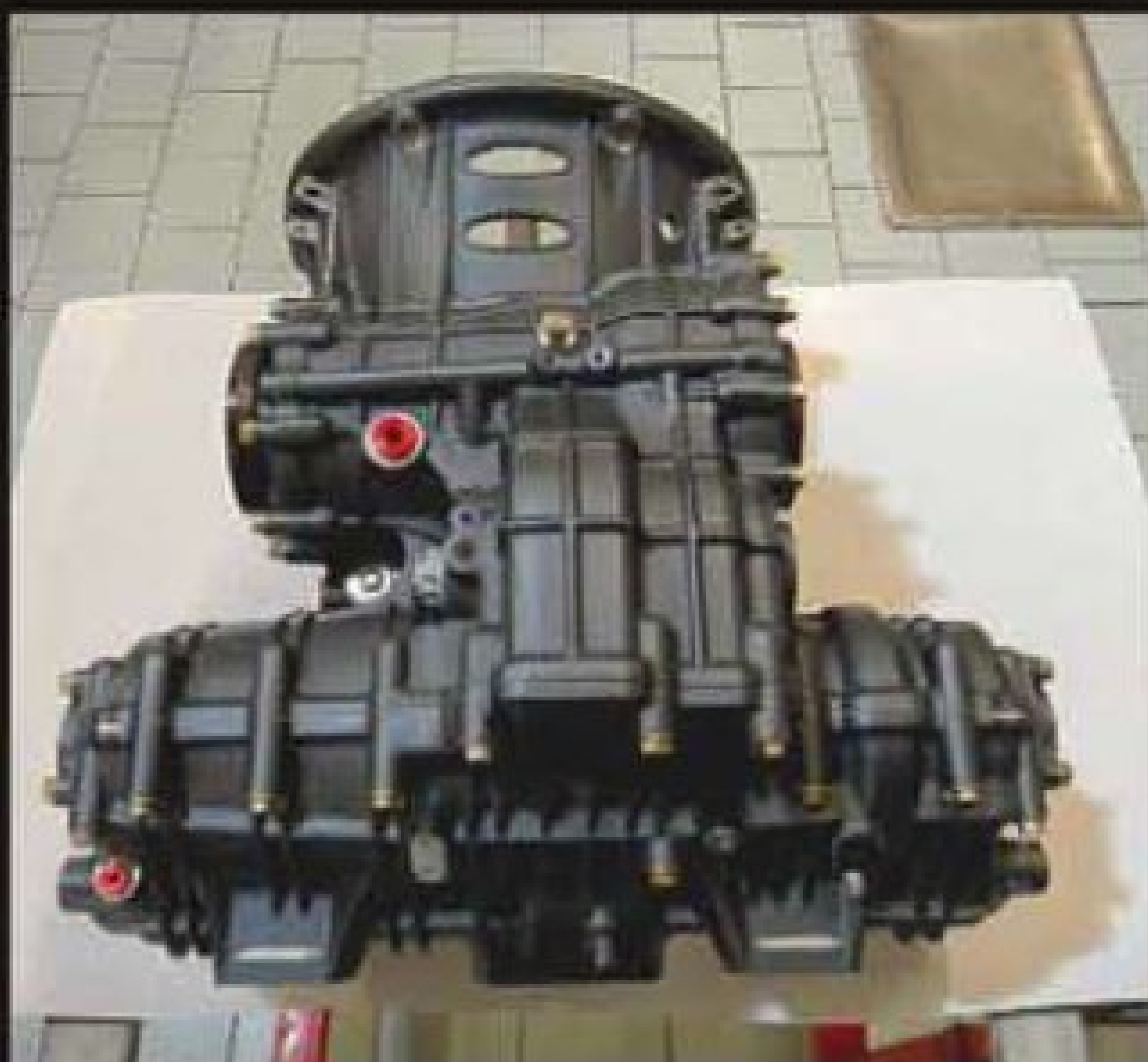
Top: Horacio talks aerodynamics. Right: rear view with flaps raised. Above: every bolt used on the car is titanium. Below: Xtrac gearbox is a transverse unit, offering better weight distribution
