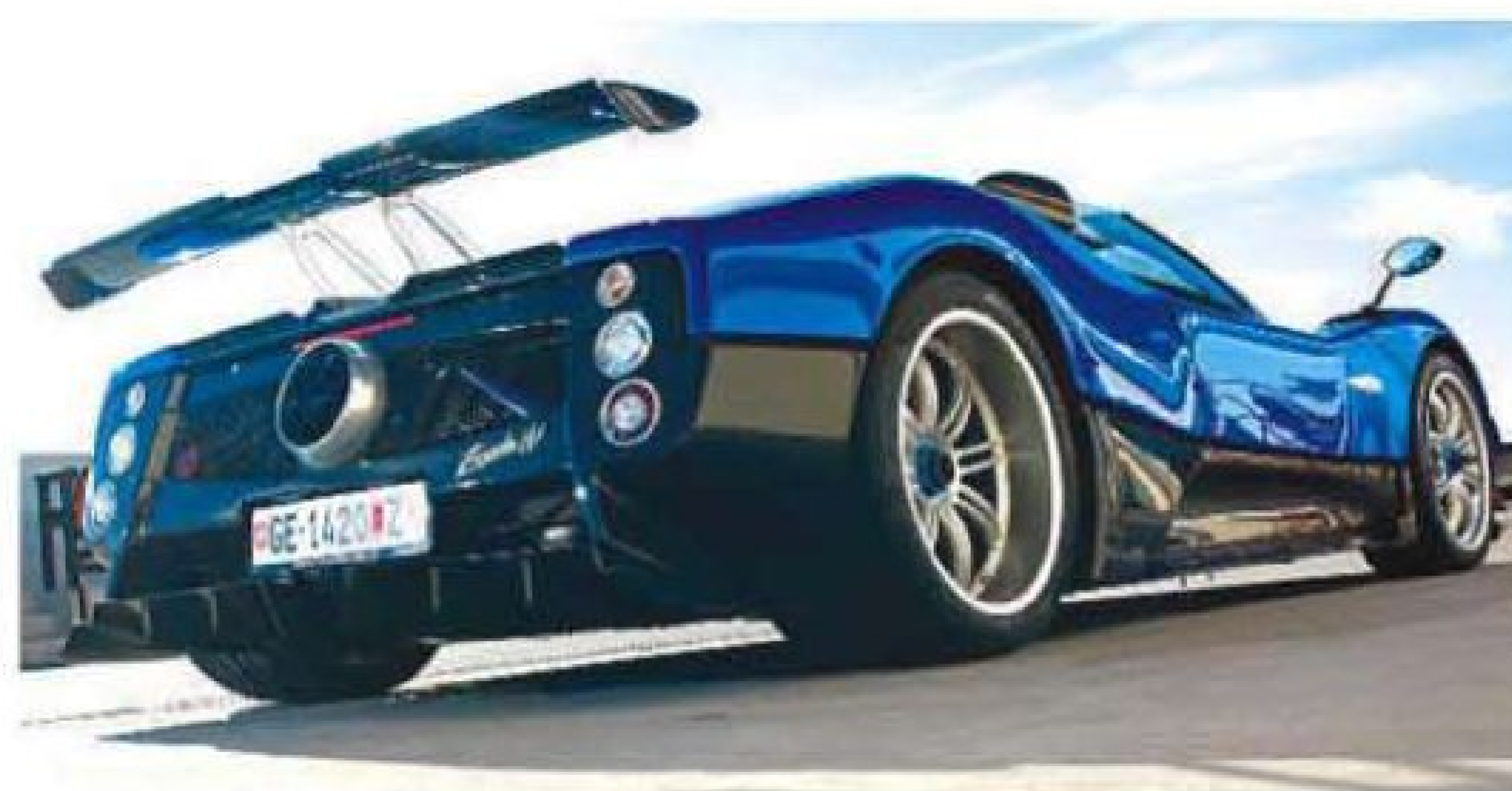
Above left: V12 is the 669bhp unit from the Cinque, but it's mated to a manual gearshift (above). Left: large rear diffuser and spoiler are also from the Cinque; car wears unique 'Zonda HH' badges
