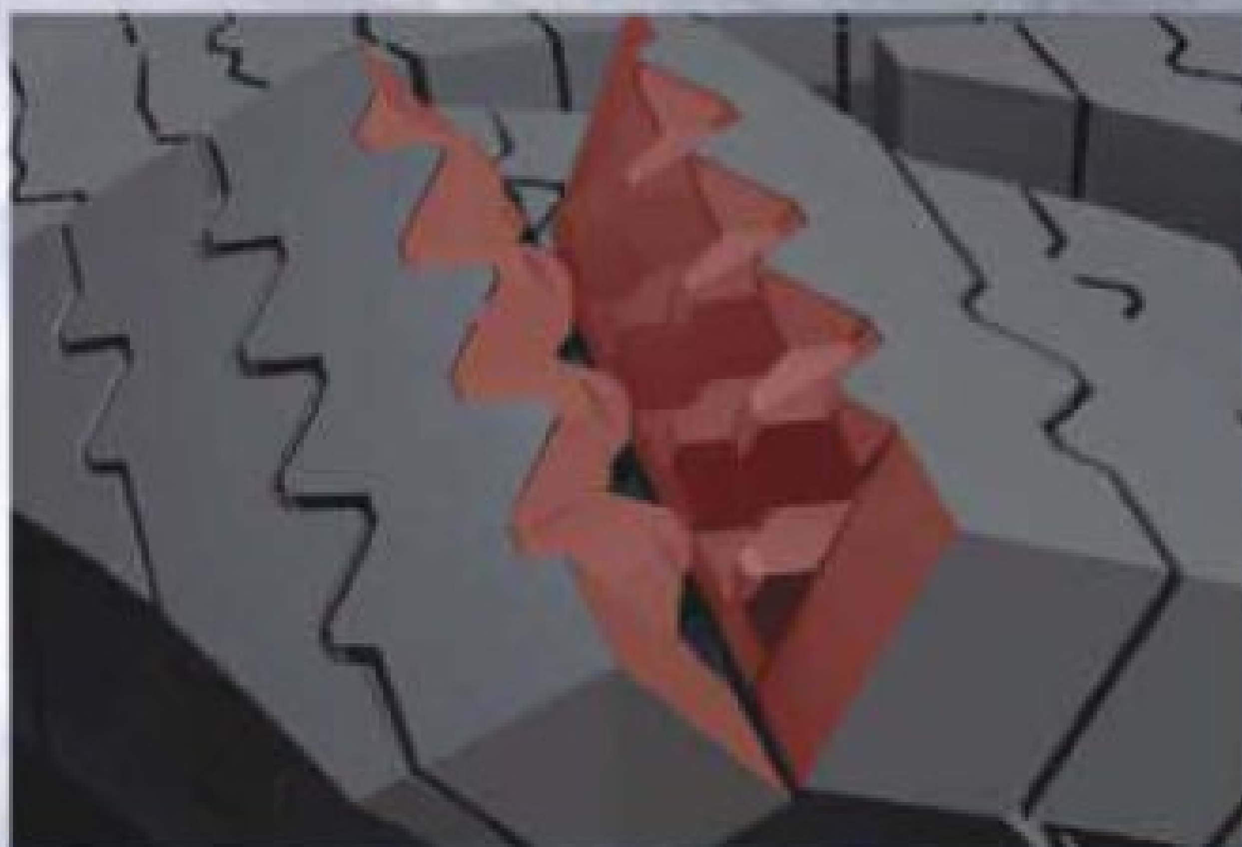
Sipes cover the tread blocks (right) and have a complex 3D cut (above)
