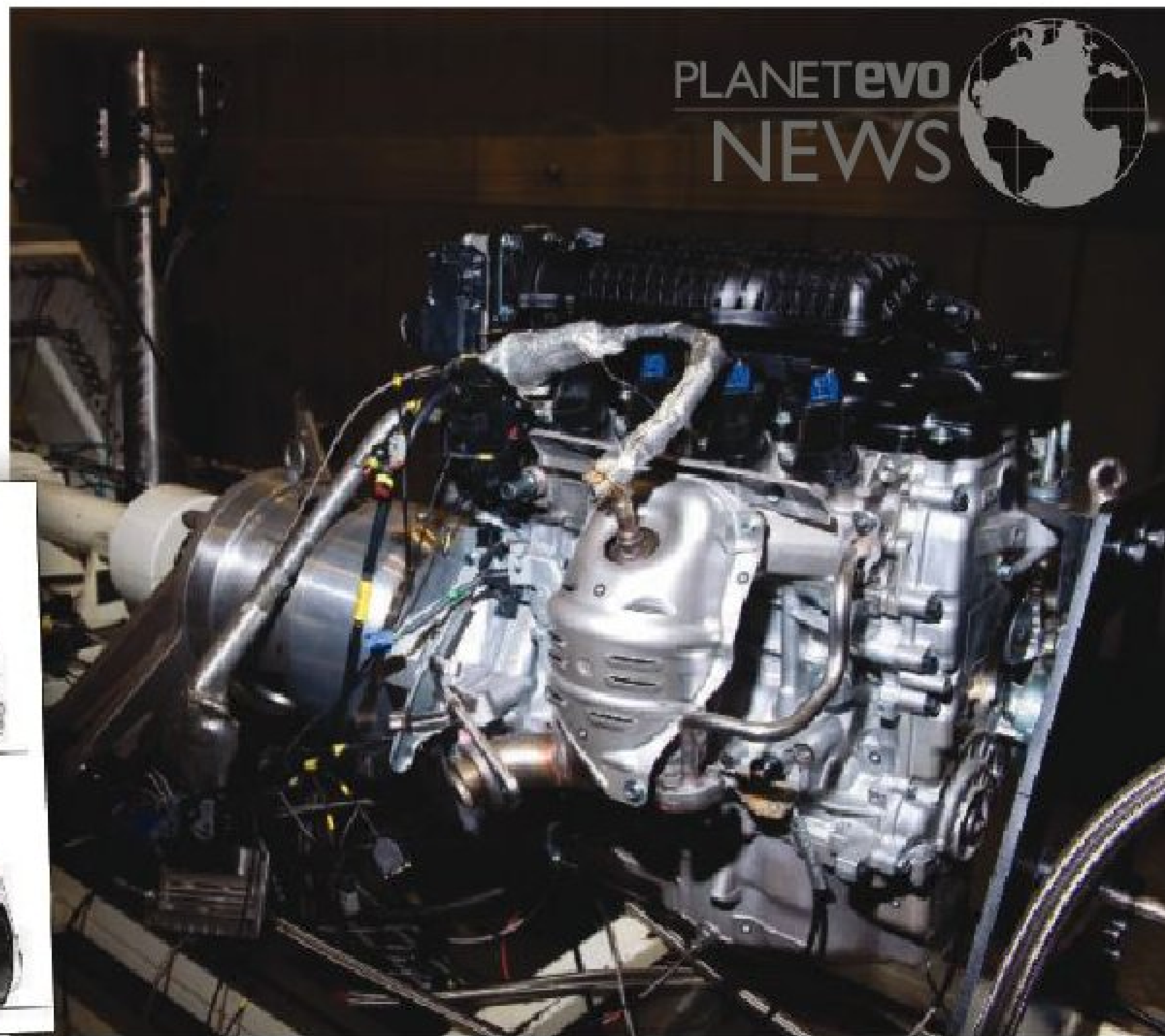
Above: concept takes shape in the Mugen workshop. Right: engine will do 20,000km on test bed. Below: concept renderings
