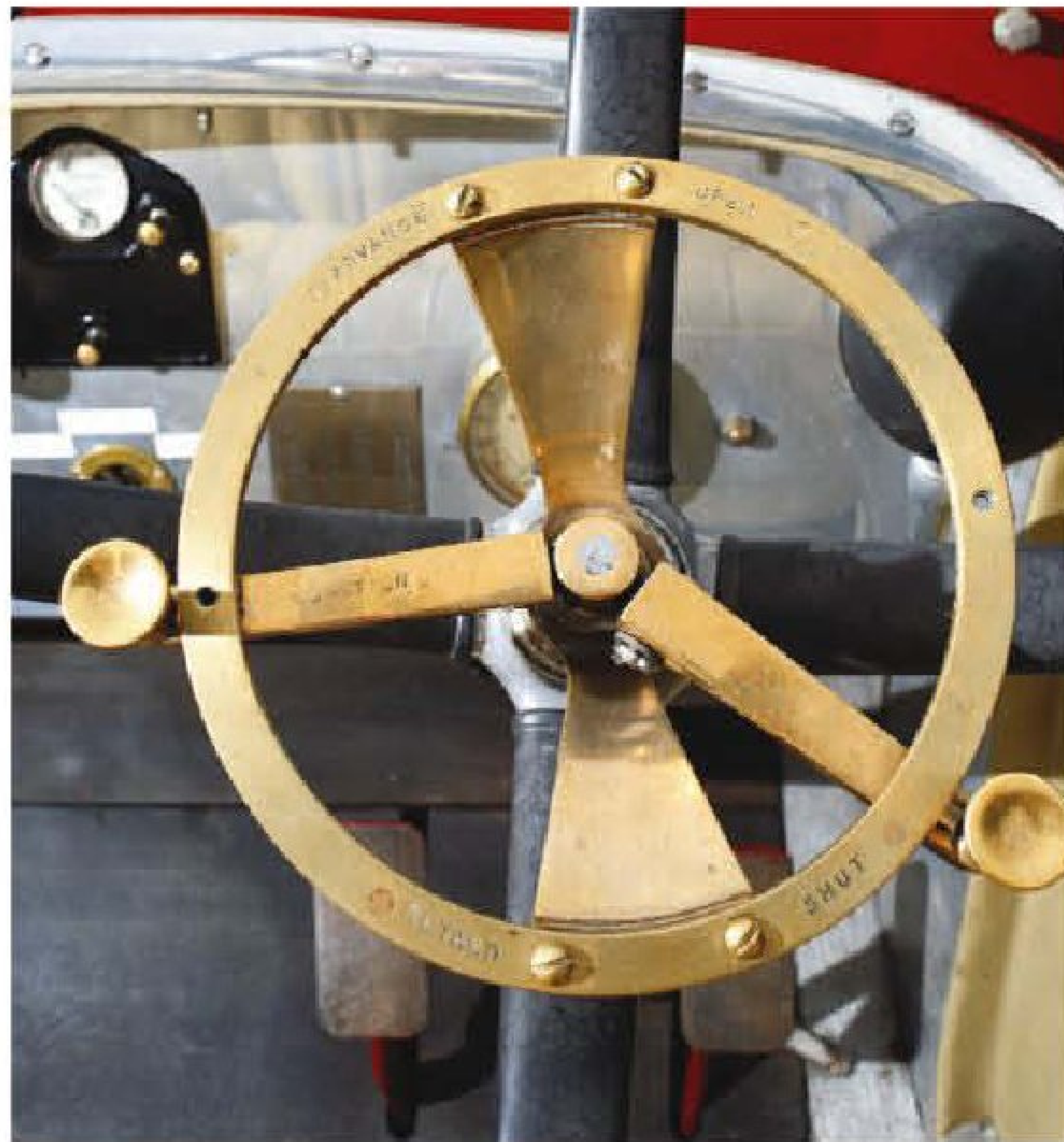
Above: mounted in the centre of the steering wheel is a hand throttle (on the right) and an ignition advance/retard control. Left: manoeuvring the Prince Henry into position for its run up the Shelsley Walsh hillclimb. Right: Catchpole powers up the famous track
