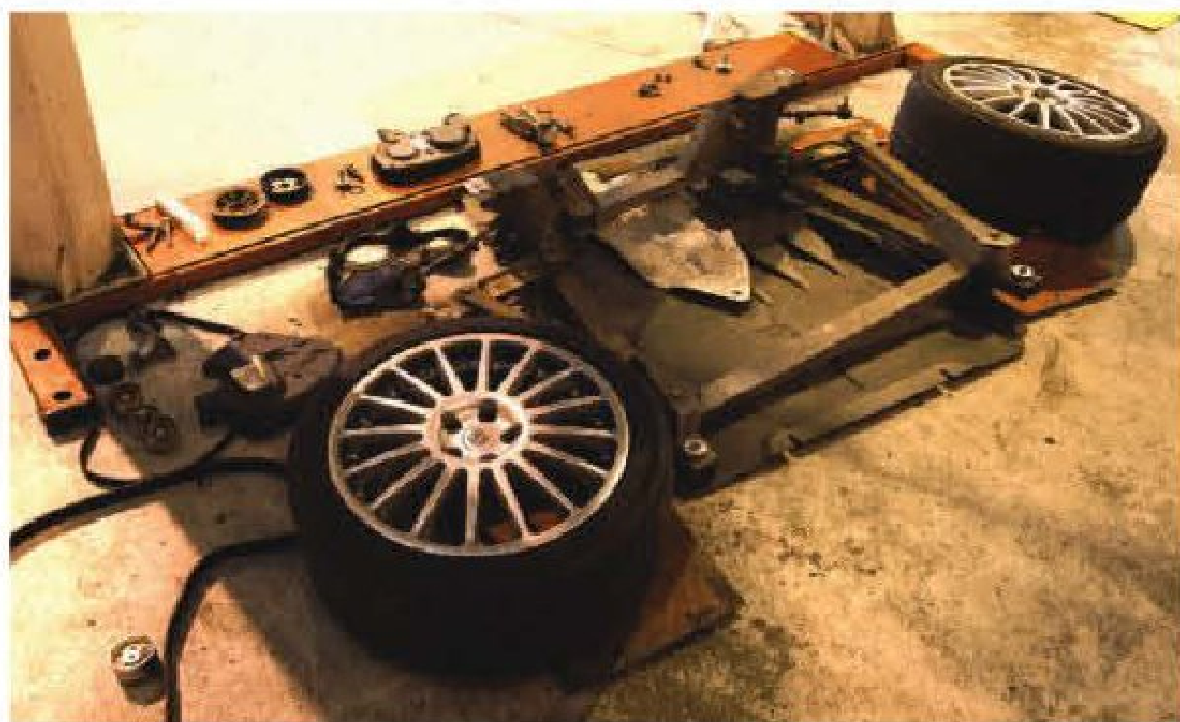
Above: Clio's rear subframe rests between the rear wheels. Right: timing belt idlers and the timing belt tensioner surrounded by the new accessories belt (left) and timing belt (right)
