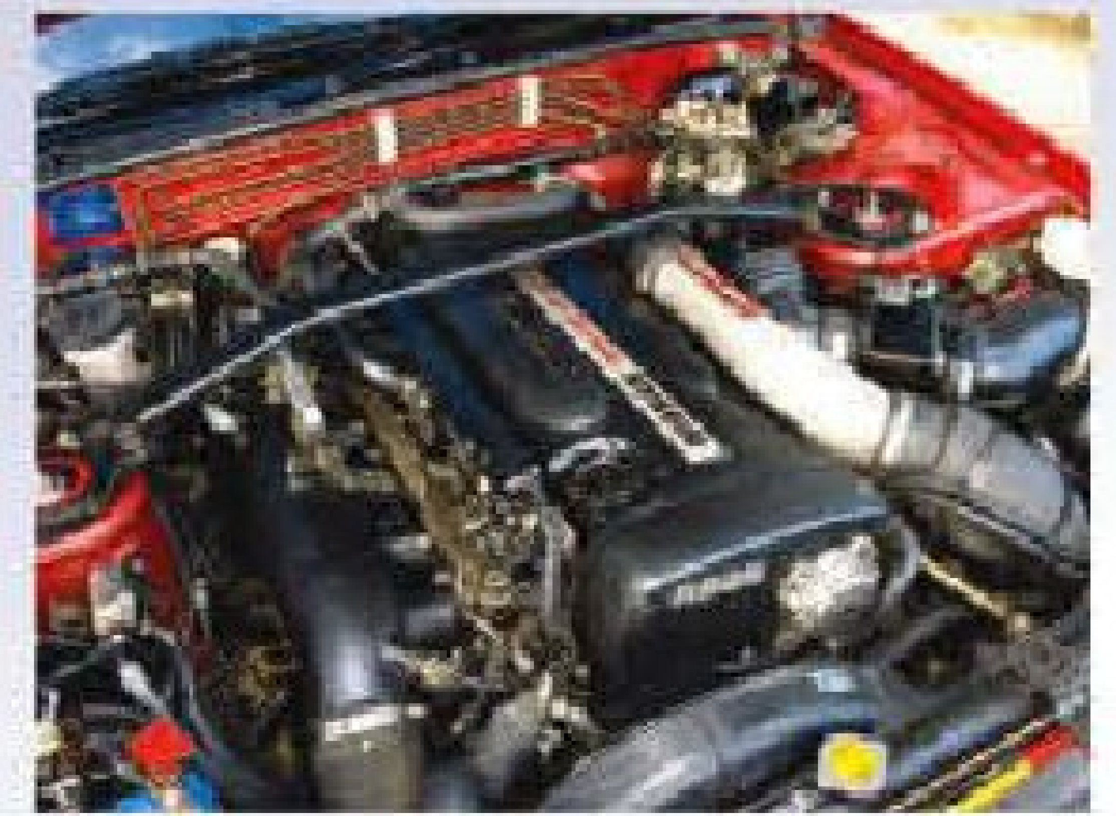
Left: Maserati's V6 displaces just 2 litres, but a pair of turbos takes its output to 330bhp. Above: R32's twin-turbo in-line six was rated at 276bhp in factory spec – but few stayed that way
