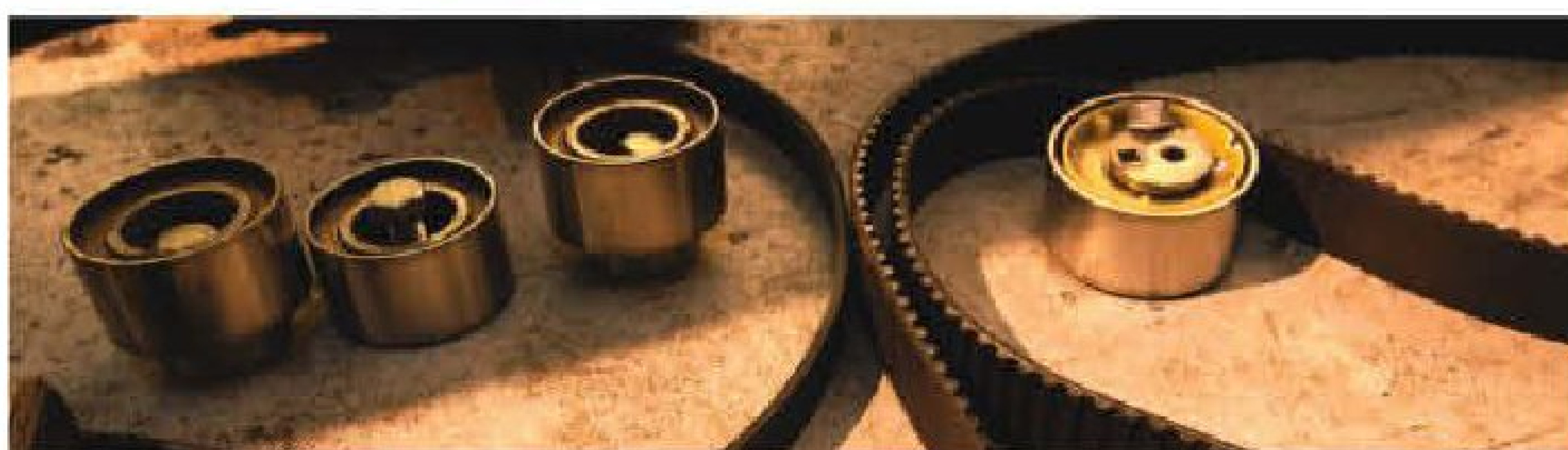
Above: Clio's rear subframe rests between the rear wheels. Right: timing belt idlers and the timing belt tensioner surrounded by the new accessories belt (left) and timing belt (right)
