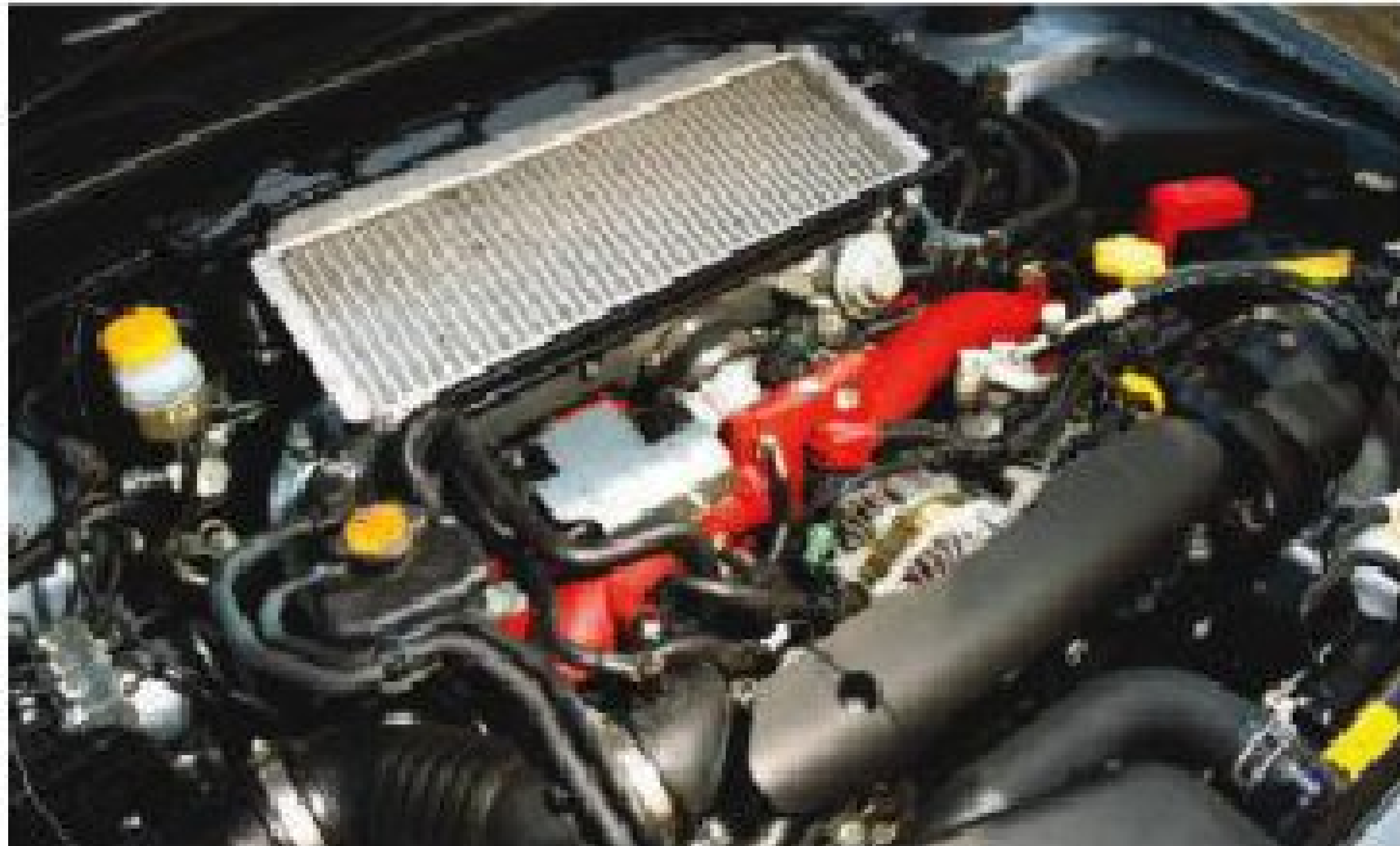
RB5 (above) runs a 2-litre turbo flat-four with 237bhp; STI's engine (below) has 2.5 litres and another 59bhp. The newer car's extra mass means power-to-weight ratios are similar, though: 195bhp/ton for the RB5, 200 for the STI
