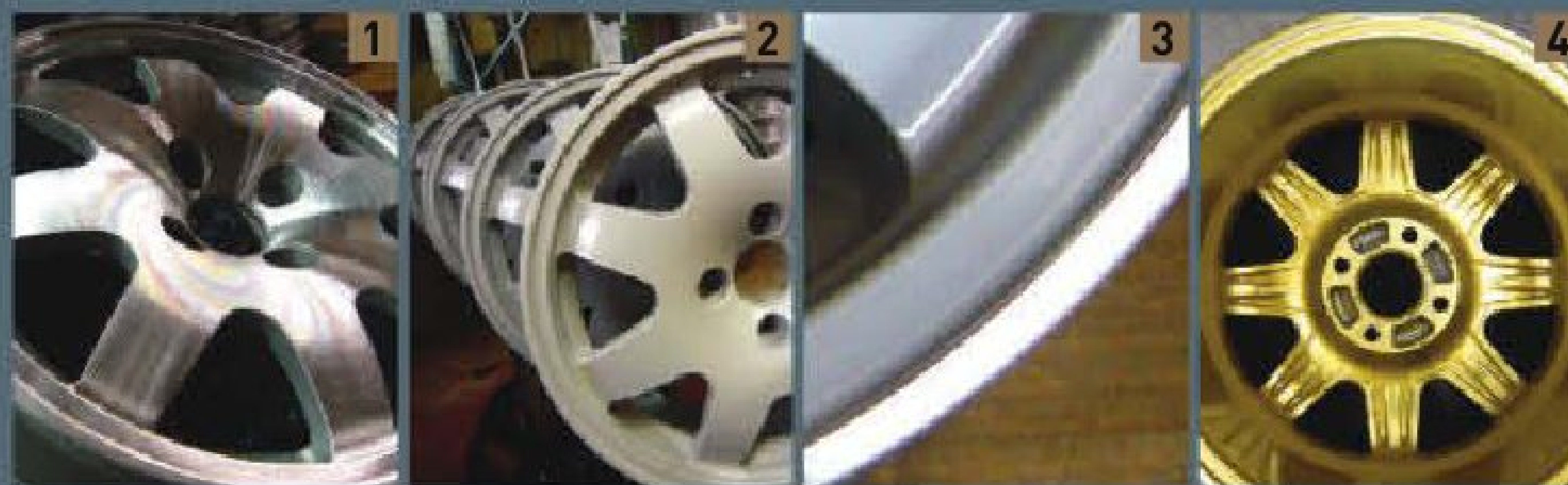
The Clio's wheels at various stages during the refurb: 1) stripped back to bare alloy, 2) powder primed, 3) lip reinstated, 4) gold applied
