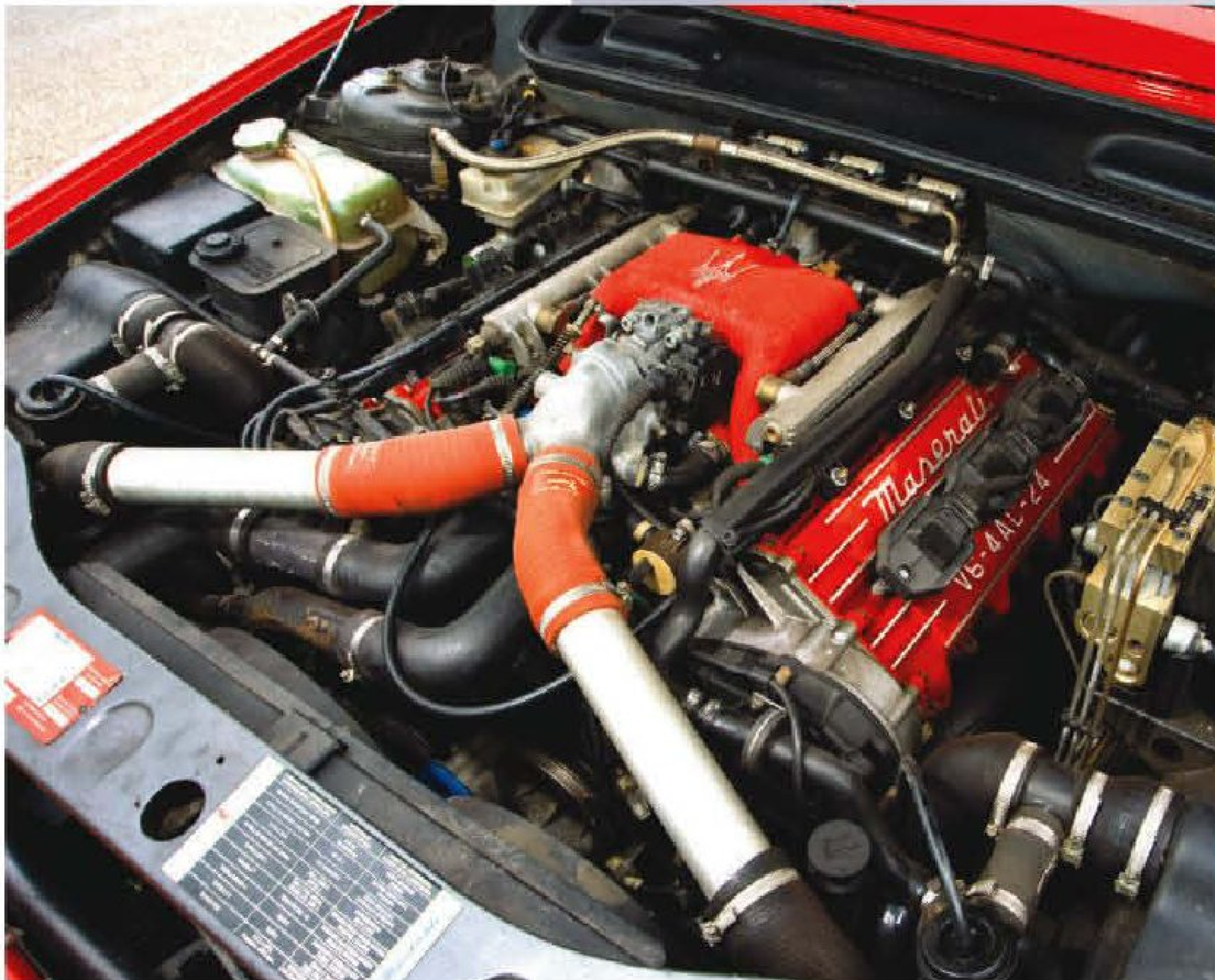
Left: Maserati's V6 displaces just 2 litres, but a pair of turbos takes its output to 330bhp. Above: R32's twin-turbo in-line six was rated at 276bhp in factory spec – but few stayed that way
