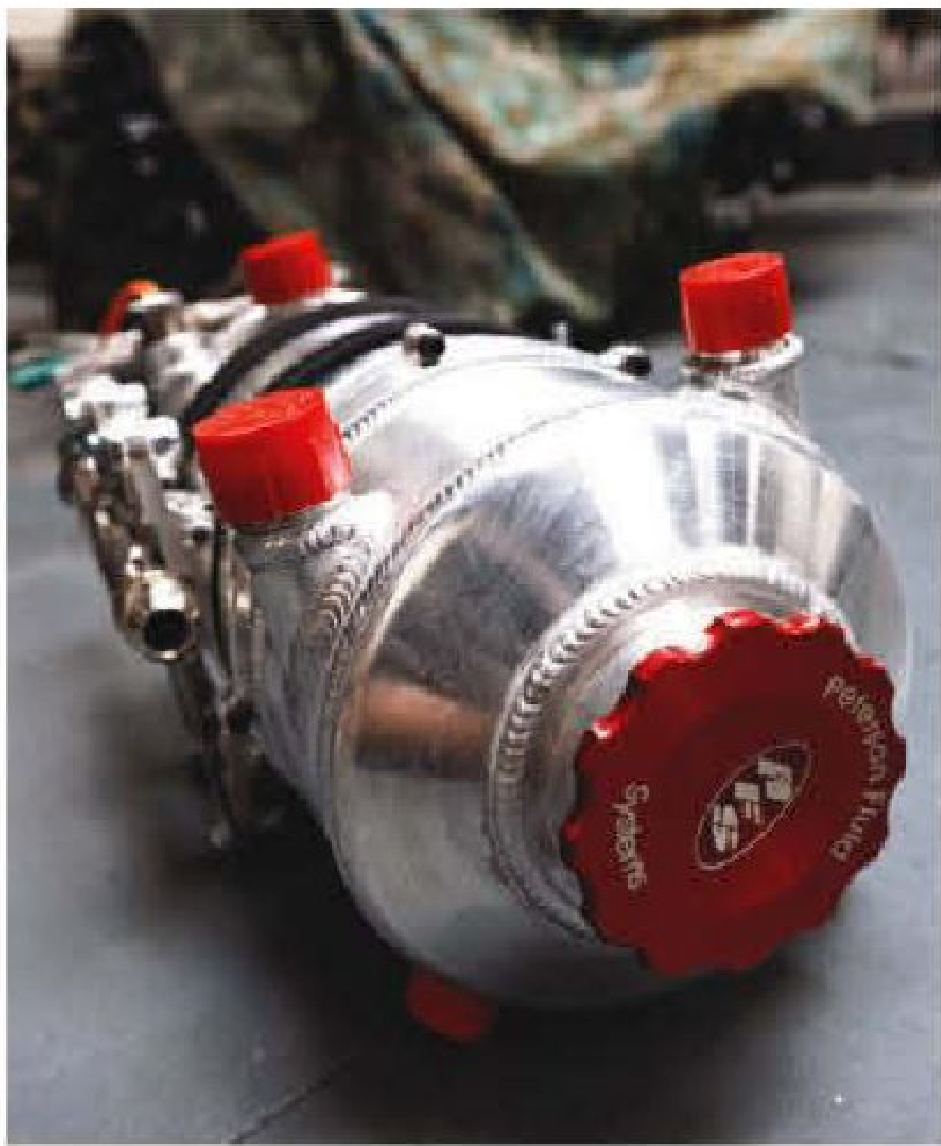
Right: Andy beside Red Victor 3's new carbon and glassfibre body, currently part-way through the painting process. Above: 1.5-gallon oil tank for the dry sump system came from Peterson Fluid Systems in Colorado. Below: 8.8-litre Chevrolet iron block is the only part of the engine carried over unchanged from Red Victor's previous incarnation
