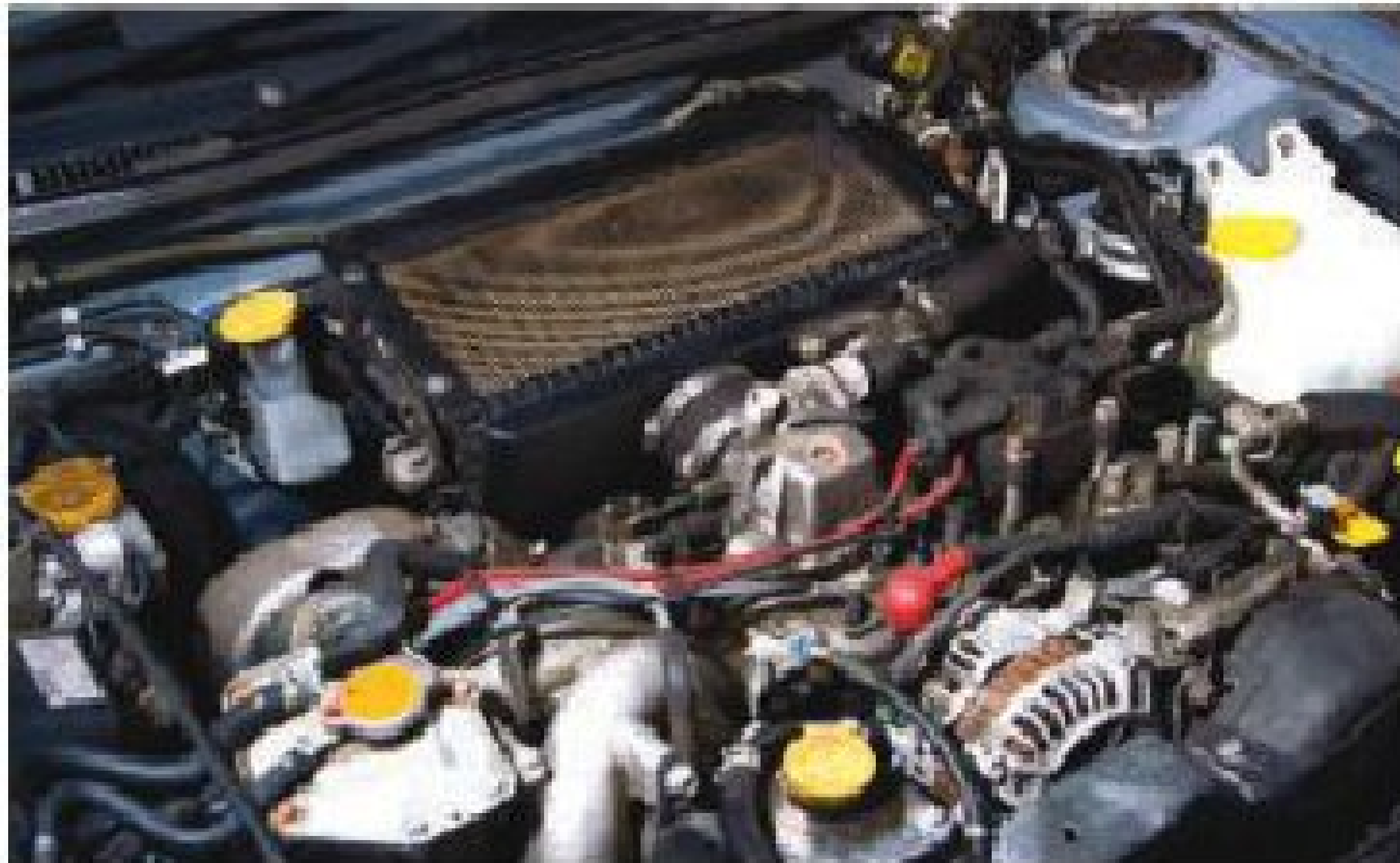
RB5 (above) runs a 2-litre turbo flat-four with 237bhp; STI's engine (below) has 2.5 litres and another 59bhp. The newer car's extra mass means power-to-weight ratios are similar, though: 195bhp/ton for the RB5, 200 for the STI
