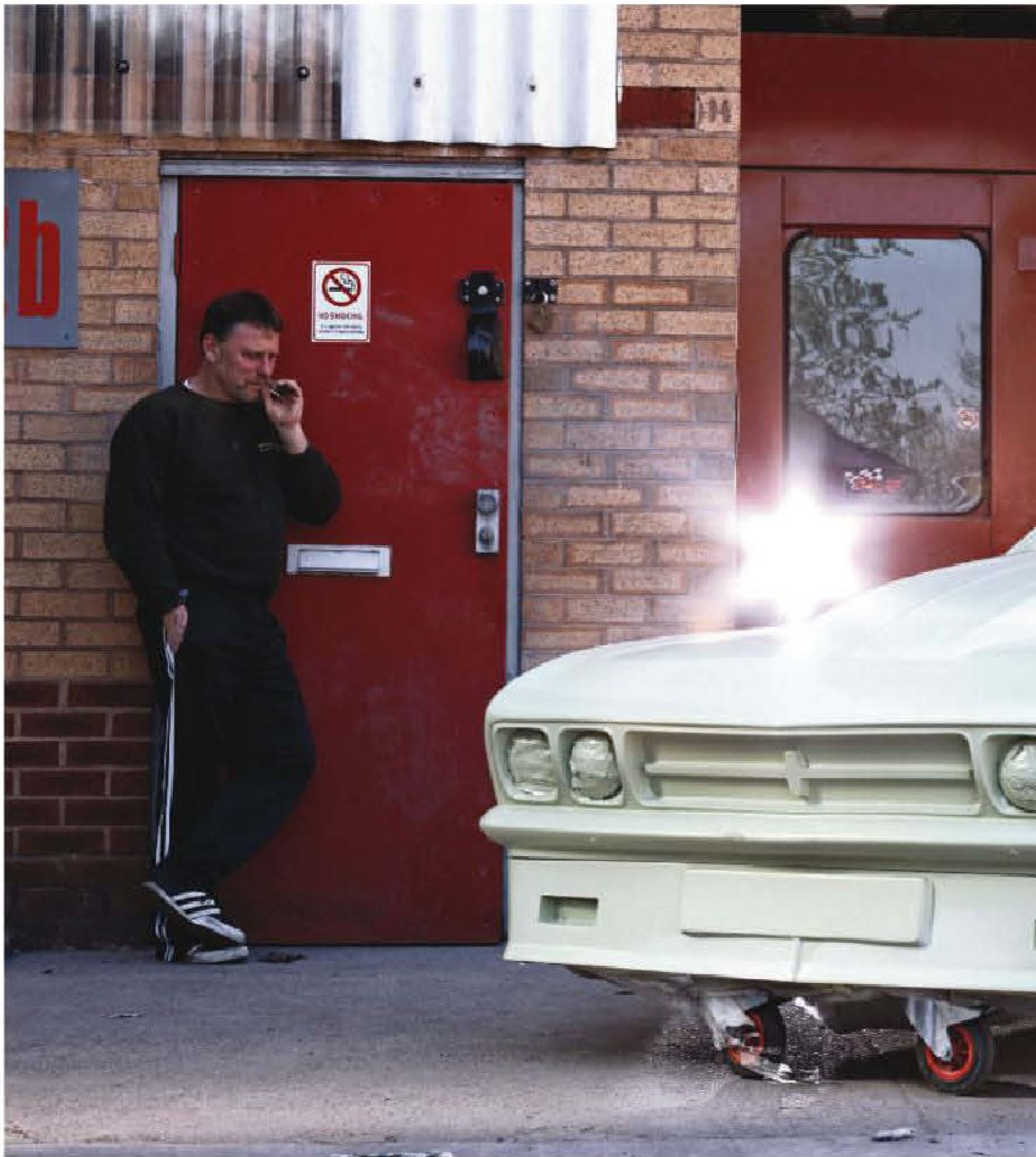
Right: Andy beside Red Victor 3's new carbon and glassfibre body, currently part-way through the painting process. Above: 1.5-gallon oil tank for the dry sump system came from Peterson Fluid Systems in Colorado. Below: 8.8-litre Chevrolet iron block is the only part of the engine carried over unchanged from Red Victor's previous incarnation
