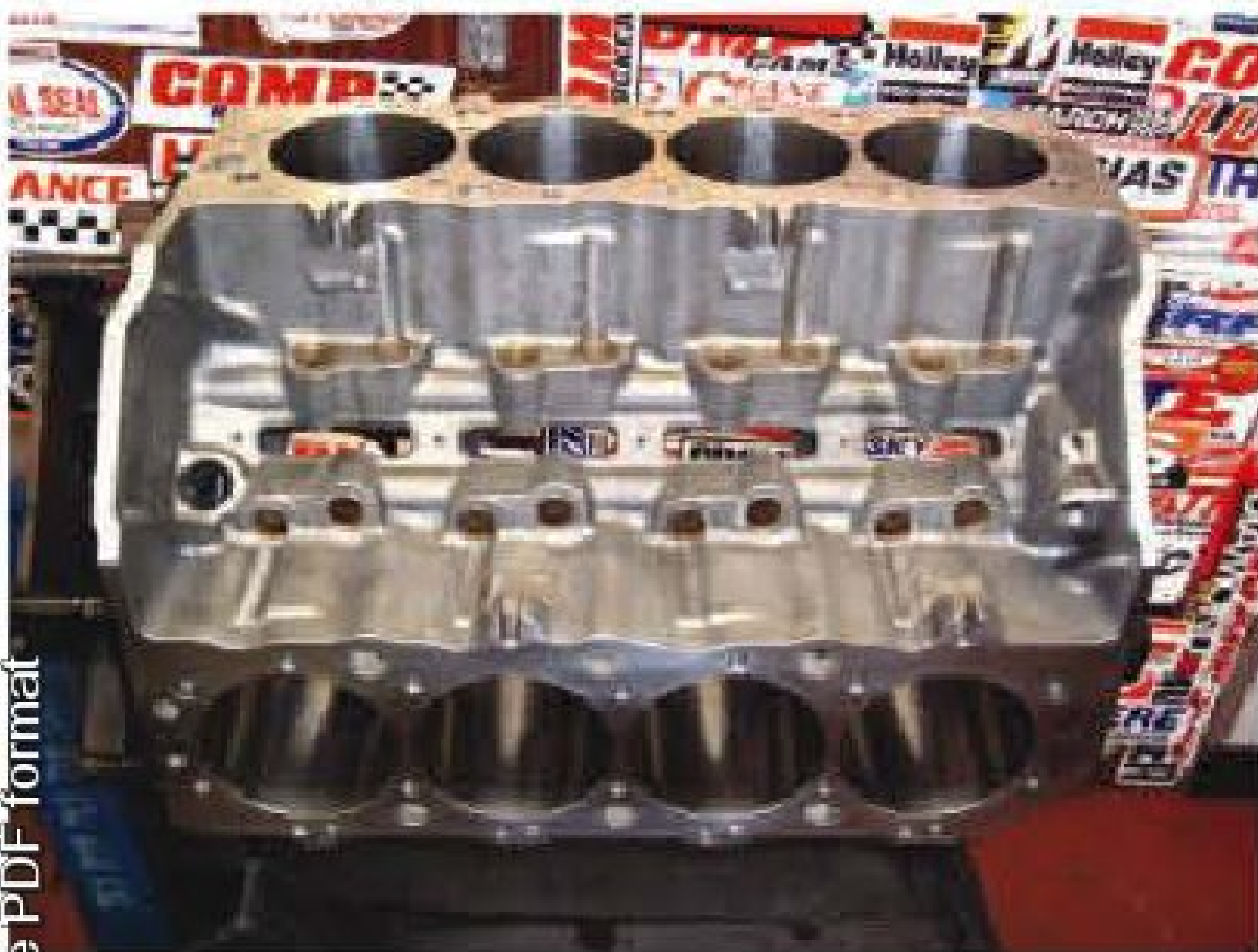
Right: Andy beside Red Victor 3's new carbon and glassfibre body, currently part-way through the painting process. Above: 1.5-gallon oil tank for the dry sump system came from Peterson Fluid Systems in Colorado. Below: 8.8-litre Chevrolet iron block is the only part of the engine carried over unchanged from Red Victor's previous incarnation
