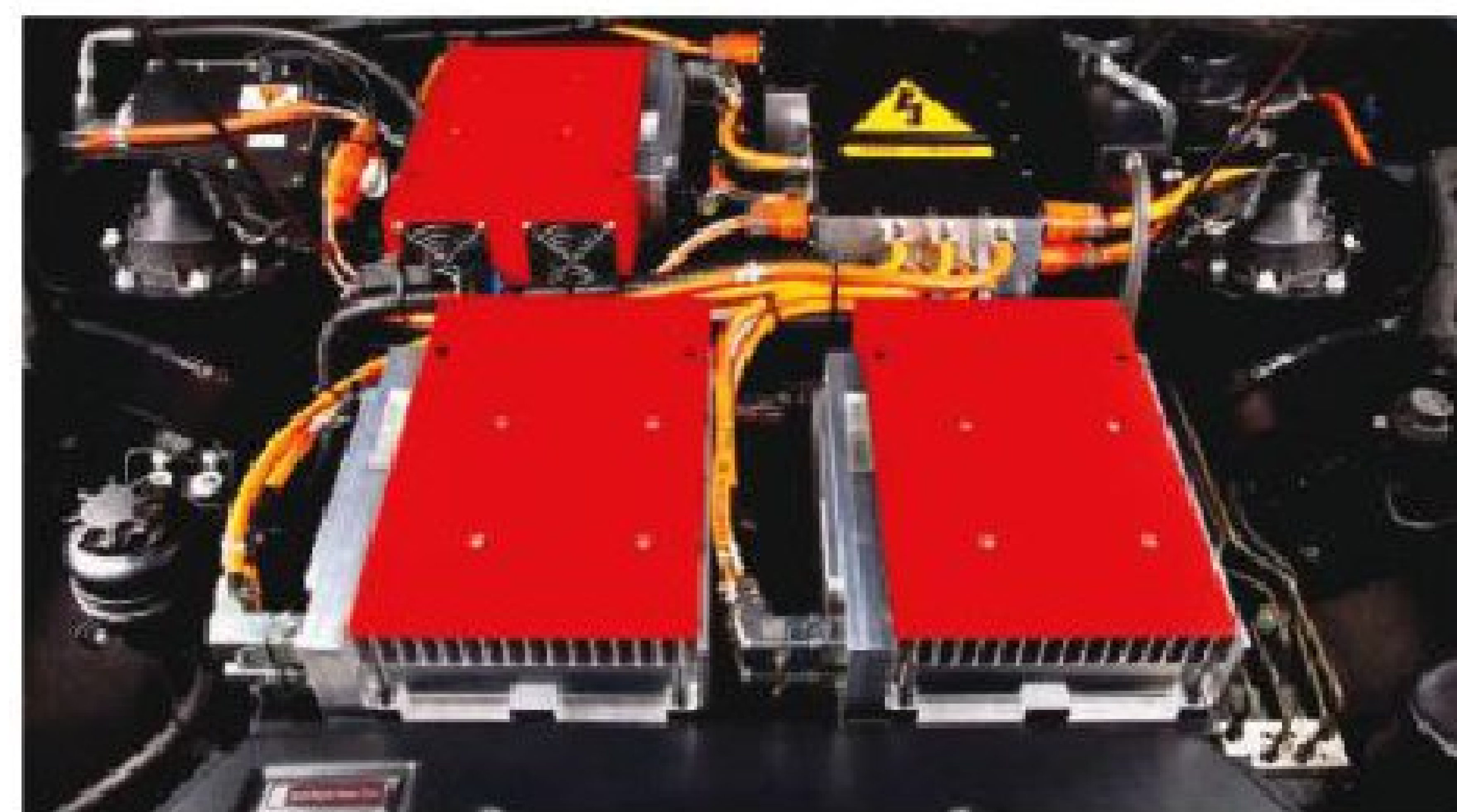
Above: trio of charging packs sits above the batteries
