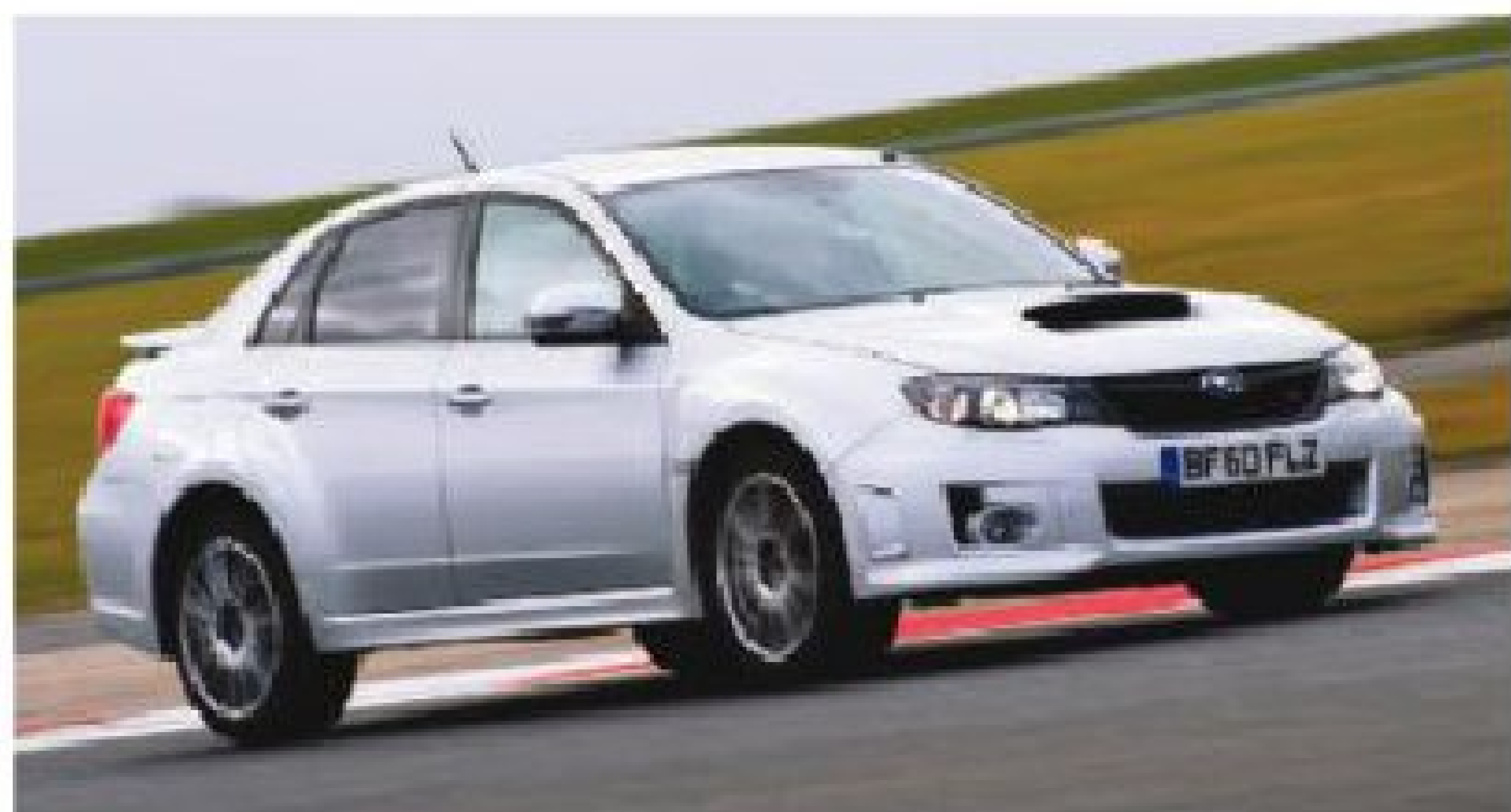
RB5 (above) runs a 2-litre turbo flat-four with 237bhp; STI's engine (below) has 2.5 litres and another 59bhp. The newer car's extra mass means power-to-weight ratios are similar, though: 195bhp/ton for the RB5, 200 for the STI
