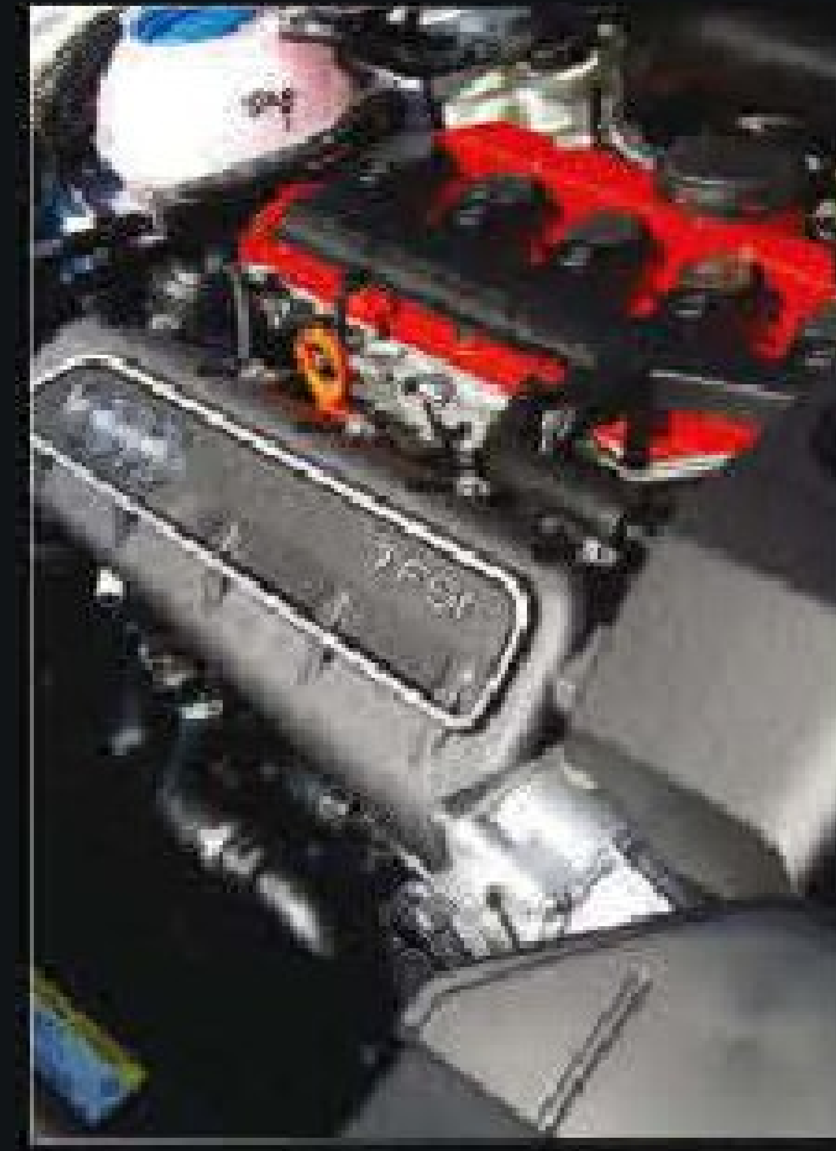
Audi Quattro concept (bottom left) features the acclaimed 2.5-litre five-cylinder turbo engine from the TT RS (left). If the car makes production – as seems likely – this arrangement should remain
