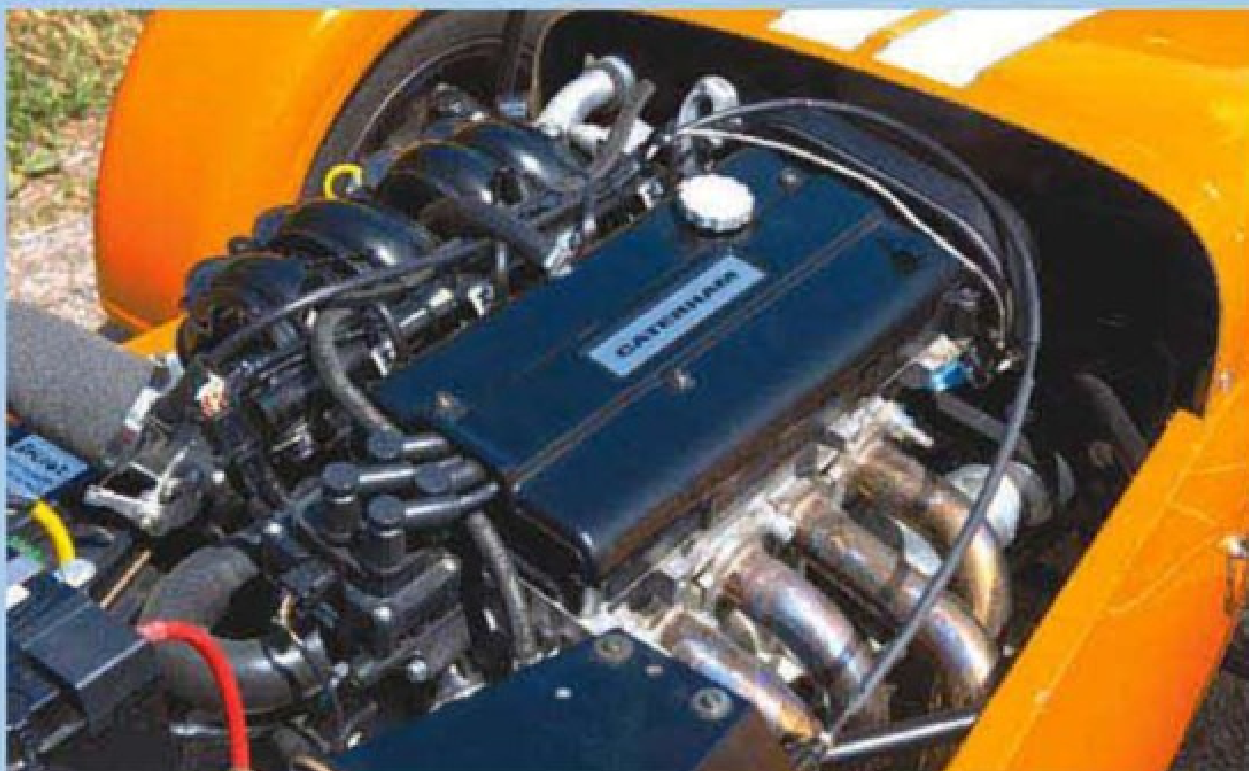
Left: Supersport's front-mounted 1.6-litre Duratec unit puts out 140bhp, giving a power-to-weight ratio of 273bhp/ton. Below left: Club Racer's mid-mounted 1.6-litre Toyota engine is shared with the standard Elise; peak power is 134bhp, but power-to-weight is down at 160bhp/ton
