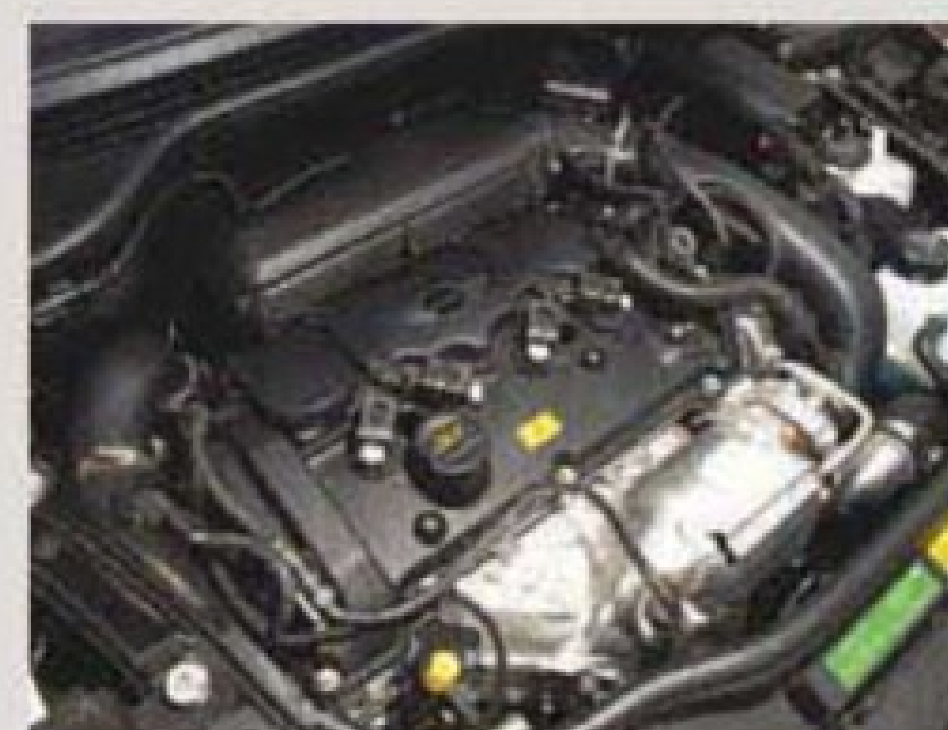
Left: turbo 1.6-litre engine gains 17bhp and 31lb ft with the Superchips upgrade
