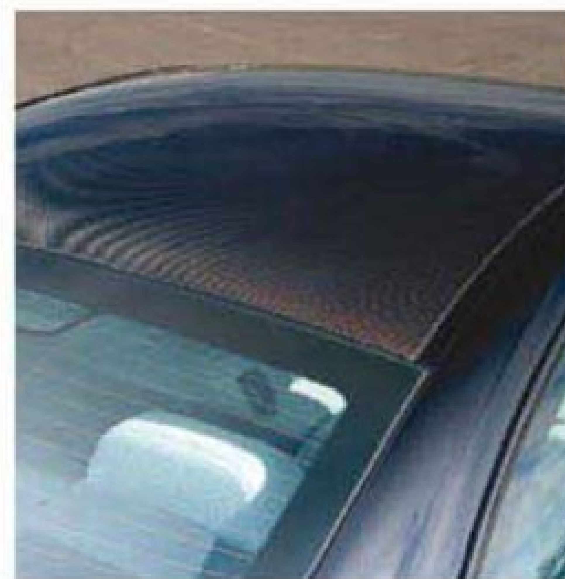
Above: carbon roof can leak. Below: quality of the shifts from the SMG gearbox can be improved with software updates. Bottom: well-equipped cabin got a head-up display as standard
