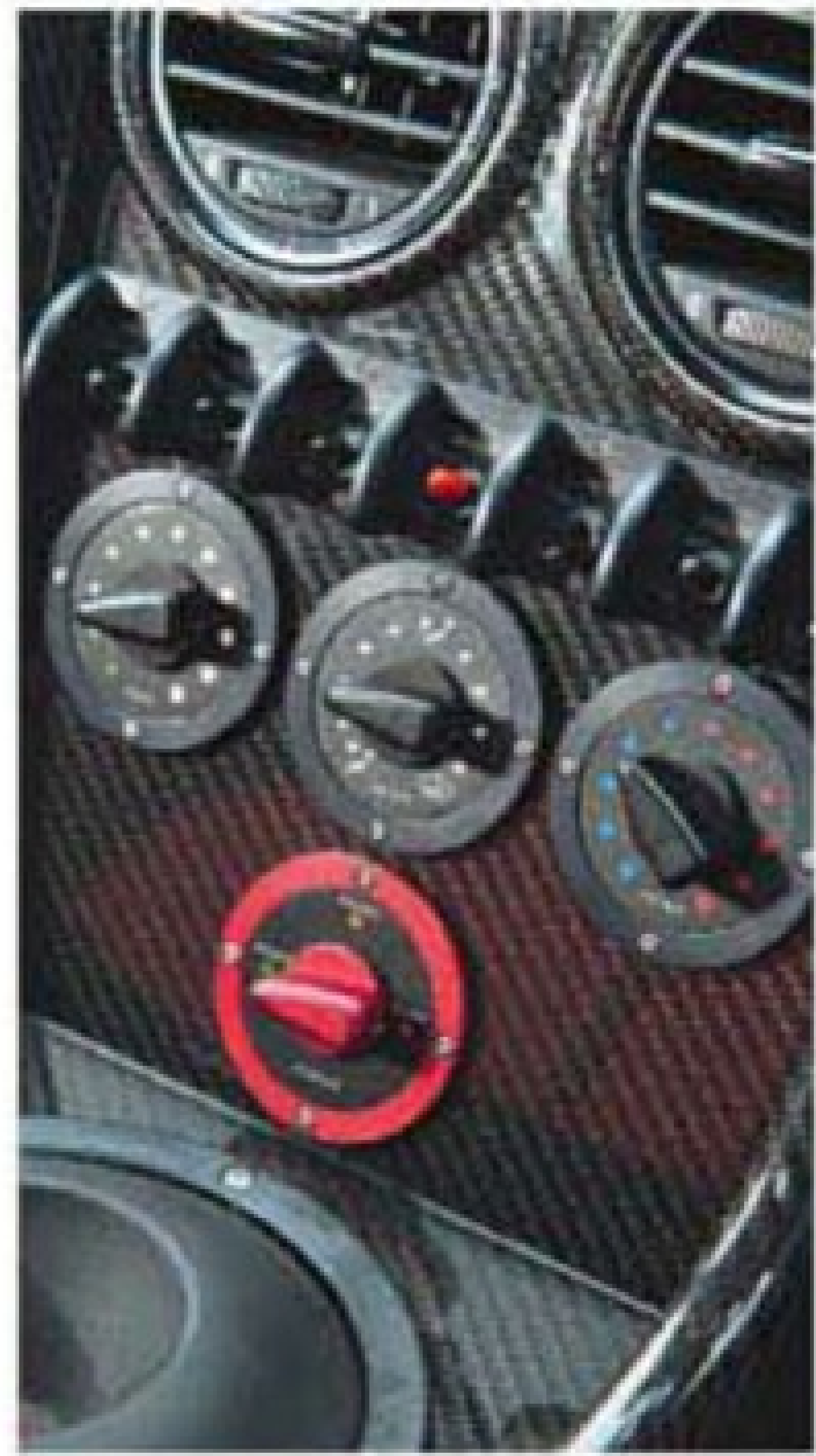
Red dial in Noble turns the wick up from 450 to 550 to 650bhp. Below: 12C's alloys look skeletal next to M600's
