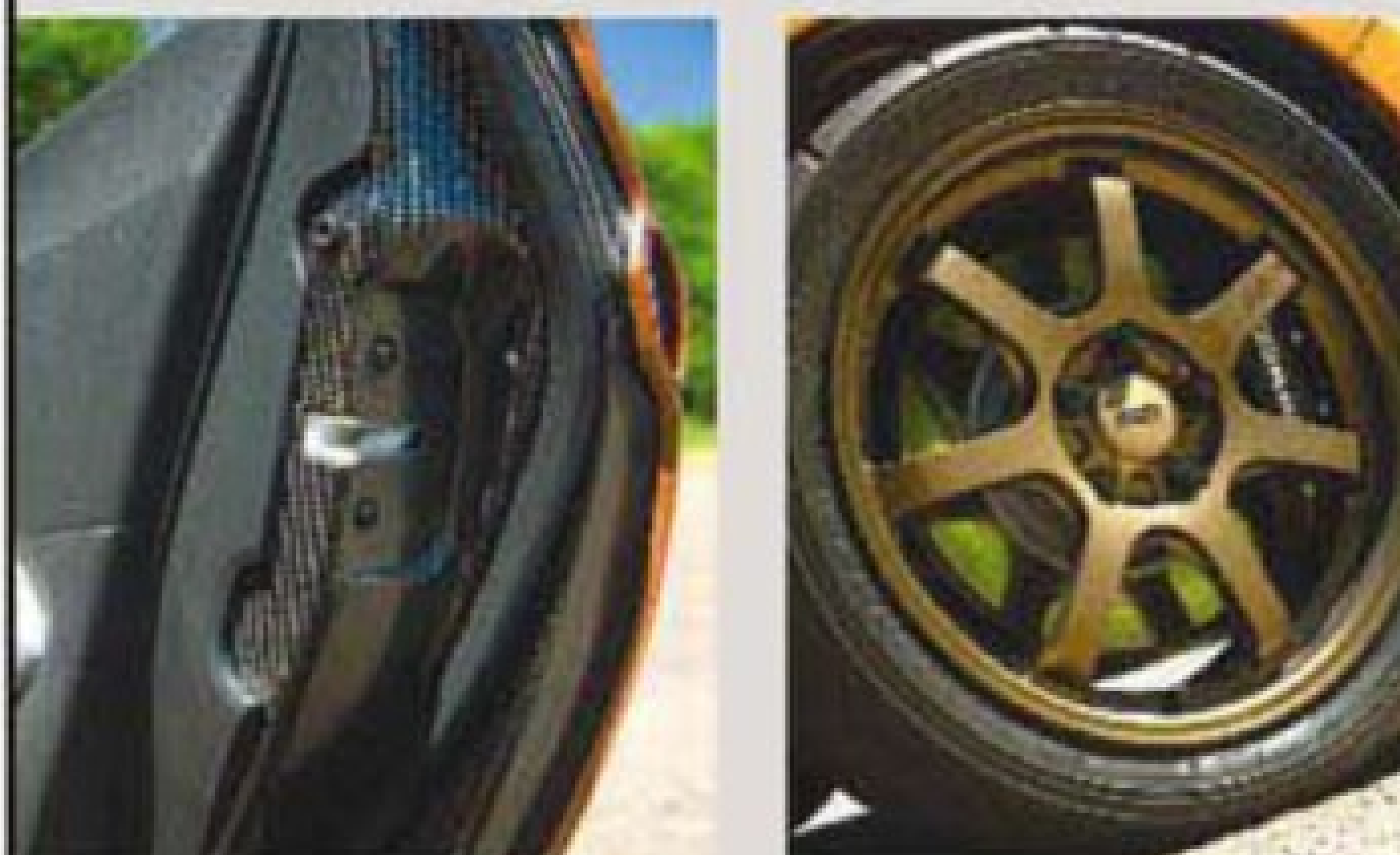
Left: carbonfibre door helps cut weight. Lightweight GP wheel is actually an option on the regular CR-Z
