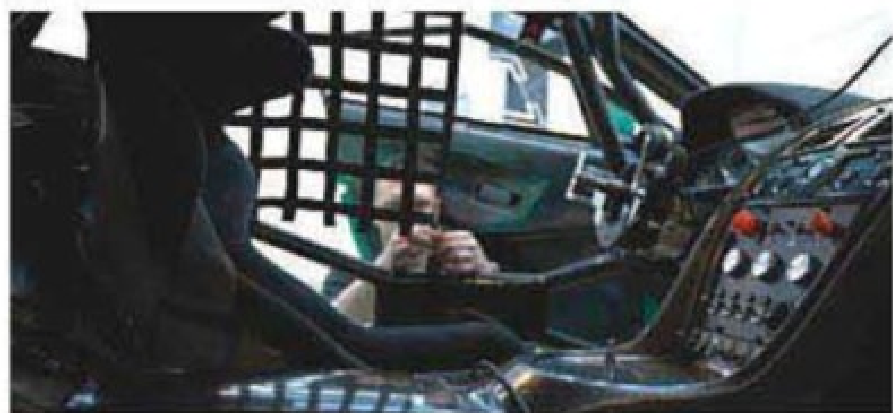
Above: combination of a roll-cage and the Zagato's smaller door aperture makes accessing the cockpit tricky. Below: race car's brakes use cast-iron discs to comply with VLN regs
