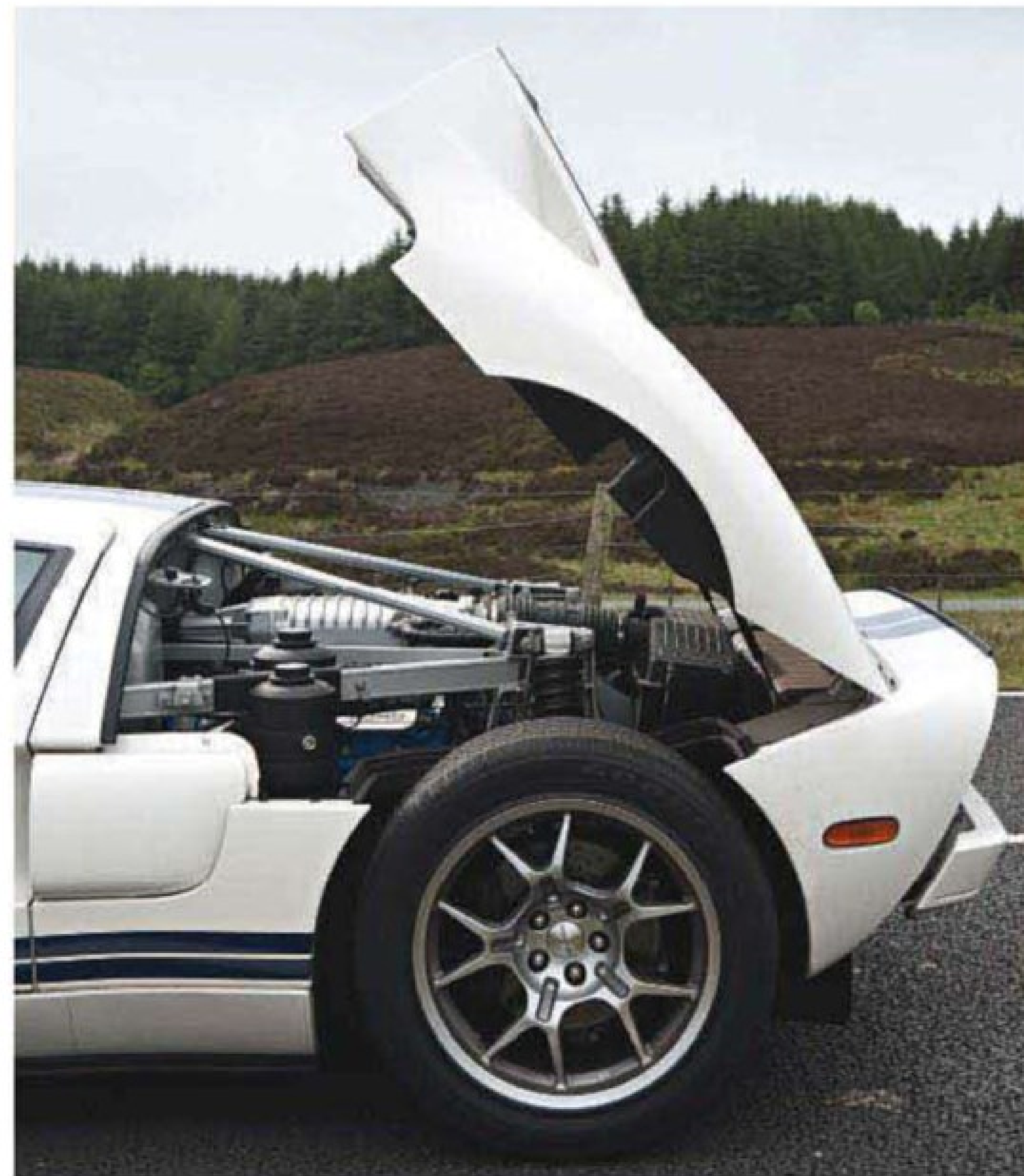
Top: Noble's twin-turbo 4.4-litre V8. Ford's supercharged 5.4-litre V8 can't match it for outright power (550bhp plays 650) but they're both compelling partners on these sort of roads
