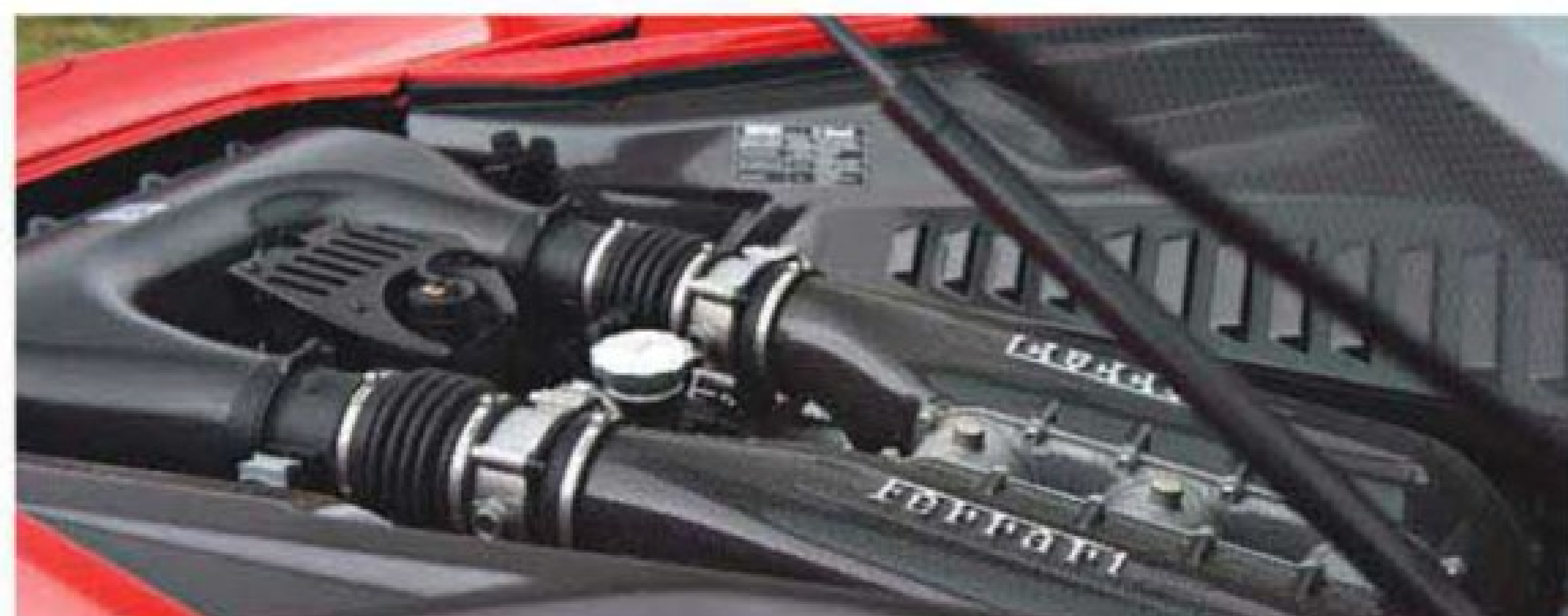
Above: Ferrari's normally aspirated 4.5-litre V8 produces 562bhp at a giddy 9000rpm. McLaren tops that with 592bhp at 7000rpm from its turbocharged 3.8-litre V8, though it can't match the 458's throttle response. Nor can it match the immediacy of its steering (left). The 12C's pace, though, is never in any doubt
