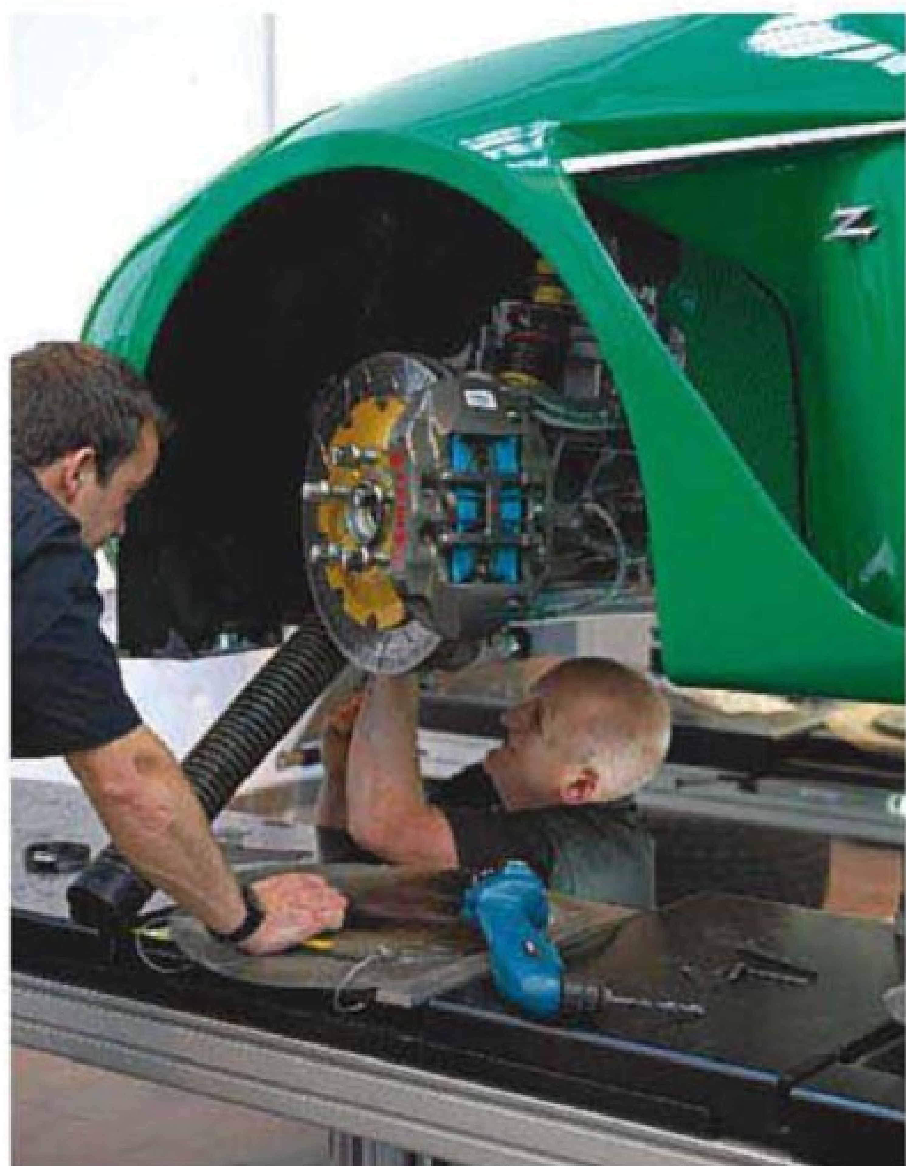
Above: combination of a roll-cage and the Zagato's smaller door aperture makes accessing the cockpit tricky. Below: race car's brakes use cast-iron discs to comply with VLN regs
