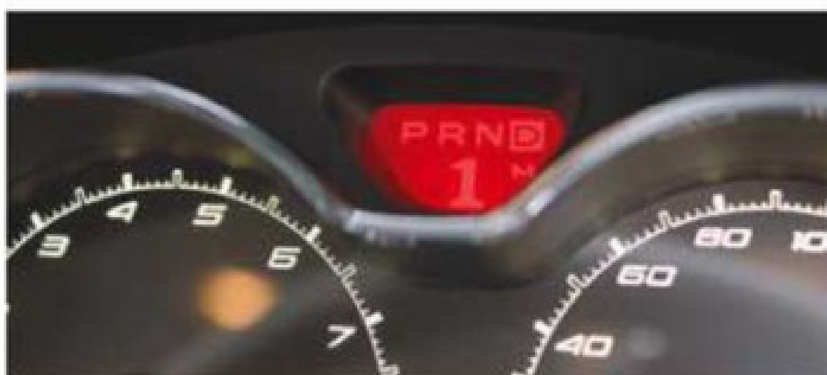
Above: readout shows what gear you're in, and whether you're in manual mode. Far right, no gear lever, just buttons and (above right) paddleshifters
