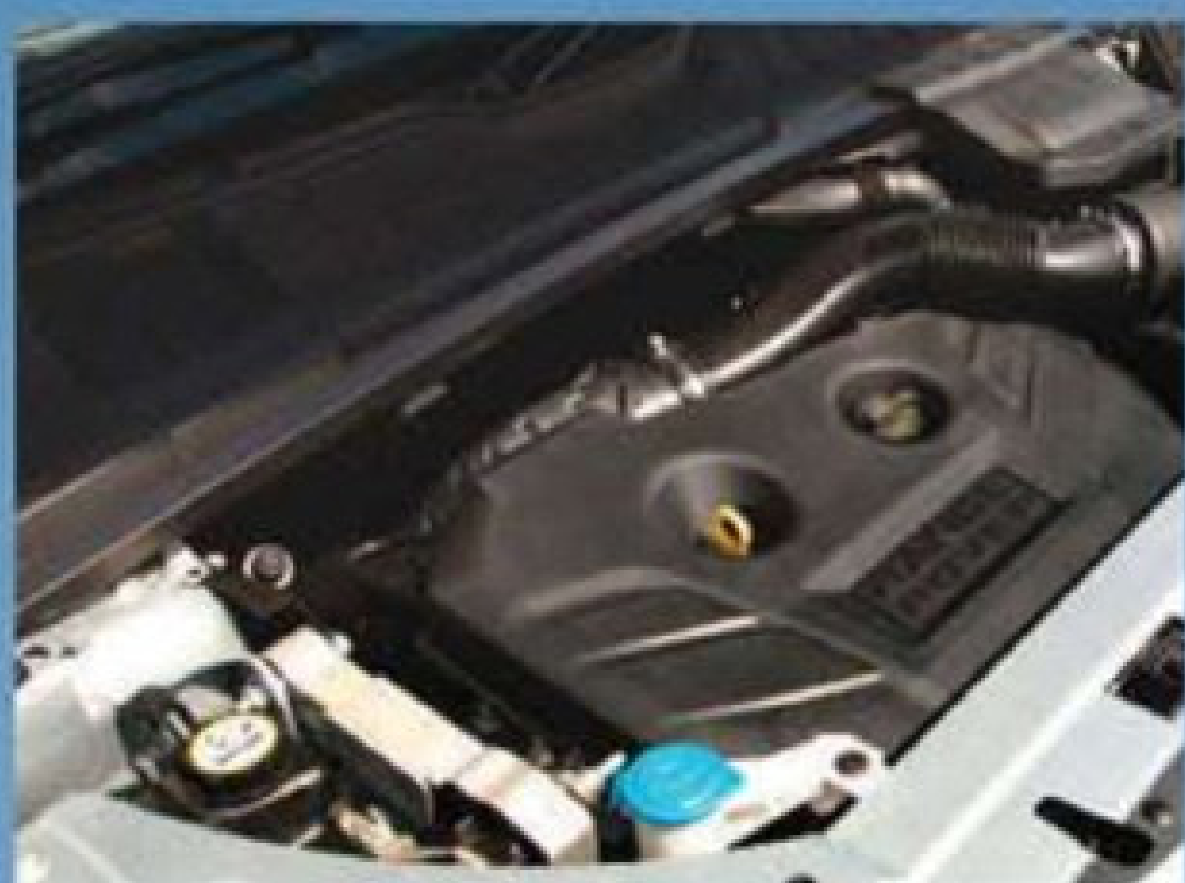
Right: 237bhp engine is a turbocharged 2-litre Ford Duratec unit; also offered are diesels with 148 and 187bhp. Far right: interior has a suitably premium feel
