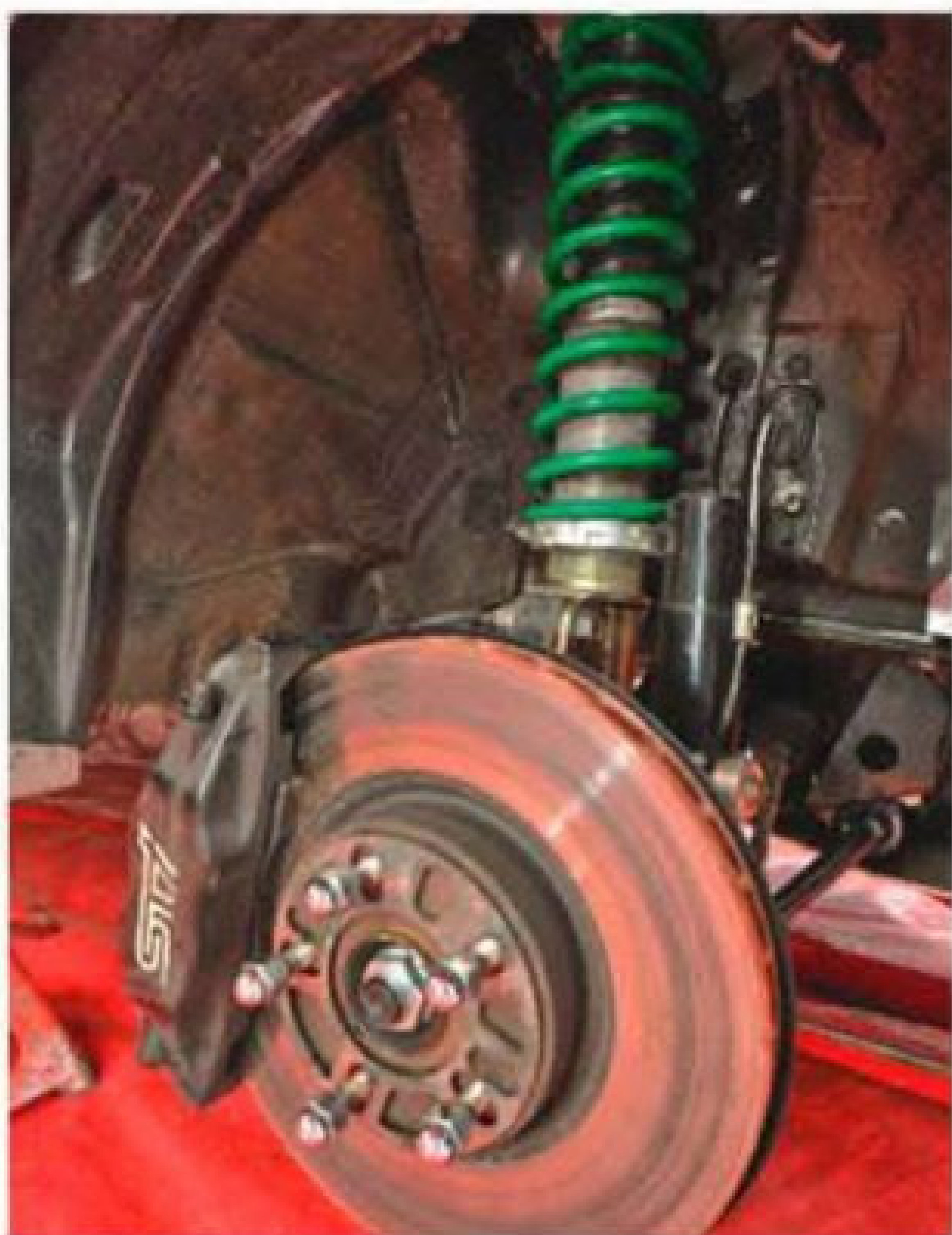
Above: Catchpole meets Higgins. Right: Tein springs and dampers are the main modification for the record attempts. Brakes are standard. Below: TT fanatics are a breed apart
