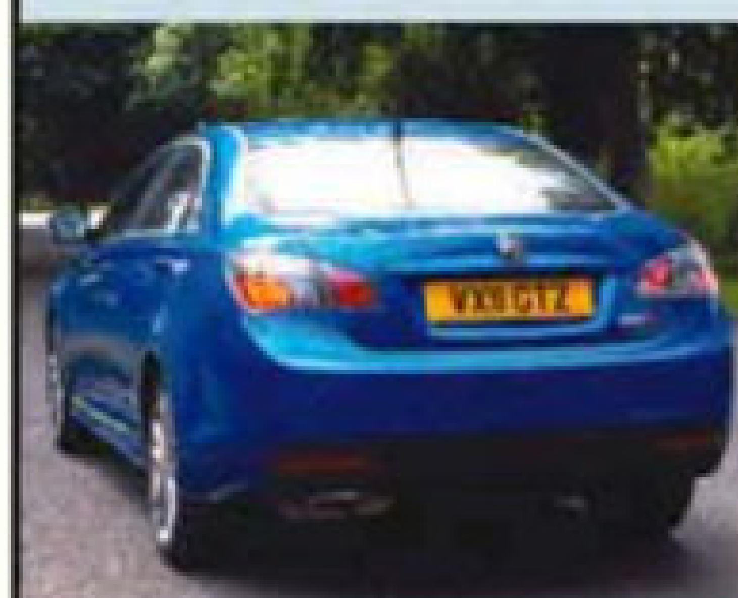
Top and left: Magnette trades the GT's high hatchback tail for a longer one containing a vast boot
