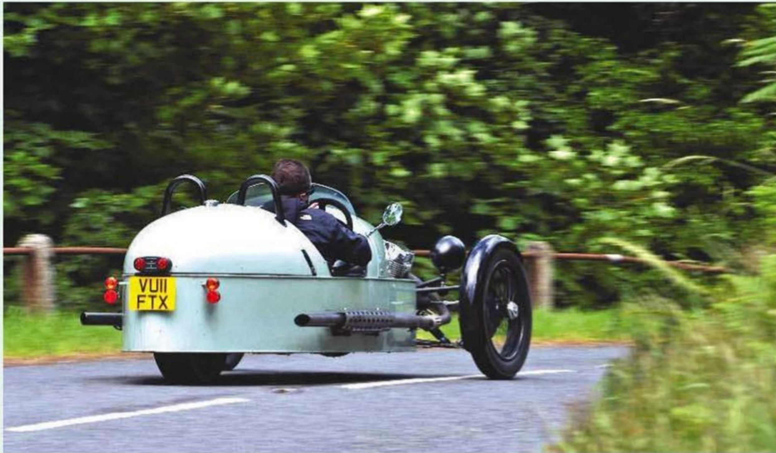
Left: air-cooled, 2-litre V-twin engine – the first in a Morgan since before WWII – sits at the very front of the car. Above: offbeat engine note is emitted from a pair of side exhausts; 3 Wheeler is Morgan's first three-wheeler in nearly 60 years
