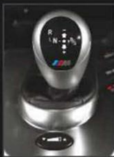
Above: hydraulically actuated SMG gearbox delivered quick shifts, but its full auto mode left a lot to be desired
