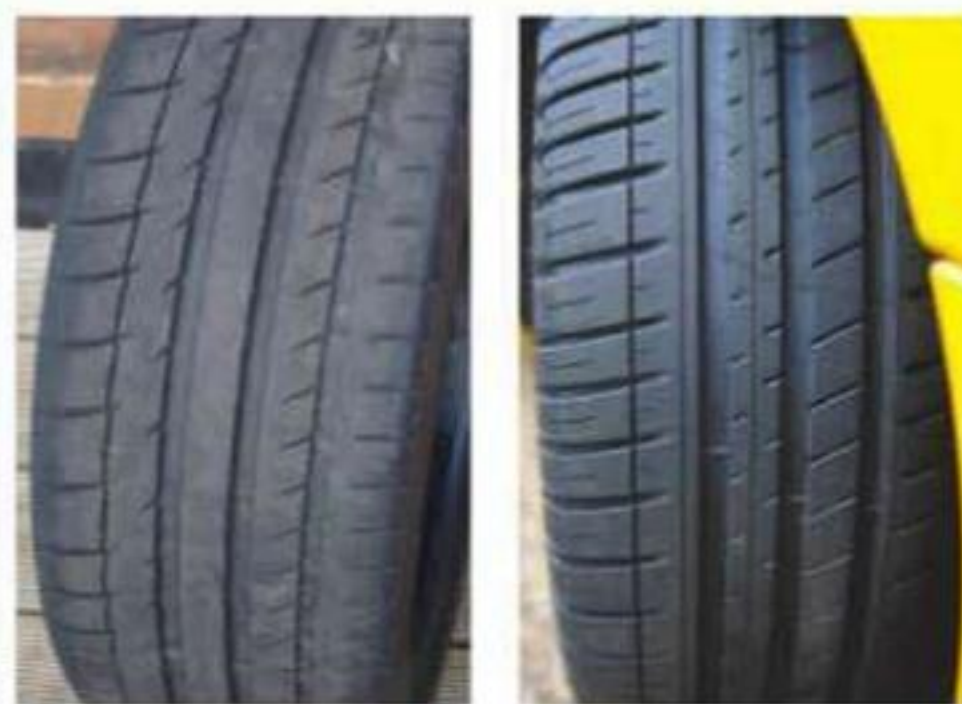
Worn Michelin Pilot Sport tyres (far left) have been replaced with a set of new Pilot Sport 3s (left) – with the fronts in a slightly wider size than before
