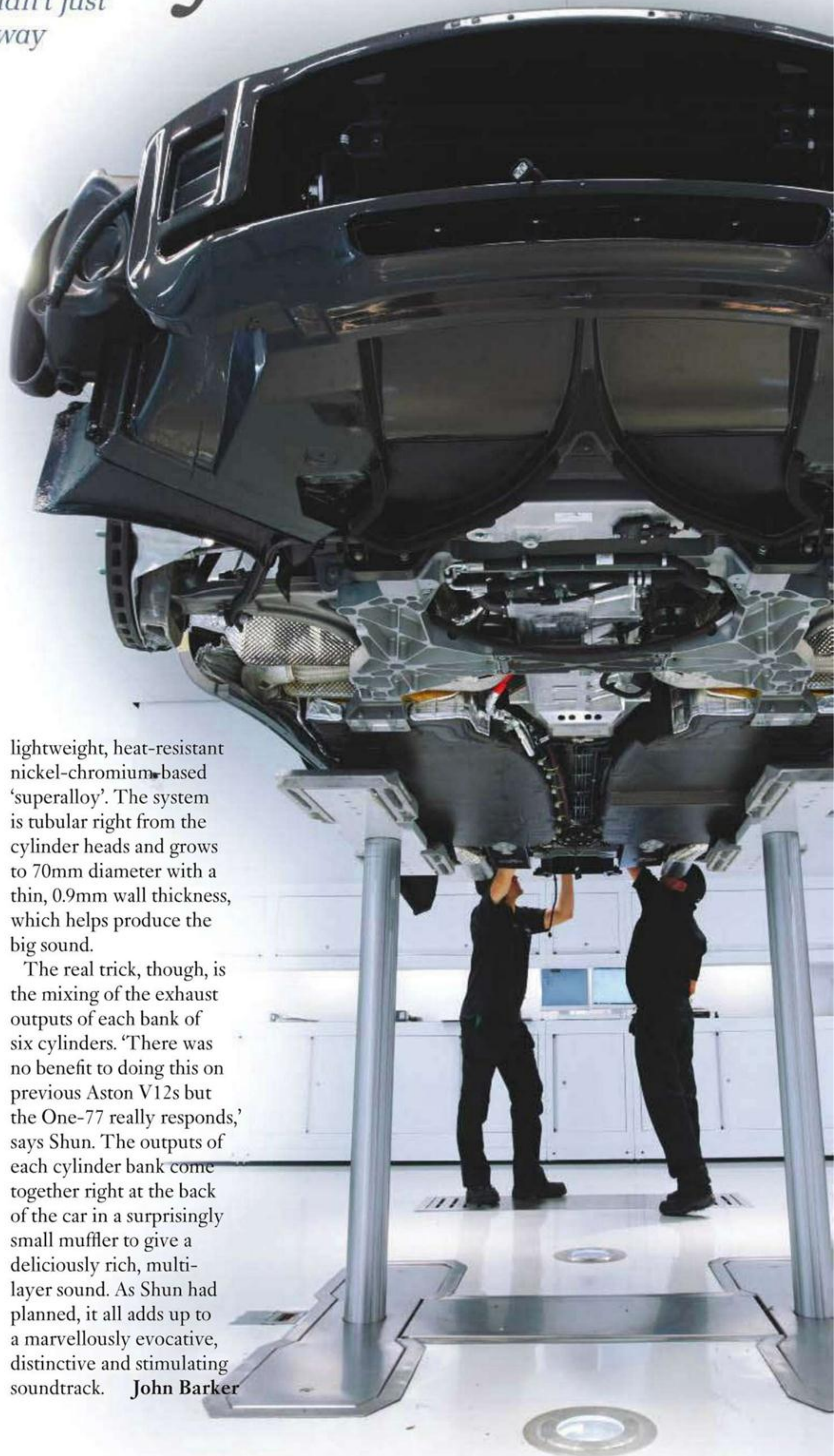
Above: 7.3-litre V12 is unique to the One-77. Left: exhaust system is made from Inconel
