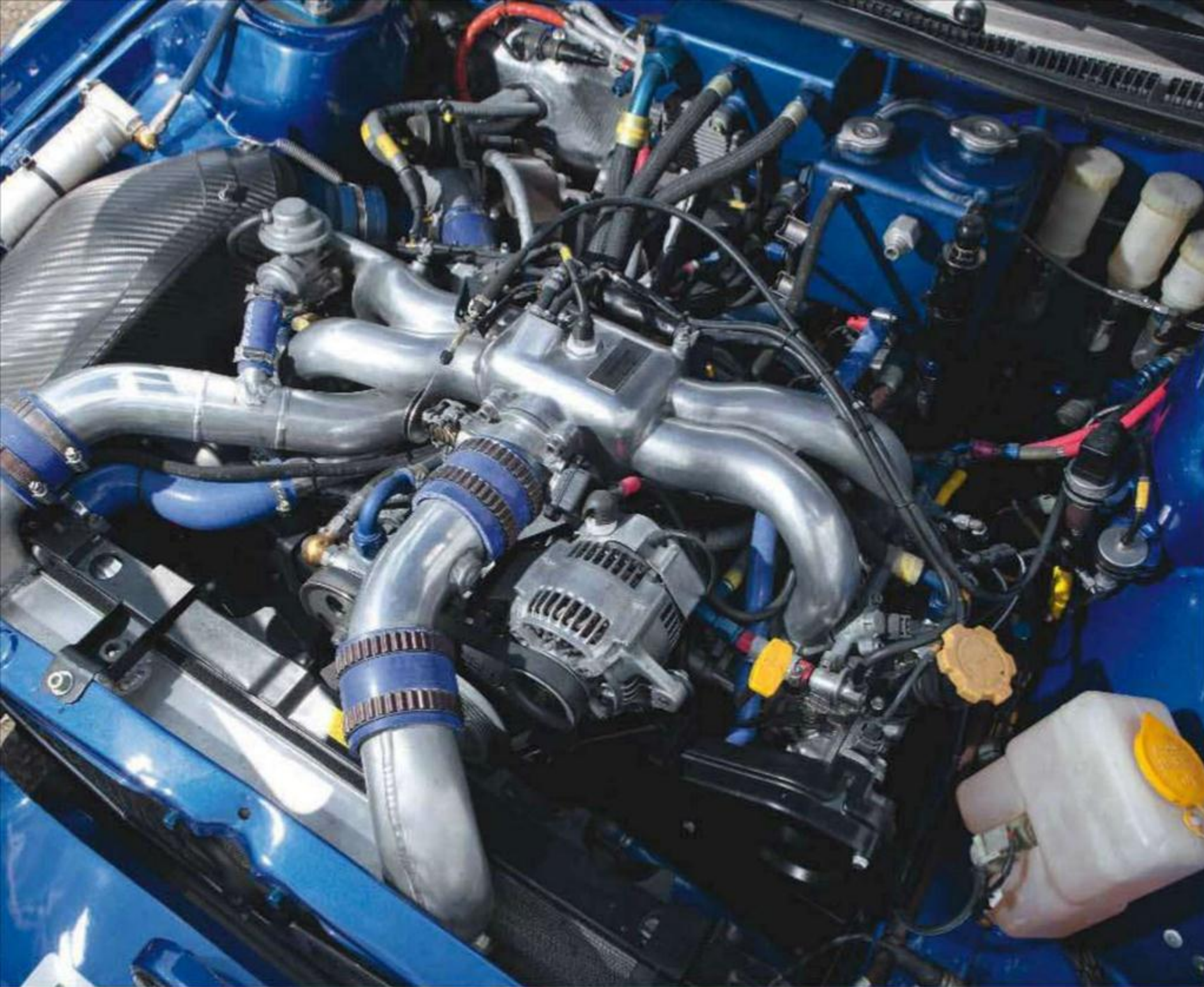
Left: turbocharged 2-litre flat-four not quite as distinctive here as in the earlier Group A Imprezas, but it is good for 310bhp. Above: roof-mounted vent feeds cool air to cockpit. Bottom: Catchpole at the wheel; headphones essential for communicating with co-driver
