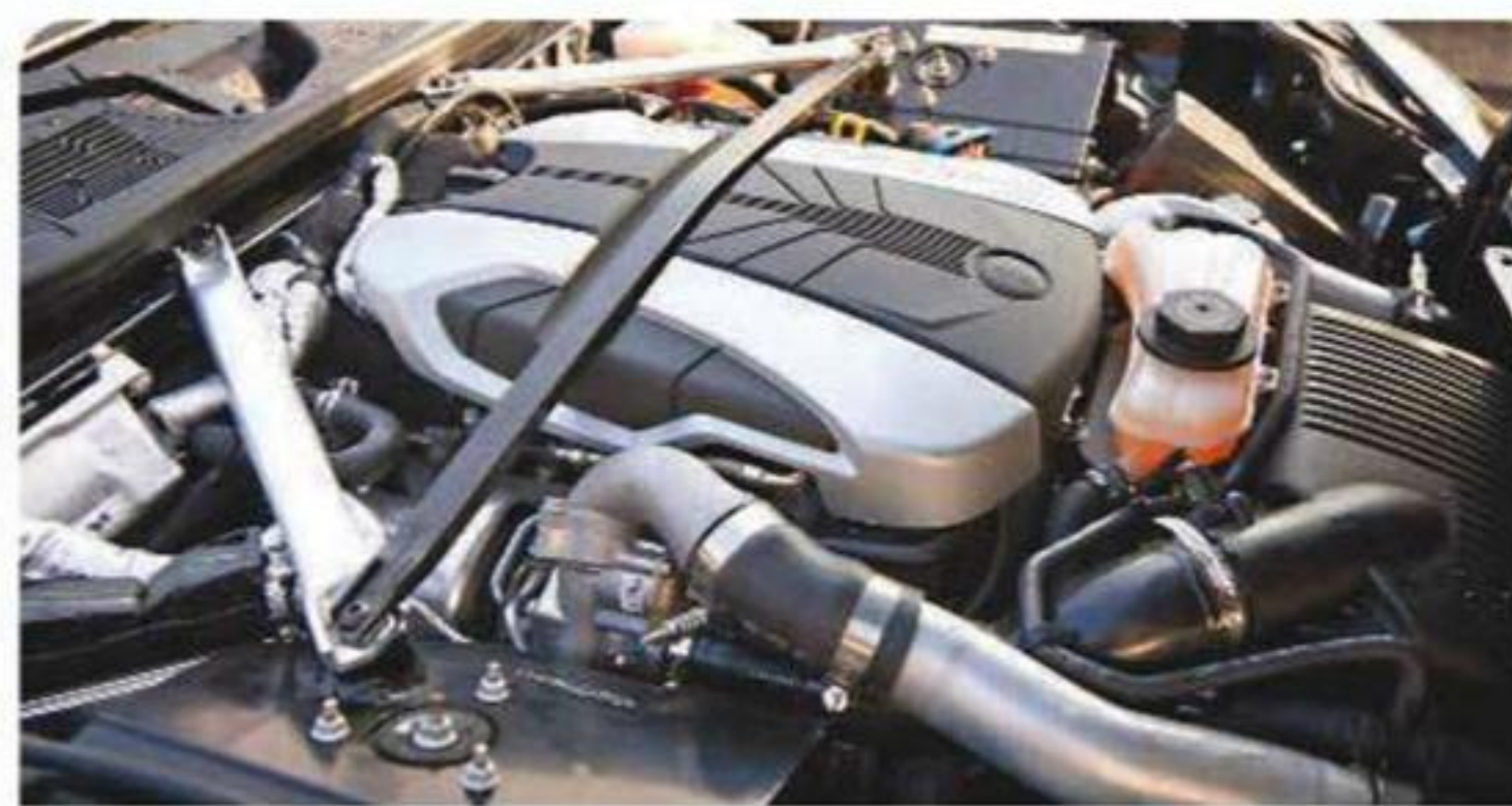
Above: 2-litre turbo motor doesn't drive the wheels but supplies power to the electric motors or charges the batteries
