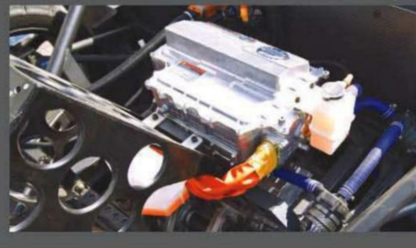
Below: AC motor's 107bhp and 207lb ft is sent to the rear wheels; 0-62mph takes 6.9sec
