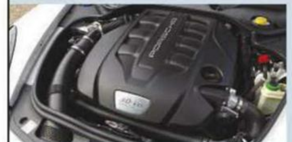
Above: V6 diesel is an Audi unit that produces 247bhp. Right: gearbox is a conventional torque-converter automatic
