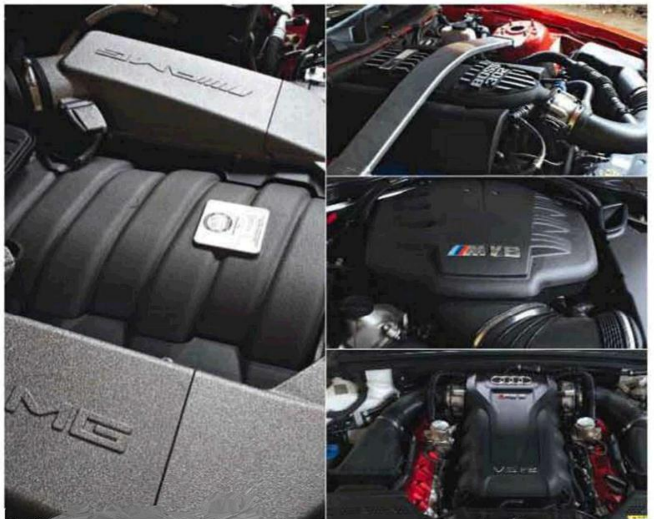
The four V8 engines, clockwise from right: Merc's 451bhp 6.2, Mustang's 444bhp 5.0 (that's 302 cubic inches), BMW's 444bhp 4.4 and Audi's 444bhp 4.8
