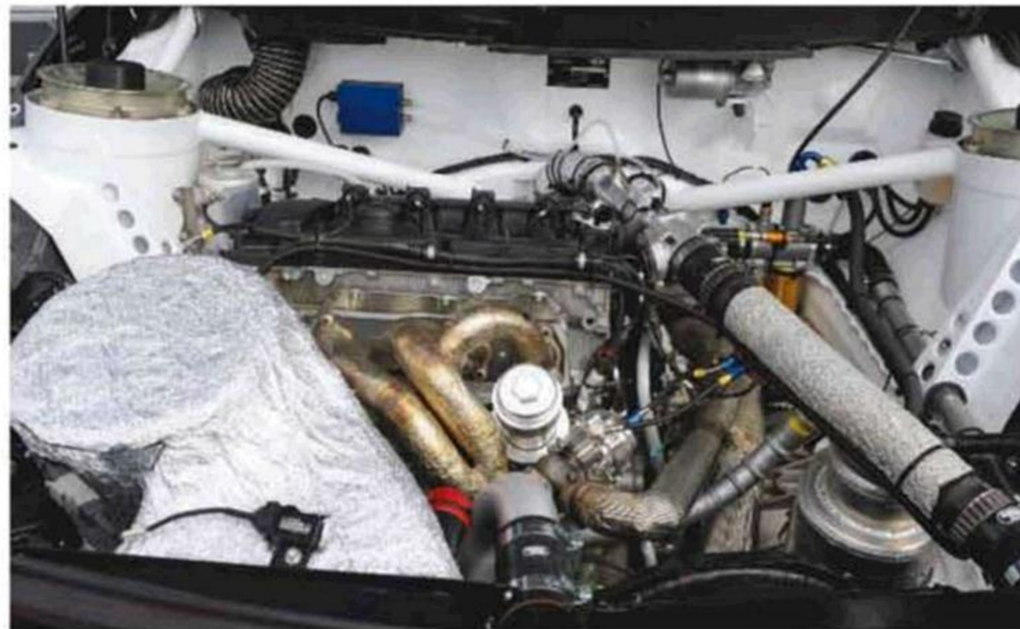
Left: 1.6-litre engine is the work of BMW Motorsport; features include a dry sump and a Garrett turbo capable of running 2.5bar of boost. Engine bay dominated by air intake box with copious heat-proofing
