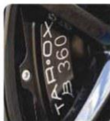
Above right: titanium tailpipes measure 100mm in diameter; difference in sound is modest. Above: ten-piston front calipers bring improved stopping power
