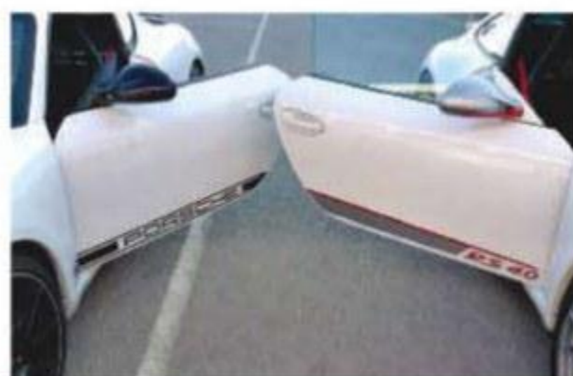
Left: Cayman and 911 share a number of components, including doors. 'M' button on 1M's wheel (far left) simply alters the throttle response
