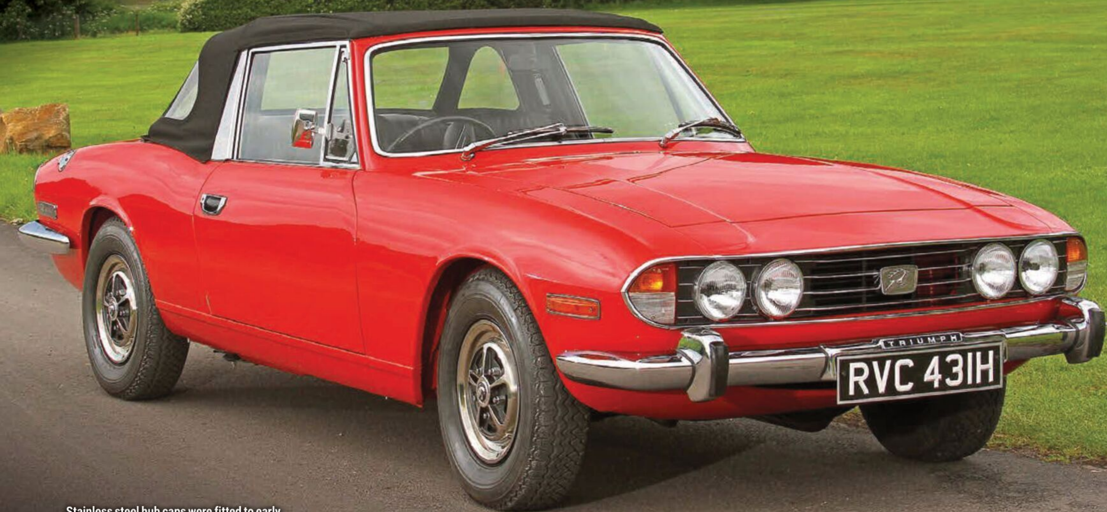
Stainless steel hub caps were fitted to early Stags. Note the lack of pinstriping.
