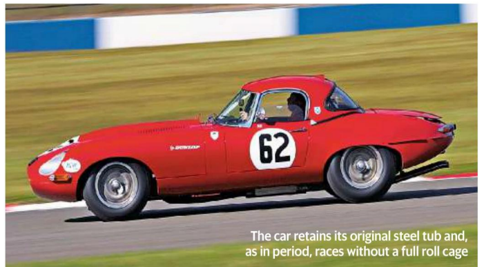
The car now has an aluminium bonnet, boot lid, doors, and hard-top, but all the original steel panels can be refitted
