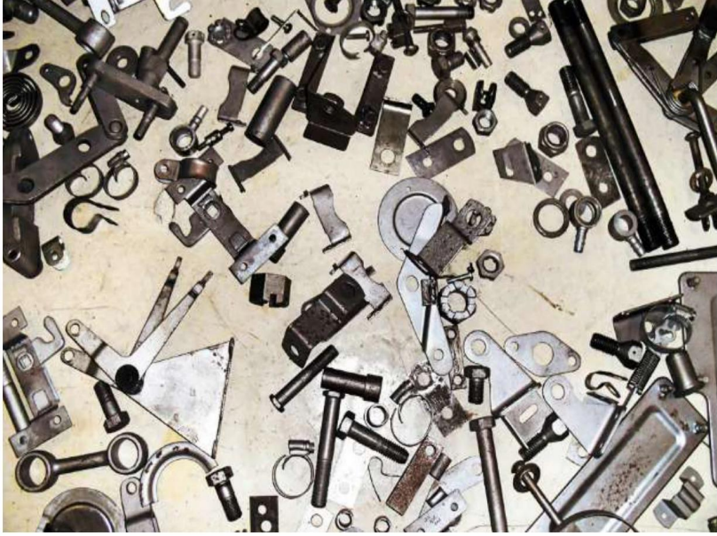
Every single fixing was bead-blasted, cadmium-plated and re-used
