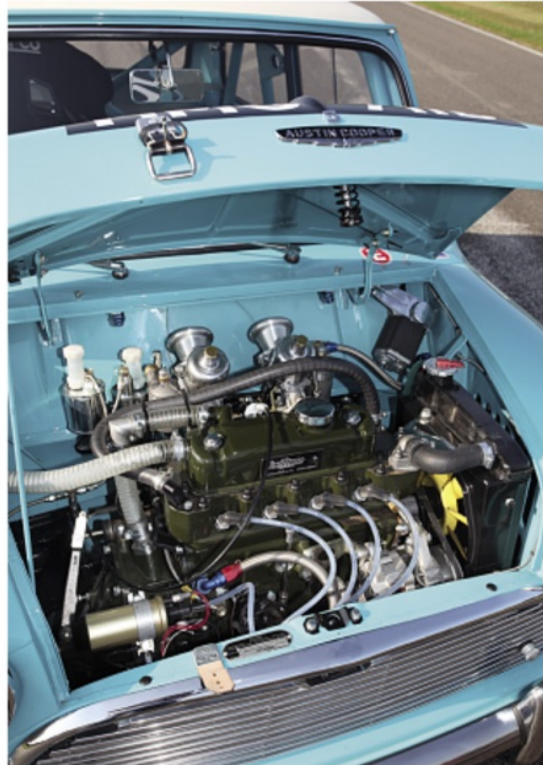
Hot Swift-tune-built engine gives around 122bhp
