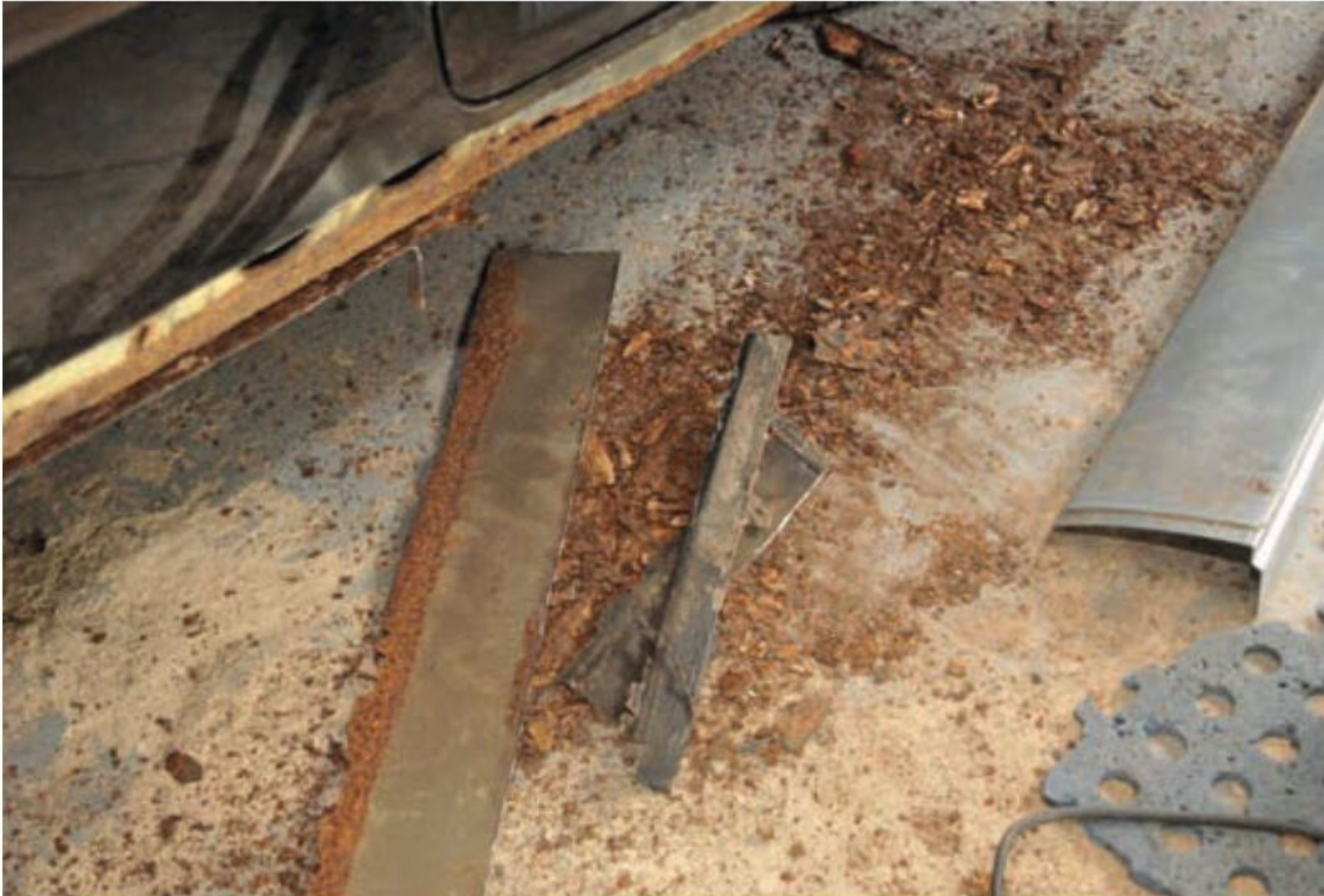
While it could have been patched, corrosion like this meant that a full replacement was likely to be cheaper long term.
