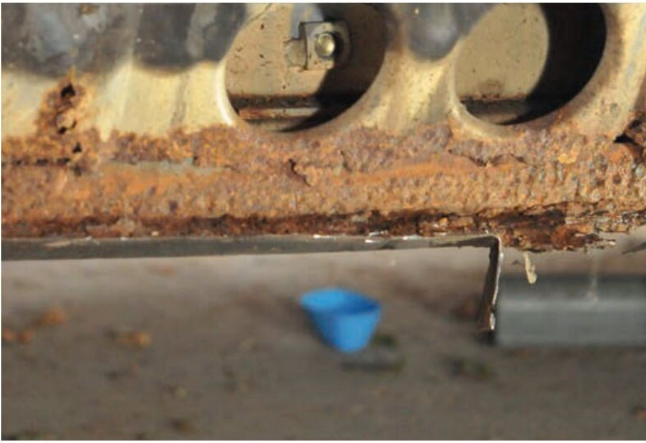
Rather than patch this sill, Paul engaged a mobile welder to replace the whole thing.
