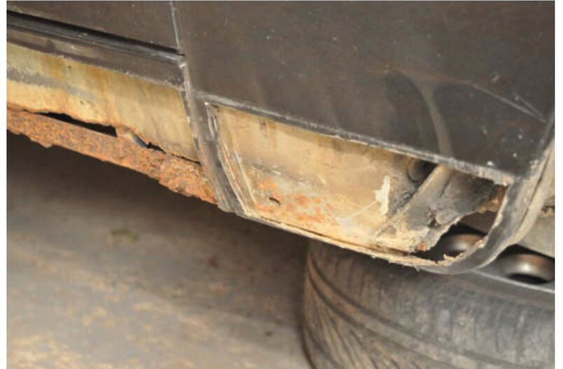
While it could have been patched, corrosion like this meant that a full replacement was likely to be cheaper long term.
