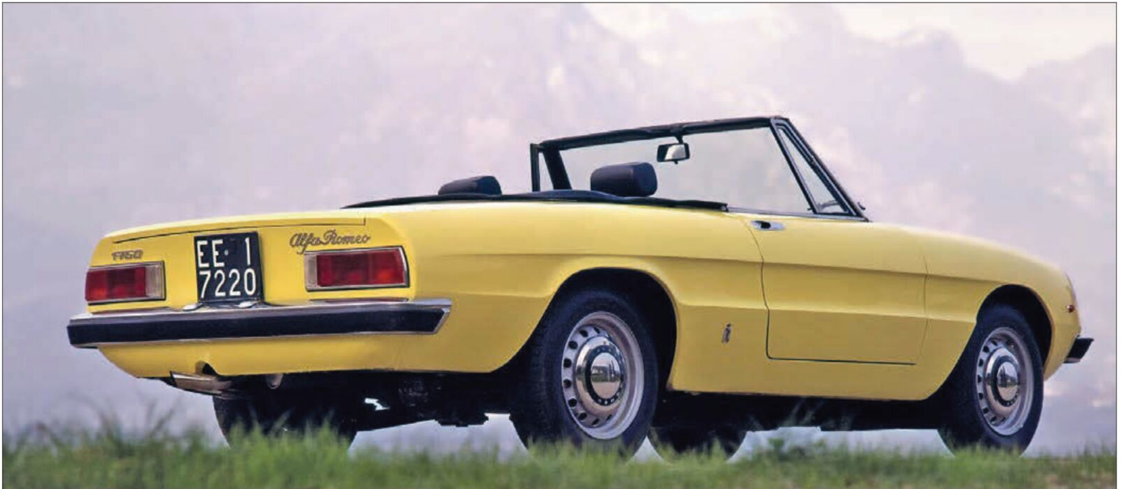
Series 2 Spider featured revised tail, doorhandles and windscreen rake. It was shorter, but offered more luggage space.
