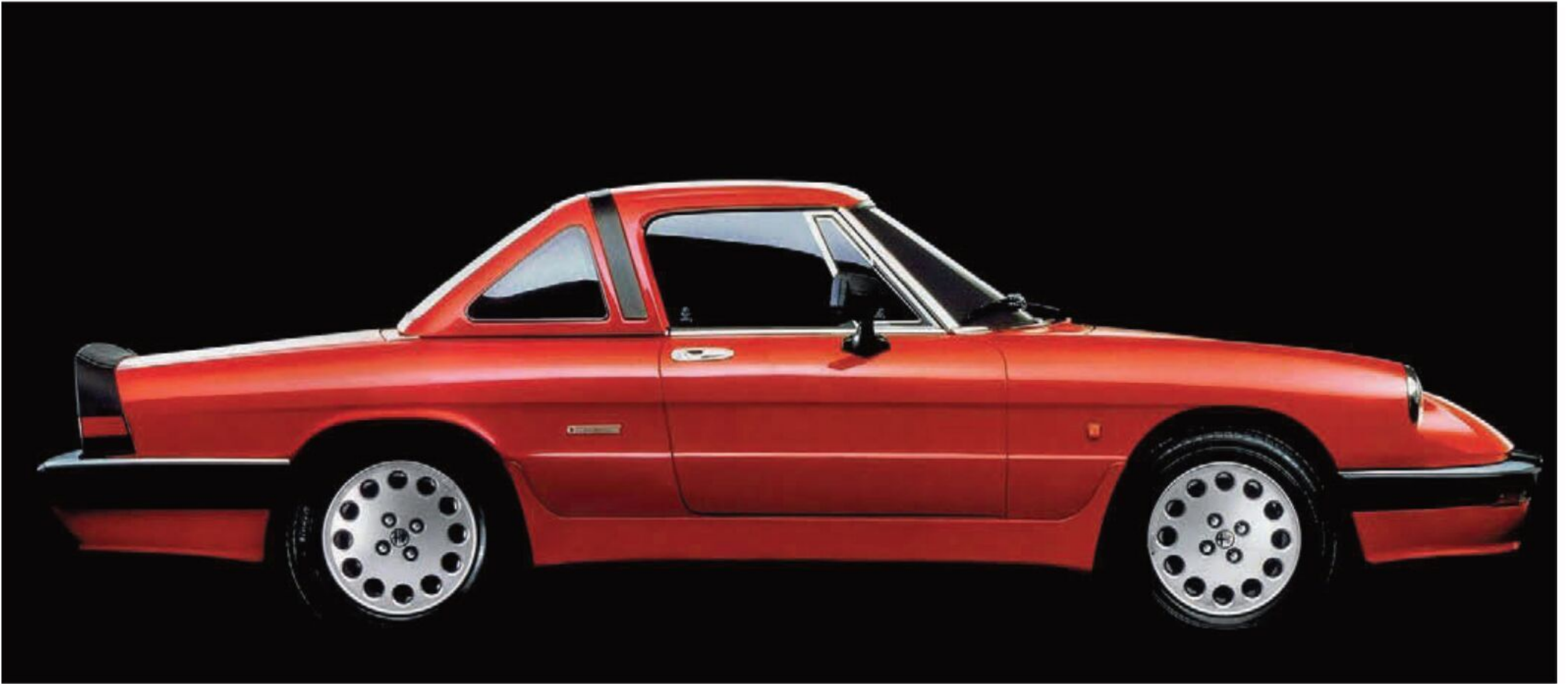
S3 Cloverleaf had big skirts and a choice of three colours. The rubber bumpers and duck tail spoiler were shared with all S3s.
