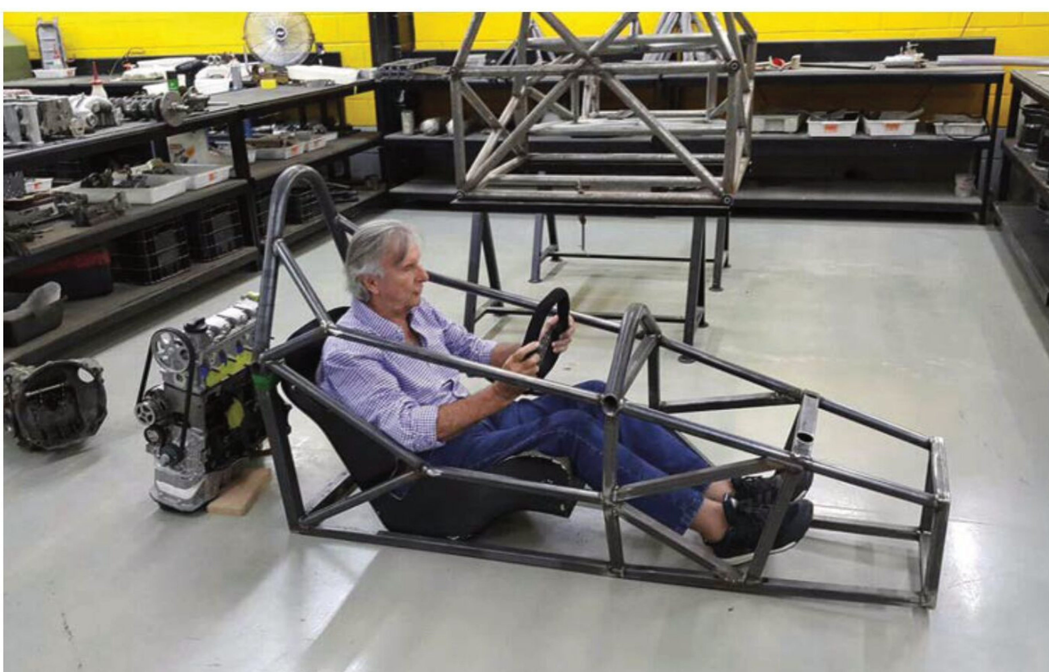
The spaceframe of Divila's Formula Vee project. The ergonomics of a design must be considered at quite an early stage
