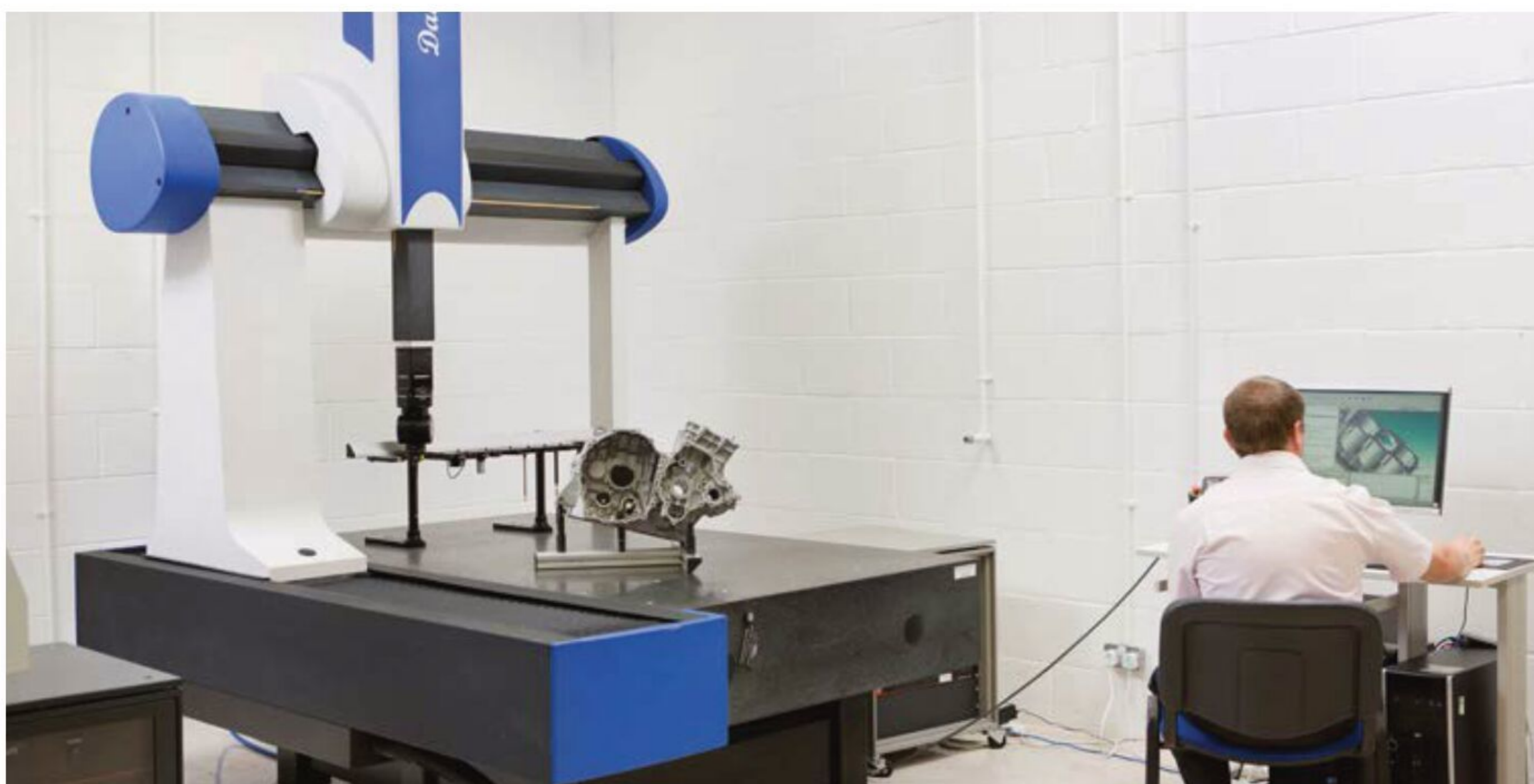
A five-axis CMM using REVO. The CMM head automatically selects a stylus from the rack via magnets in the probe's head
