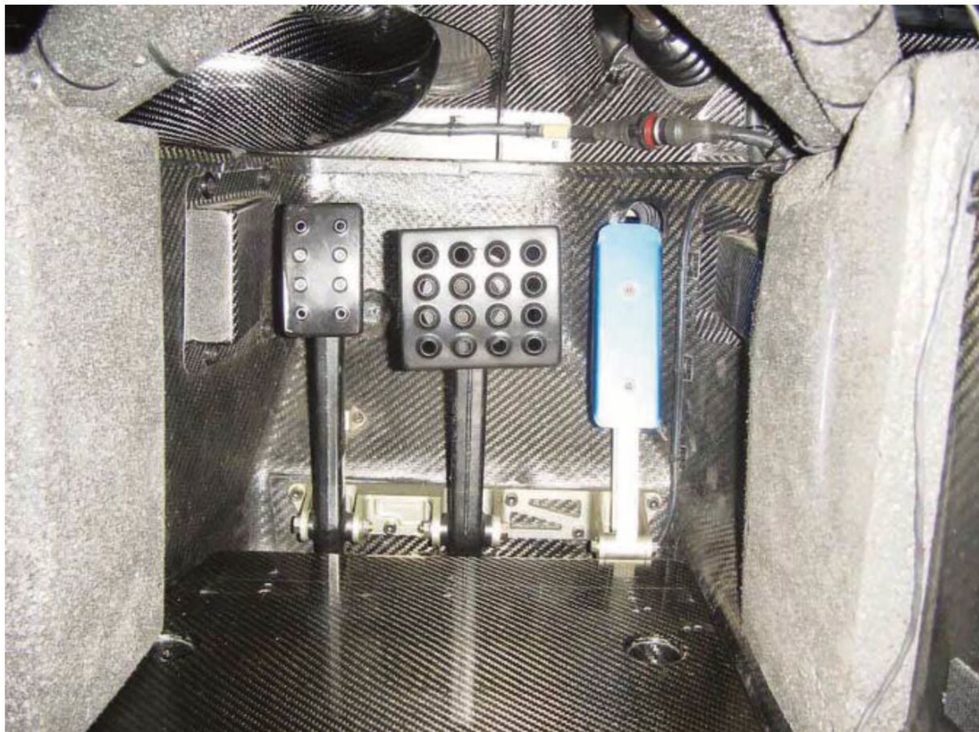
The padding in the footwell of the Nissan Super Touring Car was to protect the driver's legs during accidents
