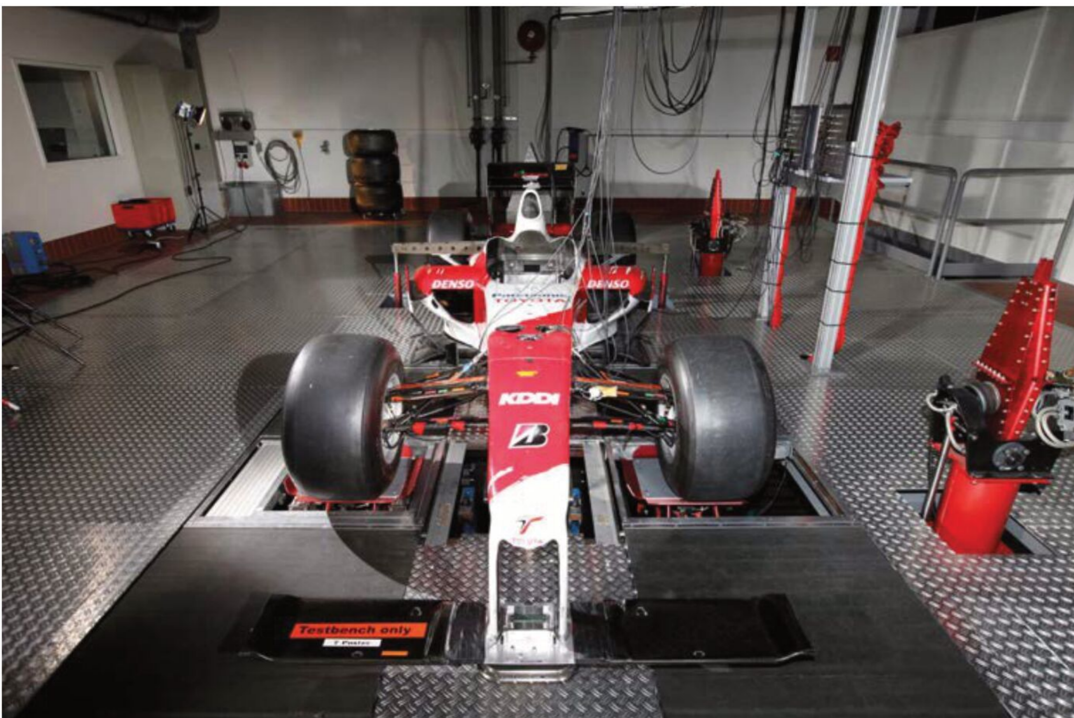
Toyota Formula 1 car in the TMG facility. Seven-post rigs are vital when aerodynamic loads also need to be taken into account
