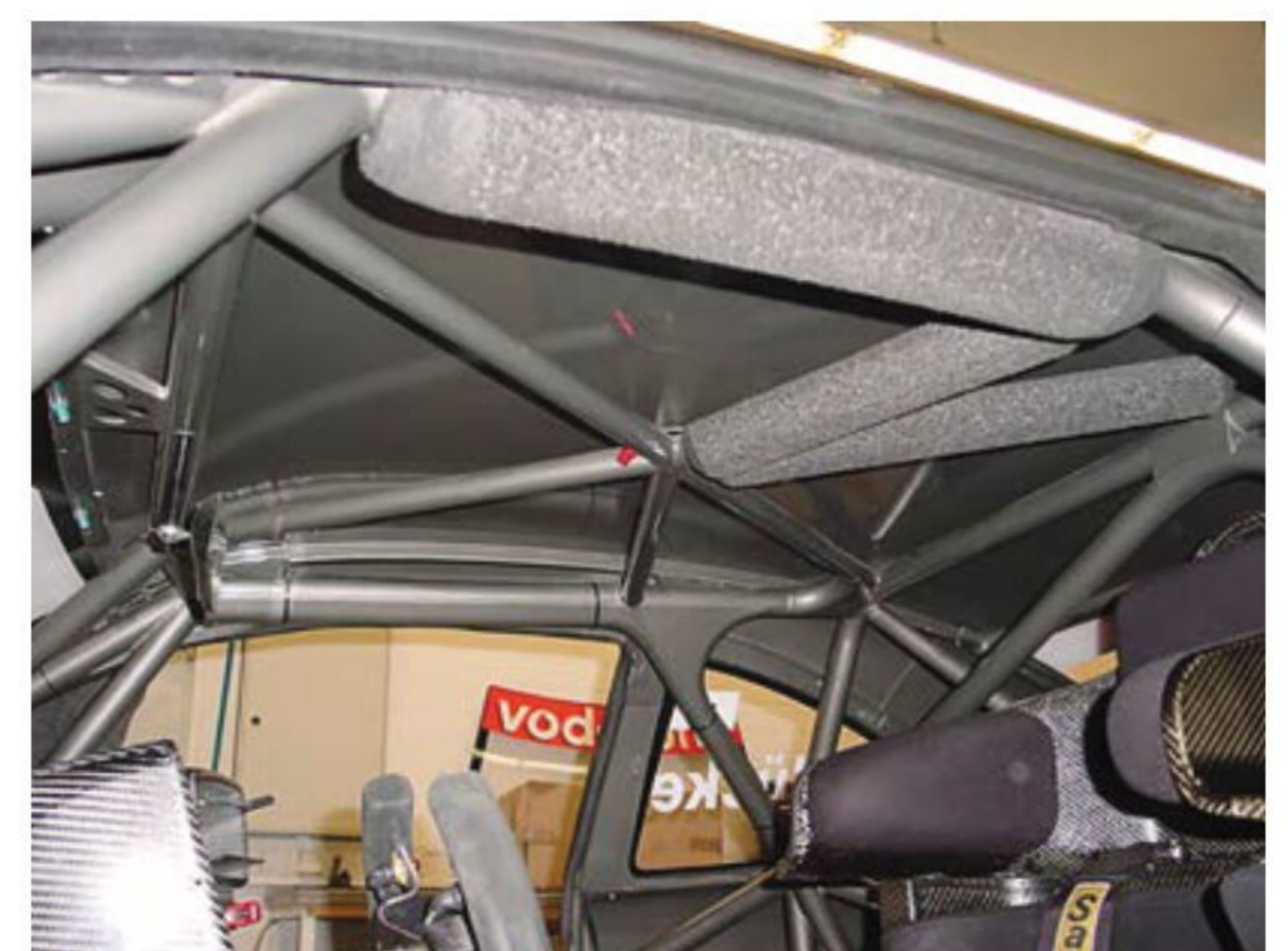
Cockpit padding is a simple, cheap, highly effective safety measure
