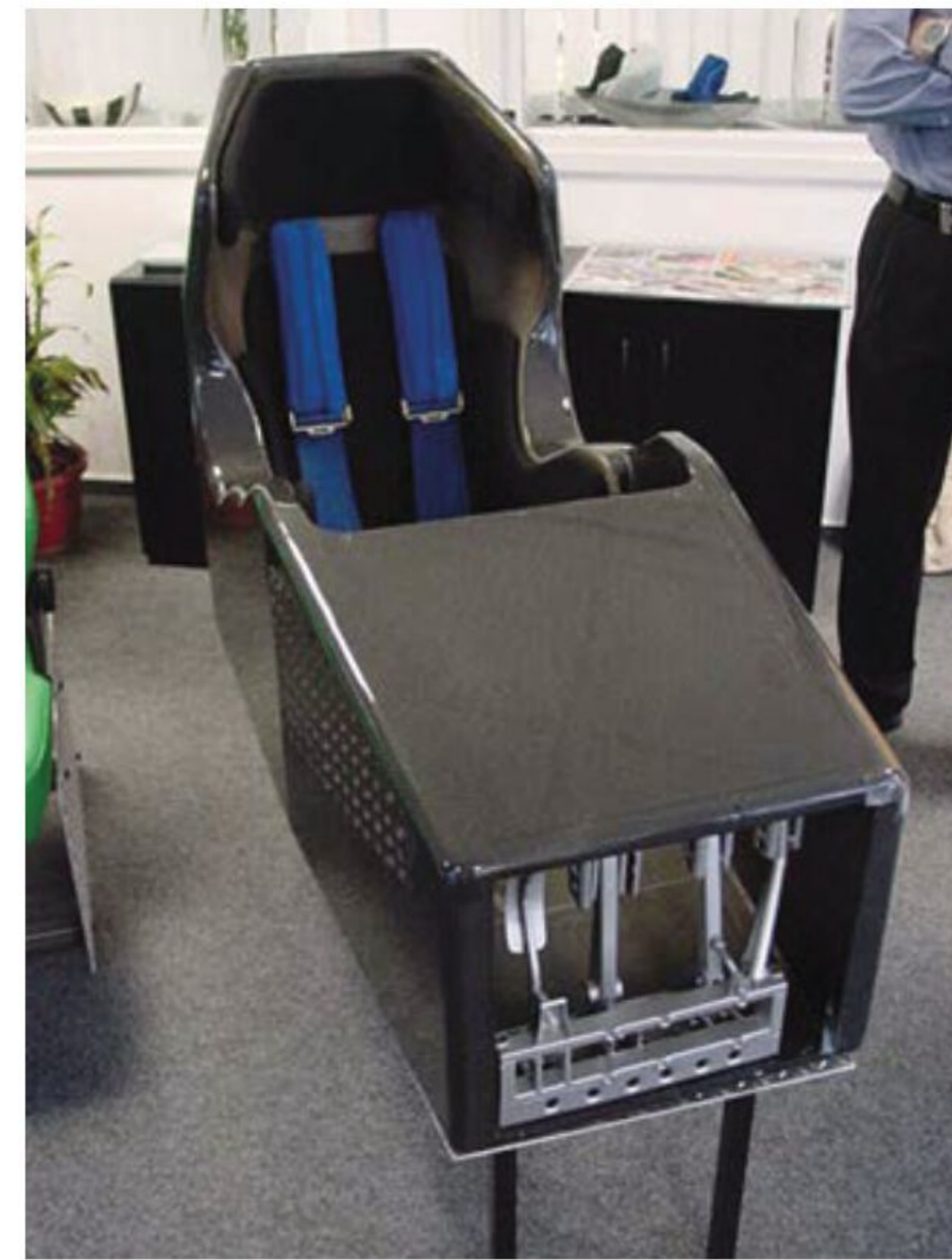
This survival cell fitted into the DTM spaceframe
