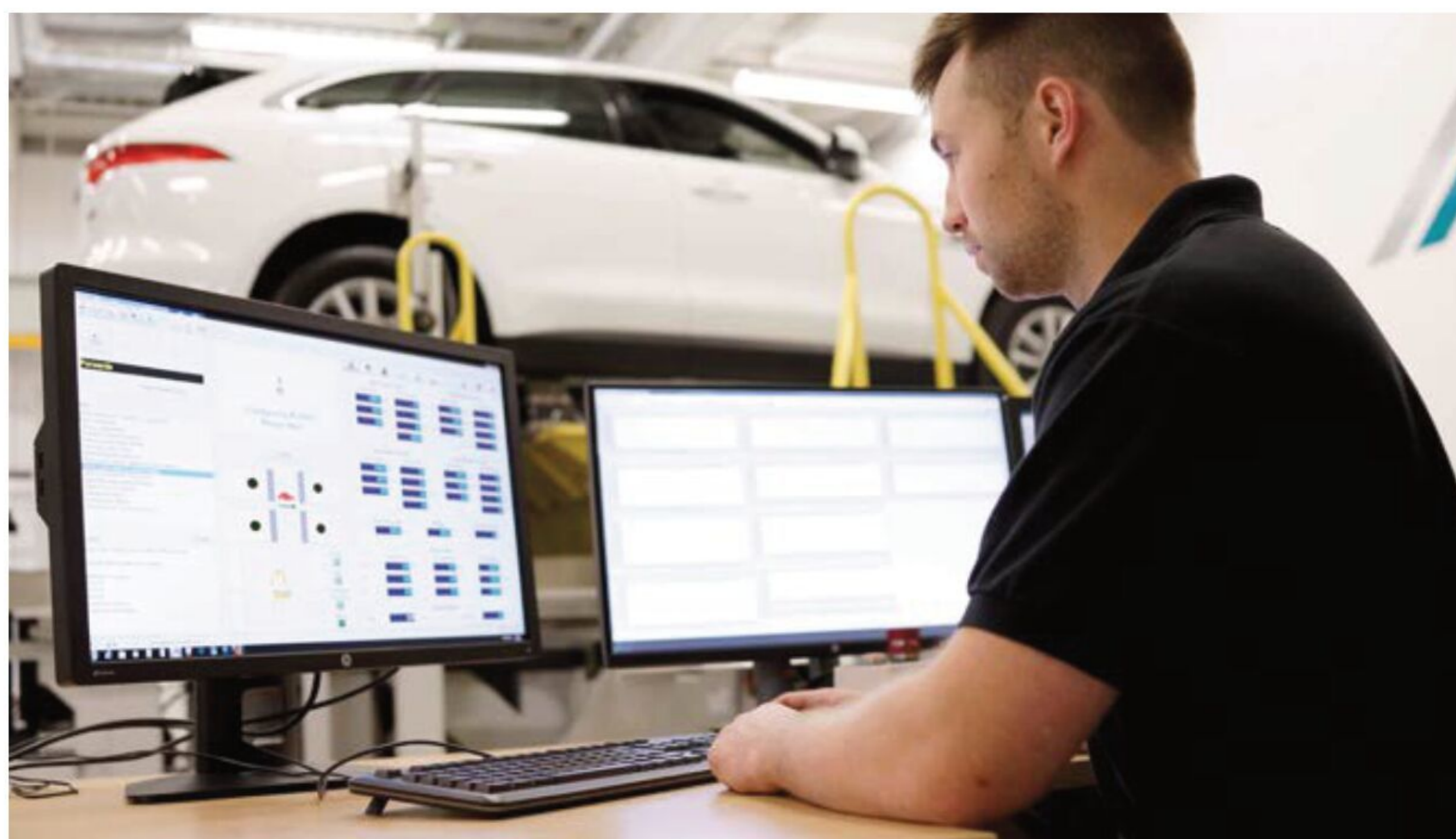
Data from the K&C tests at MIRA can be monitored live by technicians, and also stored for later analysis
