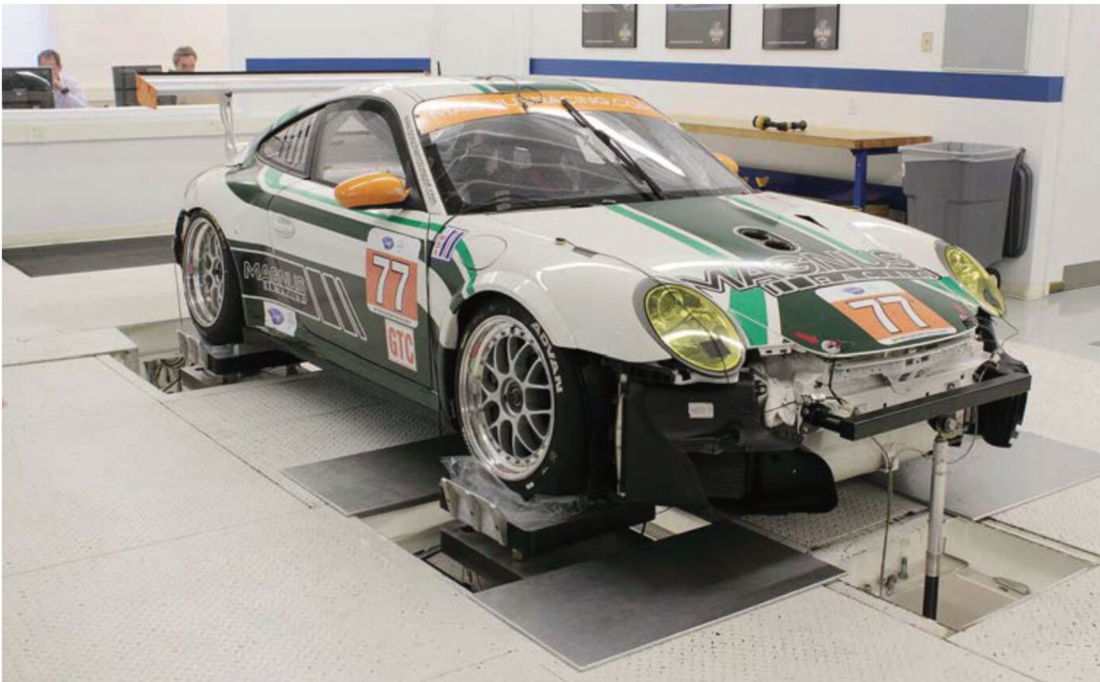
Damper manufacturers will use rigs for testing their new hardware developments. This is the Öhlins seven-post 'room'
