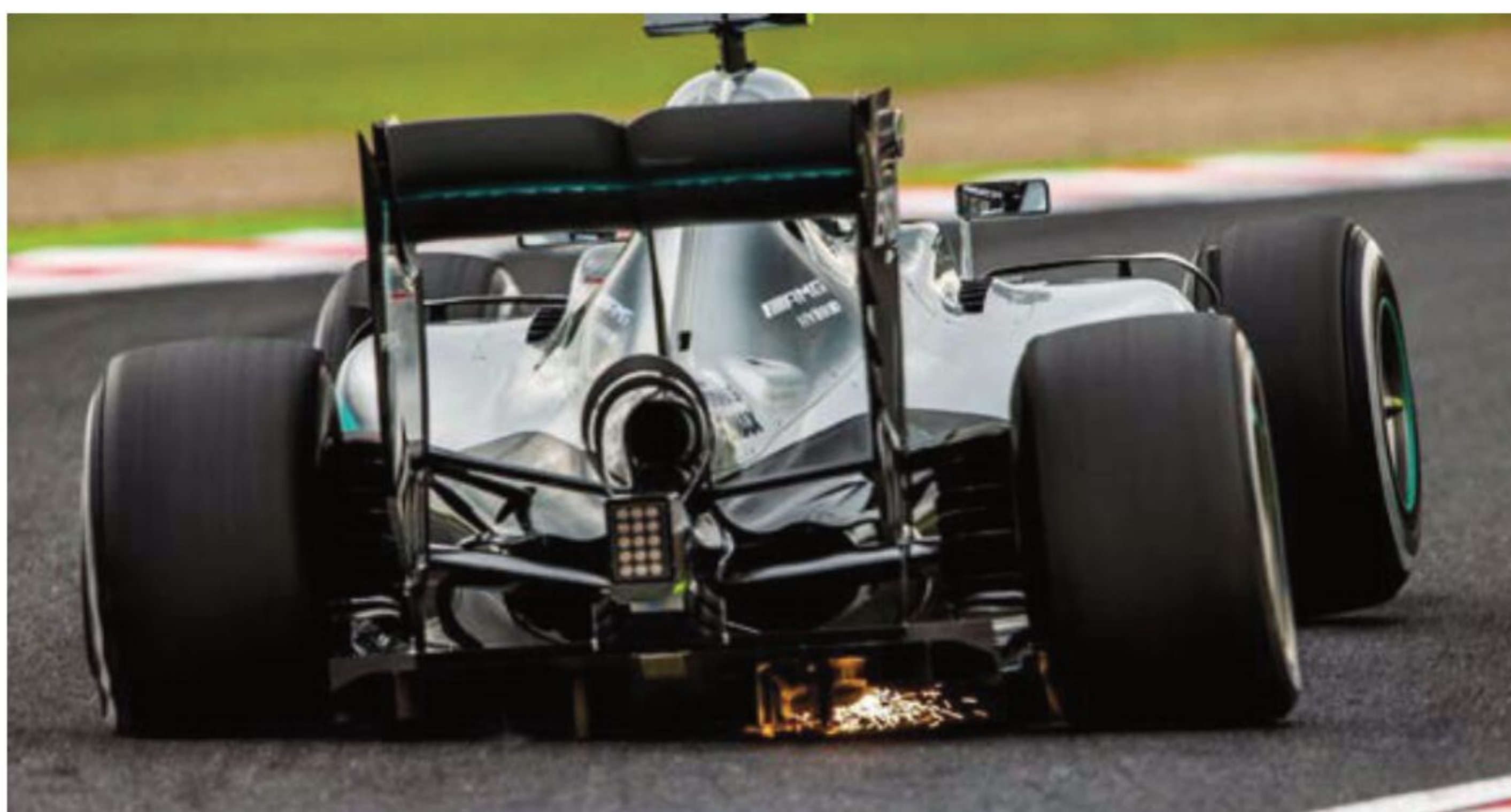
Large forces generated in cornering can cause suspension components to flex substantially
