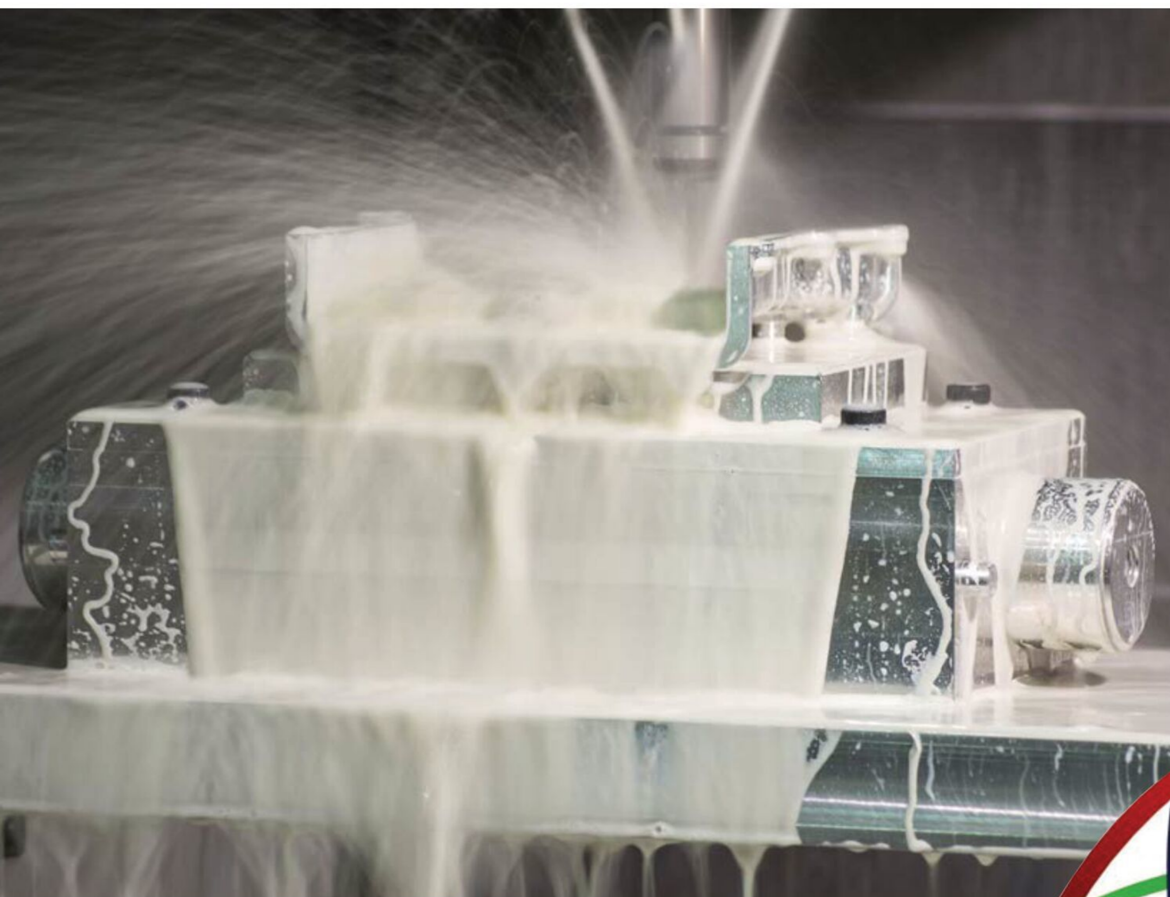
Liquid coolant / cutting agent is blasted at 1000psi to the tip of the tool, reducing the temperature generated from friction and also removing swarf, which could otherwise weld itself to the part
