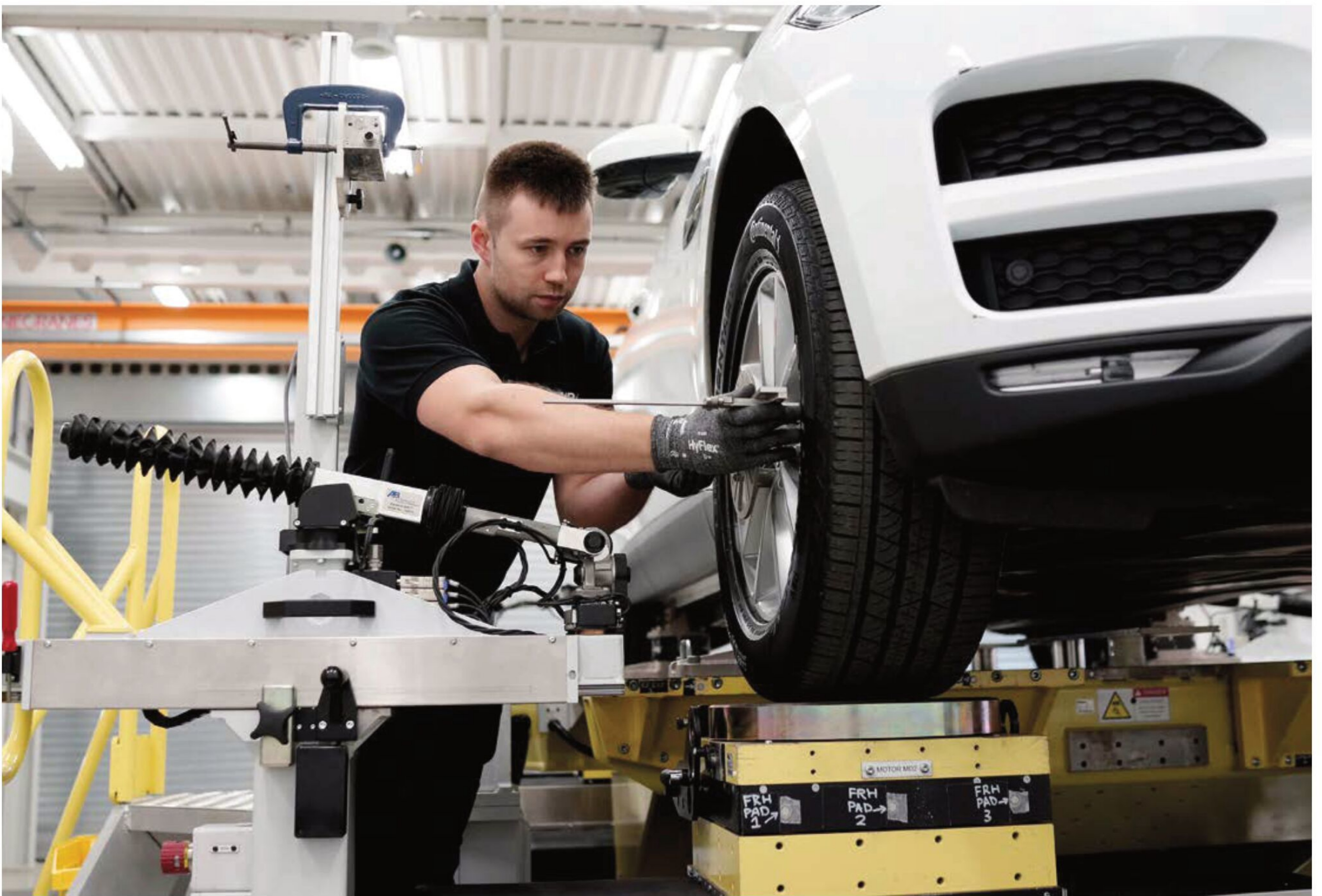
On the MIRA rig, the chassis is clamped to a large and rigid bed plate while the wheels are supported by four pads. The test car can then be actuated in pitch, heave and roll modes
