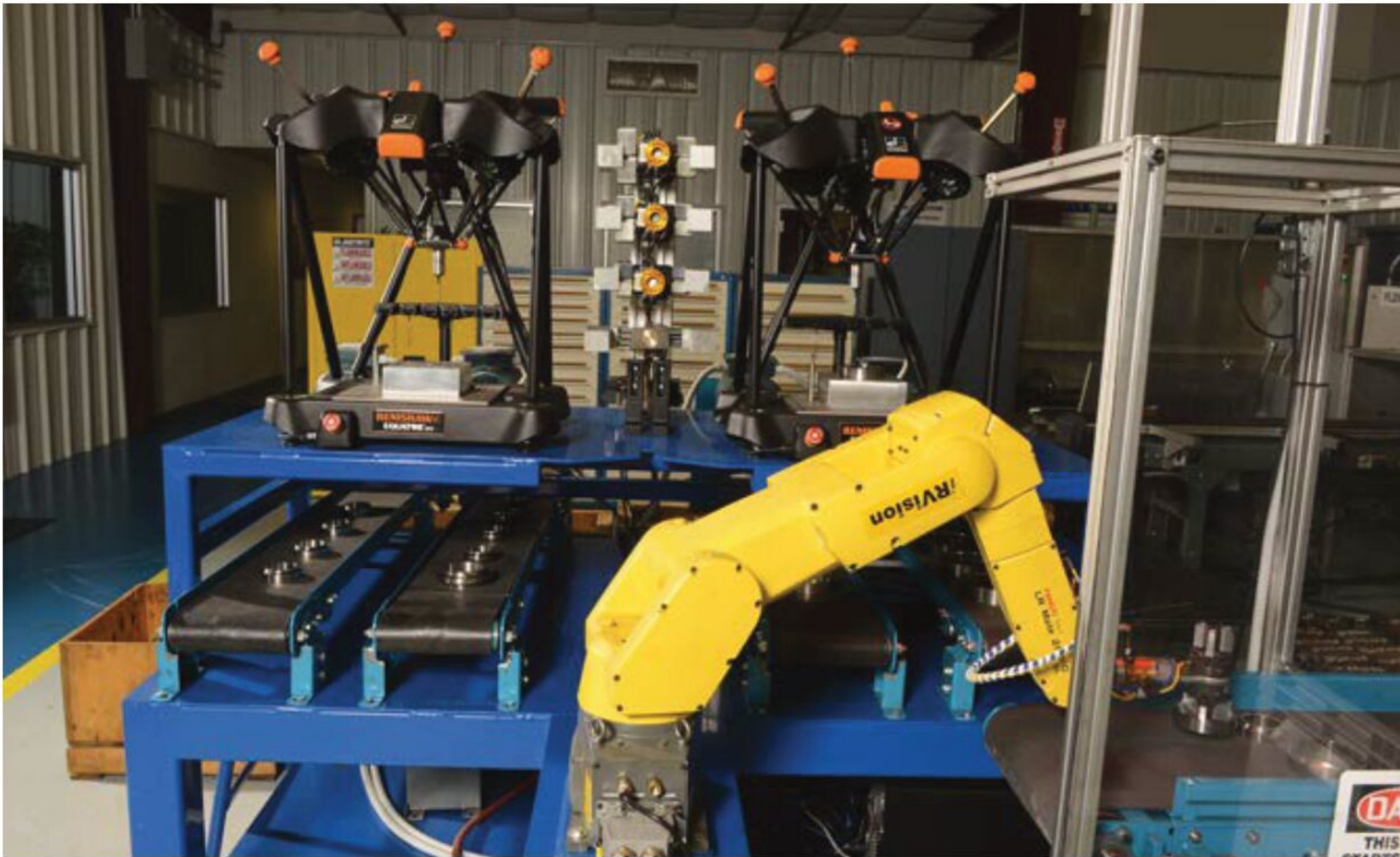
The Equator Gauge can be integrated into the manufacturing process and used to check parts as soon as they have been made. Robots move parts from the machine and automatically load them on to the Equator
