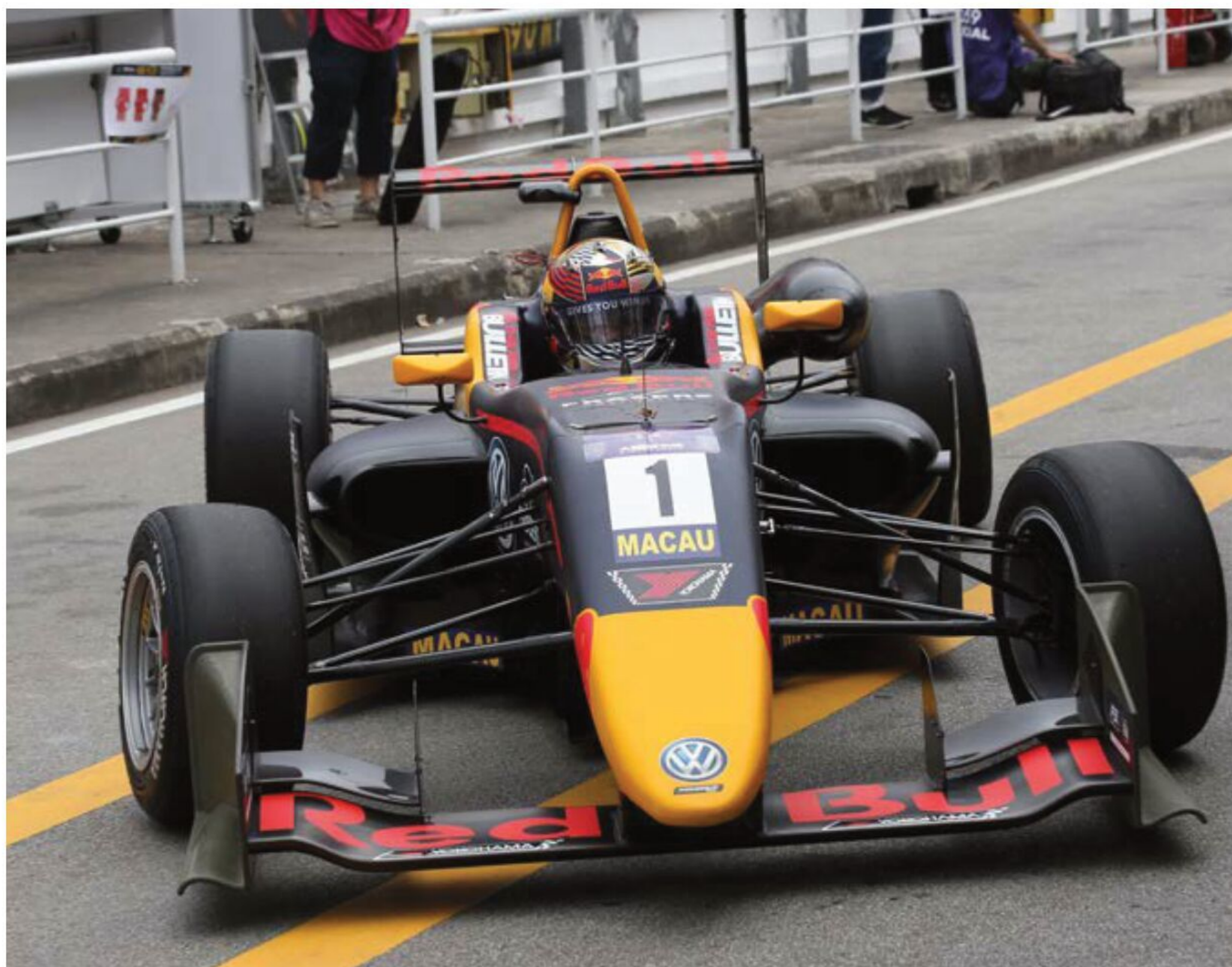
The muscular effort needed to steer a traditional Formula 3 car, which has no power steering, is surprising
