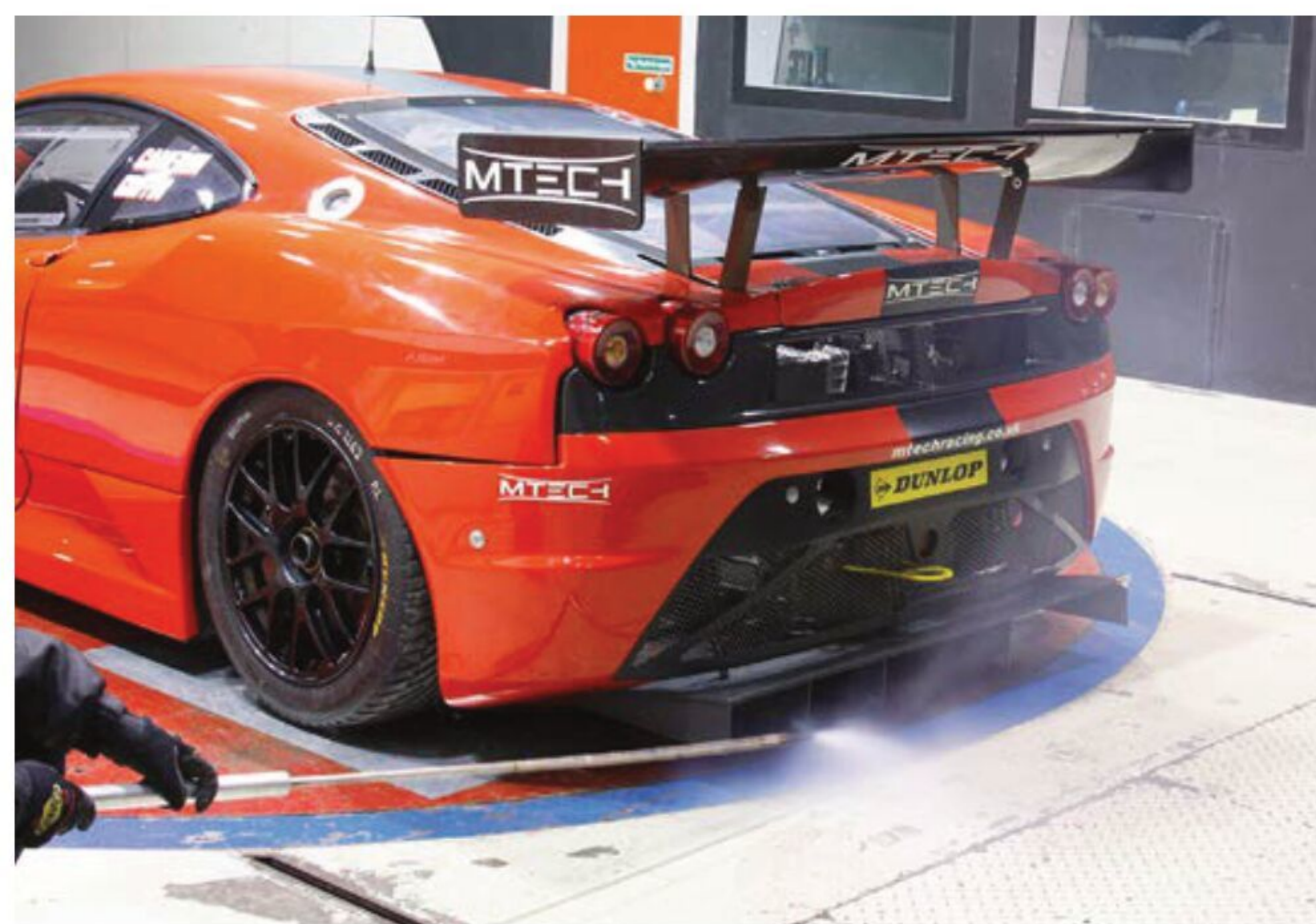
...while the flow from the outer diffuser sections was untidy, reflecting what the CFD simulations indicated. This particular Ferrari was tested in the MIRA wind tunnel in 2010
