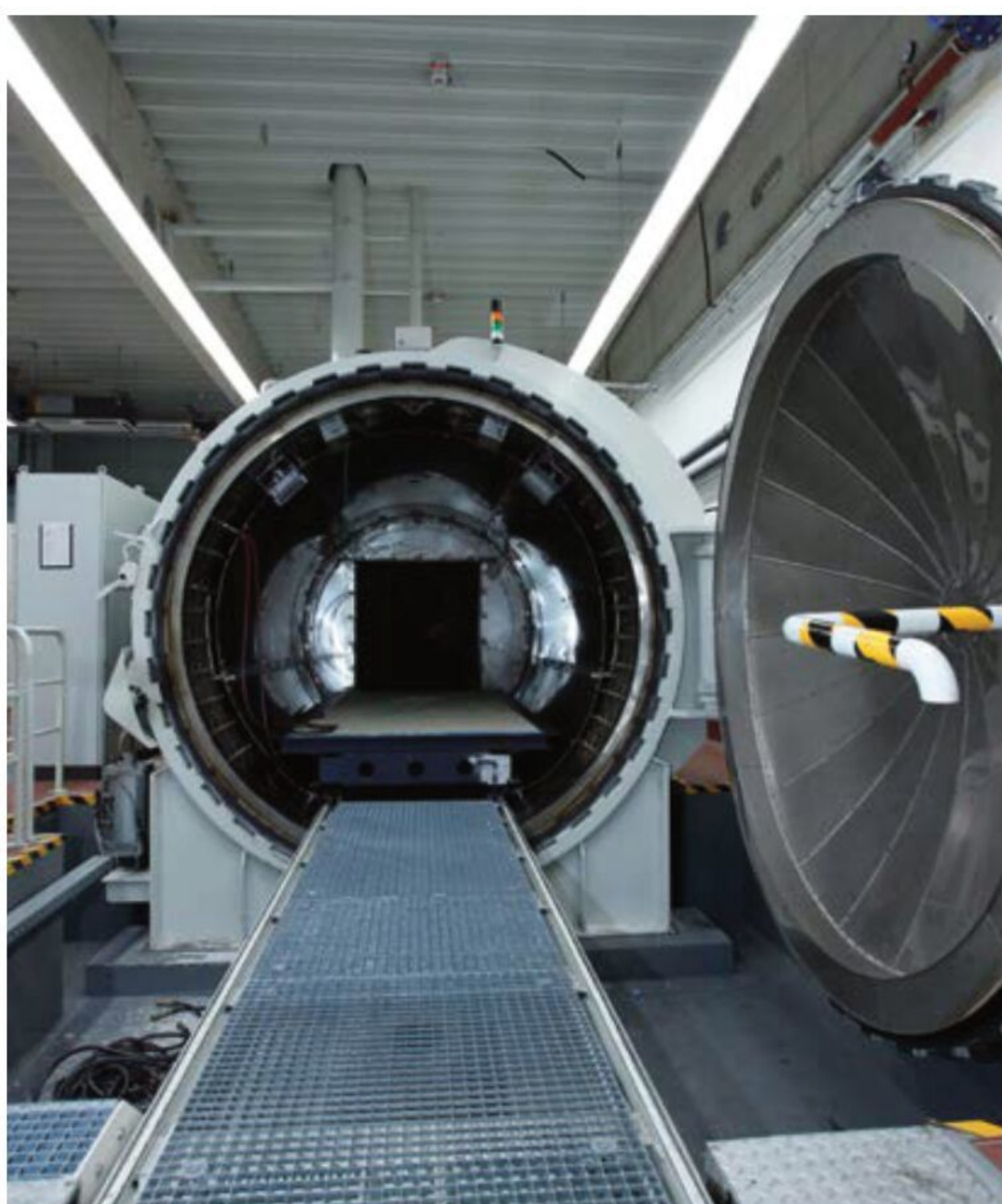
A sizeable autoclave is required for curing monocoque structures
