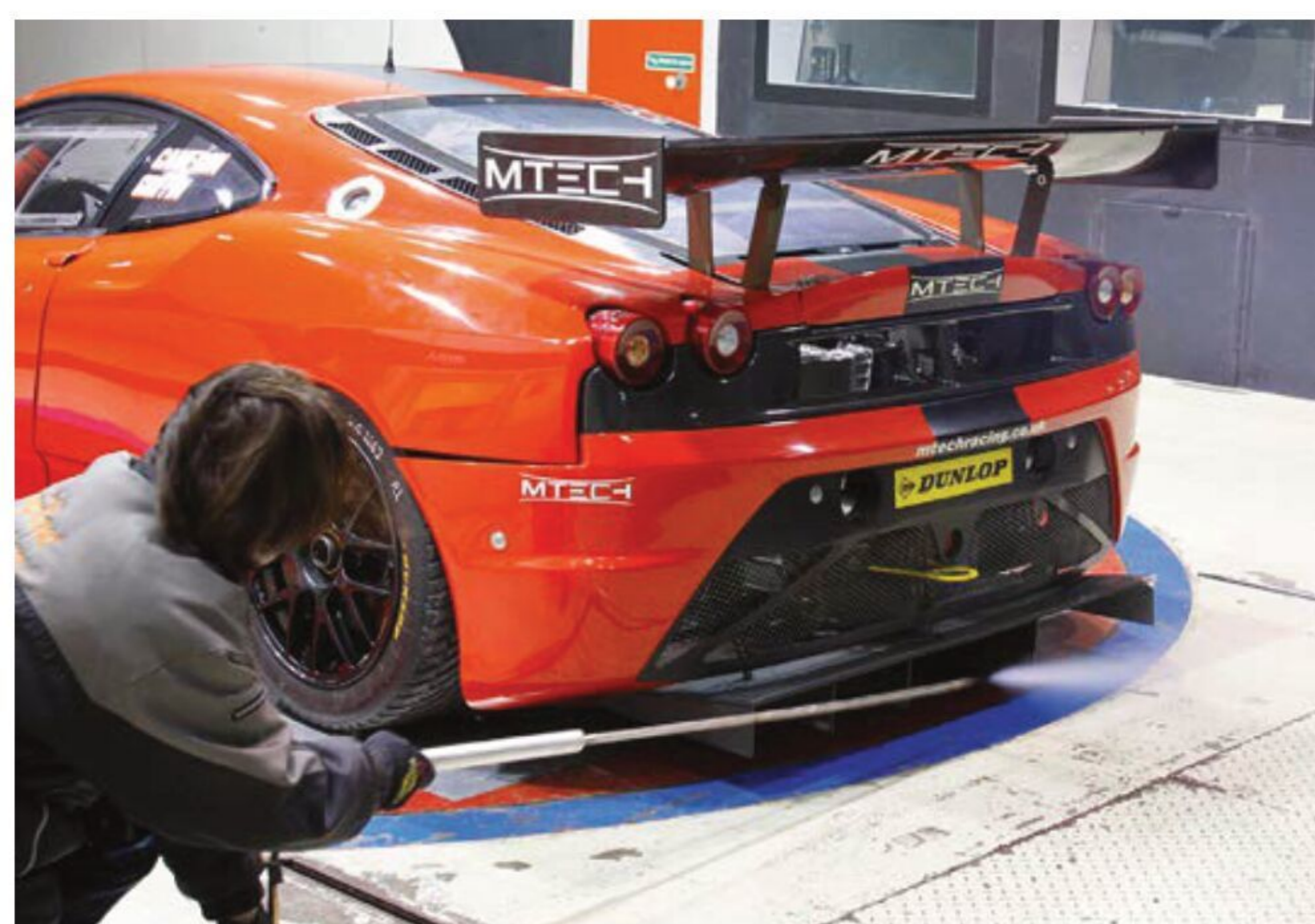
The flow from the Ferrari F430 Scuderia GT3's diffuser centre was seen to be tidy...
