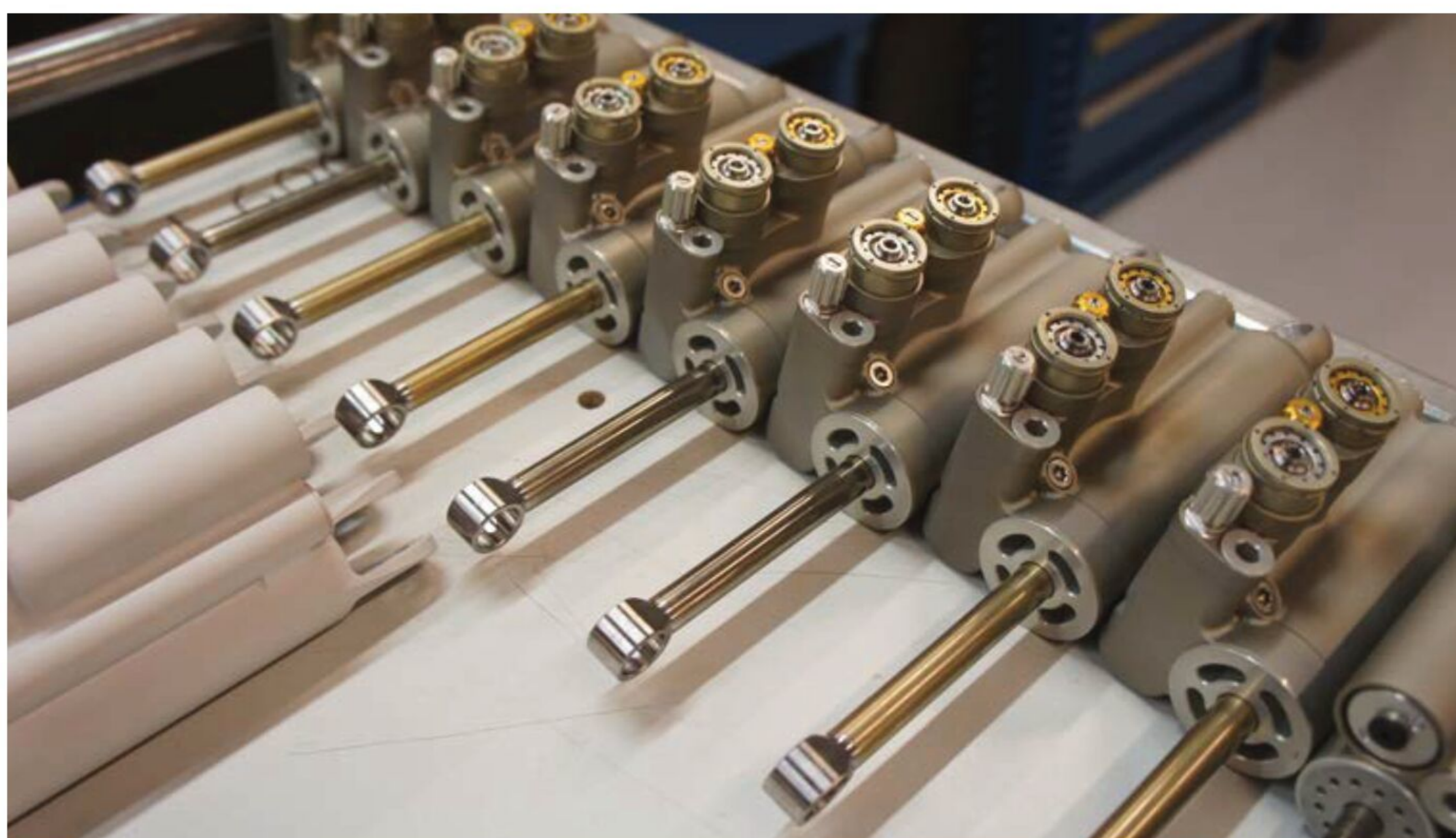
F1 dampers are used by competing teams to influence aerodynamic performance and also to control tyre temperatures
