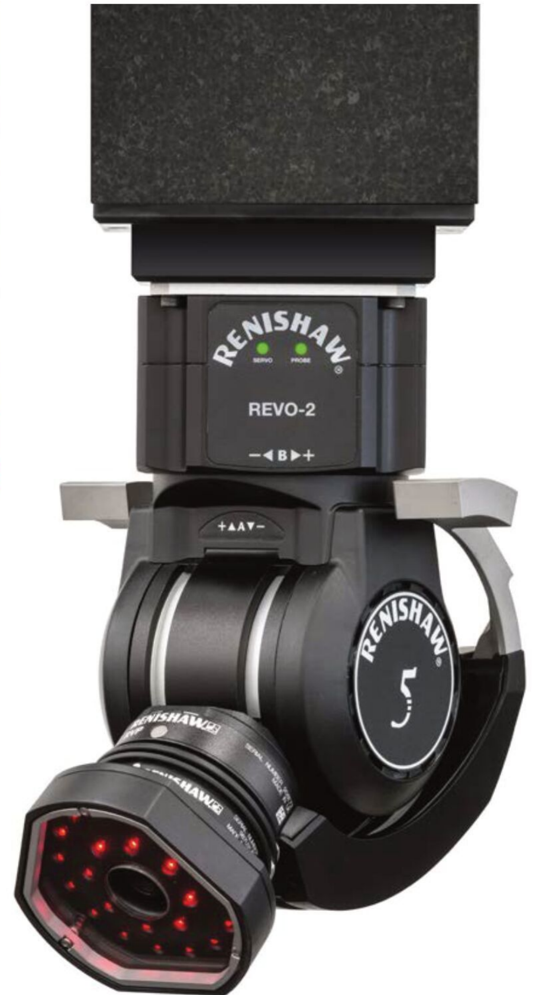
Non-contact vision probes can also be used on five-axis coordinate measurement machines, allowing the measurement of 0.5mm diameter holes, for example. A 1.3 megapixel global shutter CMOS sensor and digital signal processor are used and the grey-scales of the images translate into spatial data
