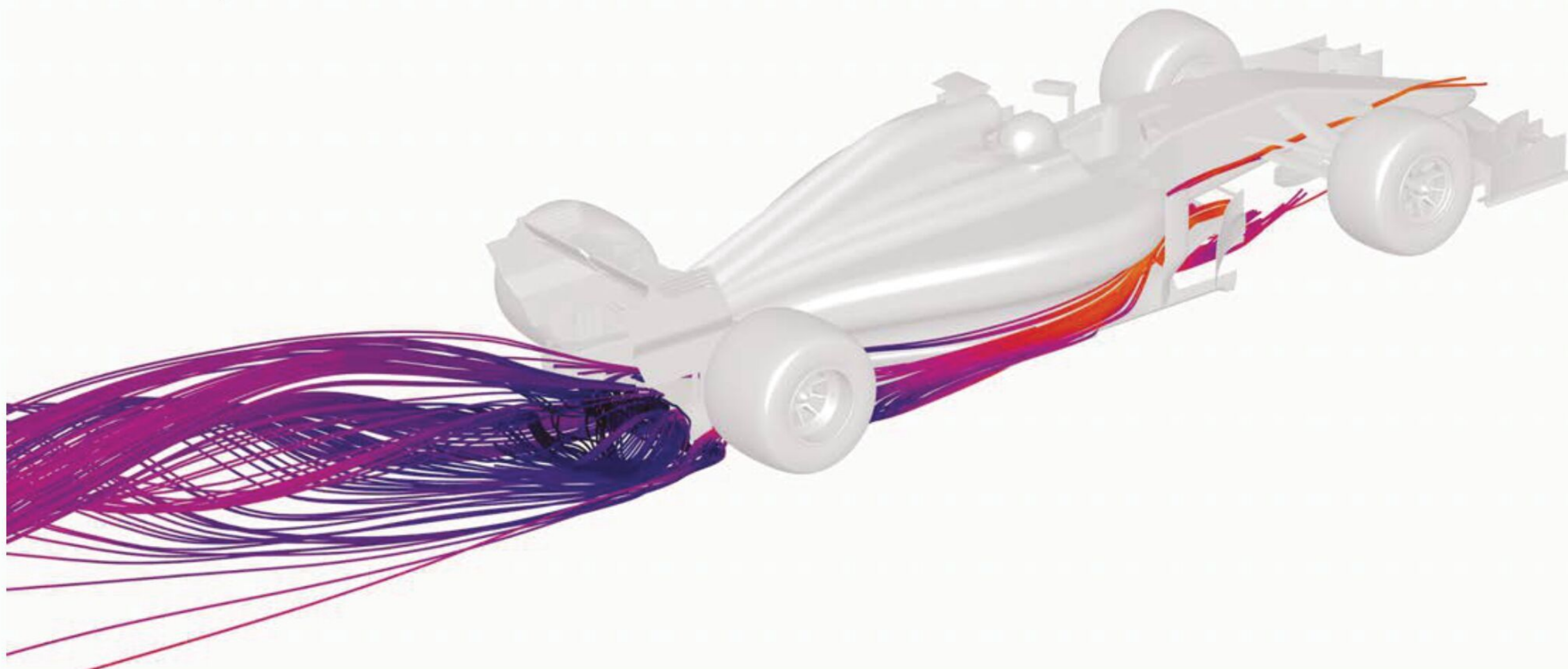
CFD showing the air stream underneath a formula car, and exiting at the diffuser
