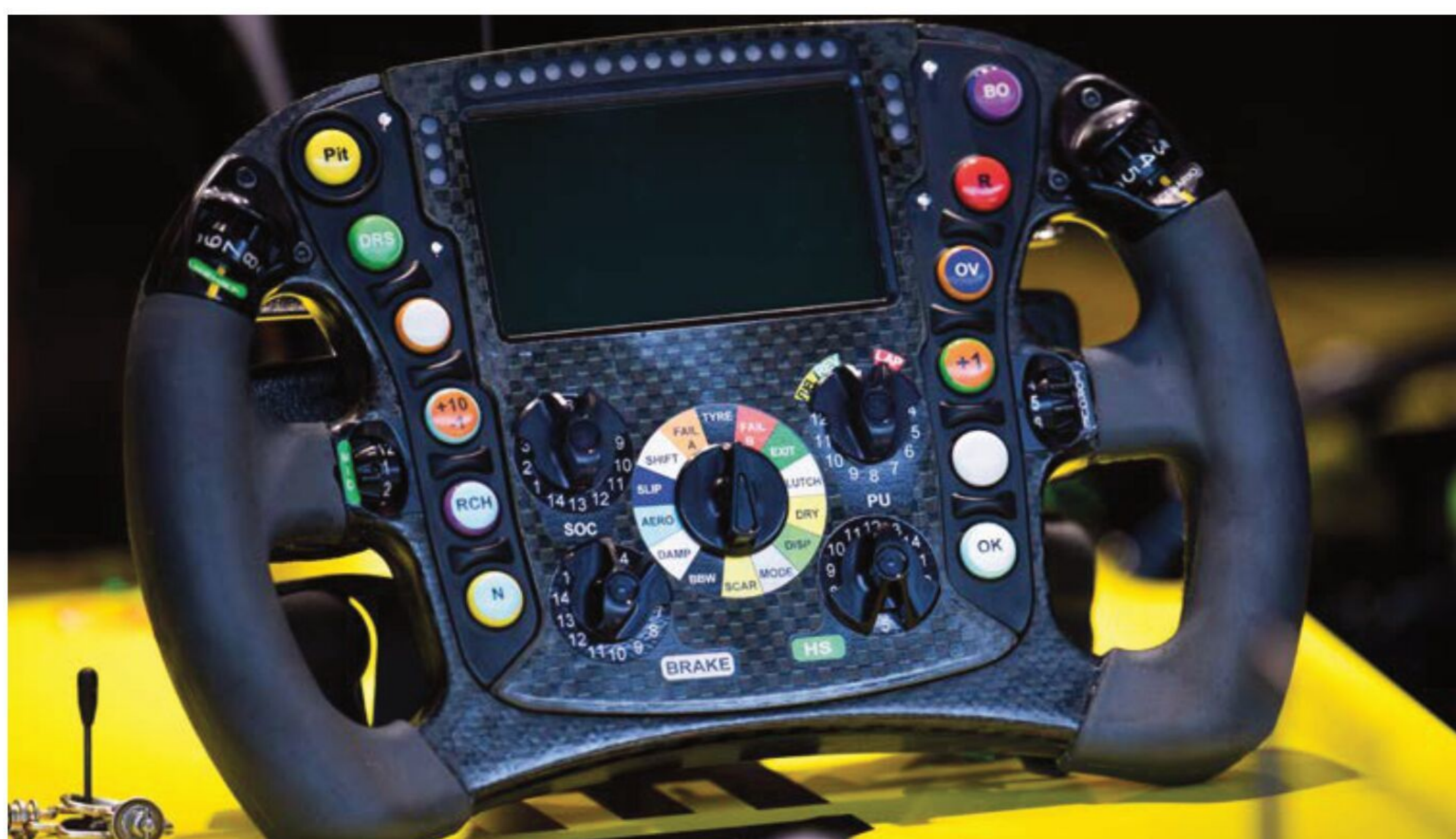
On modern, high-level racecars, most of the readouts and many of the switches are positioned directly on the steering wheel
