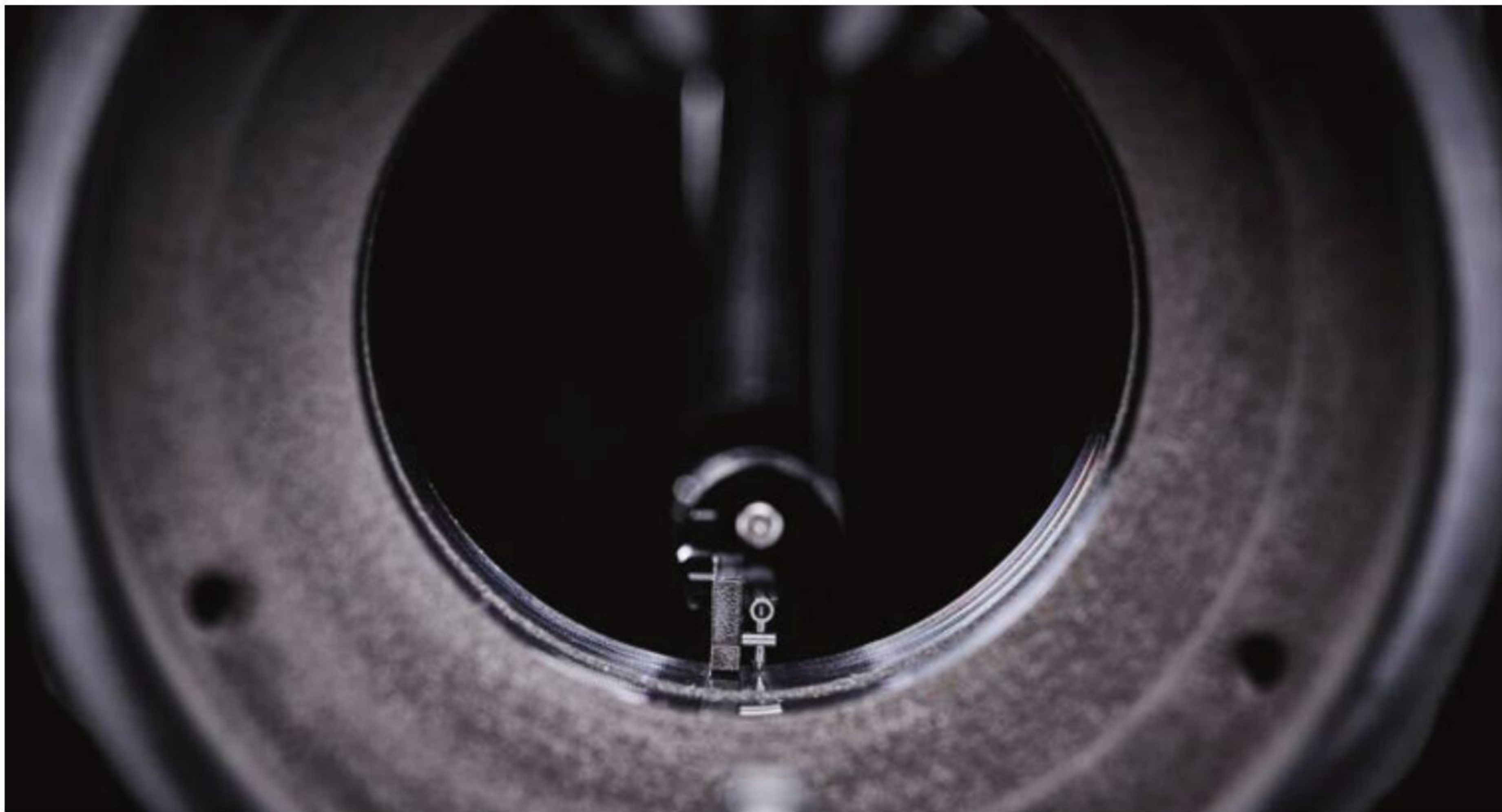
The SFP2 consists of a two micron radius diamond tip that deflects vertically as it's dragged across the surface of the component, going across the grain of the machining, thereby generating the signal in a similar way to a record player
