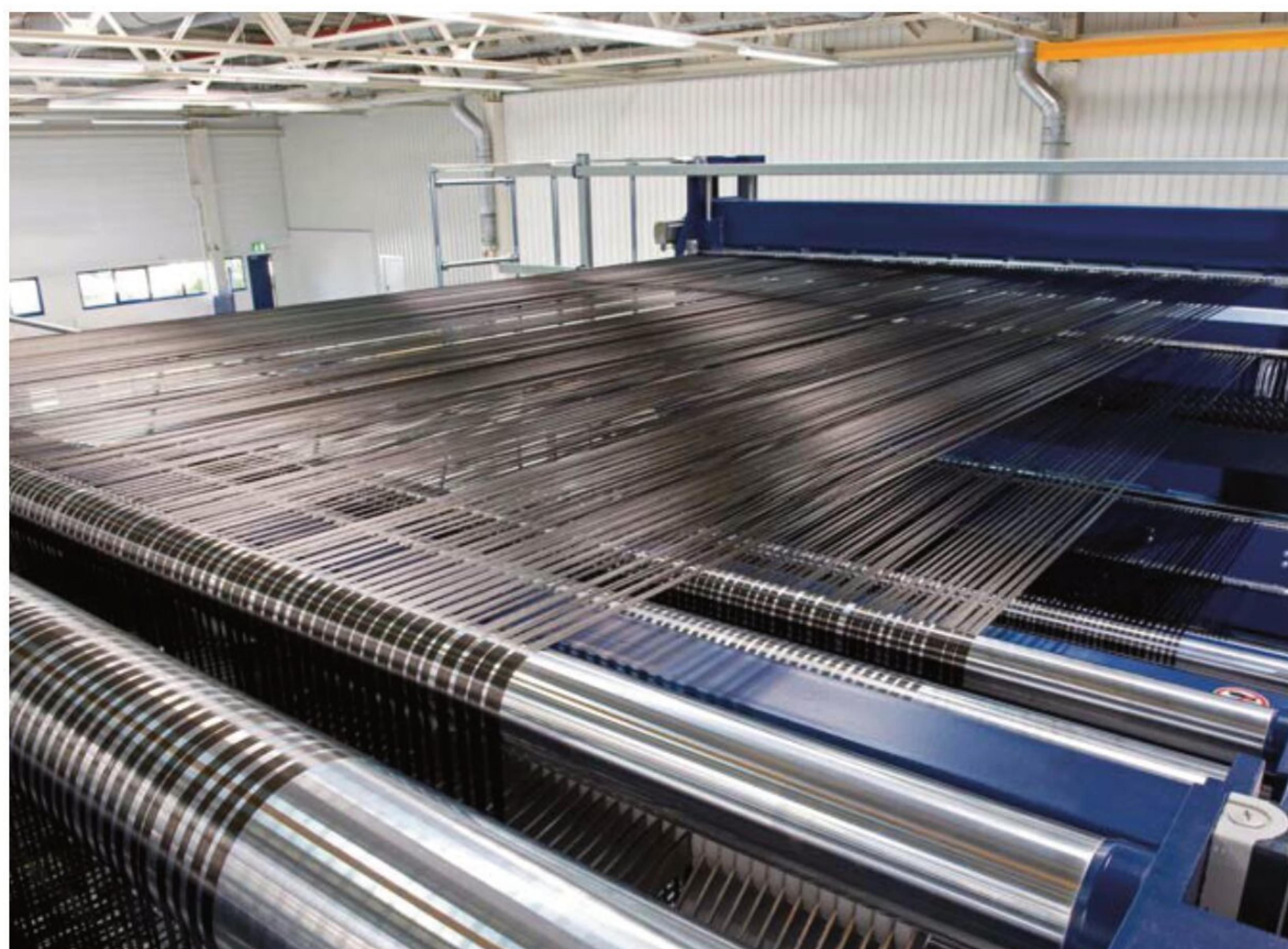
The similarity to a wool loom is not coincidental, composite strands are woven together on just such a device
