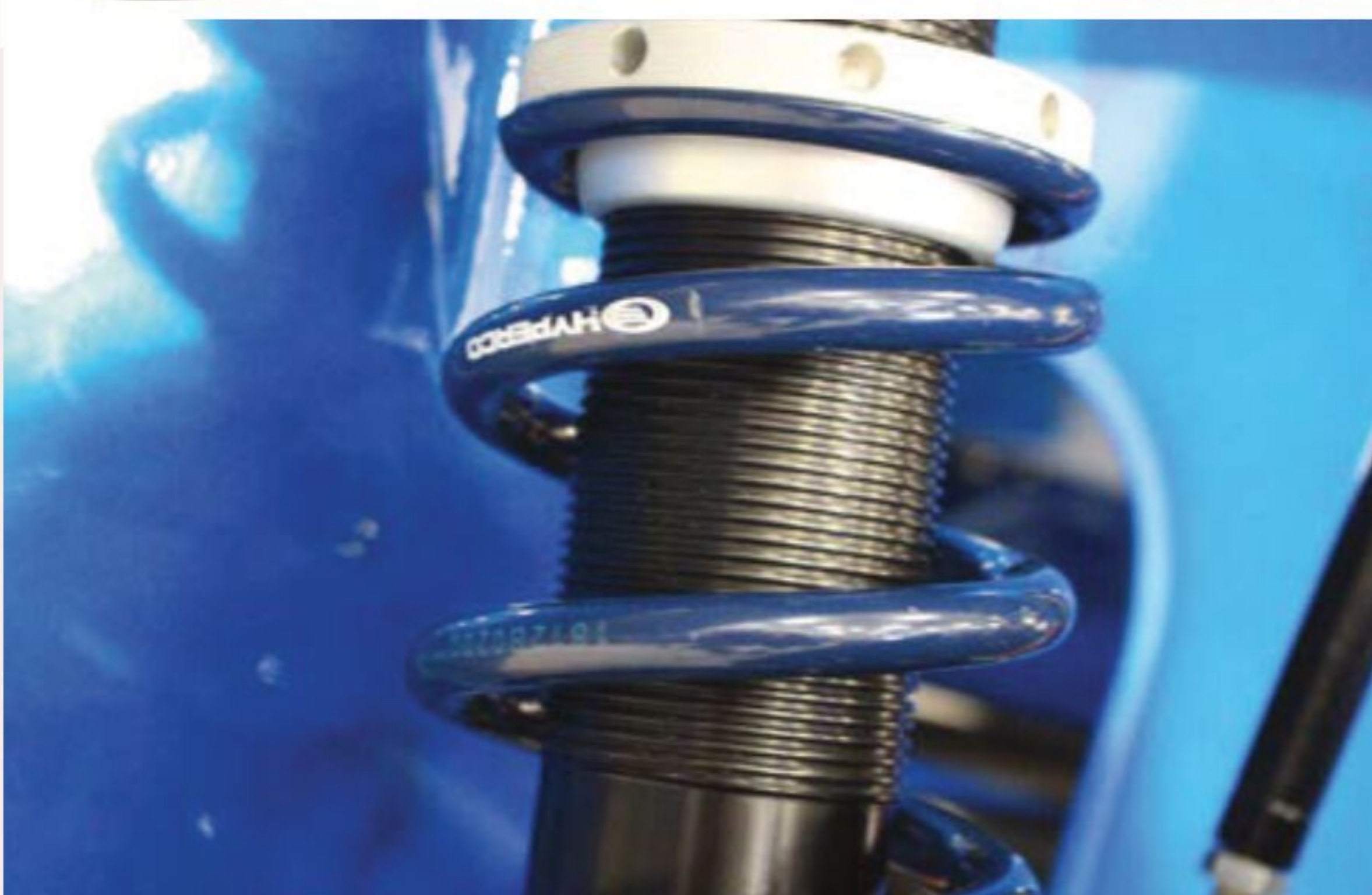
Spring perches on a coilover shock are not parallel, but sit at a slight angle
