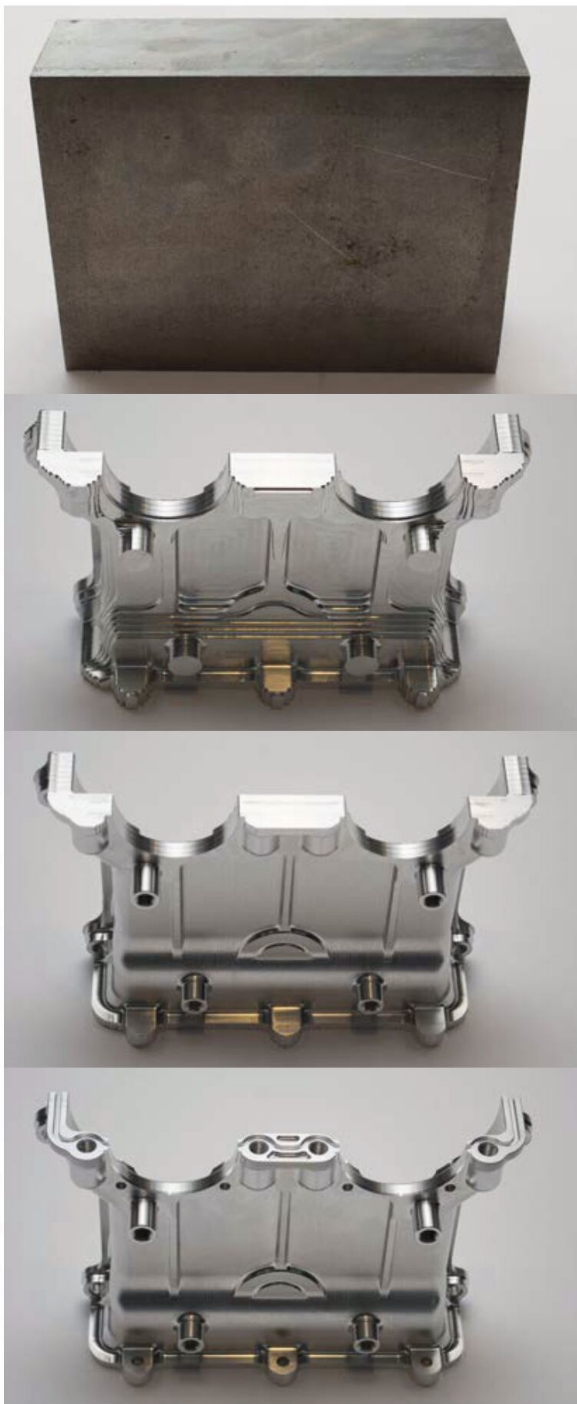
Five-axis machines have the capability to machine a part from start to finish, creating intricate shapes out of a billet of material
