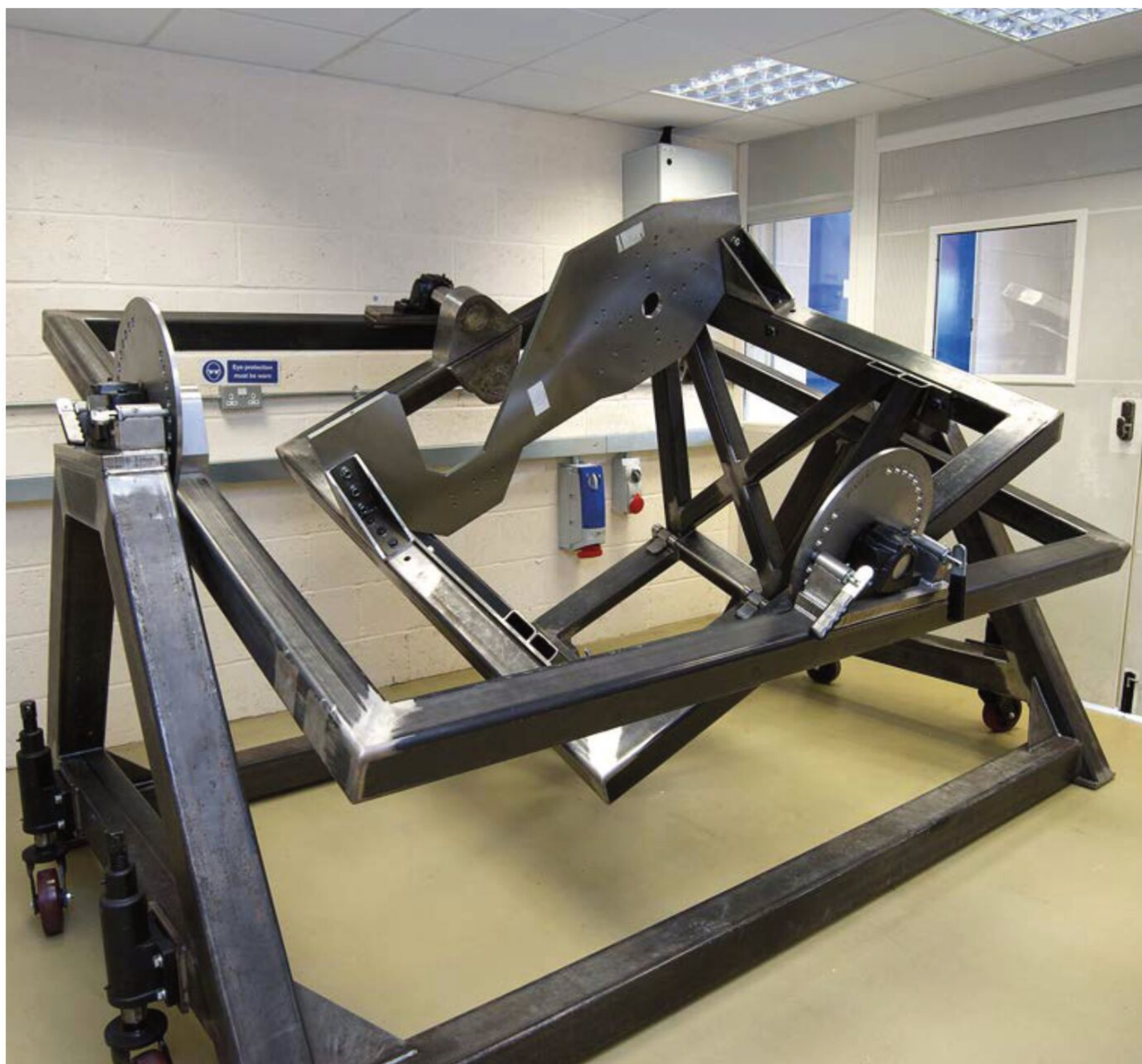
The gearbox's lubrication regime is tested on rotating rigs to understand how it stands up to the g forces seen in racing
