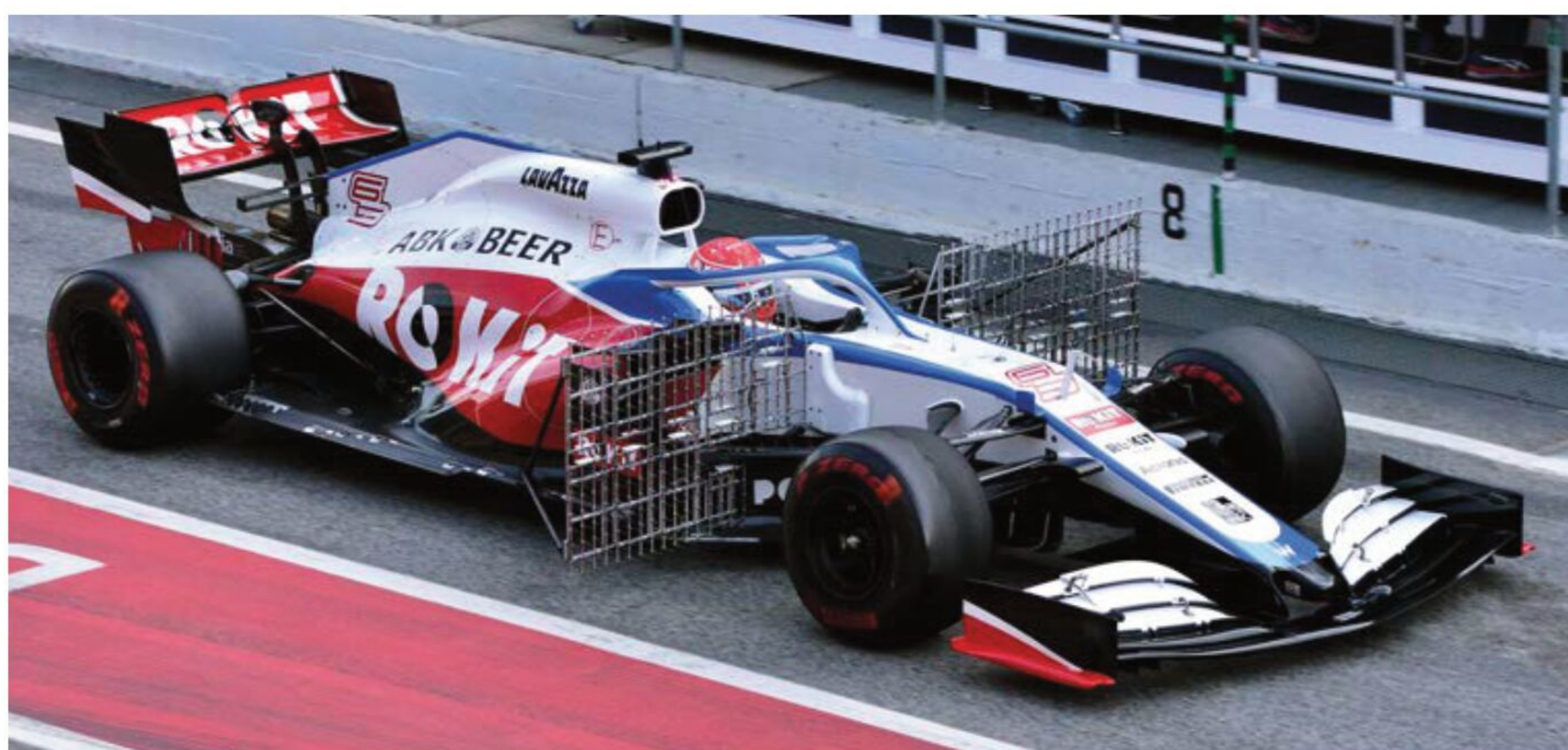
As often seen in Barcelona, all manner of measurement apparatus appear in efforts to correlate lab and CFD methods
