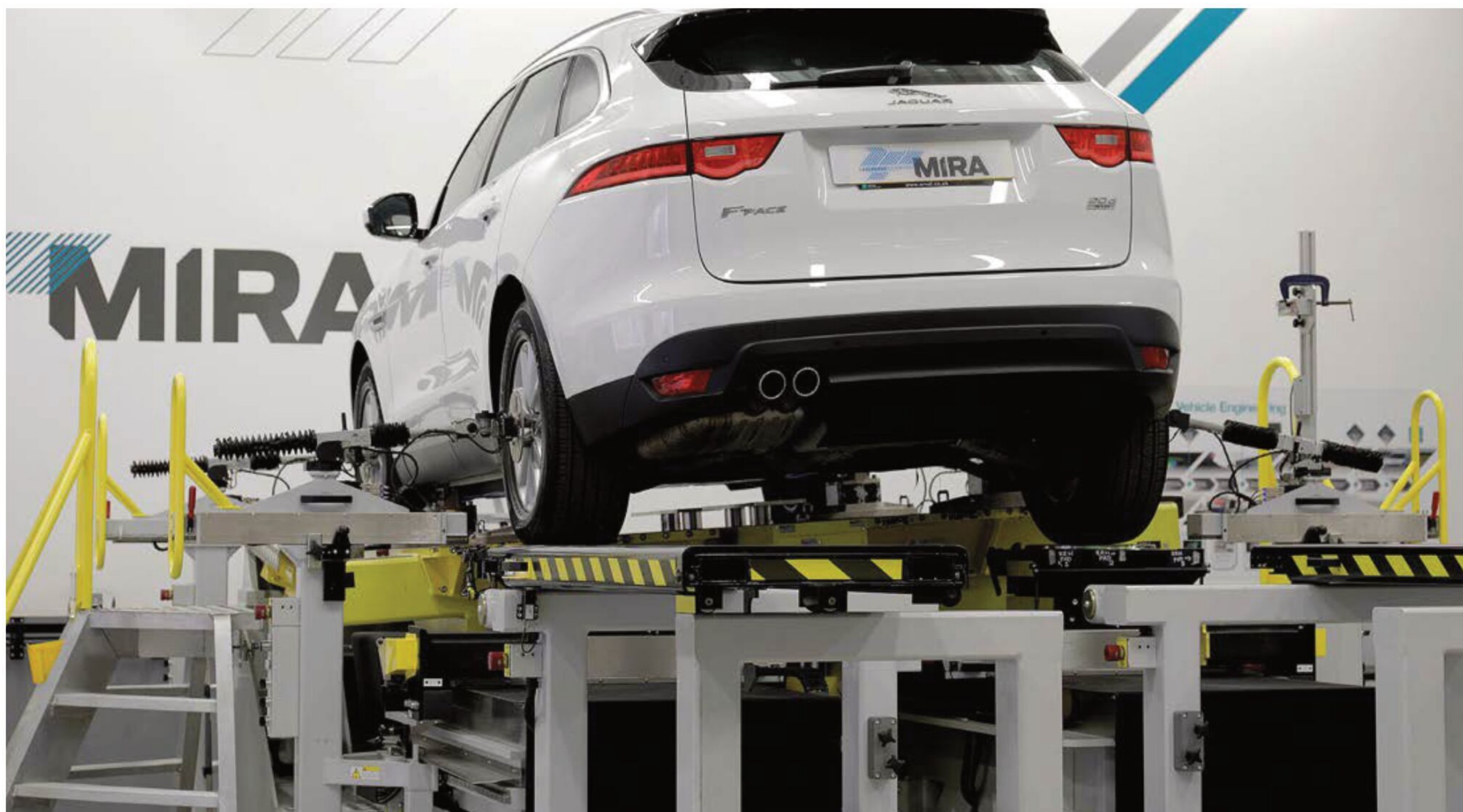
MIRA's K&C rig can simulate the forces and loads placed on a vehicle's suspension system within a controlled and repeatable environment. Roll is being replicated here
