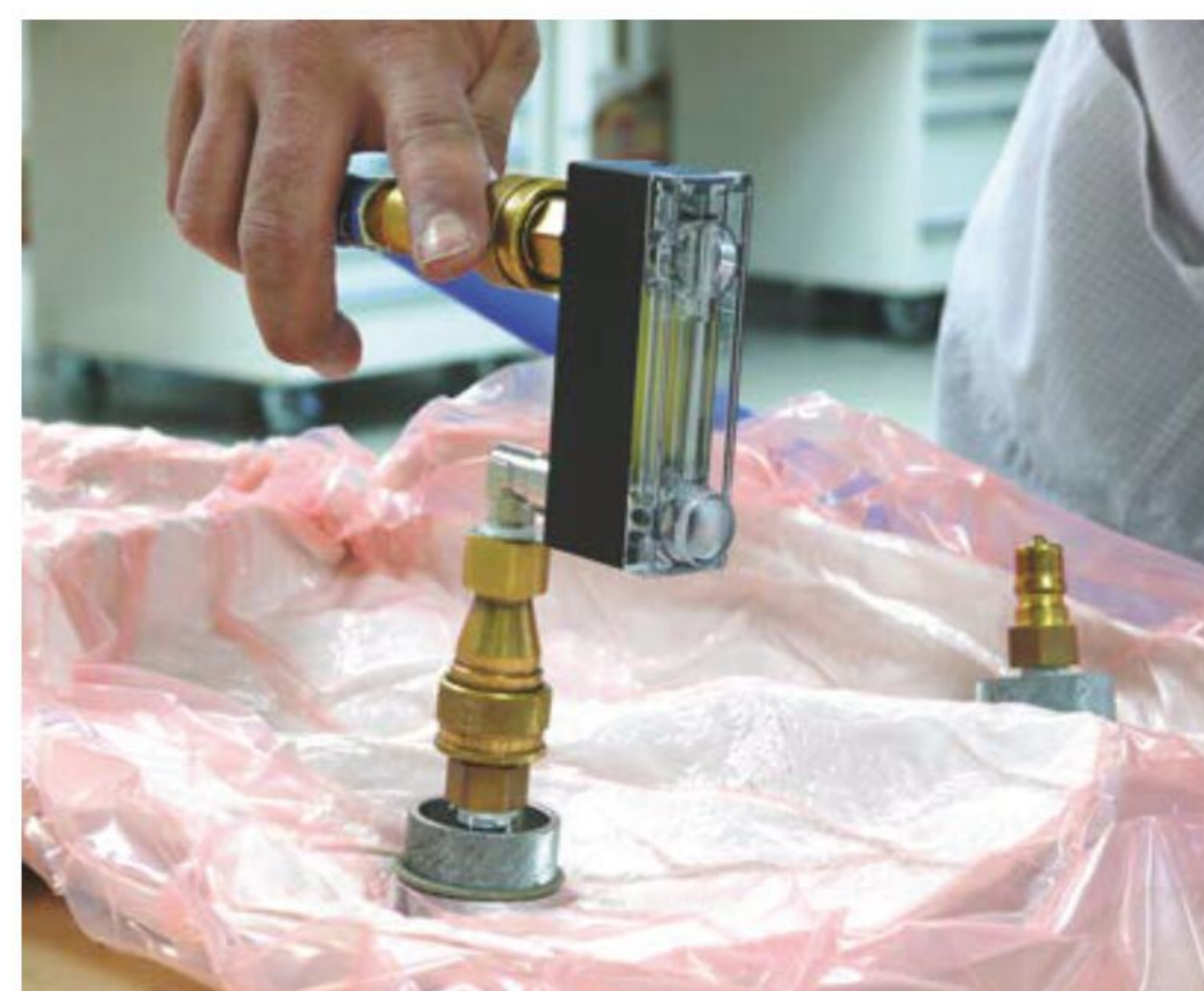
Composite parts are placed into a vacuum bag prior to curing
