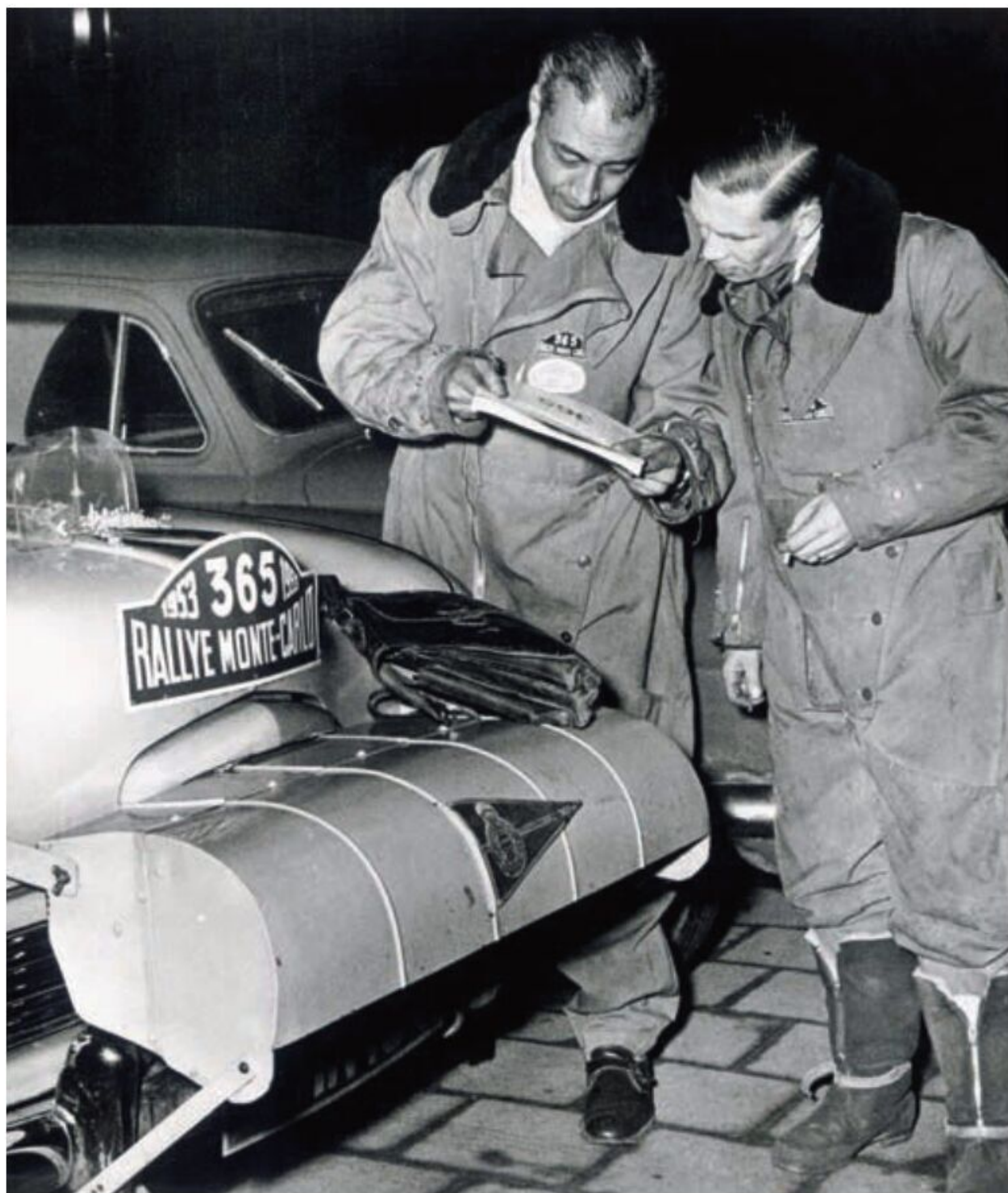
Gatsonides and Worledge in working kit ready for the start of the rally. The vast cowl at the front of the Zephyr is to stop stray light from the foglamps dazzling Gatso himself.
