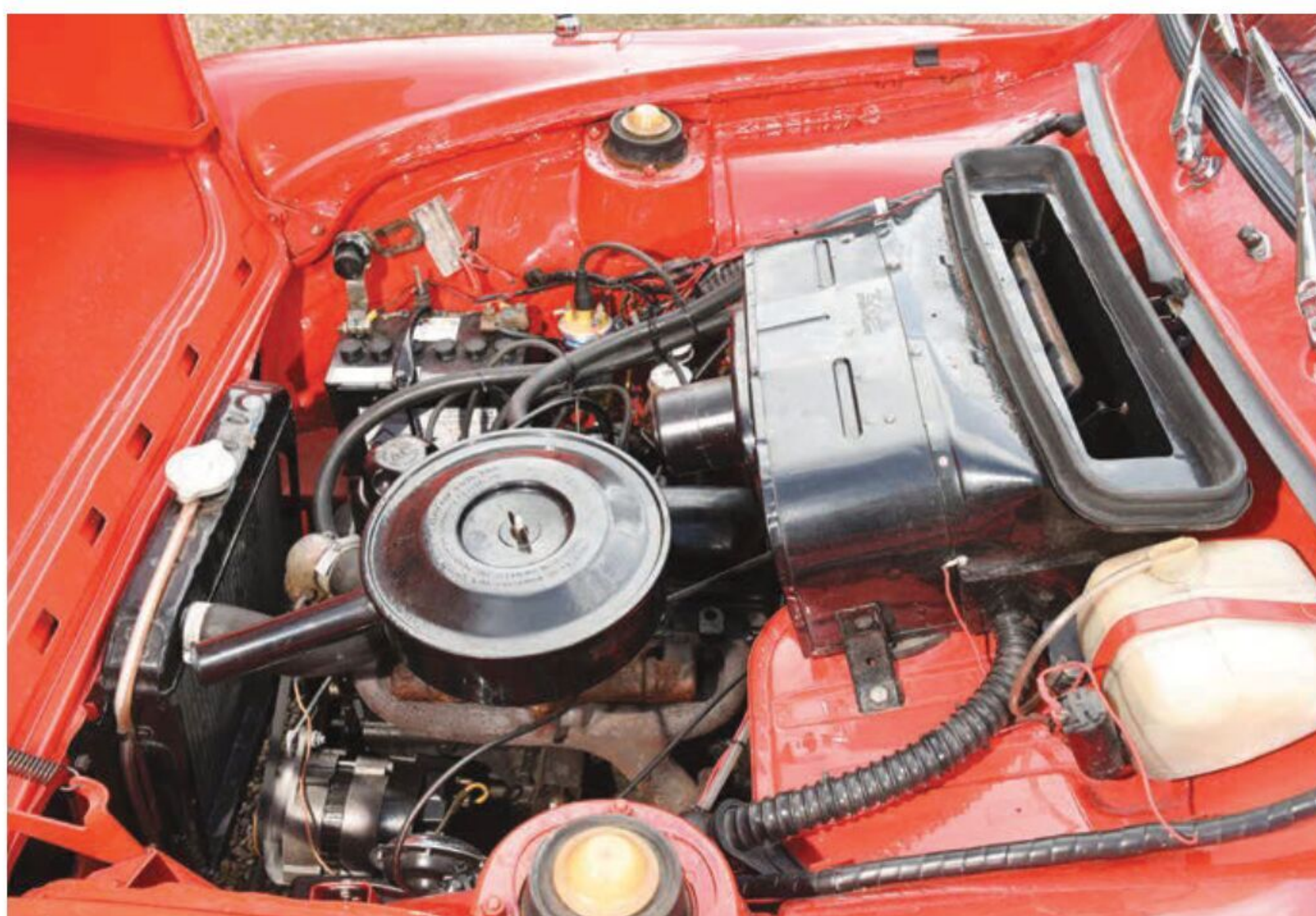
The 105E Anglia's overhead valve engine was a huge improvement over the previous model's sidevalve unit.
