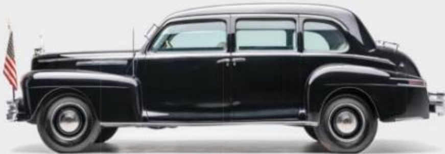
FIRST FACTORY ARMOUR PLATED PRESIDENTIAL LIMO MADE FOR FDR 1942 Lincoln Armored Limousine, H Series
