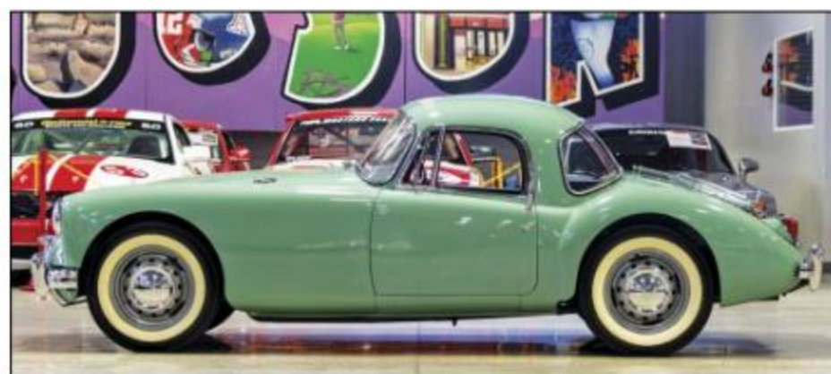
1958 MG MGA- Island green over black leather interior, BMC B-series supercharged 1489 cc 4cyl, 4-speed manual trans, 1 of 773 produced, Judson supercharger, rack and pinion steering, front independent coils, rear semi elliptic springs, chrome rear cargo rack, period correct white-wall tires, alloy wheels. $44,929 Stock #C0116 Crown Concepts (520) 900-7586
