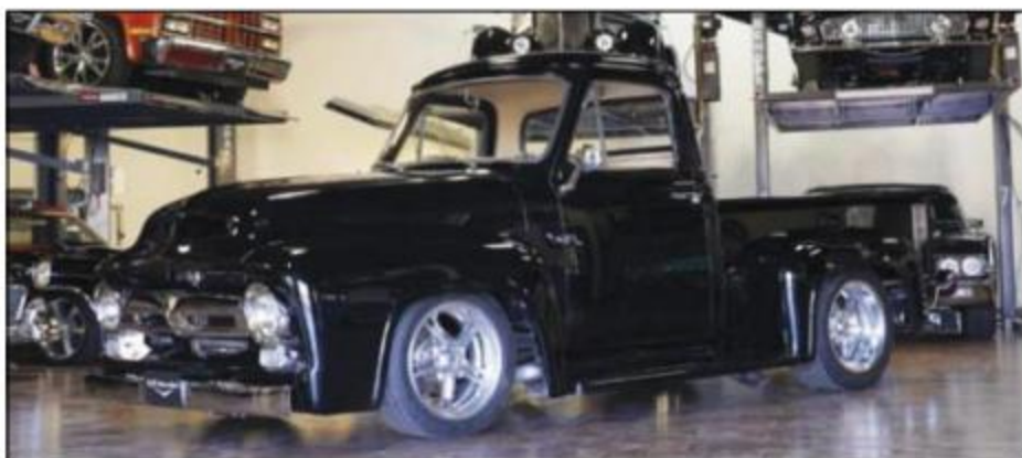
1954 Ford F100 - Black over tan leather, 502 hp 502 cu. in. V8, 4L60E auto trans, frame-off custom build, Compushift electronic control module, electronic fuel injection, Tunnel Ram intake, Sanderson Headers, Vintage Air A/C, 4 piston Wilwood disc brakes all round, 11" drilled and slotted brake rotors, custom wheels, award winner. $83,900 Stock #10180053 LC Classics (480) 925-8723
