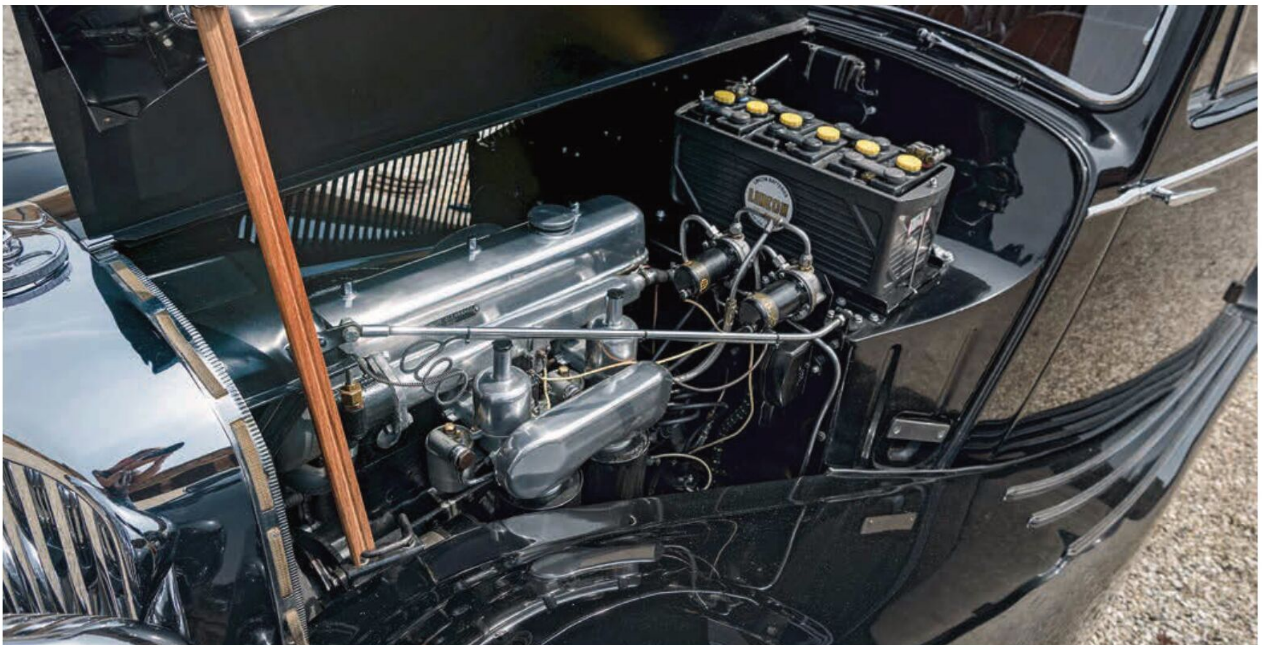
3.5-litre engine still a warmed-over Standard unit, but with automatic chokes. Wood bonnet stay a recent, and useful addition.
