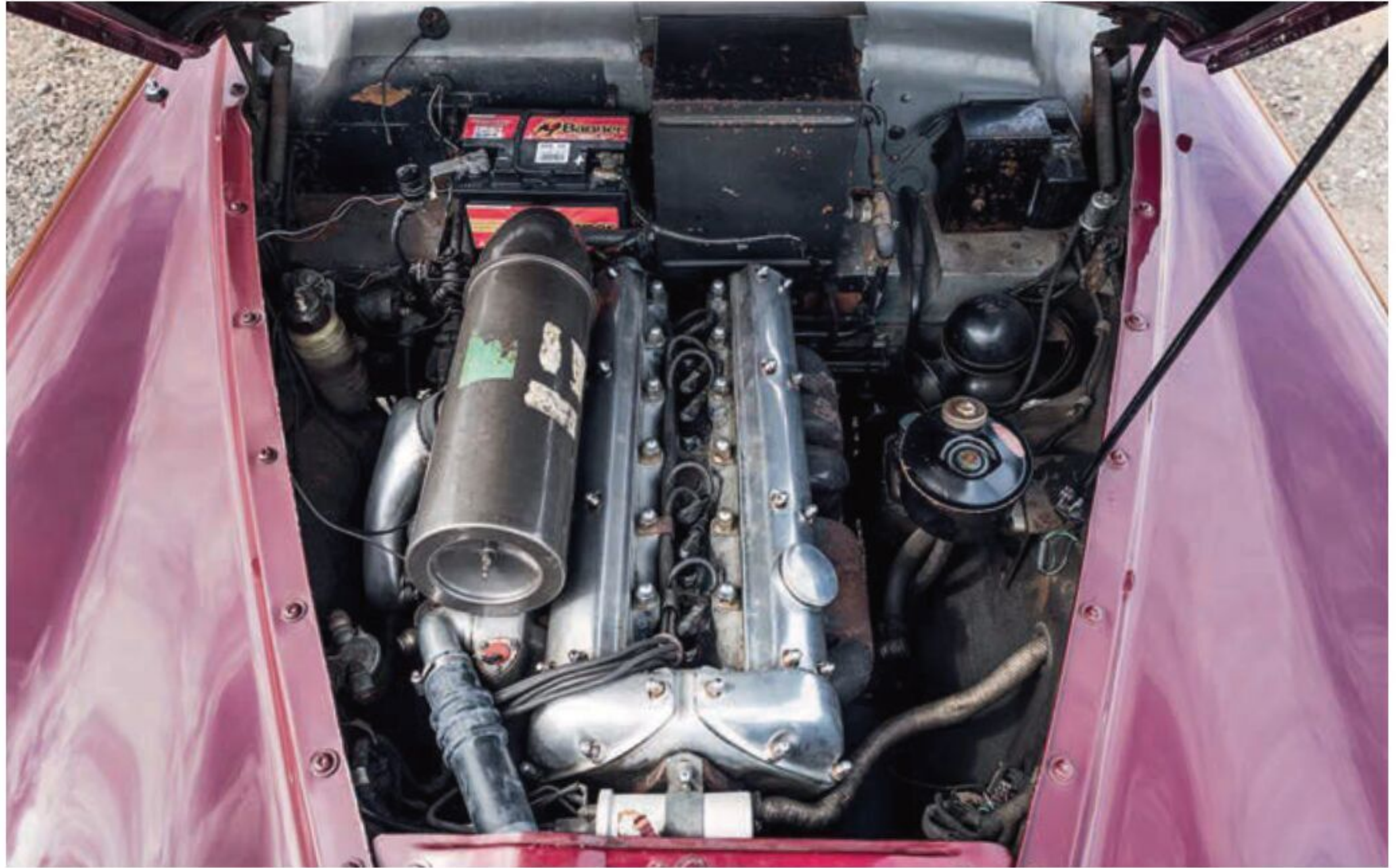
XK engine in 3.4-litre form, but with power steering now fitted.
