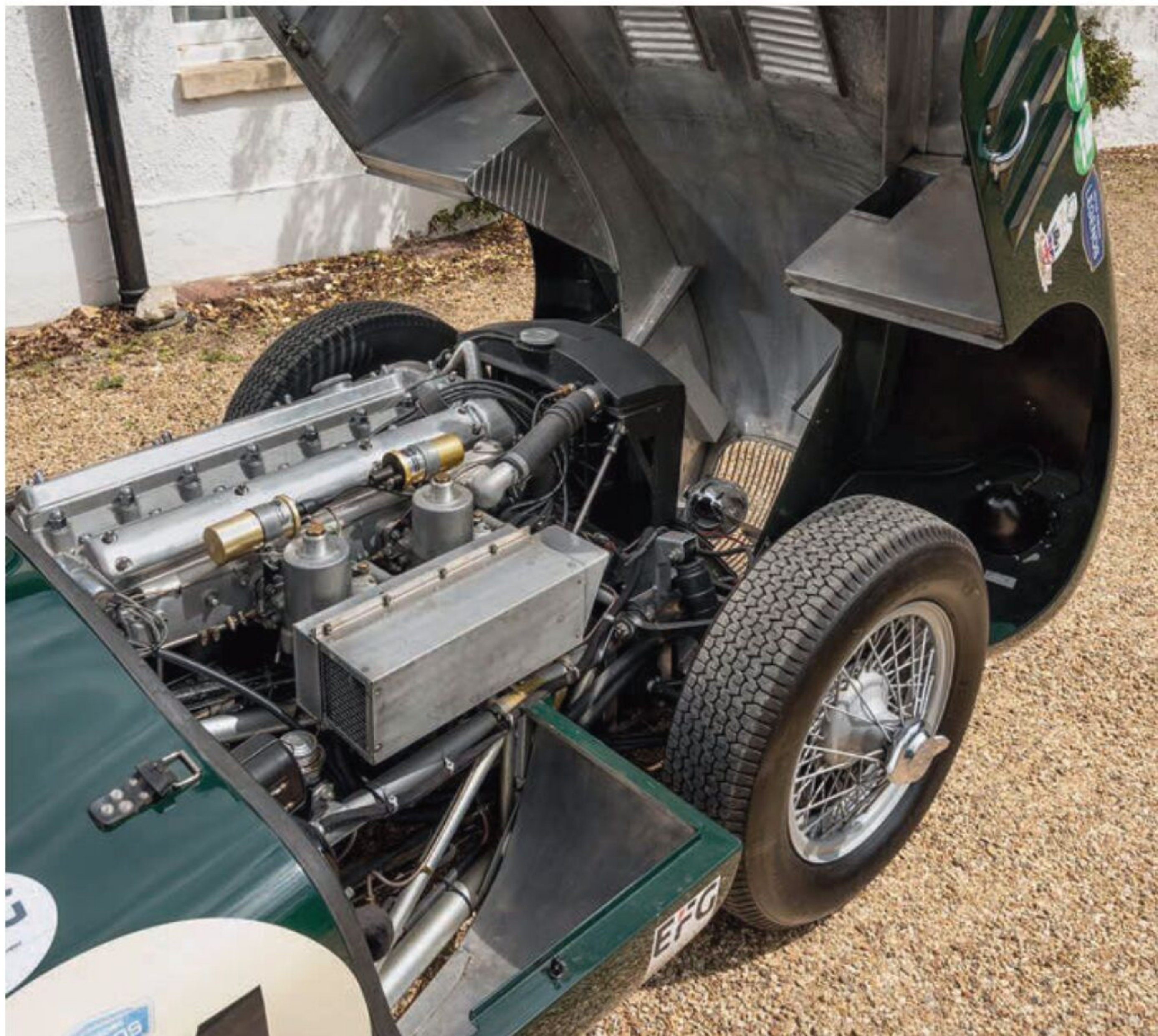
The engine was rebuilt and uprated to full race spec by Sigma Engineering.
