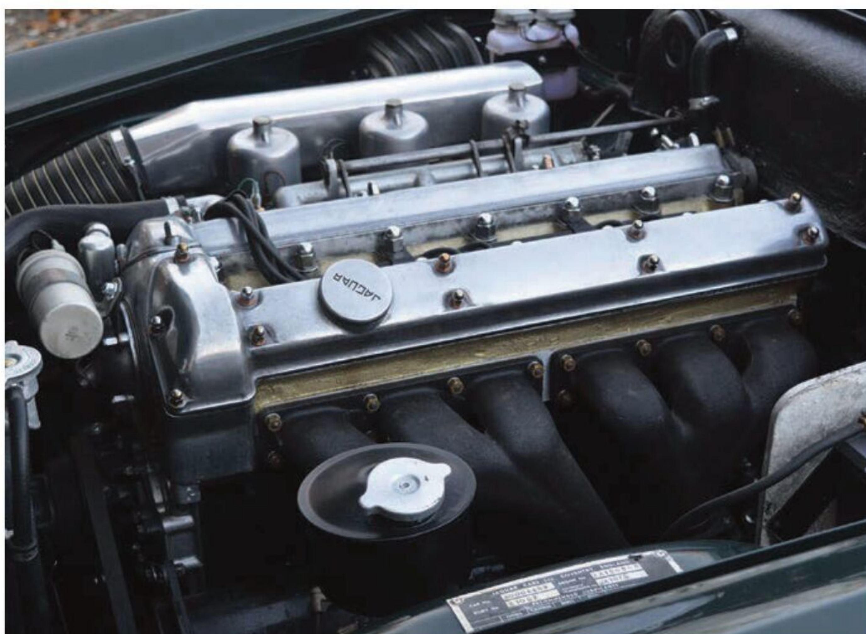
The seized 3.8-litre engine was rebuilt by XJK, in Staffordshire.
