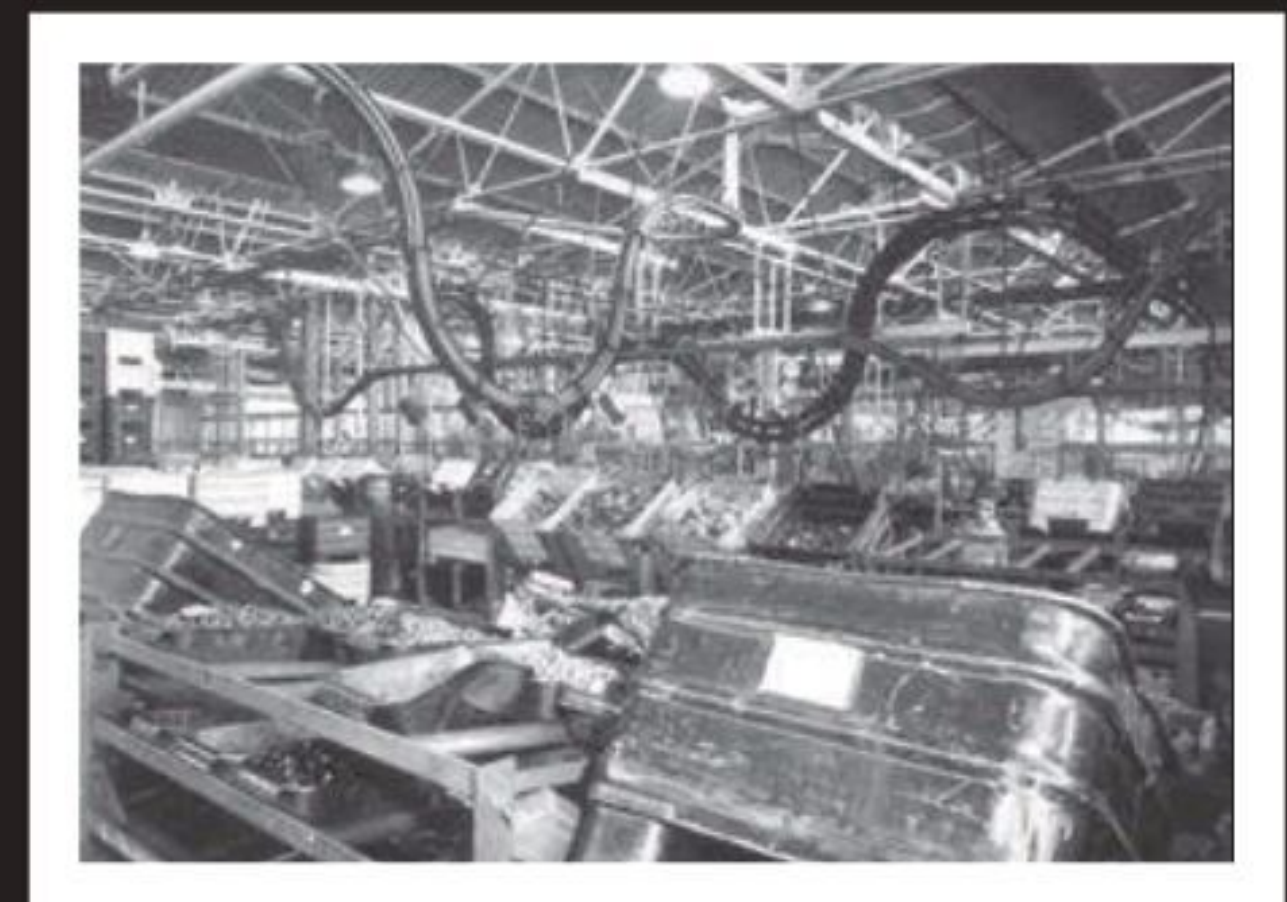
ABOVE LEFT: These CKD packs at Zetland may have contained parts to build Morris Minors, but the MGAs would have been received in much the same way. Engine components would have been assembled at Zetland, while chassis and body panels would have gone straight to Pressed Metal Corporation at Enfield.
