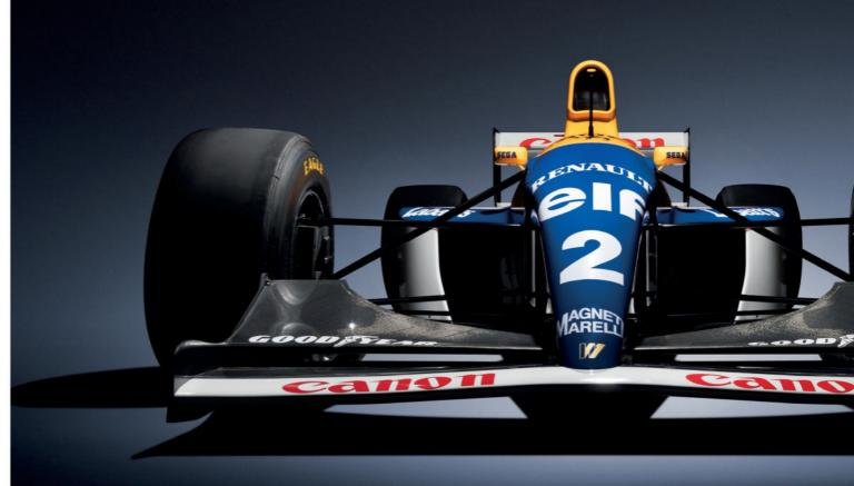
aerodynamics. "The active ride was a sort of responsive system," says Head. "In that if you had load transfer, like when you hit the brakes, the nose would dip and the back would go up. Then the system would say, 'I don't really want this,' and would correct it. And when you turned into a corner, the car would initially begin to roll. And then the system would say, 'I don't like this - this is not what I'm programmed to do,' and it would correct it."
