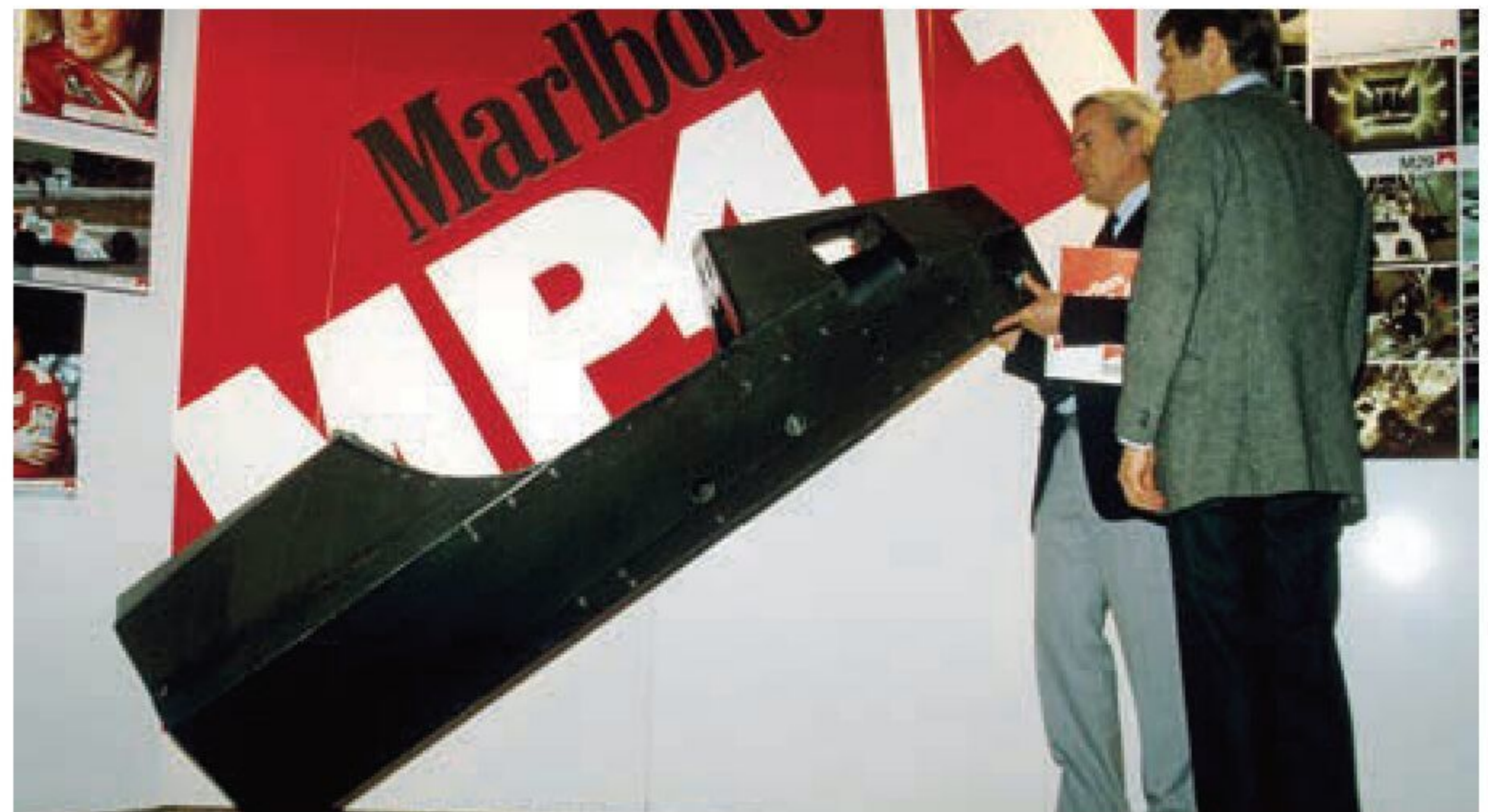
P18 Star car: A new way of thinking Grand prix racing's ground-breaker, the carbonfibre McLaren MP4/1, by Matt James
