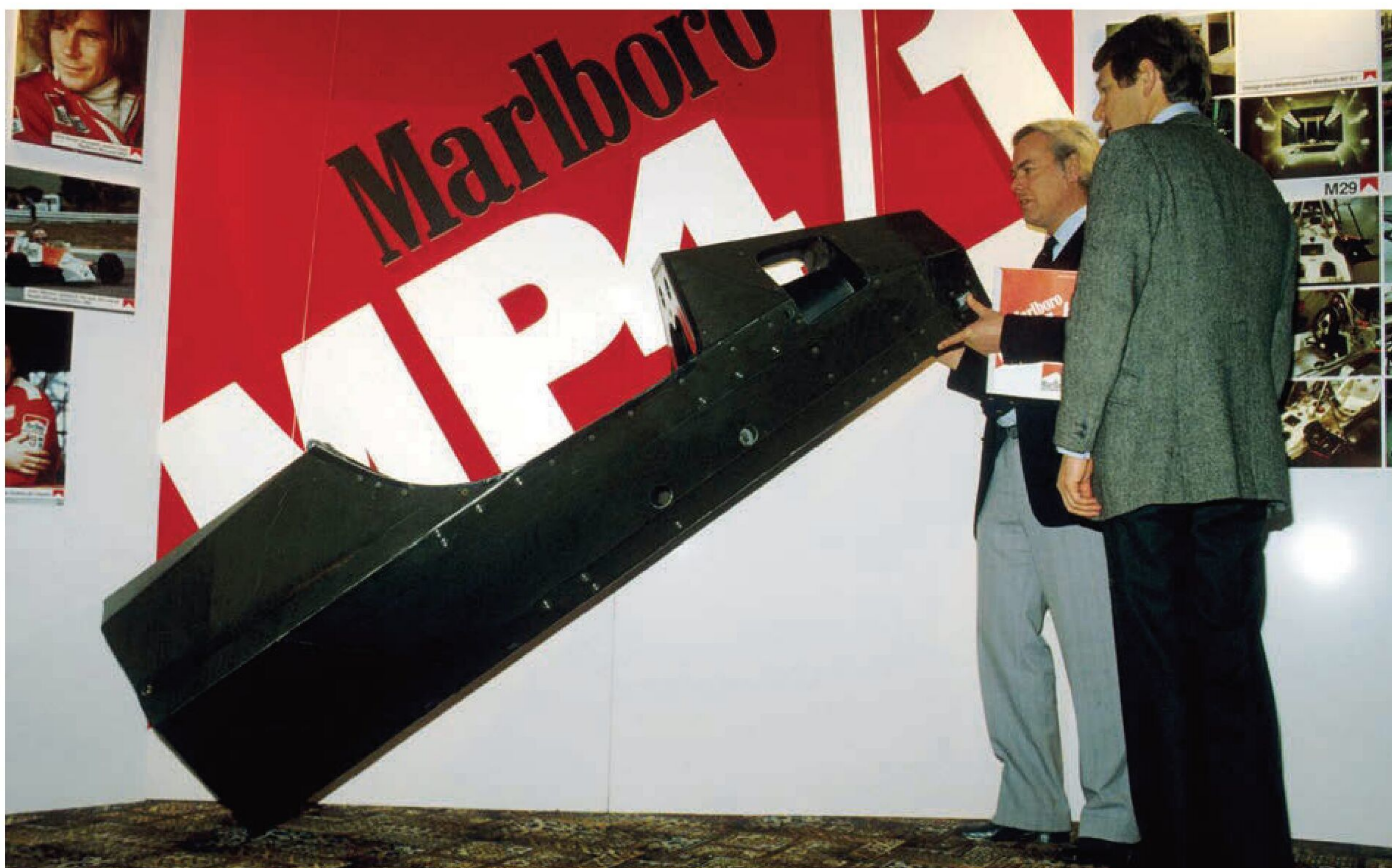
Super-light and super-strong: the Hercules-built monocoque of the MP4/1 was a revelation for Formula 1 designers
