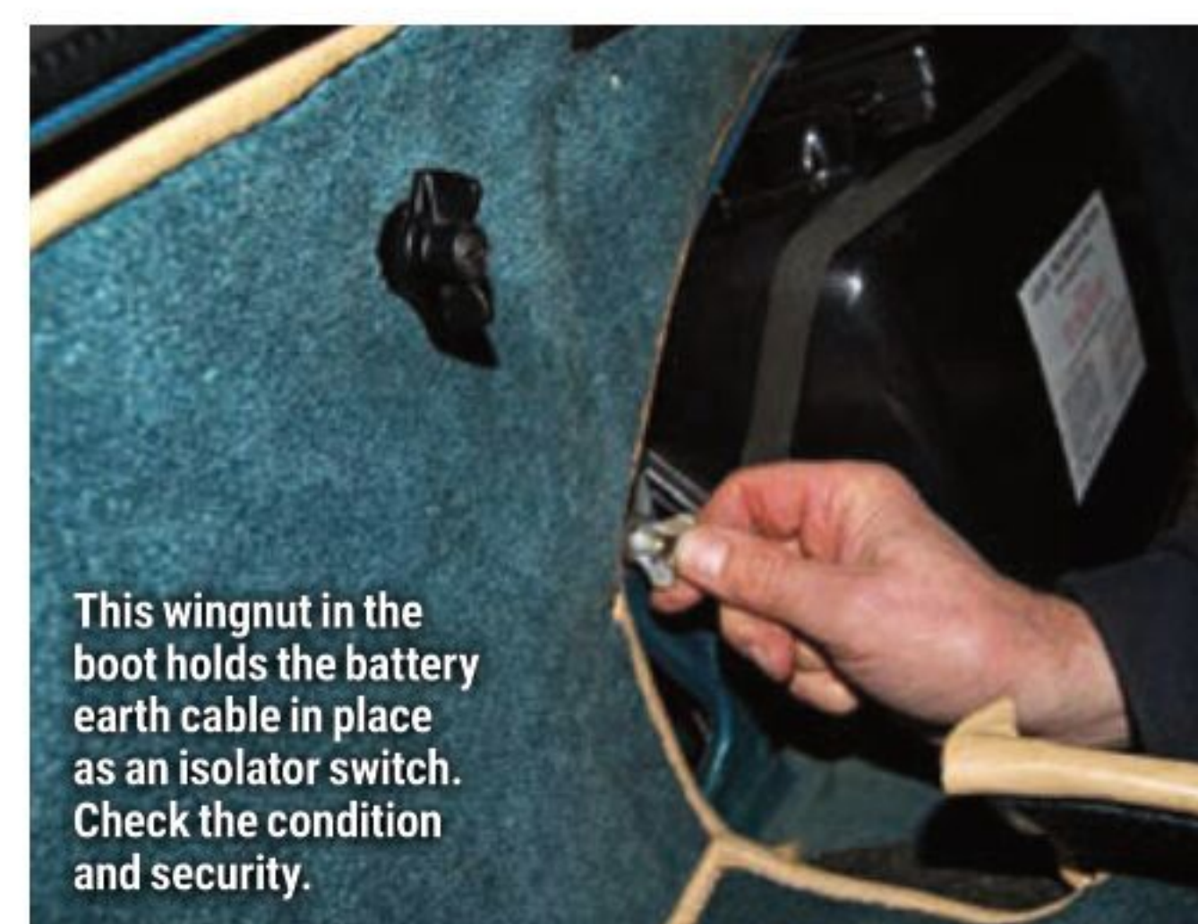
Removing the boot trim allows inspection of the inner wing structure and the tail wiring.
