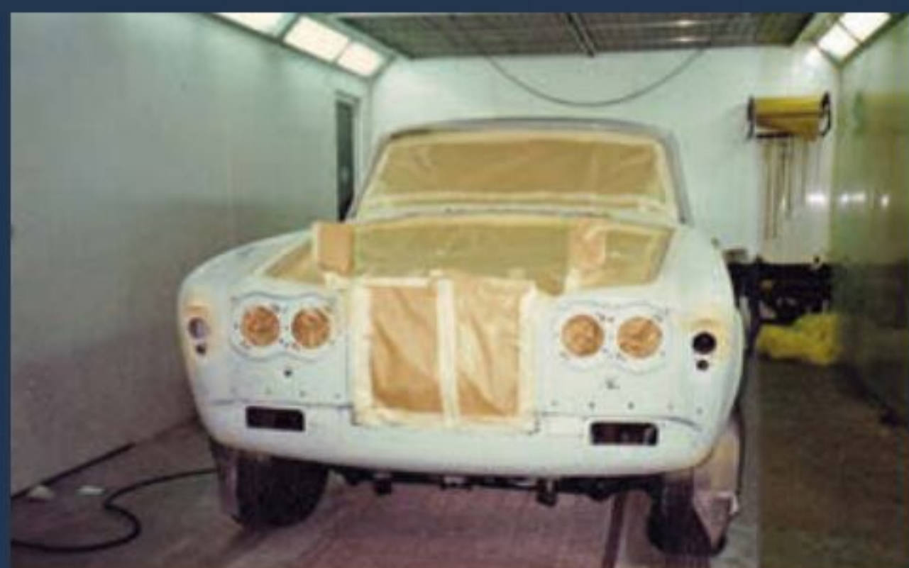
The bare rolling bodyshell was given several coats of primer after final panel alignment
