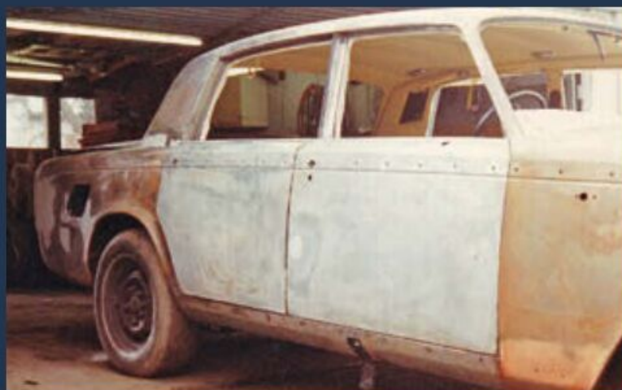
One rear door was replaced, and new front wing bottom sections were skilfully fitted
