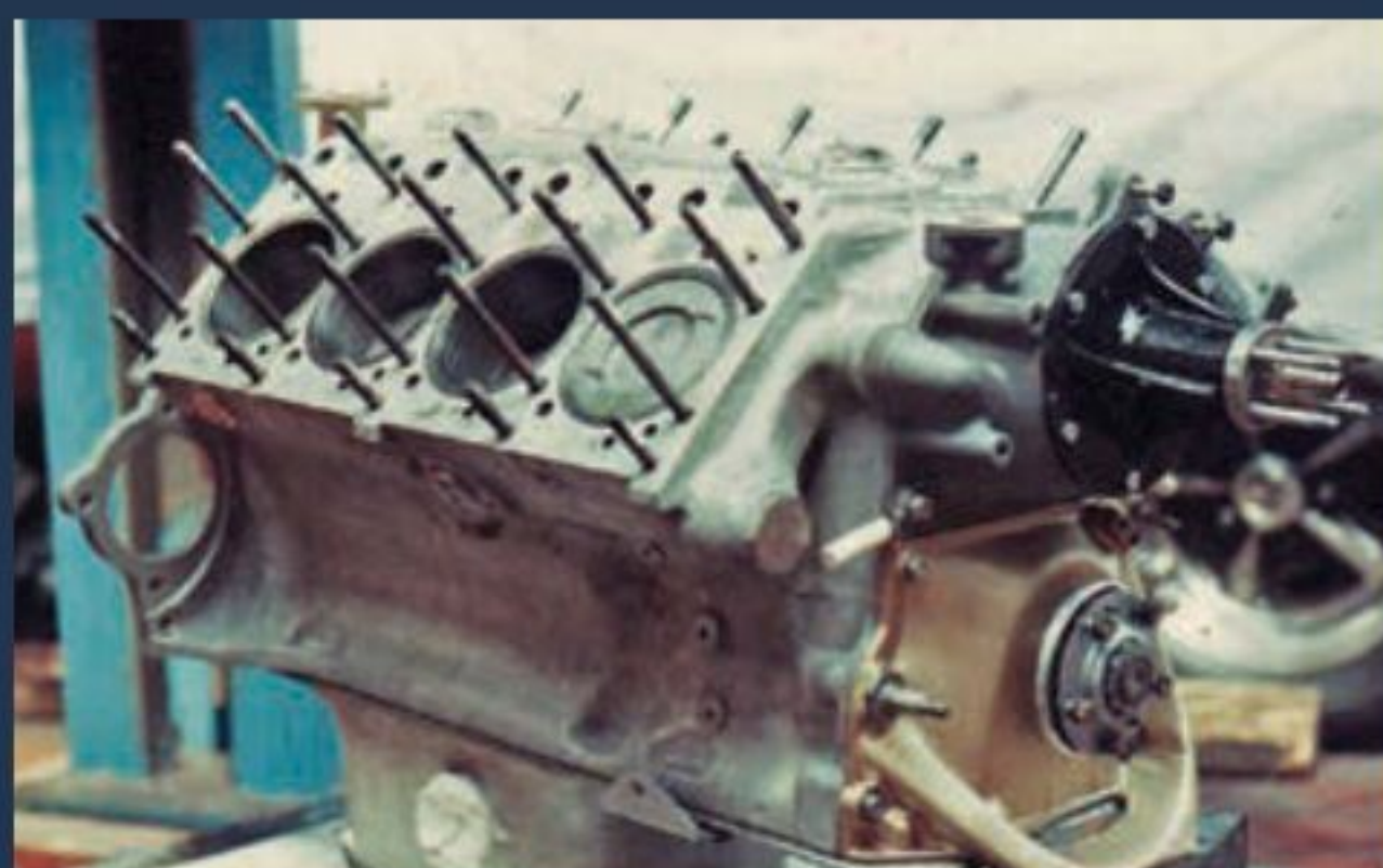
The engine was removed by Nigel and completely stripped to ascertain its true condition
