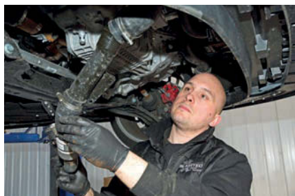
AS fitted a big boost pipe kit to the car
