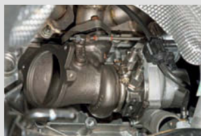
The key to the Stage 3 upgrade's huge power increase is the S242 hybrid turbo
