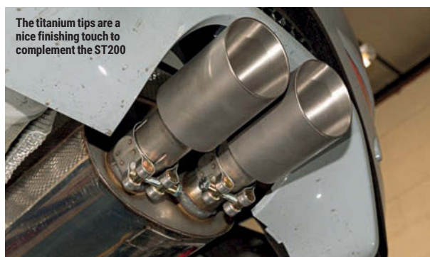
The 3in cat-back system allows exhaust gases to escape faster
