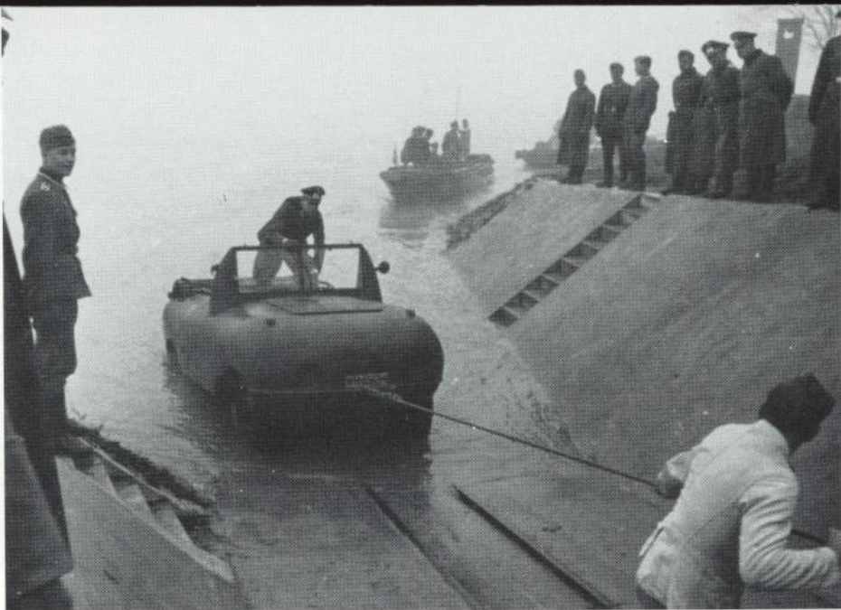
The Trippel comparison vehicle is pulled onto land with engine trouble resulting from overheating.
