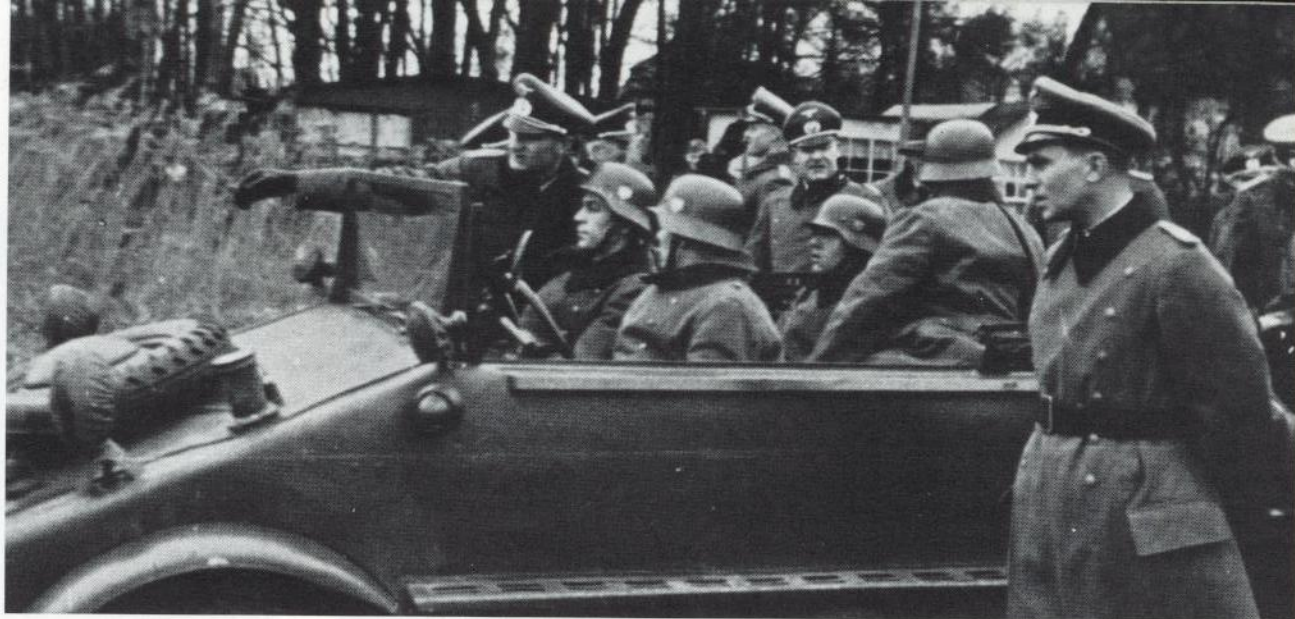
Schwimmwagen Type 128 being tested at the H.V.A. Test Center in Wünsdorf. The photo shows the first prototype with its Kübelwagen-like body.
