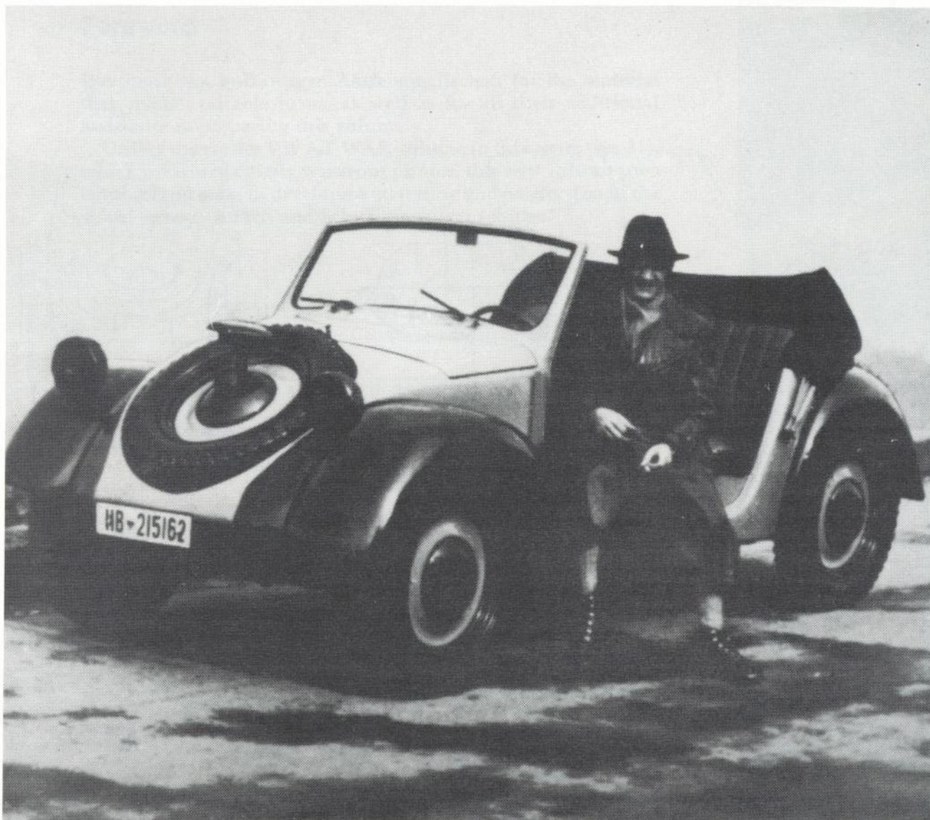
The first model of the VW Kübelwagen Type 62. The body still resembles that of the Beetle or its convertible version. This styling did not suit the military, as it looked too civilian.
