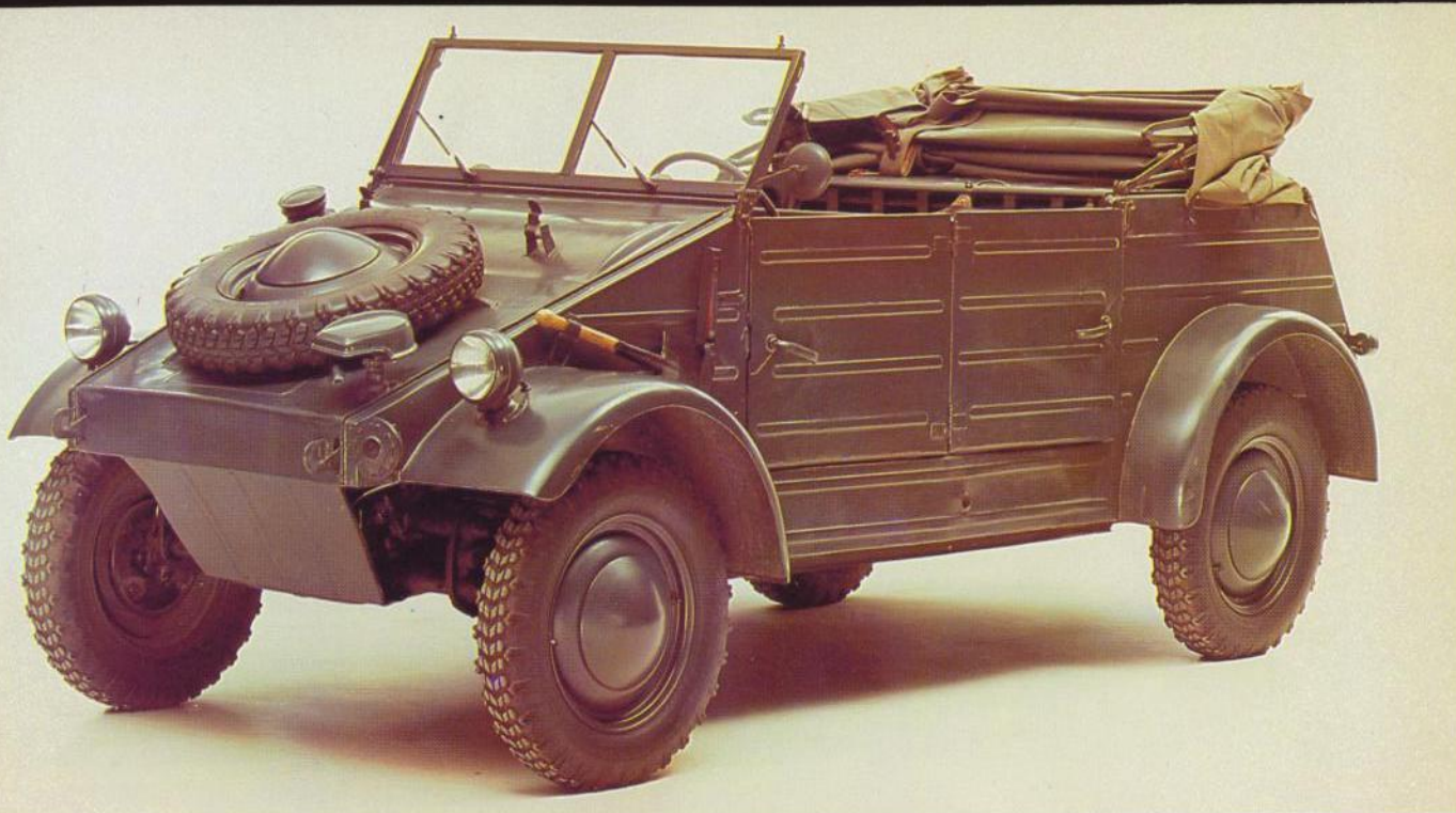
Volkswagen Kübelwagen Type 82, museum piece of the Volkswagen AG — Chassis number 2-047 471, built 1944 — because of material shortages, the fenders of this vehicle were welded on and the windshield divided.
