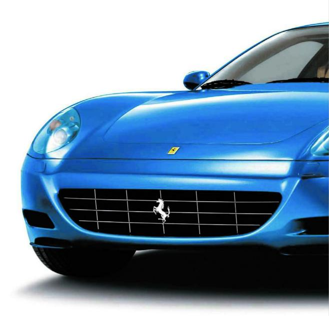
which represents Ferrari's first use of an all-aluminum vehicle with a V12 engine. The use of so much aluminum makes the car strong but light.
