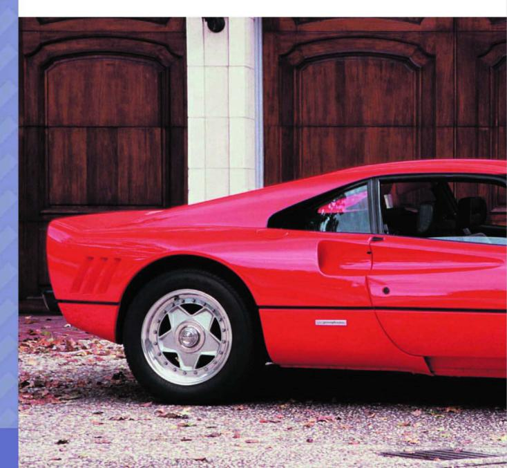
The 288 GTO was designed to meet international Group B racing regulations. Though the category didn't succeed, Ferrari went ahead with production of its new supercar, which featured such materials as Kevlar and Nomex composite, aluminum, fiberglass, and carbon fiber in its internal construction.
