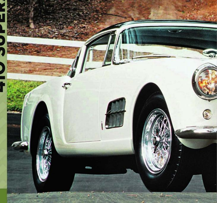
For the Paris show that fall, Ferrari unveiled a second version of the 410, the 410 Superfast. Built on a slightly shortened chassis, the Superfast featured dramatic styling, with Pinin Farina devising a unique greenhouse with no A pillars, a large backlight but huge wedgeshaped B pillars, and large and sharply creased tail fins flying over small rear bumper bars.
