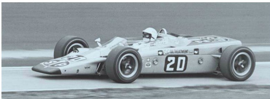
Art Pollard with the Pratt & Whitney turbine-powered Lotus 56 in the 1968 Indianapolis 500. He retired after 168 laps with a broken fuel pump drive.
