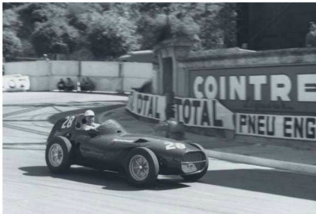
Moss in the 1958 Monaco Grand Prix. The nose of the Vanwall was shortened to reduce the possibility of accidental damage.
