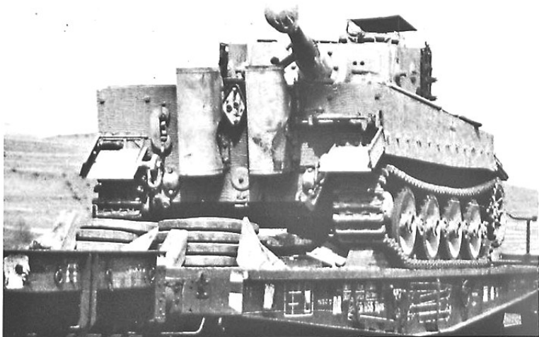
Starting with Fgst.Nr.250635, Tigers (such as this one completed in December 1943) had a rear travel lock. Fittings to mount a C-hook on the hull rear had been added starting in September and the track tool storage box had been dropped in late October 1943. The rectangular canvas ran guard has been erected over the commander's cupola. (BA)
