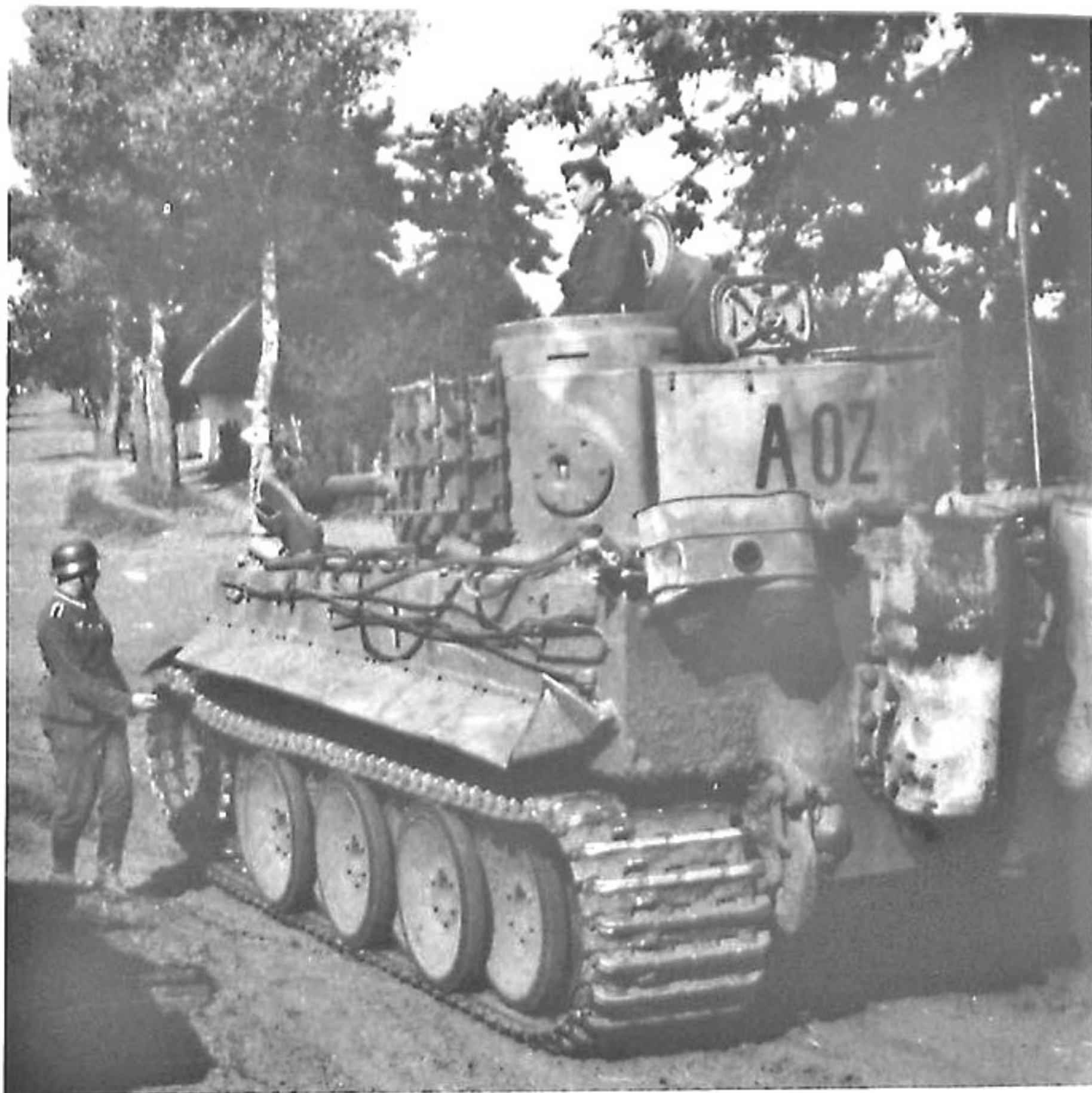
Starting with Fgst.Nr.250251, the larger Maybach HL 230 P45 engines were installed in Pz.Kpfw.Tiger Ausf.E, which is externally identifiable by two holes in the crank starter base plate. At the same time, the frames welded to the hull rear for mounting the rear fenders and tail lights were dropped. They were replaced by new hinged rear track guards (with cut-outs for the convoy light), supported by three hinge-plates welded directly to the hull rear (which have been torn off of this Tiger) (BA)
