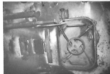
The inside of the turret roof from the adjustable interior light to the loader's hatch.
