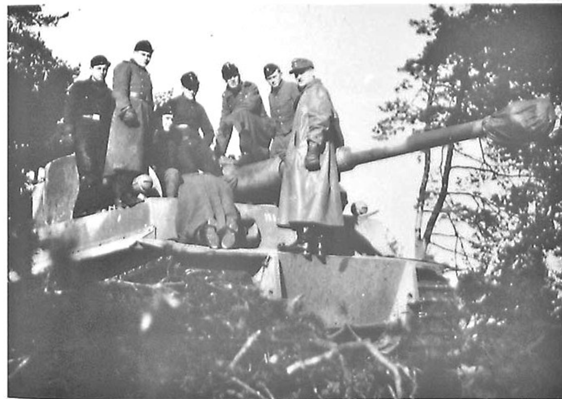
Pz.Kpfw.Tiger Ausf.E (Fgst.Nr.250159 completed in March 1943) with ring retainers for the track pins. The unit has sprayed camouflage paint onto the gun barrel which would burn and turn black after rapid firing. (MJ)
