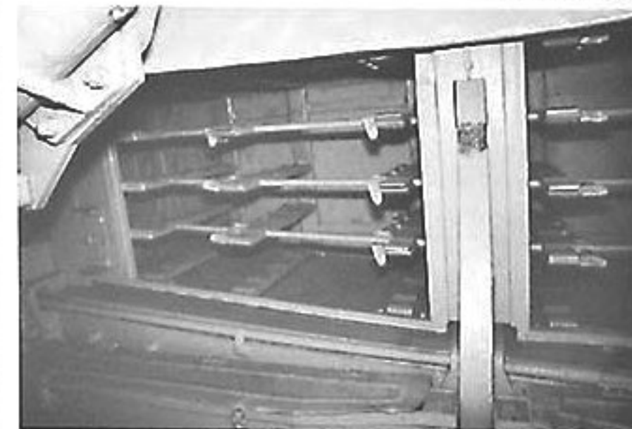
Ammunition racks on the right side, with each bin in the sponson holding 16 rounds and each lower bin holding 4 rounds.
