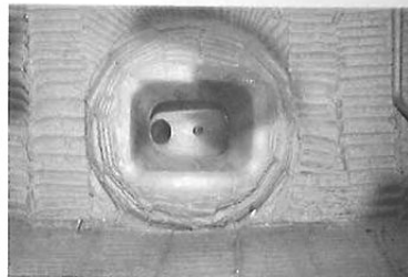
The tab on the glacis was for securing a plug (secured by a chain) for sealing the machinegun ball mount.
