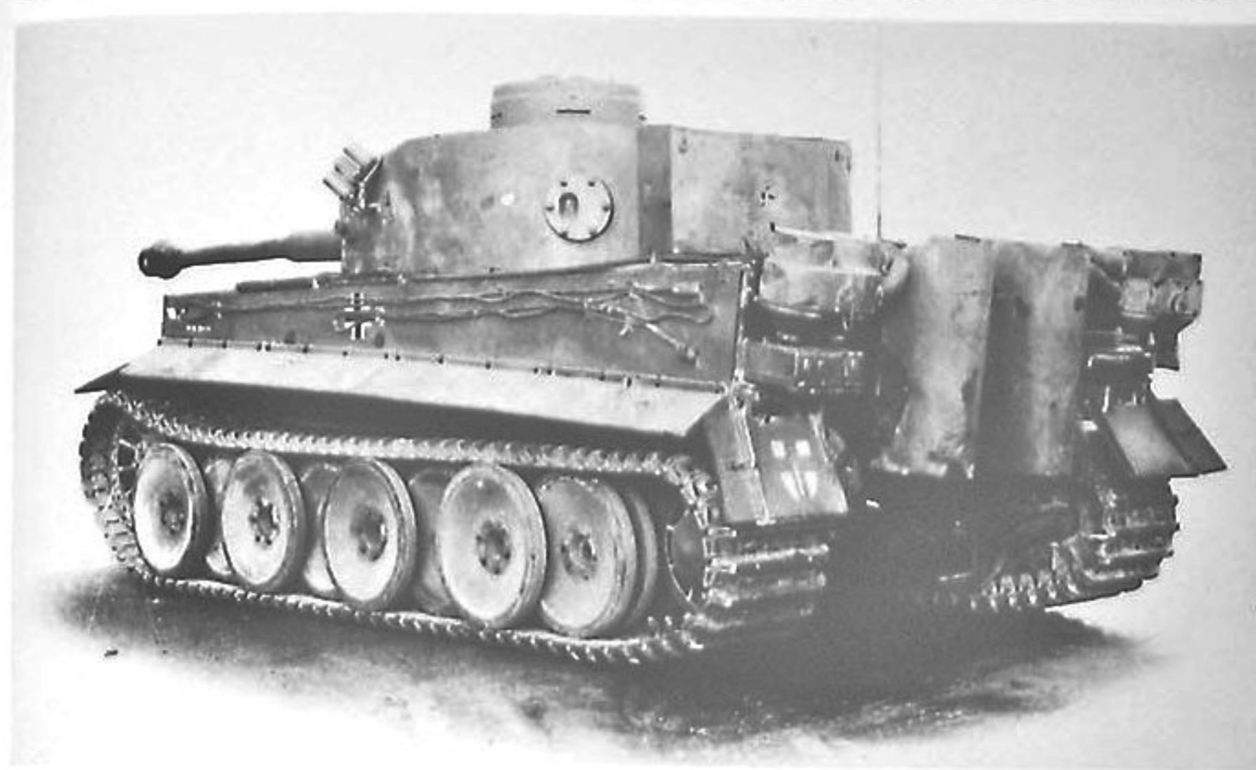
Pz.Kpfw.VI H Ausf.H1 (Fgst.Nr.250122 completed in February 1943) with Marschketten (725 mm wide operational tracks) and Verladeketten (520 mm wide transport tracks). In the right-side view, the outer roadwheels have been removed revealing the roadwheel rims reinforced by two bolts flanking each of the original six bolts. (TTM)
