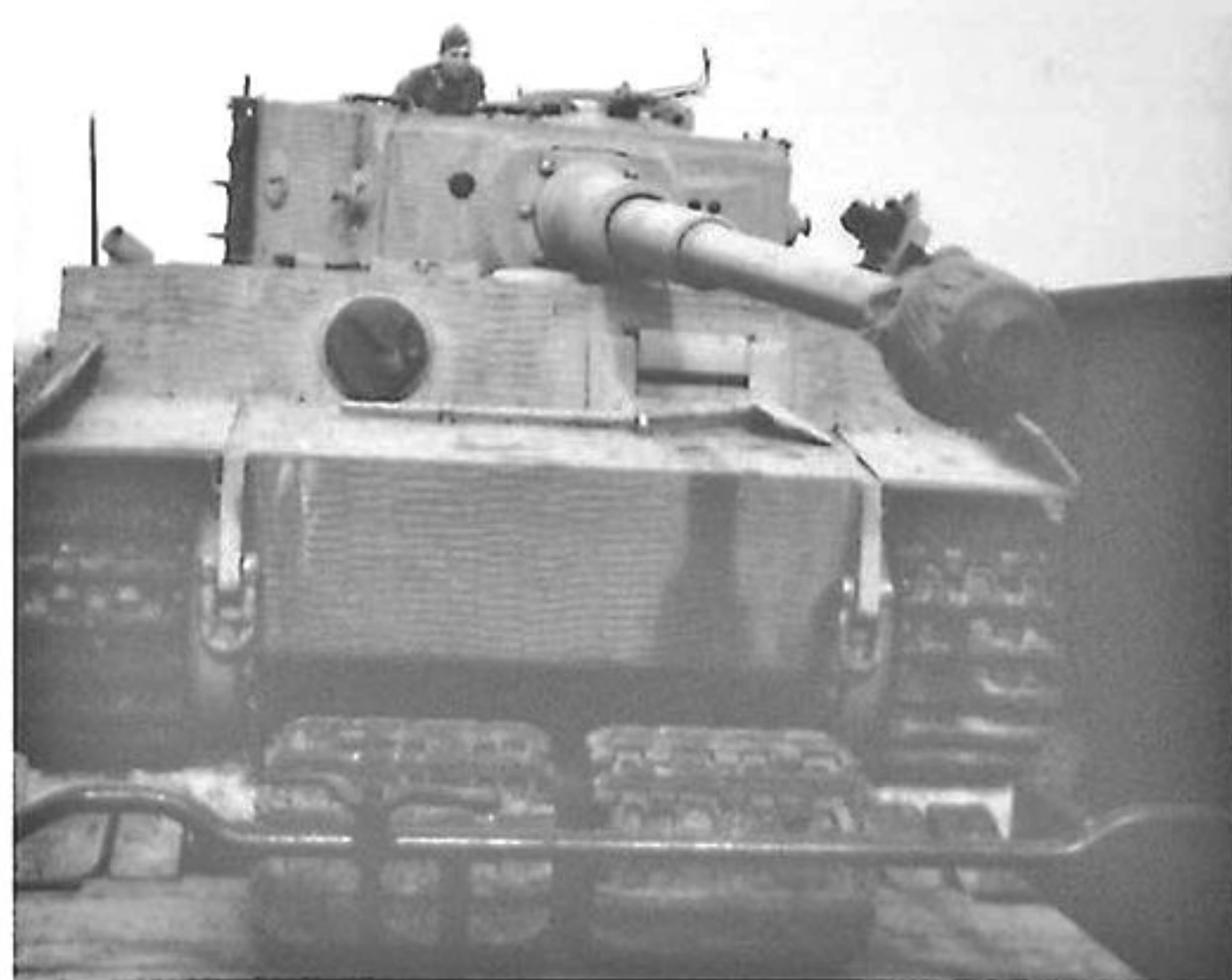
Several minor modifications are present on this Pz.Kplw.Tiger Ausf.E completed in September 1943, including reversal of the shovel mounts on the glacis, welding a tab to the glacis for securing a chain to the machinegun ball mount plug, deletion of the right headlight, and reversal of the direction in which the last two S-Mine dischargers were fired. (BA)
