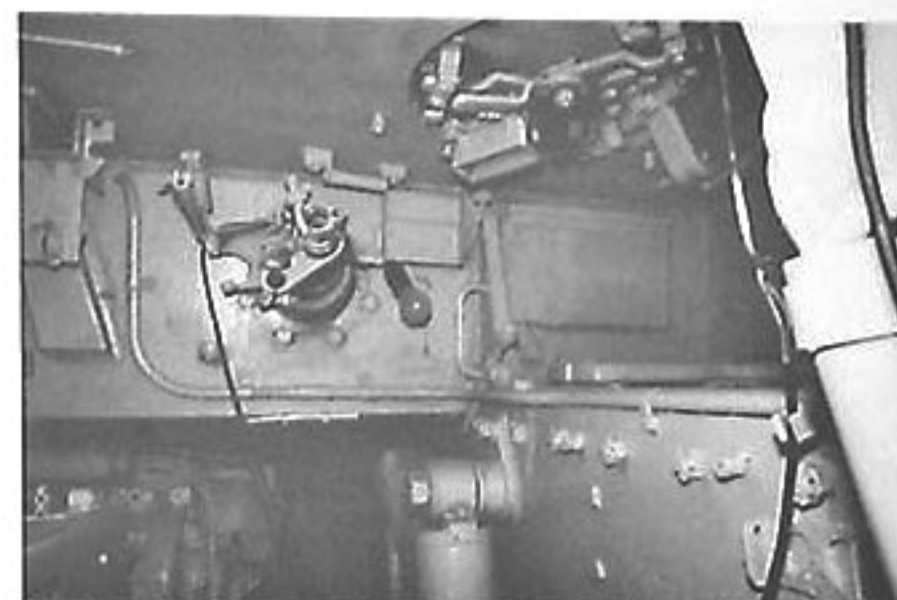
The radio operator's position with the ball mount for the hull machinegun. The radio racks mounted over the transmission housing are missing.
