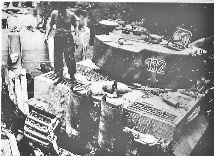
This Tiger I with the s-Pz.Abl.510, completed in late May/early June 1944, has three slits cut into the commander's cupola to drain off rainwater and still has the 3-bolt escape hatch hinge trimmed to clear the turret ring guard. (WS)
