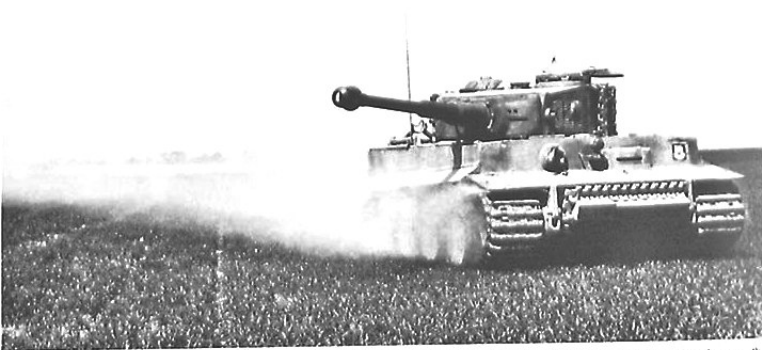
Completed in December 1943, this Tiger issued to s.SS-Pz.Abt.101 has a rear travel lock, still has fasteners for mounting a shovel across the glacis, and has the headlight mounted in the center of the driver's front plate (a modification which was initiated in October 1943). (BA)
