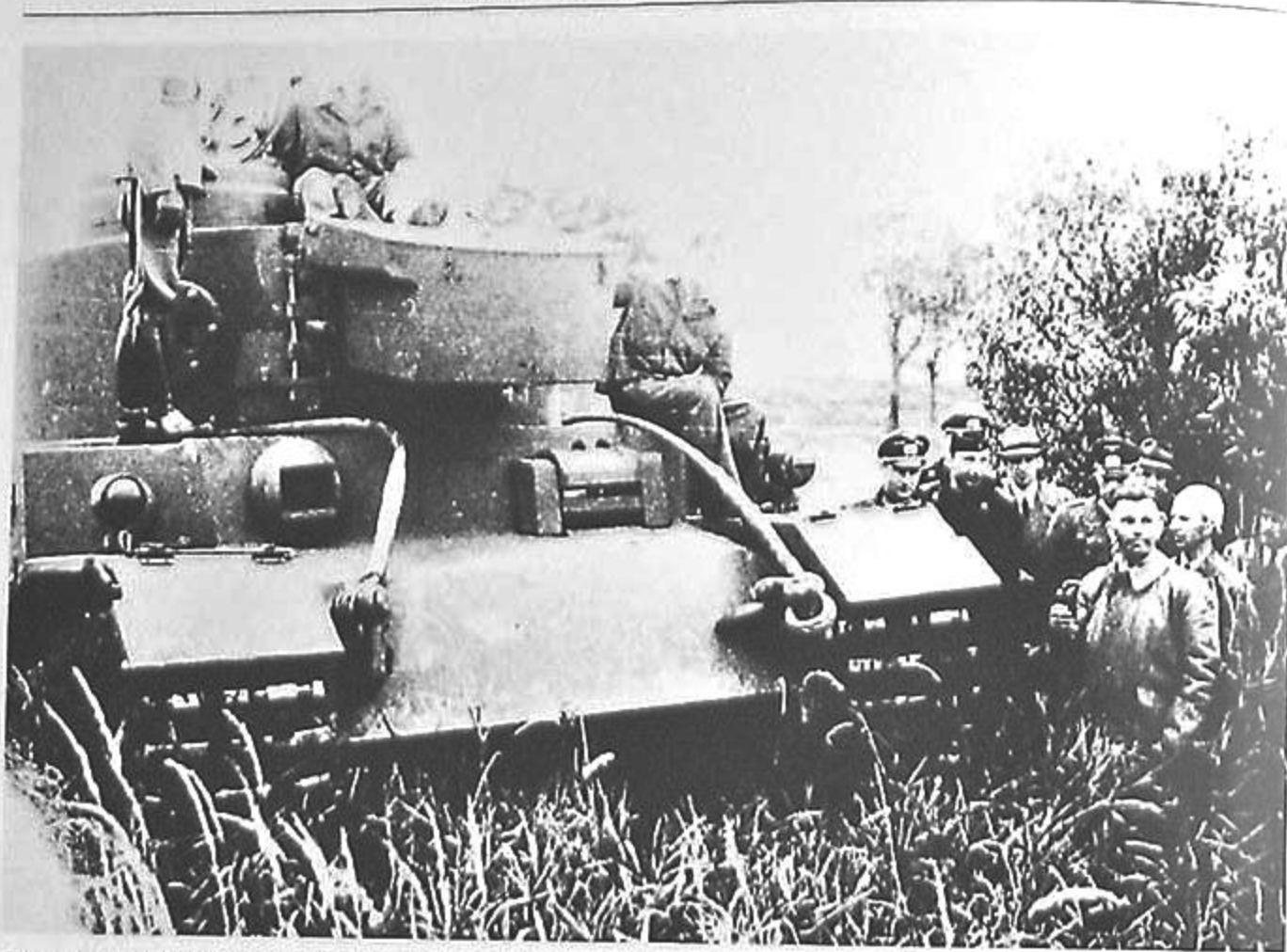
One of several VK 45.01 (P) with short sided turrets issued to schwere Panzer-Abteilung 503 for troop testing and training. This Tiger (P) was purposefully driven through a marshy area to test its flotation. (WJS)
