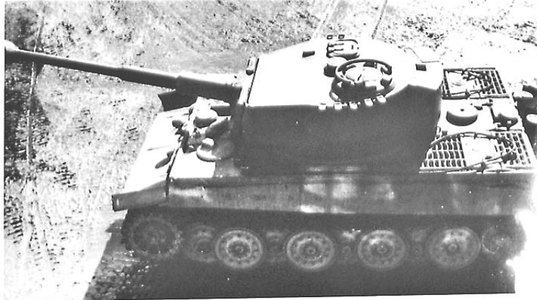
These photographs, taken at the Henschel assembly plant, are of a Pz.Kpfw.Tiger Ausf.E completed in late February/early March 1944. It has the smaller 600 mm diameter rotor, engine starter plate with mounting bolts, and tool stowage on the deck rearranged due to the turret ring guard. It still has a 25 mm thick turret roof with the deflector guard surrounding the loader's hatch (RFP).
