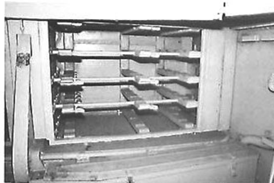
The Fgst.Nr.250031 dkr 42 was stamped into the side support (where the paint is missing) between the ammunition racks on the right hull side. "dkr" was the secret three-letter code for Henschel.
