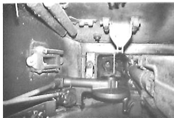
The left aperture in the gun mantlet has been plugged, while the rest of the mounting remained unchanged for the conversion to the monocular TZ.F9c telescopic gunsight.
