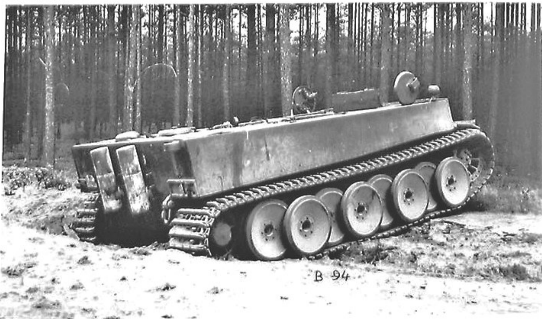
Wa Pruef 6 confiscated the first production series chassis (Fgst.Nr.250001 completed in May 1942) for testing. It is shown here after the steering mechanism broke. Periscopes had been installed in the hatch lids for the driver and radio operator but, as was the usual practice with Wa Pruef 6 test vehicles, it was not outfitted with any tool stowage. (BA)
