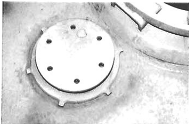
The armor cap protecting the ventilation fan with a base ring with six tabs for securing the sheet metal cap used for submerged loading.
