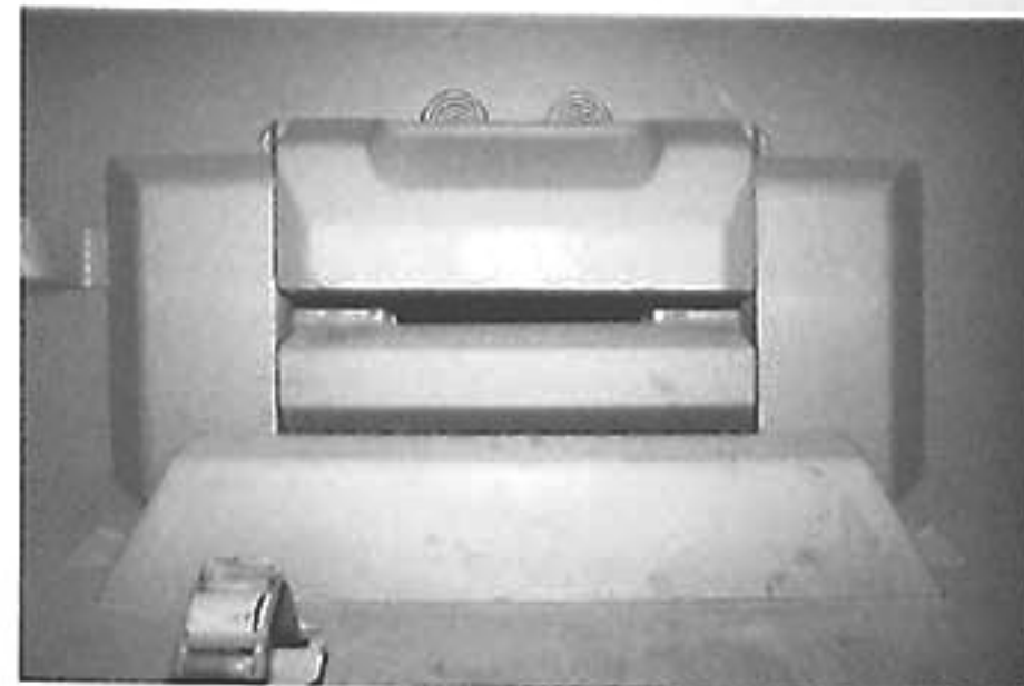
The driver's visor in the open position with apertures for the binocular K.F.F.2 driver's periscopes. The fastener on the glacis is for holding a shovel.
