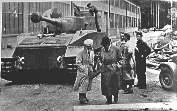
ABOVE AND OPPOSITE TOP: Dr. Ferdinand Porsche on a visit to Nibelungenwerk in August 1942 where his Typ 101 chassis were being assembled. This is one of the first eight VK 45.01 (P) which had the short-sided turrets designed and assembled by Krupp in Essen. (WJS)
