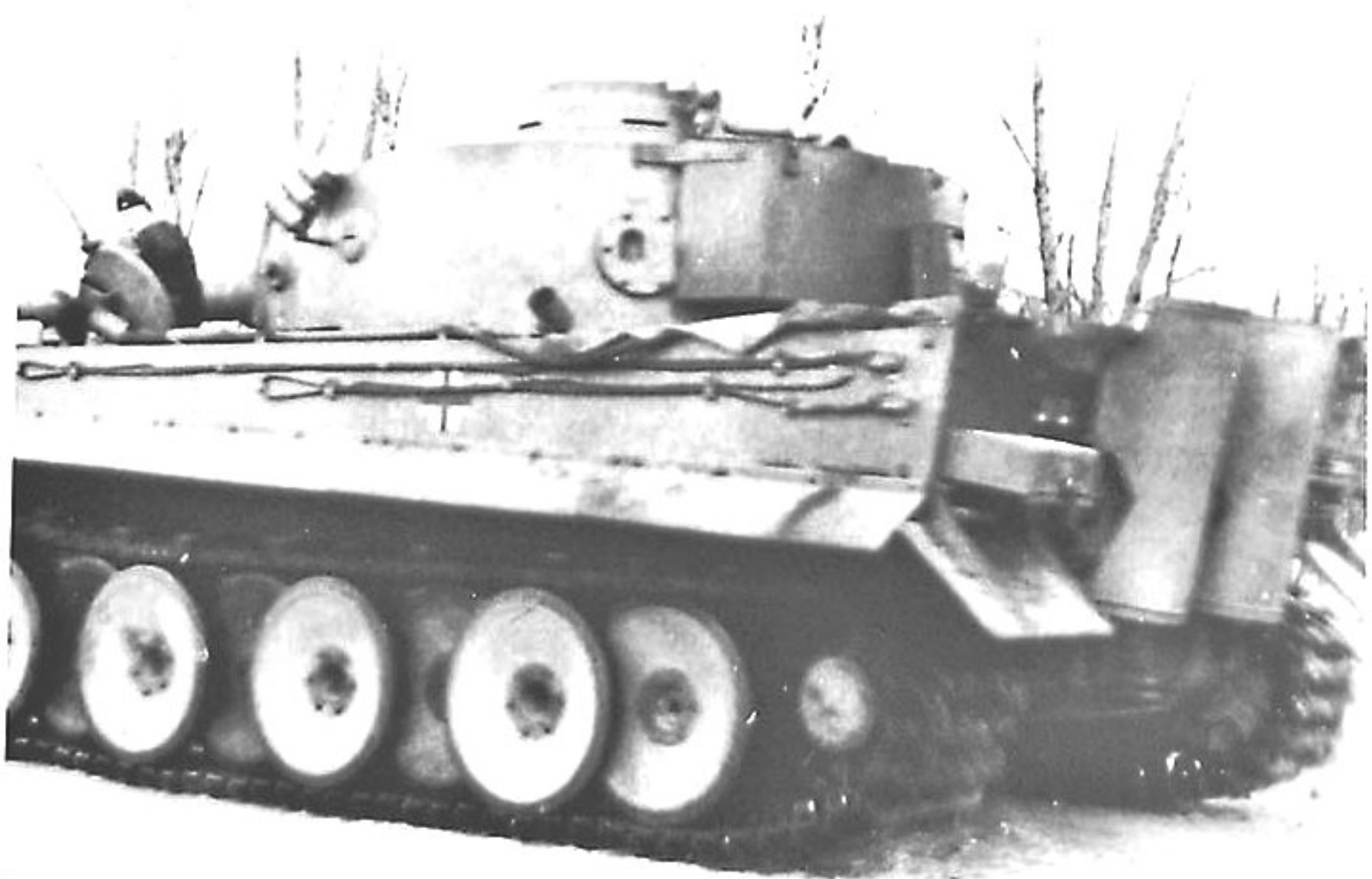
This Tiger, completed in January 1943 and issued to s.Kp./Pz.Rgt.GD, has five S-Mine dischargers, standard sheet metal guards for the mufflers, and an oversized stowage bin (in place of the factory supplied Pz.Kpfw.III stowage bin). (WS)
