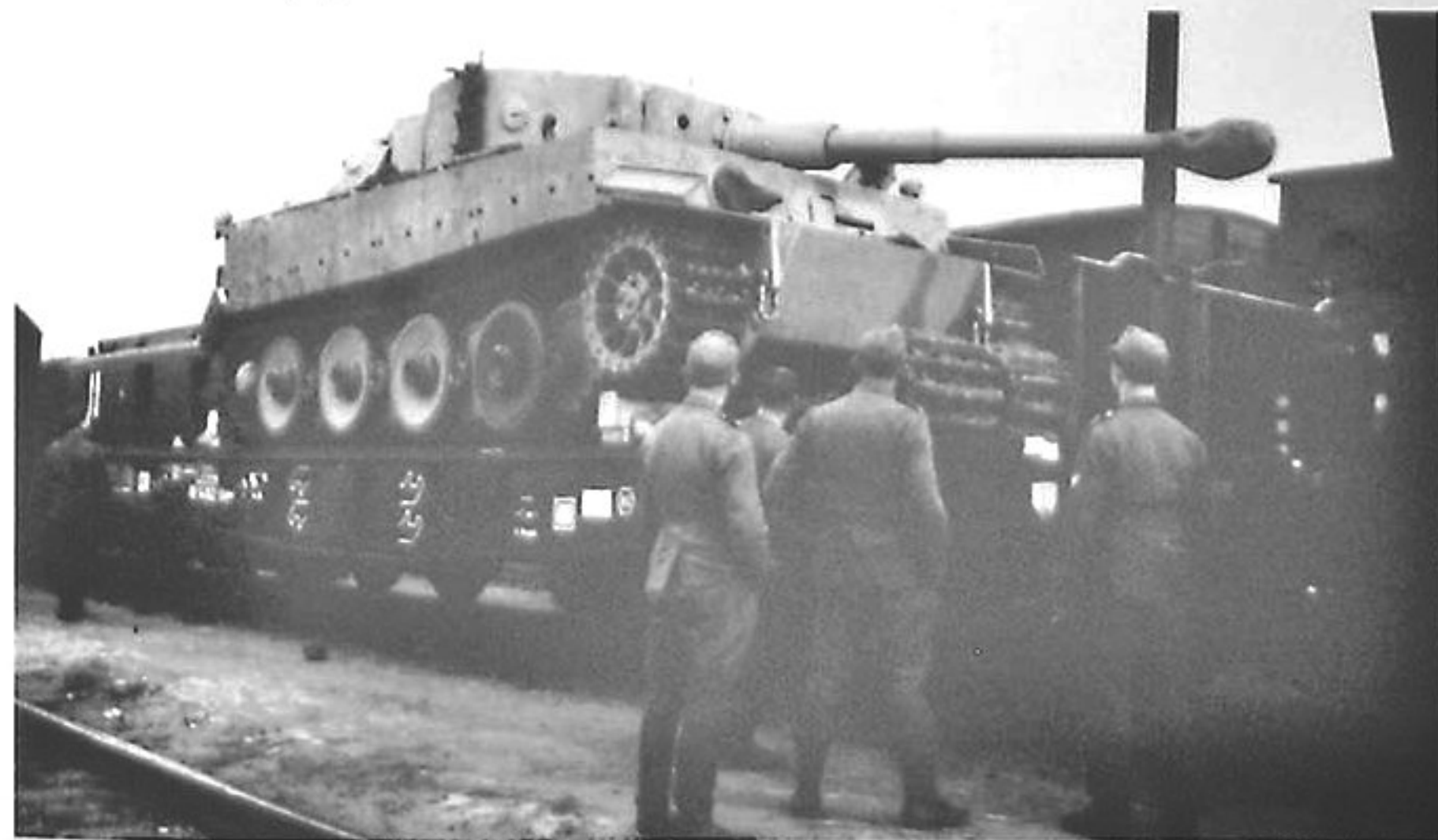
Several minor modifications are present on this Pz.Kplw.Tiger Ausf.E completed in September 1943, including reversal of the shovel mounts on the glacis, welding a tab to the glacis for securing a chain to the machinegun ball mount plug, deletion of the right headlight, and reversal of the direction in which the last two S-Mine dischargers were fired. (BA)
