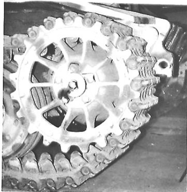
The machined drive sprocket wheel hub with sheet metal locking tabs to secure the bolts.
