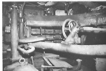
Ammunition racks in the left front pannier behind the gunner's seat (without cushion) and the elevation wheel with main gun trigger.
