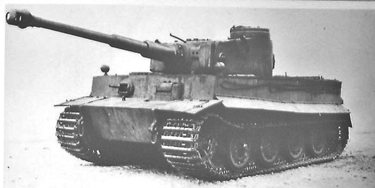
This production series Pz.Kpfw.VI (H) Ausf.H1 (Fgst.Nr.250053), completed in December 1942, was confiscated by Wa Pruef 6 for testing and subsequently modified by cutting the full side extensions for tow shackles and changing to the gummigefederten Stahllauffrollen (rubber-cushioned, steel-tired roadwheels). (WJS)
