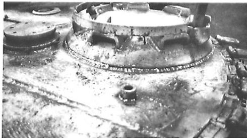
The turret roof was constructed using two 40-mm-thick plates and three slits were cut into the commander's cupola to drain off rainwater on this Tiger I (Wanne Nr. 251113 amp completed in May 1944) - now on display at Vimoutier, France. (HLD)
