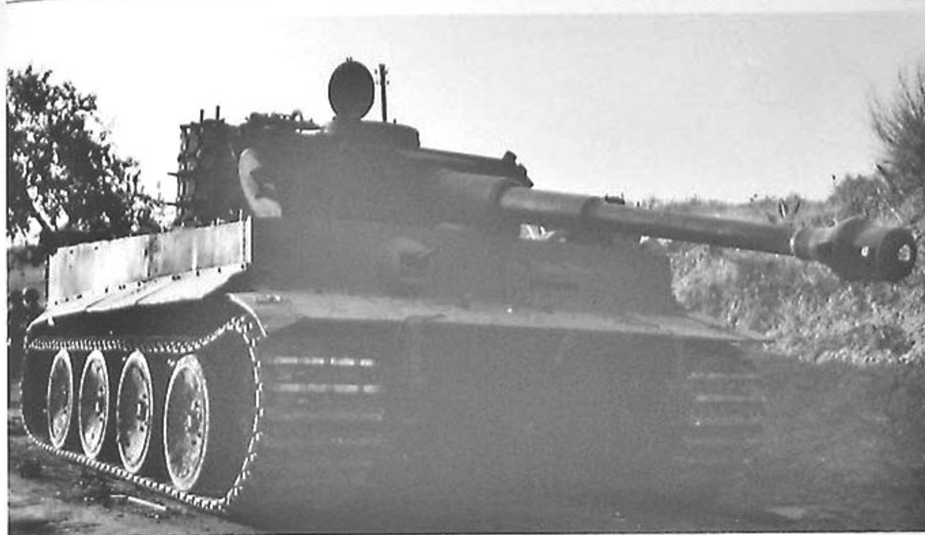
A Pz.Kpfw.Tiger Ausf.E (within Fgst.Nr. series 250200 to 250208 completed in April 1943 and issued to the 2.Kp./s.Pz.Abt.504 ) with three track holders on the right turret side and single upper chamber Feibel air cleaners. (NA)
