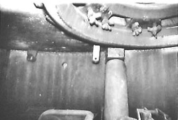
The seven periscopes in the commander's cupola were held in place by tabs, tightened with battery nuts. This is a Prismenspiegelkuppel (commander's cupola with periscopes) 921512/62 which did not have a 12-hour indicator ring.
