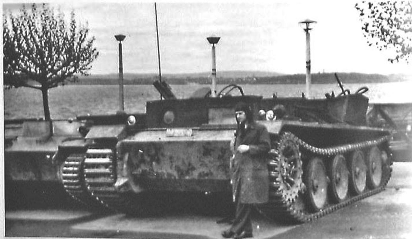
The only VK 36.01 chassis completed by Henschel was sent down to Maybach in Friedrichshafen (Lake Constance in the background) for trials (WJS)
