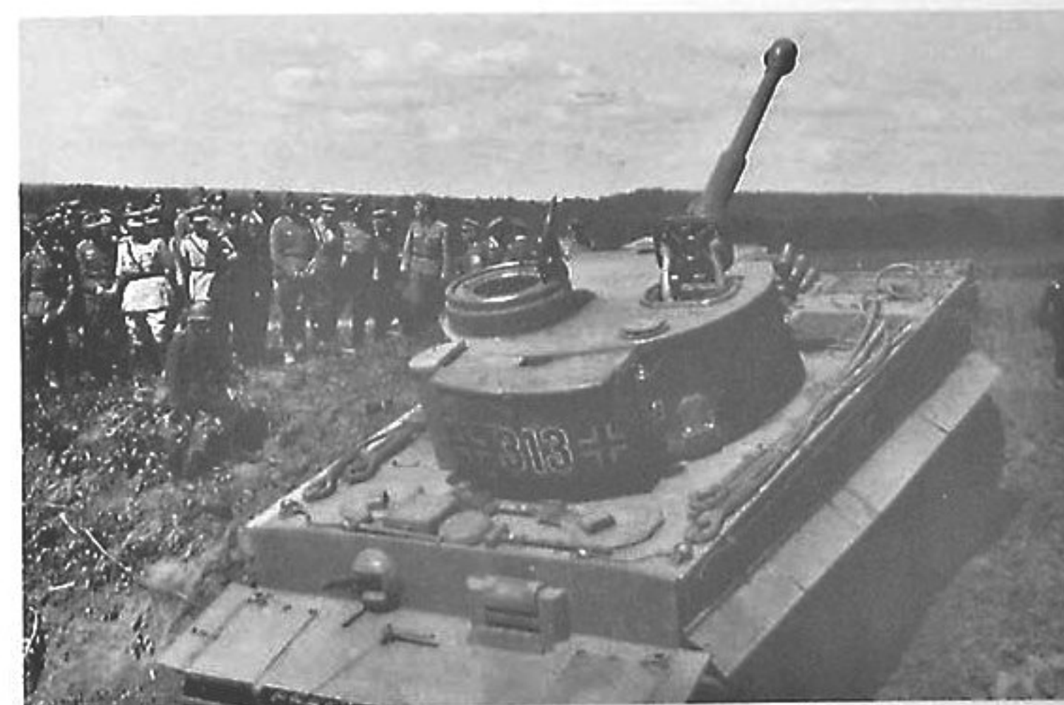
Completed in December 1942 and issued to the 2.Kp./s.Pz.Abt.502 (renamed 3.Kp./s.Pz.Abt.503), this is one of the first Pz.Kpfw.VI H Ausf.H1 with the emergency escape hatch in the turret in place of the machinegun port. The armor guards over the penetration in the hull roof for the headlight wiring had been redesigned. It still has normal stowage with five gun cleaning rods but has been modified by the unit (welding the driver's periscope holes shut, mounting a larger stowage box on turret rear, mounting a fire extinguisher beside the stowage box, and adding brackets to hold water cans on the rear). (BA)
