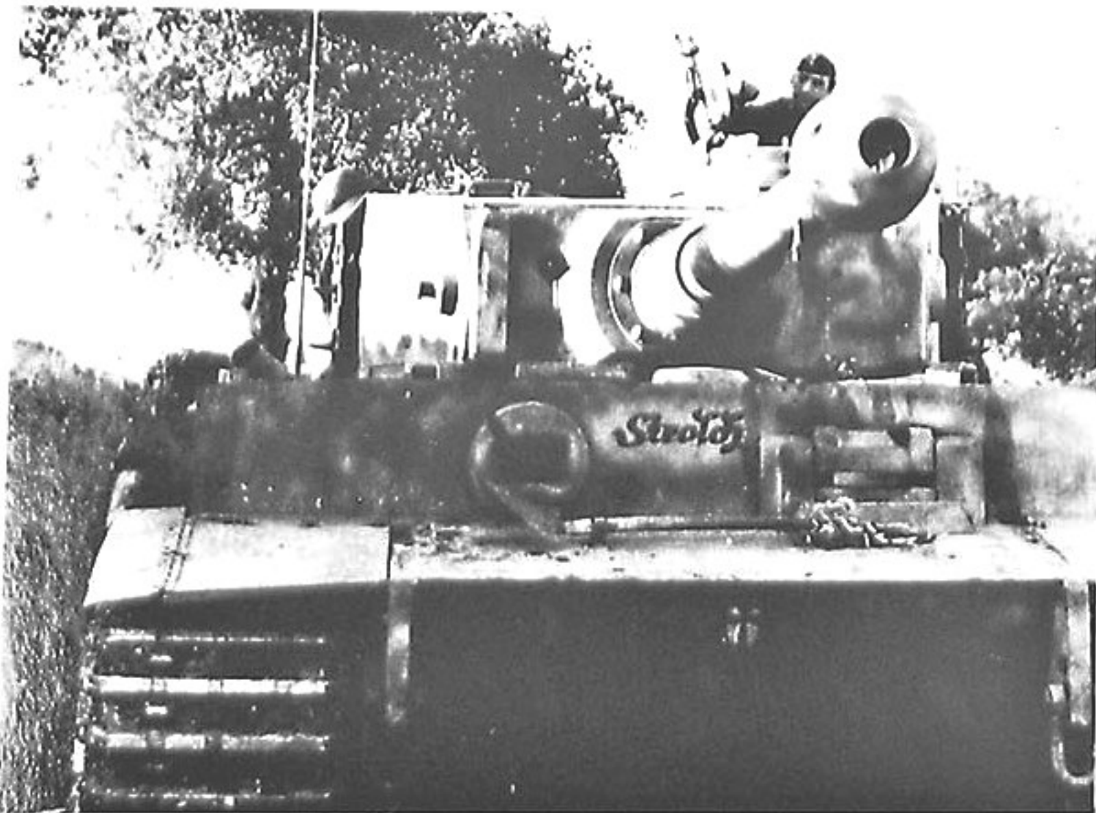
The smoke candle dischargers were dropped (starting with Turm Nr.286) and the toggle bolts to hold the sealing cap onto the machinegun ball mount were dropped in June 1943 as shown on this Pz.Kpfw.Tiger Ausf.E completed in July 1943. (BA)
