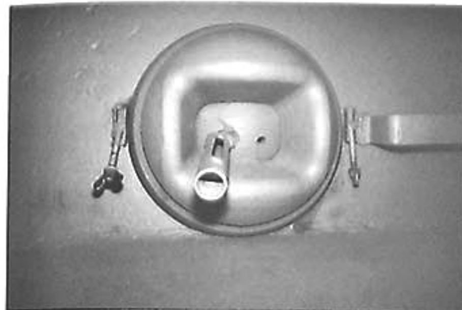
The machinegun ballmount flanked by pivoting toggle bolts for retaining a cover seal during submerged fording.
