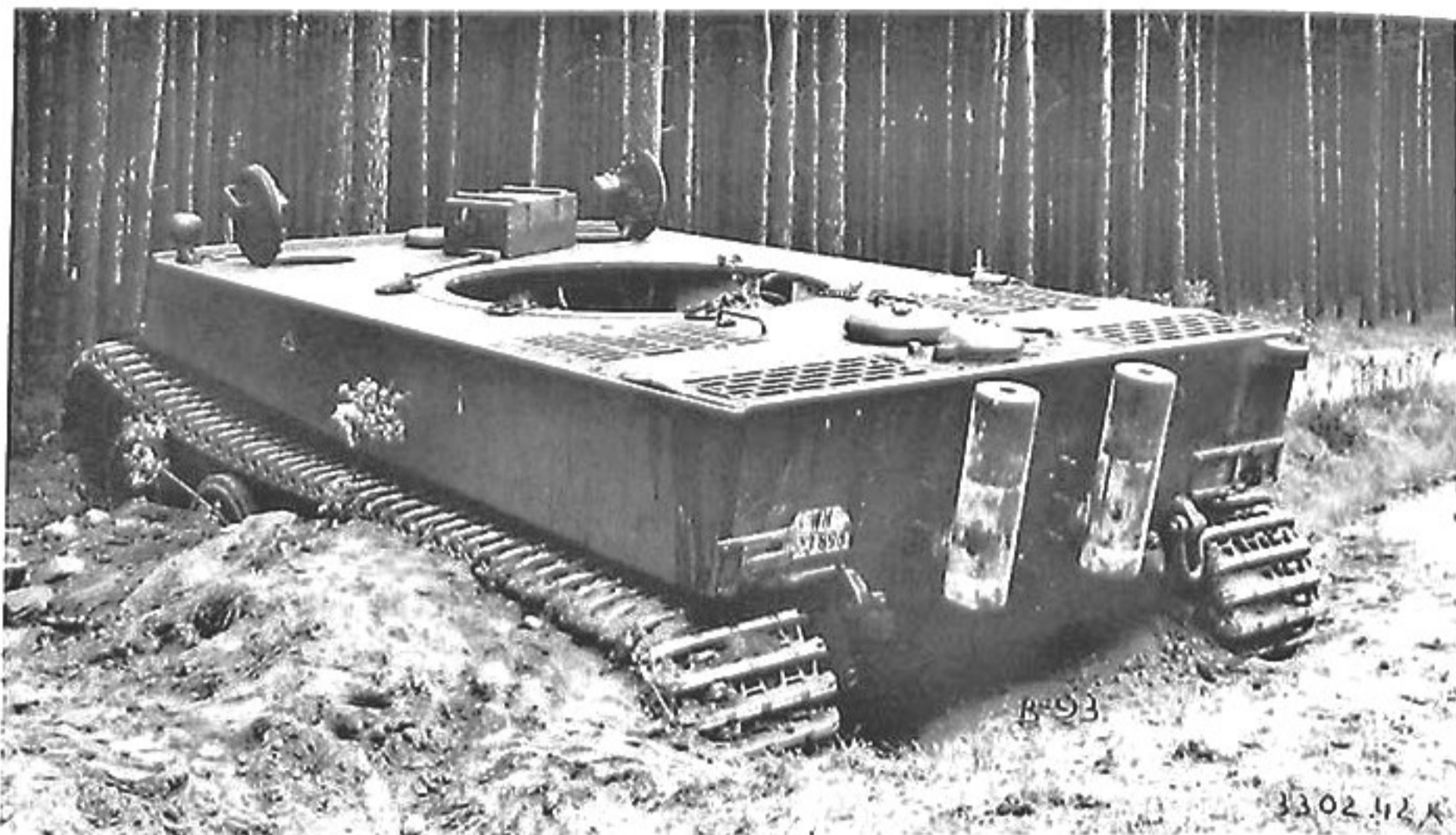
Wa Pruef 6 confiscated the first production series chassis (Fgst.Nr.250001 completed in May 1942) for testing. It is shown here after the steering mechanism broke. Periscopes had been installed in the hatch lids for the driver and radio operator but, as was the usual practice with Wa Pruef 6 test vehicles, it was not outfitted with any tool stowage. (BA)
