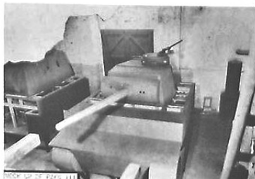
The wooden model of the Rheinmetall-Turm mit 7.5 cm Kw.K. L/70 (designated Pz.Kpfw.VI H Ausf.H2) with pistol ports on the turret sides, an emergency escape hatch on the right side, a communication port on the left side, and a machining-in ball mount on the rear. (APG)
