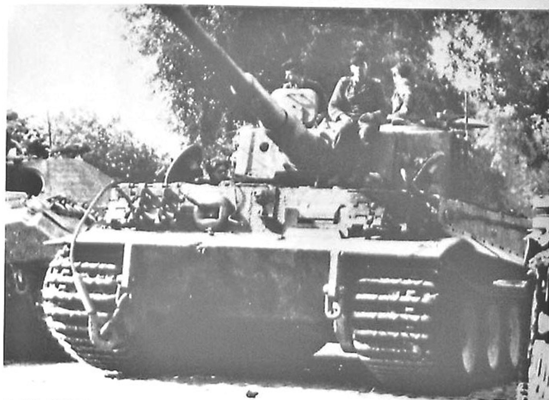
Tiger I (Fgst.Nr.250641 completed in November 1943) was one of the first with an external travel lock. The unit did not weld a bar across the front of the hull to carry spare track links. (WS)
