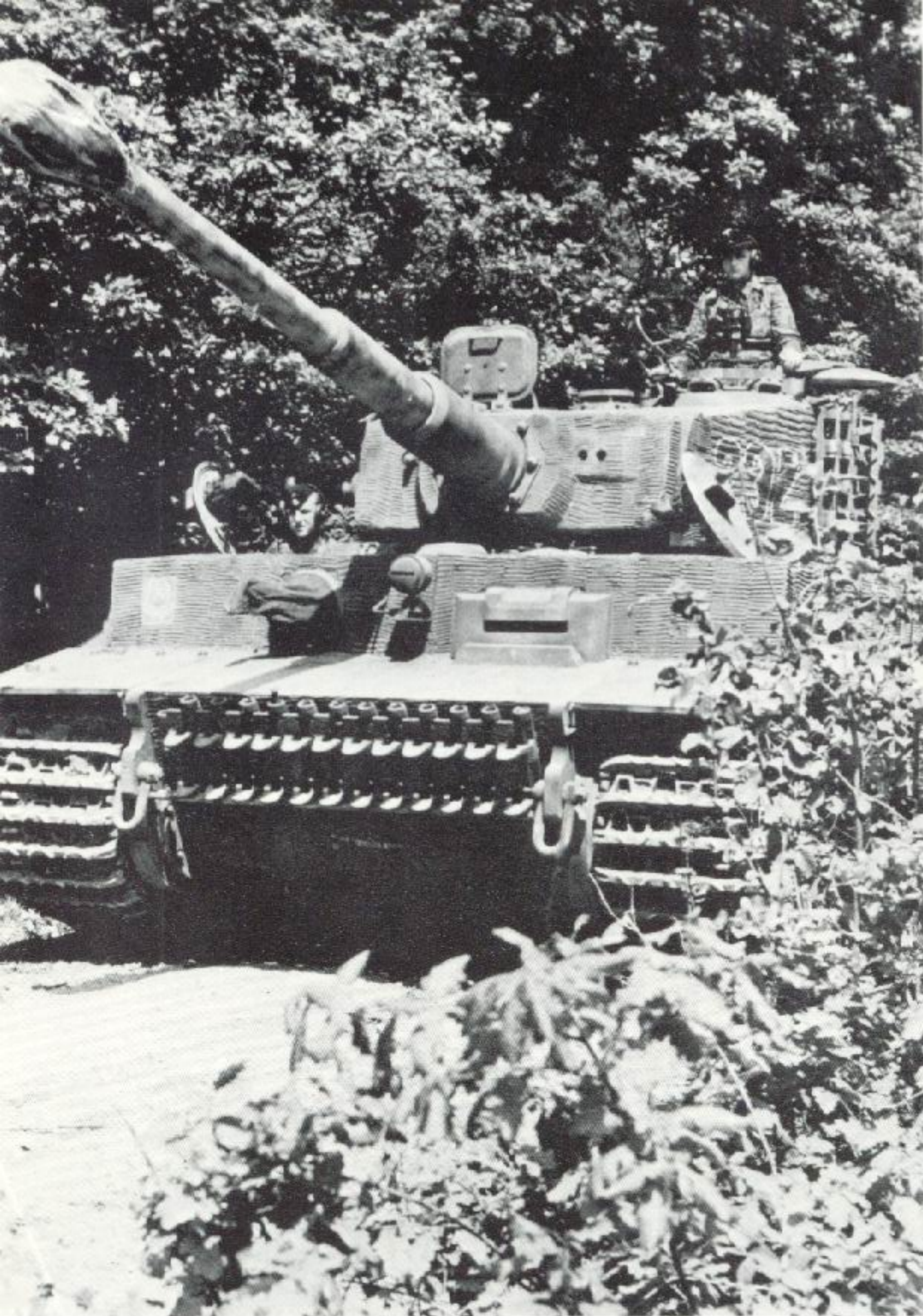
Left: A Tiger I with the symbol (two crossed keys) of the 1st SS Panzer Corps. It was carried on the right (as here) or left front plate. This tank, unlike the other, shows the rippled Zimmerite covering.
