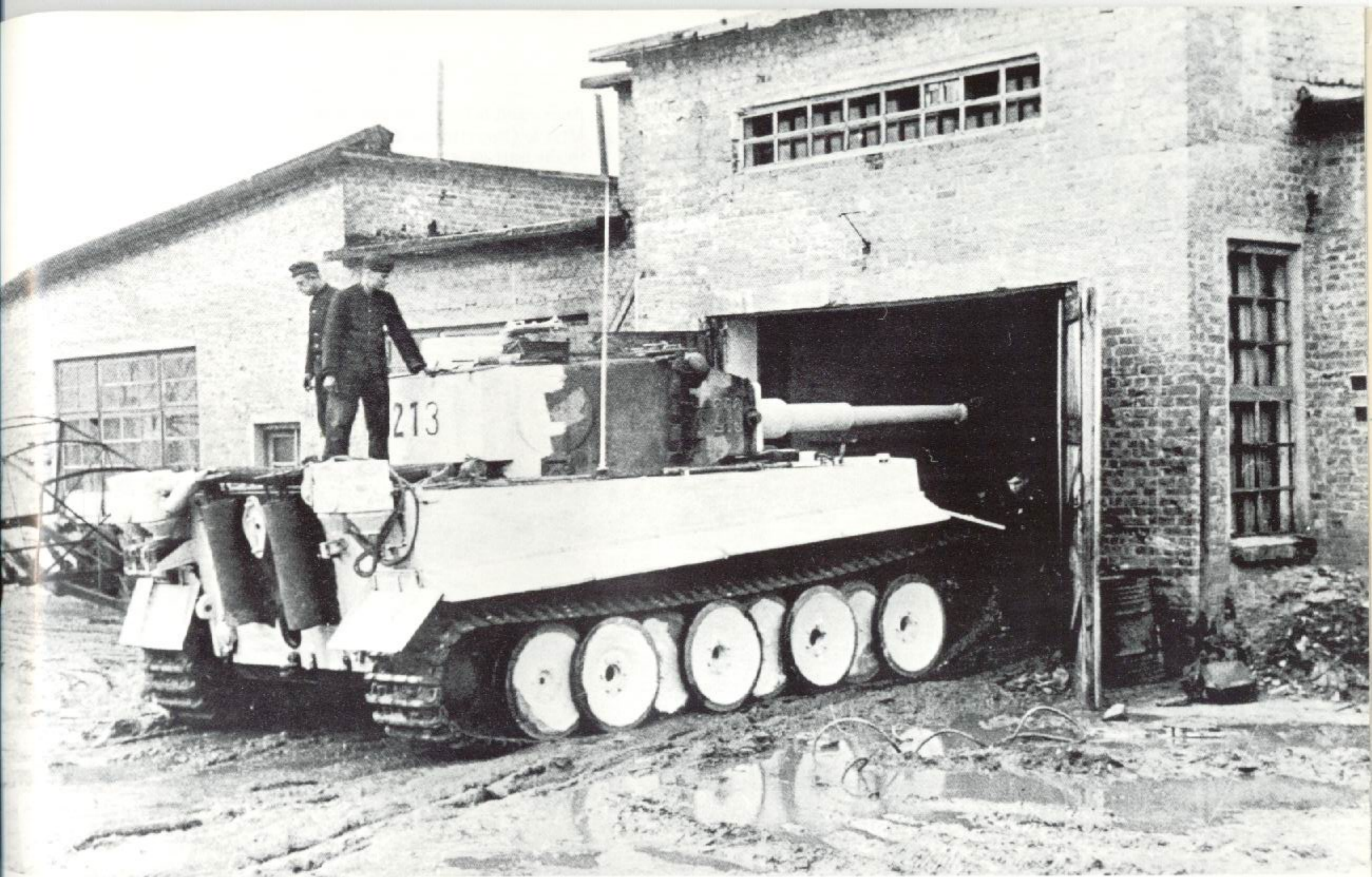
Here a Tiger has been given a good coat of winter paint — probably at a repair depot. The exhaust system and turret are not yet finished, though the former was generally not painted; it was not allowed on account of the heat. Note the Feifel ventilators on this Tiger, a sign that this Tiger was once intended for service in Africa.
