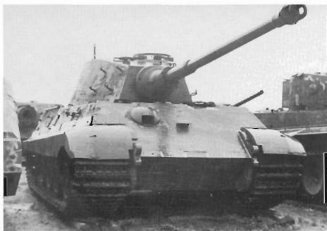
This King Tiger, with the production Henschel (Krupp) turret, is located in Kubinka (near Moscow). To its left is a Maus super-heavy tank. Photo: Queissner.
