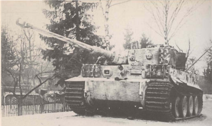
These two photos depict the same Tiger I Ausf. E. The vehicle was captured by the Soviet Army. Note the spare tracks mounted on the front of the tank. This Tiger has received a coat of Zimmerit anti-magnetic paste. Photo: Queissner
