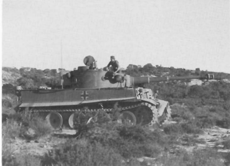
An early Tiger in Tunisia. The Feifel air filters are visible on the rear of the vehicle. Although the box-like Tiger I was poorly shaped, its extremely thick armor and powerful armament made it a formidable battle tank.
