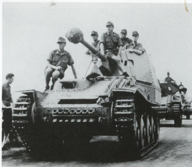
Always short of mobile-antitank vehicles, the Germans modified close to a thousand obsolete Czech-made light tanks into fairly effective Panzerjägers (tank hunters) by mounting in an open-topped superstructure, either captured Soviet 76mm antitank guns or German-made 75mm antitank guns. In its final production form as pictured, the vehicle was known as the Marder III. Far from perfect, these make-shift vehicles served a useful purpose until replaced by newer generations of Panzerjägers . Private collection
