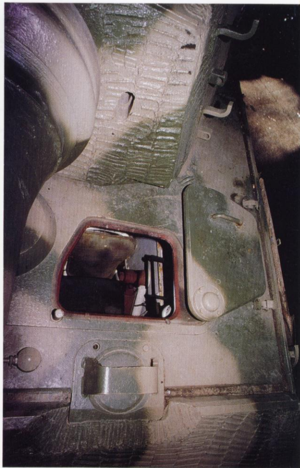
An overhead picture of the driver’s compartment of the Tiger II currently on display at the French Tank Museum. Both the vehicle’s driver and bow gunner had identical pivoting hatches which folded neatly on the upper hull when not closed down. In front of the open hatch can be seen the top of the driver’s rotating periscope. Directly above the driver’s open hatch can be seen the small opening for the gunner’s TZF9d monocular sighting telescope. Tank Magazine
