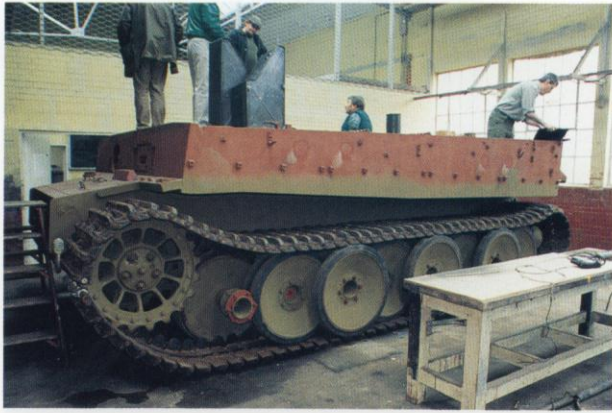
This interesting picture of the Tiger I located at the British Army Tank Museum, shows to good advantage both the box-like hull of the vehicle and its interleaved road wheel arrangement. The picture was taken in 1993 and shows the vehicle in a maintenance bay of the museum. In order to restore this vehicle to operational condition after so many years required that the tank be stripped down to its basic components and basically rebuilt from the ground-up. Notice the Tiger's turret has already been removed as well as all the exterior fixtures. Jacques Littlefield
