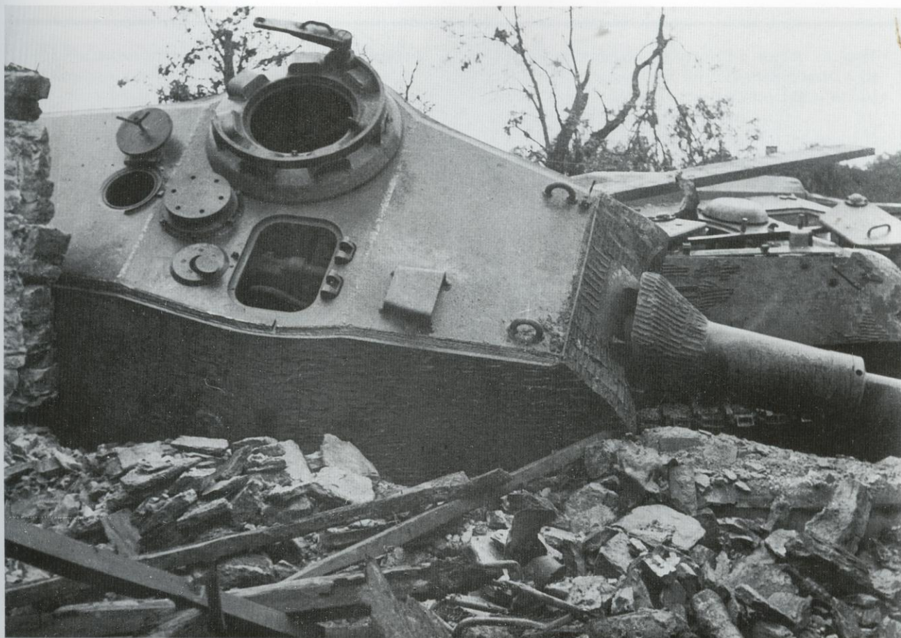
A disabled Tiger II, fitted with a Porsche turret, shows many of the upper turret details. At the top of the picture is the Panther tank type commander's cupola, which is missing its hatch. Underneath the commander's cupola is the loader's hatch opening, which is also missing its hatch. Right behind the loader's hatch opening is the smaller opening for a
