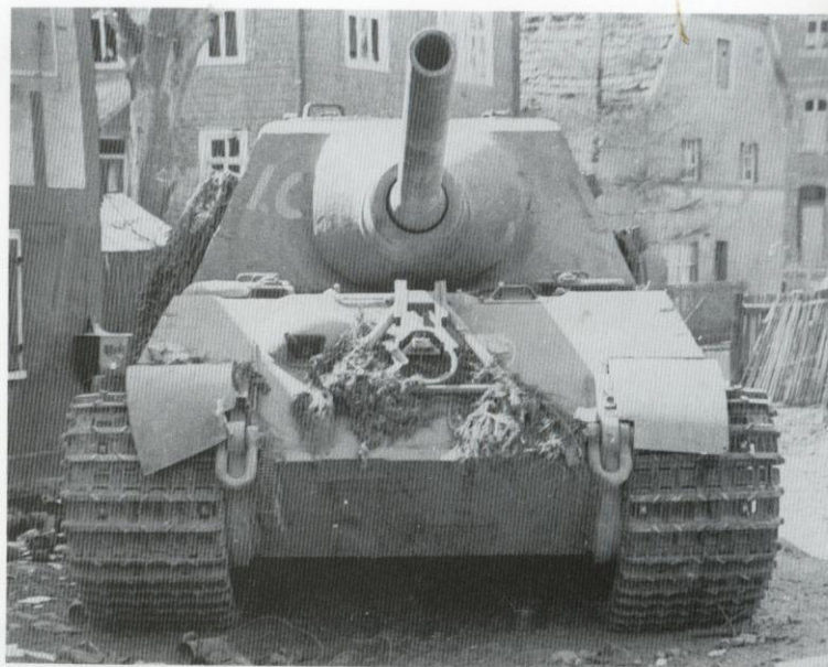
This frontal view of an abandoned Jagdtiger , armed with a 128mm gun, is from a US Army technical intelligence dated 10 May 1945. This vehicle was knocked out by a German Army Panzerfaust (rocket launcher). The report doesn't state who fired the Panzerfaust . However, the Panzerfaust was often used by Allied troops when they captured them, since it packed a much bigger punch than the American-made bazooka. The frontal armor on the vehicle's superstructure was almost 10in thick. The object lying flat on the vehicle's front hull plate is a travel lock, which helps to steady the large gun when not in combat.
