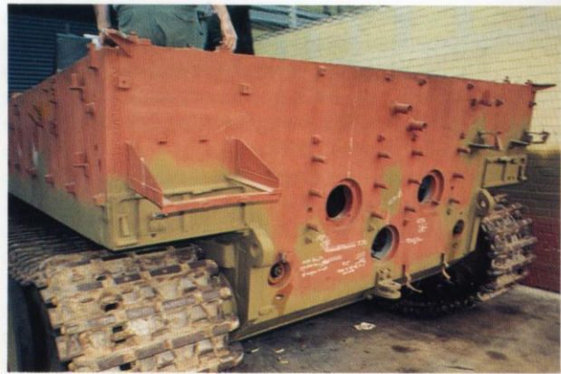
Taken in 1993, this rear three-quarter shot shows the stripped-down hull of the British Army Tank Museum's well-known Tiger I which is being restored to operational condition. Visible in this picture are three rear engine access holes. The two holes at the mid-line level of the rear engine armor plate are for the muffler exhaust pipes. The two smaller holes on either side of the rear engine armor plate are for making adjustments to the vehicle tracks. The larger hole in the lower middle section of the rear armor plate is for the hand operated inertia starter. Jacques Littlefield
