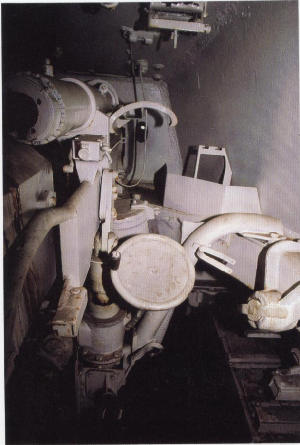
This picture was taken inside the Tiger II located at the French Army Tank Museum and shows the view of the vehicle's loader looking towards the front of the turret. In the center of the picture is the auxiliary turret traverse hand wheel for the loader. The coaxial 7.92mm machine gun is not mounted in this vehicle, although the small opening in the front of the turret through which the muzzle of the gun is fired is visible. Tank Magazine
