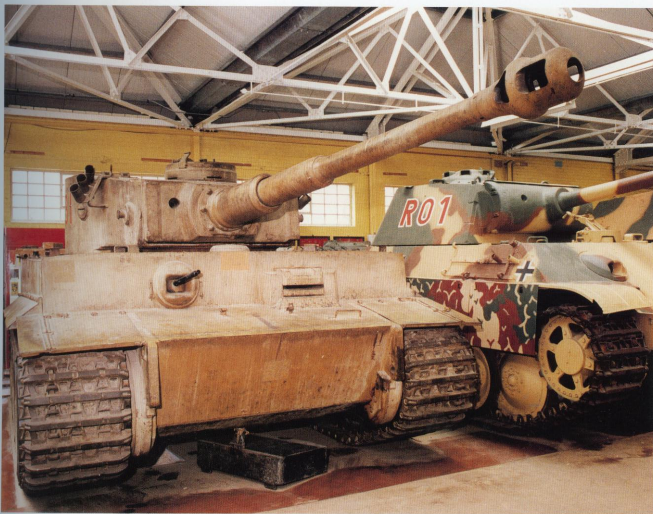
On display at the British Army Tank Museum is this early model Tiger I captured in North Africa. The thick box-like steel armor construction of the hull is clearly evident when compared to the well-sloped frontal hull armor of the Panther tank parked next to it. The front hull and turret armor of the
