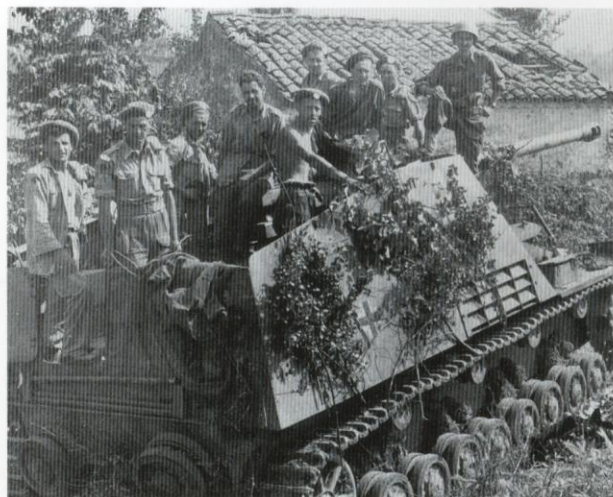
Before tanks like the Tiger I could be built in large numbers, the Germans needed to field vehicles carrying enough firepower to destroy heavily-armored Soviet medium and heavy tanks. In an attempt to deploy the 88mm gun on a fully-tracked chassis as fast as possible, the Germans developed a self-propelled tank destroyer known as the Hornisse . Based on components of both the Mark III and Mark IV medium tanks, the Hornisse housed the very potent 88mm gun in a fixed mount, lightly armored, open-topped superstructure. Carrying forty rounds of main gun ammunition, the Hornisse had a four man crew. Later renamed the Nashorn , the Germans built over 473 during the war. The Hornisse/Nashorn pictured was captured by Allied troops. British Tank Museum
