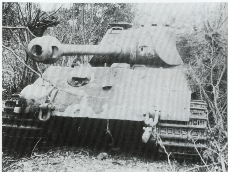
The thick well-sloped frontal armor of the Tiger II was virtually impenetrable to most Allied antitank rounds except at very close ranges. Even the sides of the Tiger II turret and hull could stop most Allied guns under 85mm. This Tiger II took a high-velocity hit on the mantle that covers the hull-mounted machine gun. The hit failed to penetrate, but did gouge out a piece of the armor surrounding the machine gun firing port. Notice that this Porsche turret has one of its sighting ports plugged, as it was fitted with the same single-lens sight found on the Henschel turrets. British Army Tank Museum
