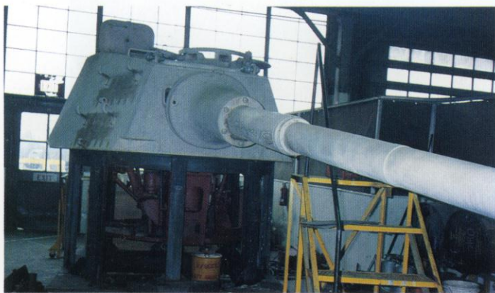
The turret of Tiger 332 was removed at the Patton Museum to allow easier access to the vehicle's hull during the rebuilding process. The Henschel turret—as fitted to Tiger 332—was a little over 7in thick on its front plate. The turret sides were about 3in thick, with the roof of the turret being a little less than 2in thick. Unlike the fifty Porsche turrets which mounted a monobloc (one-piece) barrel, Henschel turreted tanks had a two-piece barrel which was easier to build. Patton Museum
