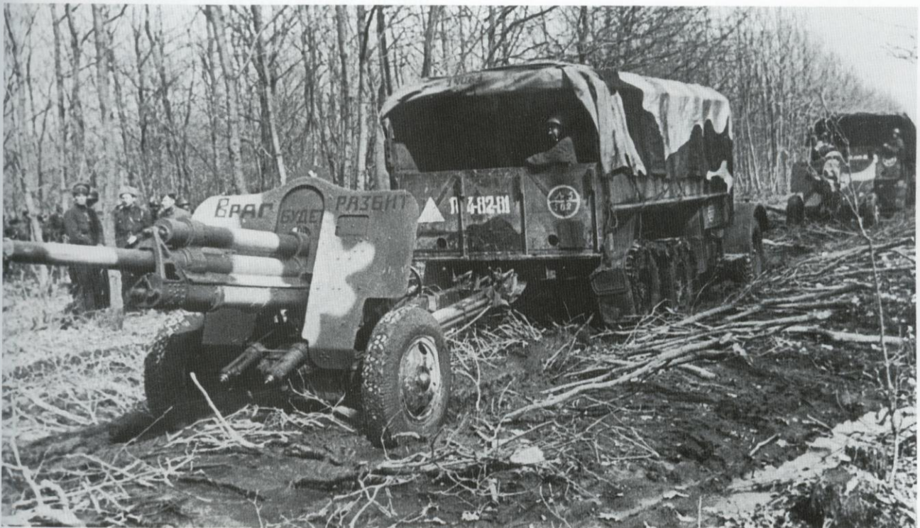
One of the mainstays of the Soviet Army's towed antitank-gun fleet during World War II was the 76.2mm field gun. Seen here being towed into combat by a truck fitted with rubber tracks around its rear wheels, the 76.2mm field gun was an
