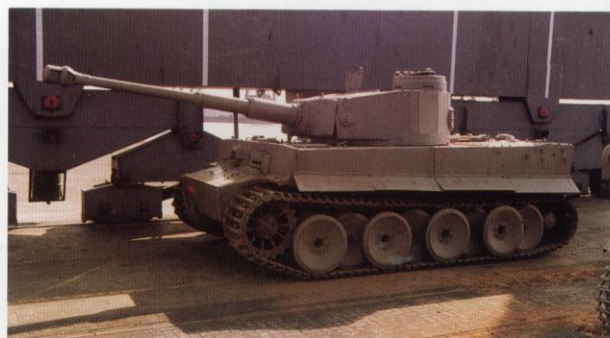
Armor protection on the hull sides of the Tiger I was about 2in thick. The rear engine hull plate and the bottom of the hull was roughly an inch thick. The horseshoe shaped turret of the Tiger I was 4in thick on the front and 3in thick on the sides and rear. The vehicle pictured is the Tiger I that used to be on display at the US Army Ordnance Museum and is now on a ten year loan to the German military museum system. The vehicle is seen here on its arrival in Germany on a dock were it was unloaded from the ship that delivered it. Thomas Anderson
