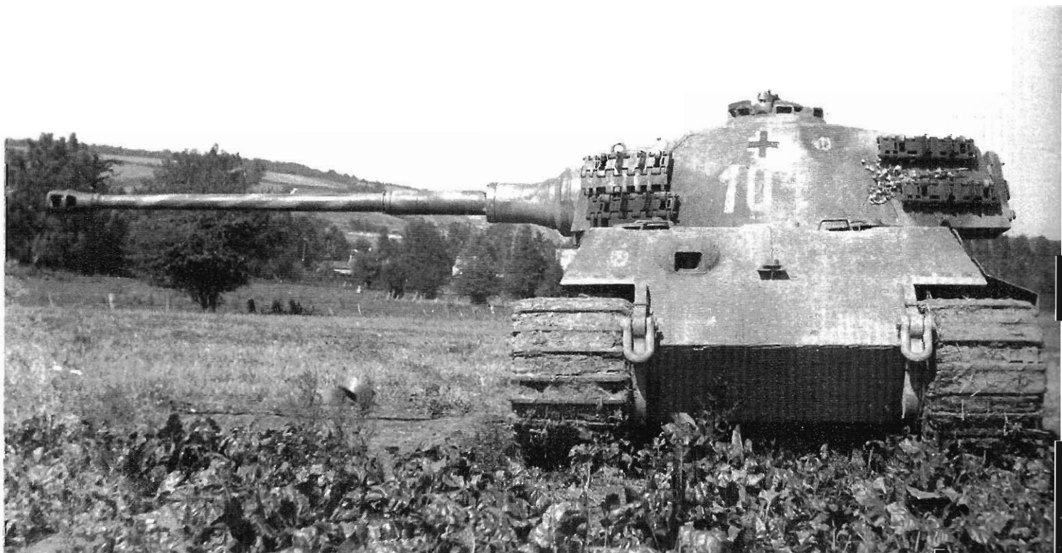
Shown after capture, Tiger Ausf.B (Fgst.Nr.280093, Turm Nr.280124), completed by Henschel on or about 18 July 1944, was issued to 1.Kompanie/schwere-SS-Panzer-Abteilung 101 . Now on display at the College of Military Science in Shrivenham, England, it has the 40 mm thick loader's hatch and the welded base commander's cupola along with three Pilze welded to the turret roof. But it didn't have mounts for the poison gas recognition panels welded onto the top of the gun mantlet and rear of the turret roof. (TMA)
