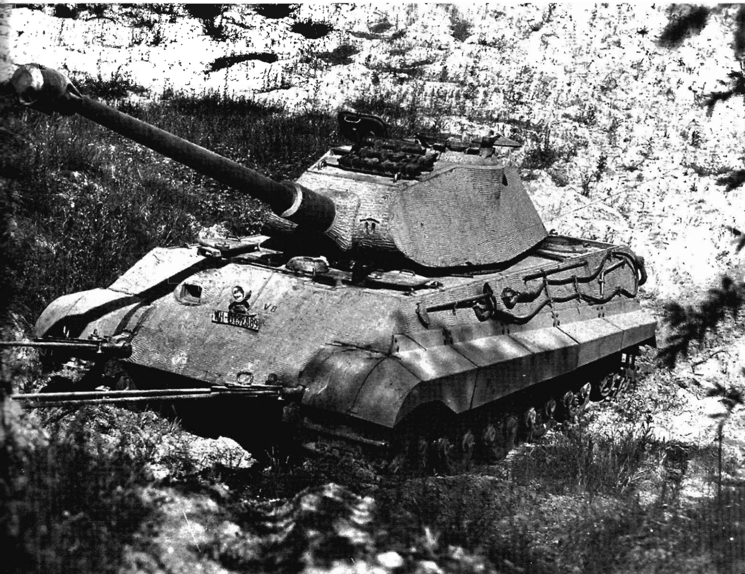
ABOVE: Tiger Ausf.B (Fgst.Nr.280008), completed by Henschel in February 1944, was issued to the Panzerversuchsstelle in Kummersdorf, and identified it by stenciling "212" in a circle and "V8" on the glacis plate. It has Zimmerit (anti-magnetic coating), the curved exhaust pipes, and Gg 24/800/300 cross-country tracks. (BA)
