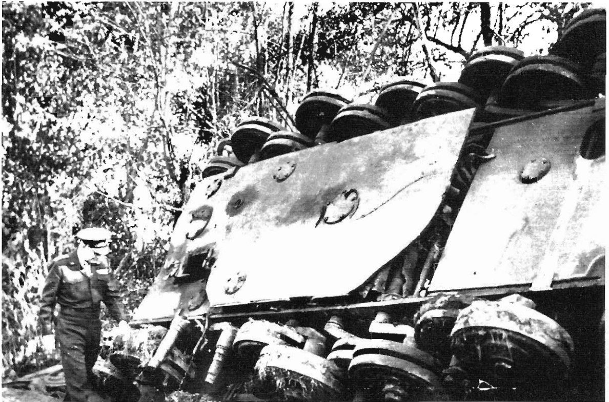
Details of the drain covers and escape hatch on the bottom of the hull are seen in this photo of a Tiger Ausf.B being paid a visit by General Eisenhower. The trailing roadwheel suspension arms on the right side and leading roadwheel suspension arms on the left side are also revealed. (NA)
