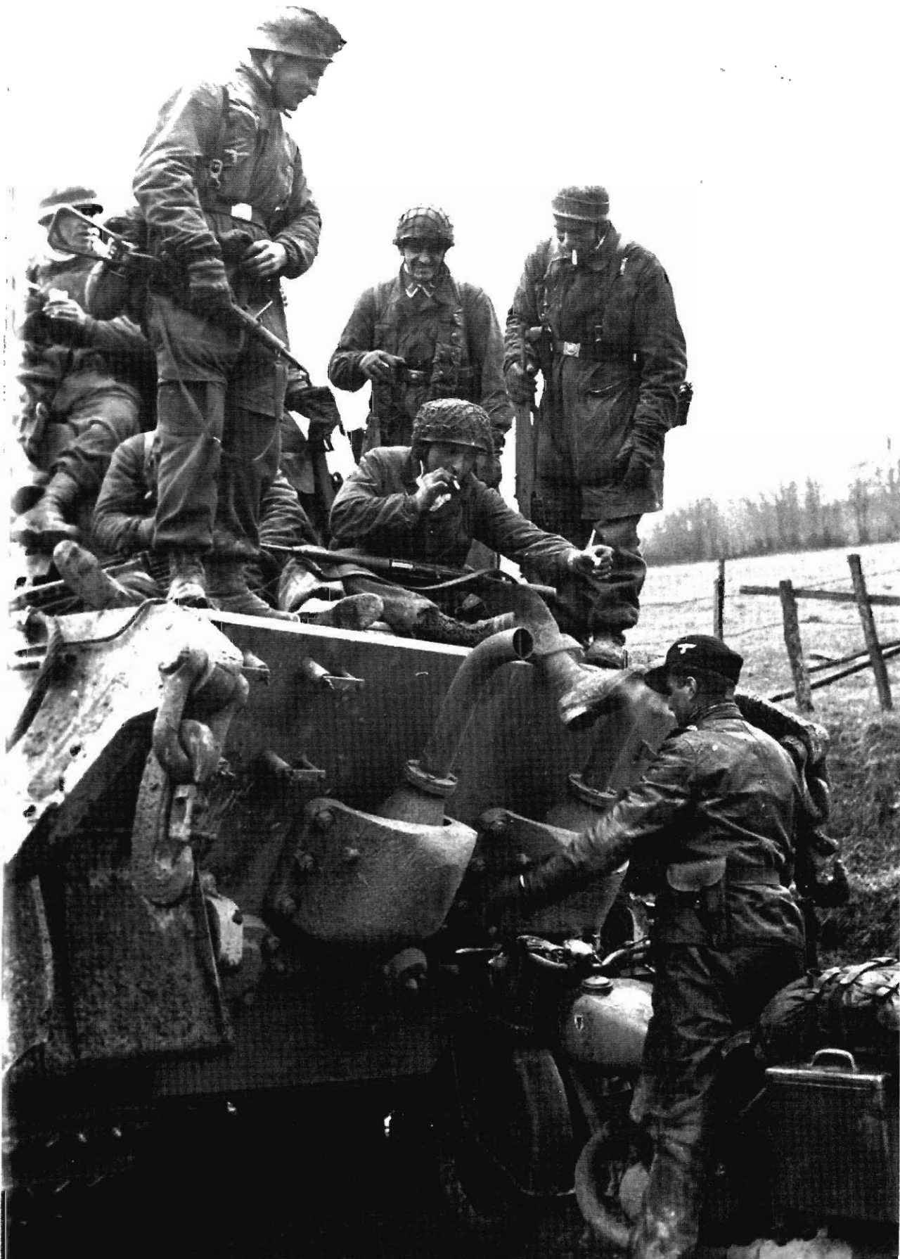
rear of a Tiger Ausf.B completed by Henschel in October or November 1944 and issued to schwere SS-Panzer-Abteilung 501 . The hangers mounting the jack were no longer welded onto the lower rear. The tube for venting the fuel system penetrated the rear deck plate, ran down over the side, and continued forward ending just behind the rear holder for the wrecking bar. (NA)
