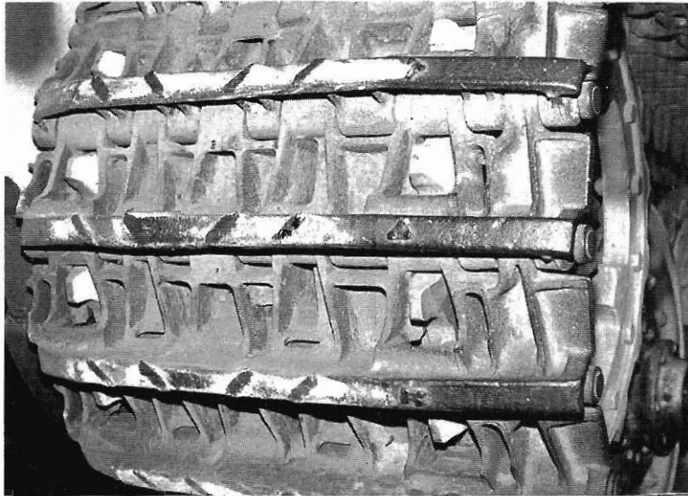
Closeup of the single link Kgs 73/800/152 track with an 18-teeth drive sprocket on Tiger Ausf.B (Fgst.Nr.V2) on display at The Tank Museum in Bovington, England. (TLJ)
