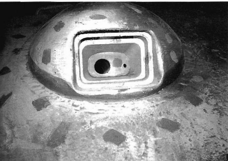
The stepped aperture in the armor guard for the hull machinegun ball-mount that was welded to the glacis plate. The smaller hole was for the Z.F.2 sight.
