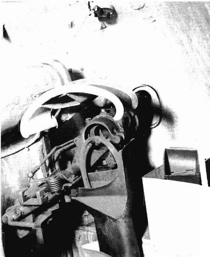
LEFT: The mount for the M.G.34 in the right front corner of Turm Nr.280091 on Tiger Ausf.B (Fgst.Nr.280243). Details of the belted ammunition feed tray, foot-operated firing linkage, and spent cartridge chute can be clearly seen. (NA) RIGHT: The safety switch on the right side of the gun, the loader's hand wheel for the auxiliary traverse, and the boot and lower housing for the gun elevating gear are all seen in this view of the inside of Turm Nr.280091 on Tiger Ausf.B (Fgst.Nr.280243). (NA)
