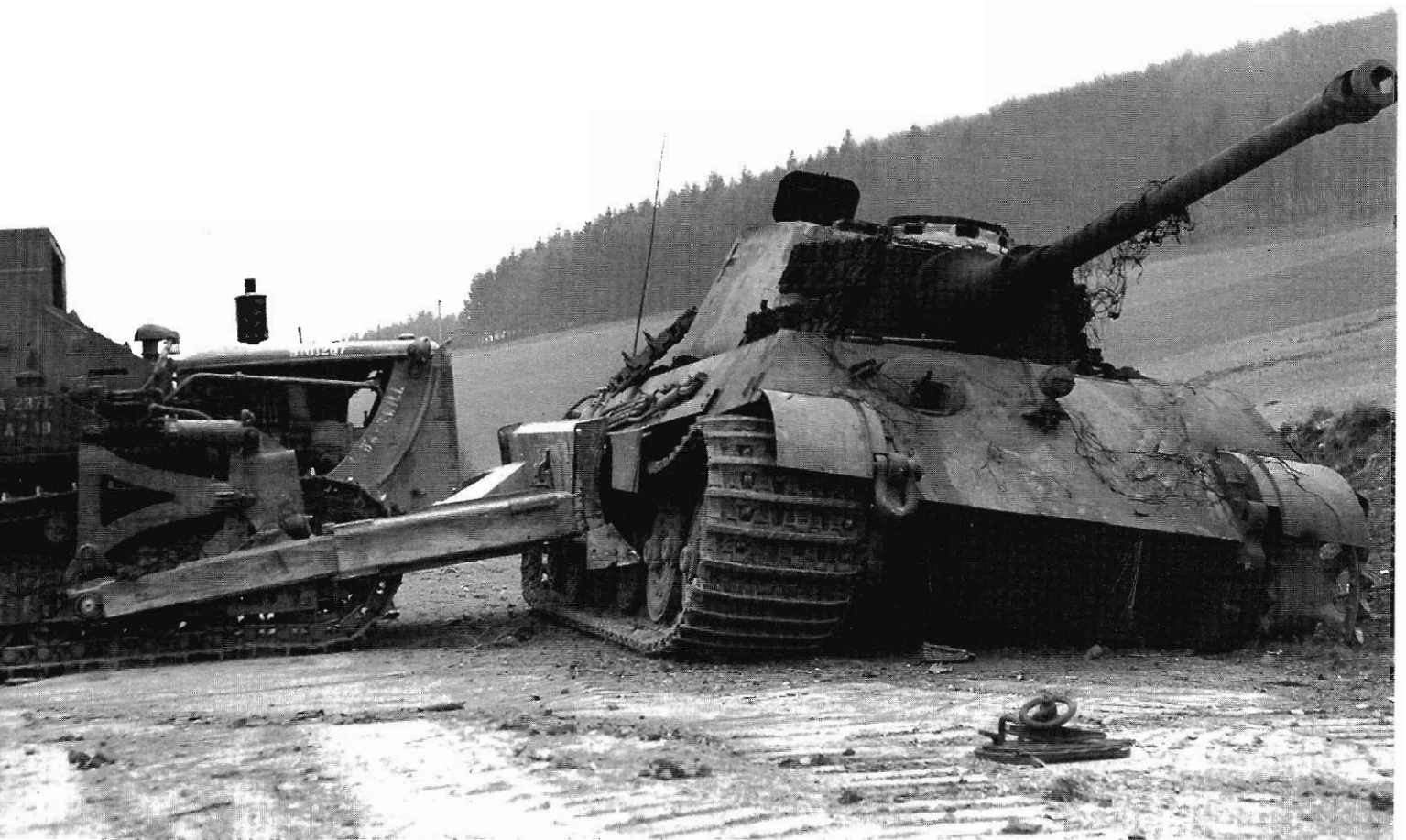
One of the last Tiger Ausf.B , completed by Henschel in March 1945, had the front mud guards with reinforced ribs and the single link Kgs 73/800/152 tracks driven by 18-teeth drive sprockets. Pairs of single link tracks were also hung on the turret sides as spare track links, and the ring for mounting the anti-aircraft machinegun was still welded to the cupola periscope guards.
