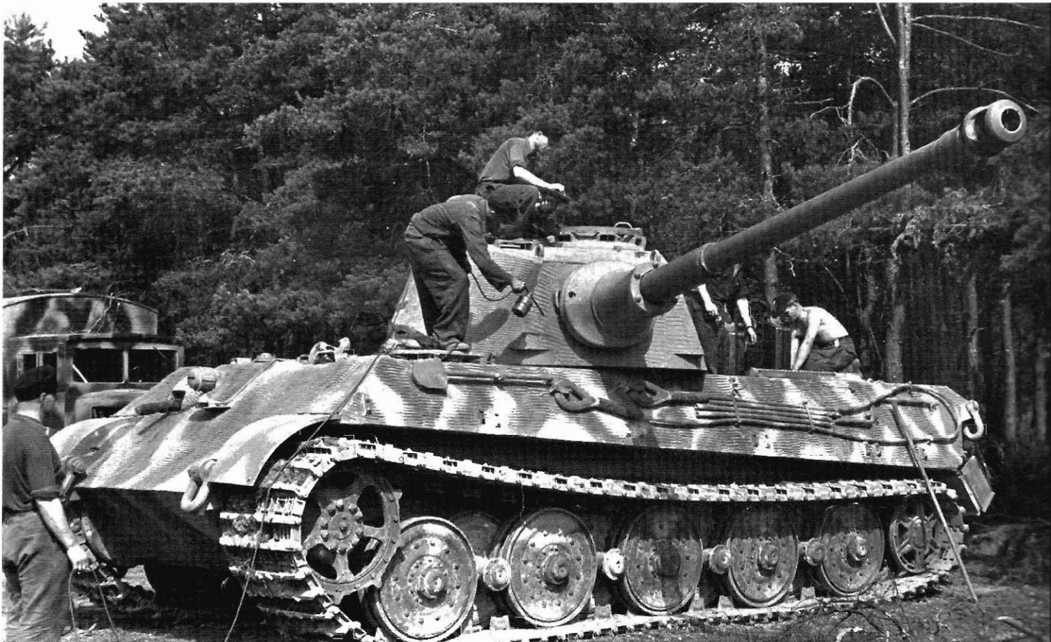
As shown in this photo of a Tiger Ausf. B , completed by Henschel in early July 1944, the maintenance platoon was equipped with an air compressor and was responsible for spray painting the Panzers with camouflage patterns that would blend in with the local terrain. (BA)
