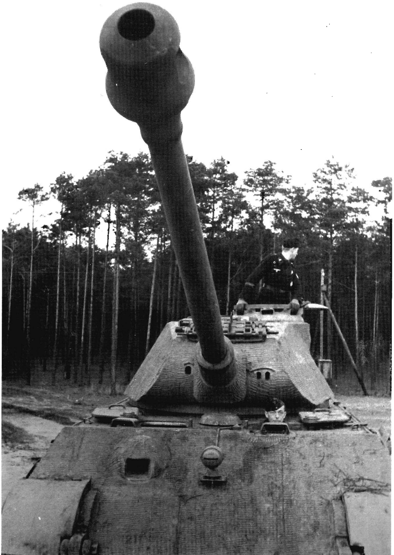
Tiger Ausf.B (Fgst.Nr.280006) , completed by Henschel in February 1944, was issued to the Panzerversuchsstelle in Kummersdorf. It is identified by "211" inside a circle and "V6" stenciled on the glacis plate. It was outfitted with the monobloc 8.8 cm Kw.K.43 L/71 gun with the heavy muzzle brake and the binocular T.Z.F.9b/1 gun sight. It does not have a Turmfugenschutzring (turret ring guard) bolted to the top of the hull. (BA)
