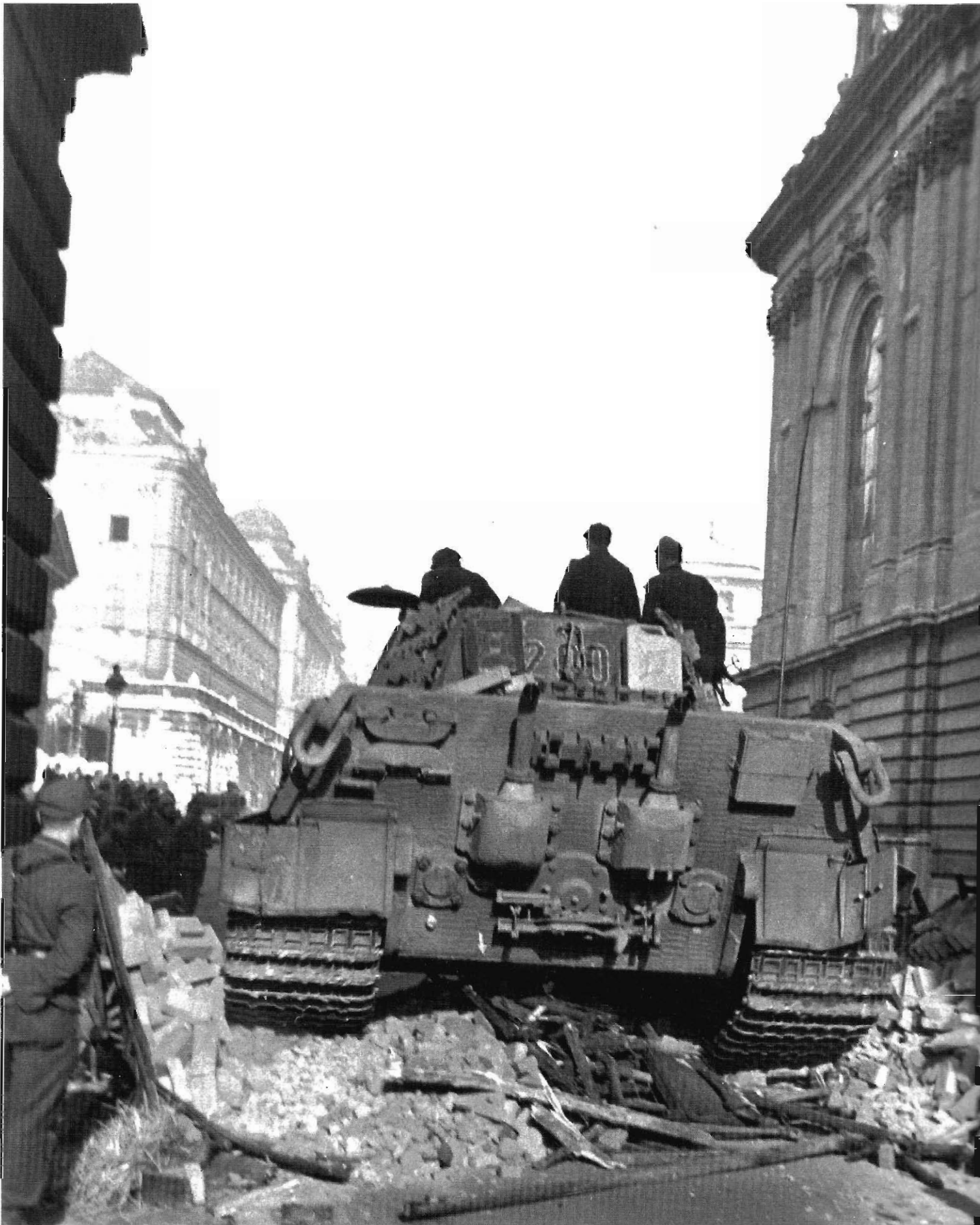
Details of the rear of a Tiger Ausf.B , completed by Henschel in late August/early September 1944 and issued to the schwere Panzer-Abteilung 503 . Very few changes were made to the tool and equipment stowage layout during the production run of the Tiger Ausf.B . The 20-liter "Jerry Can" hung on the turret rear and the track link bracing the exhaust pipes are both examples of crew mods. (BA)
