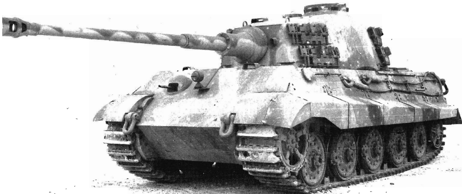
This Tiger Ausf.B completed by Henschel early in 1945 has the extended rain guard welded onto the turret front over the gun sight aperture. It is unique in having the first type of Gg 24/800/300 Gelaendekette (cross-country tracks) hung as spare track links on the turret sides. (WJS)
