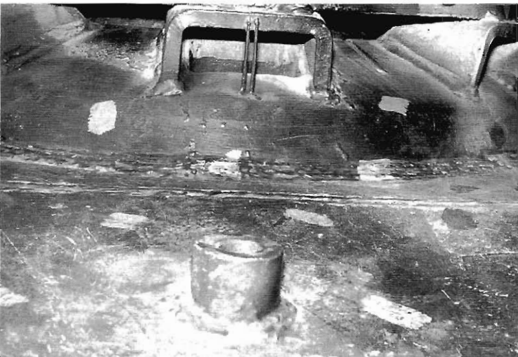
The double wire welded to the front periscope guard, used by the commander to guide the gunner onto target.
