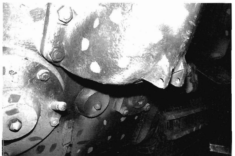
Two palls and the offset port (in the large cover to the rear of the engine) were for the Kurbelwellen-Benzinanlasser (gasoline engine starter). A crank for turning the engine by hand was fed through a ring pivoting on the two eyelets on the exhaust pipe armor guard and inserted into the small port just below the right-hand exhaust pipe.
