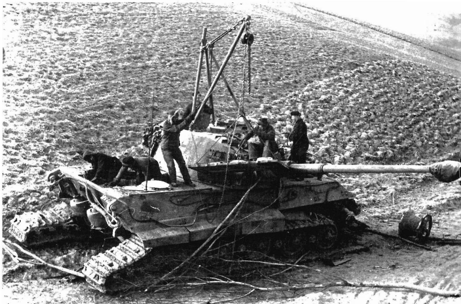
A very rare shot of the Behelfskran 2t , mounted in the three Pilze on the turret roof of this Tiger Ausf.B , being used to remove the rear deck of the engine compartment. The loader's hatch is still the 15 mm thick forging. (BA)
