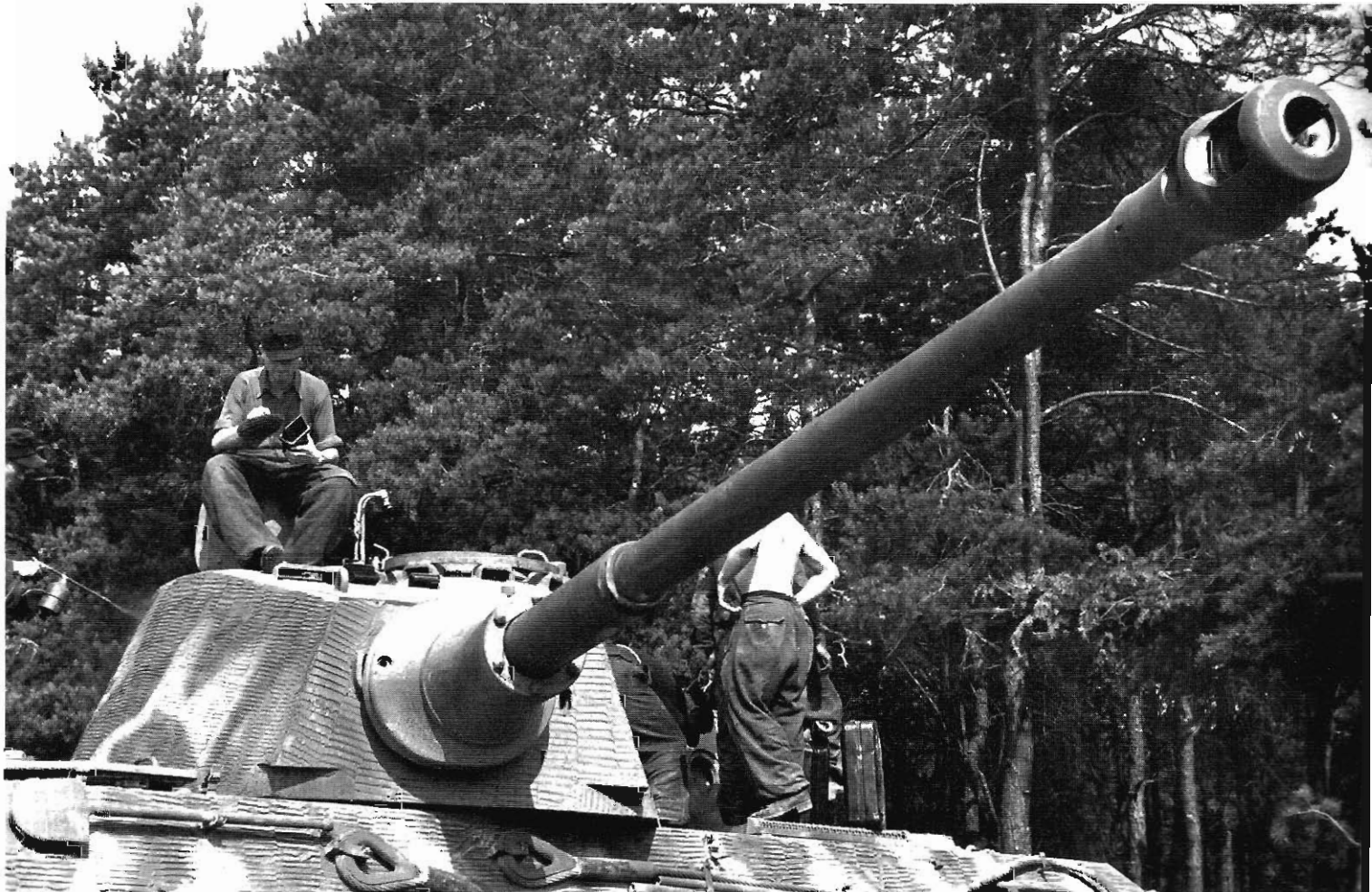
This Tiger Ausf.B with Serien-Turm was completed at Henschel in late June 1944 and issued to the 3.Kompanie/schwere Panzer-Abteilung 503 . It had the new 40 mm thick loader's hatch, three Pilze welded onto the turret roof for the Behelfskran 2t , and the lighter muzzle brake for the 8.8 cm Kw.K.43 L/71 , but didn't have spare track hangers welded onto the turret sides. (BA)
