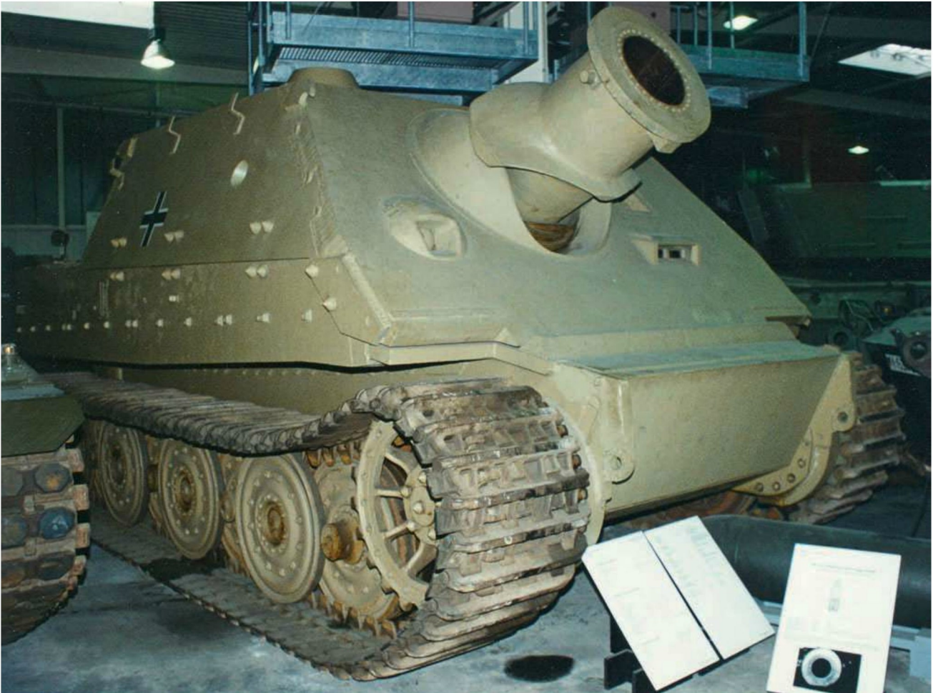
On display at a German military museum is an example of an odd-looking vehicle armed with a large breech-loaded mortar that fired a rocket-assisted projectile weighing more than seven hundred pounds to a distance of almost four miles. The Germans mounted this weapon on the chassis of a Tiger E tank. Michael Green
