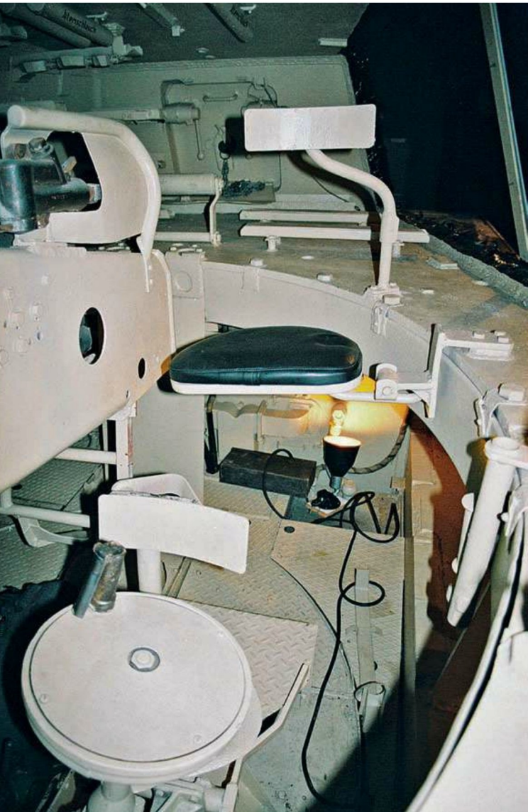
Seats for the Tiger B tank gunner and vehicle commander are visible in this picture. Clearly visible in the foreground is the manually operated traversing hand-wheel for the gunner who sits below and in front of the commander. Both the commander's seat bottom and backrest fold to one side when not required. Michael Green
