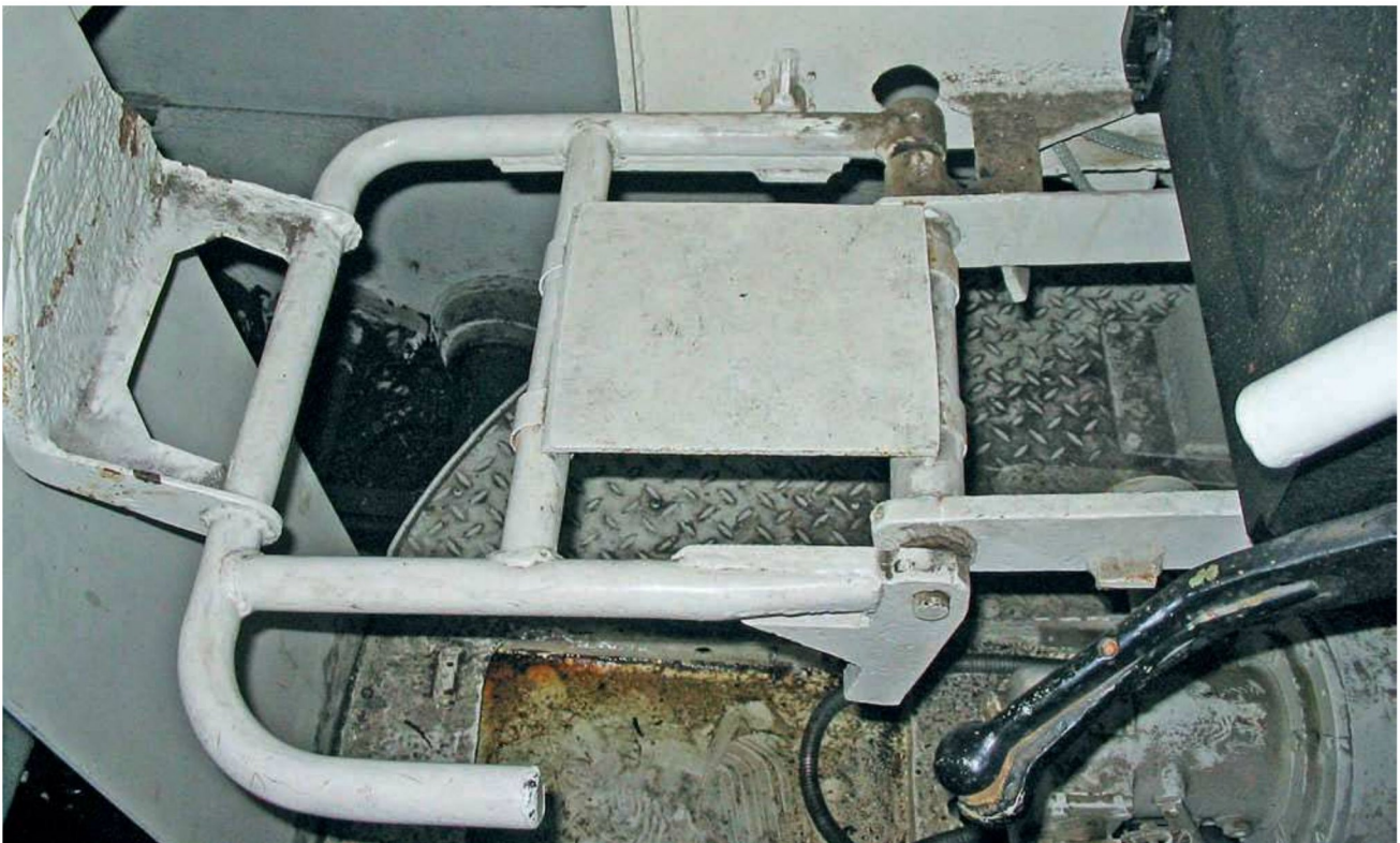
Instead of the canvas sack that caught the ejected spent main gun cartridge cases on the Tiger E tank, the Tiger B tank featured a foldable metal tray behind the breech housing. When a spent metal cartridge case ejected from the breech, it struck the deflector plate seen at the rear of the tray, and then dropped onto the tray, at which time the loader picked it up and hurled it out a small overhead hatch. Frank Schulz
