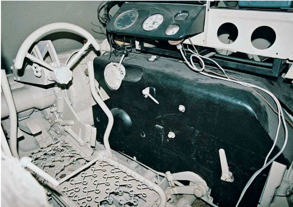
The driver's position on a Tiger B tank with the steering wheel and the large transmission housing, which separated the driver from the radioman, located on the other side of it. Also seen in this picture is the shift control unit for the driver and the two backup steering levers on either side of his seat. Michael Green
