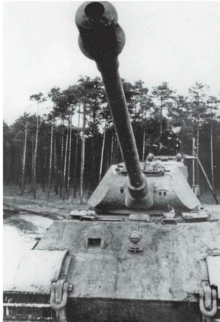
The Tiger B tanks fitted with Krupp/Porsche turrets featured an articulated binocular sighting system like the ones on many Tiger E tanks. The two openings in the front of the tank's turret for the binocular optical sighting system are clearly visible in this head-on photograph of a Tiger B tank fitted with a Krupp/Porsche turret.
