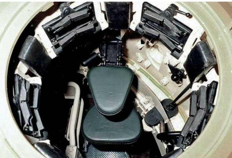
Looking down the tank commander's hatch on a Tiger E tank, featuring the original drum-type cupola, both of the commander's seats are visible. The upper seat allowed the tank commander to sit and to look out over the top of his cupola, while the lower seat allowed him to sit and look out through the vision slits of the cupola. Tank Museum, Bovington
