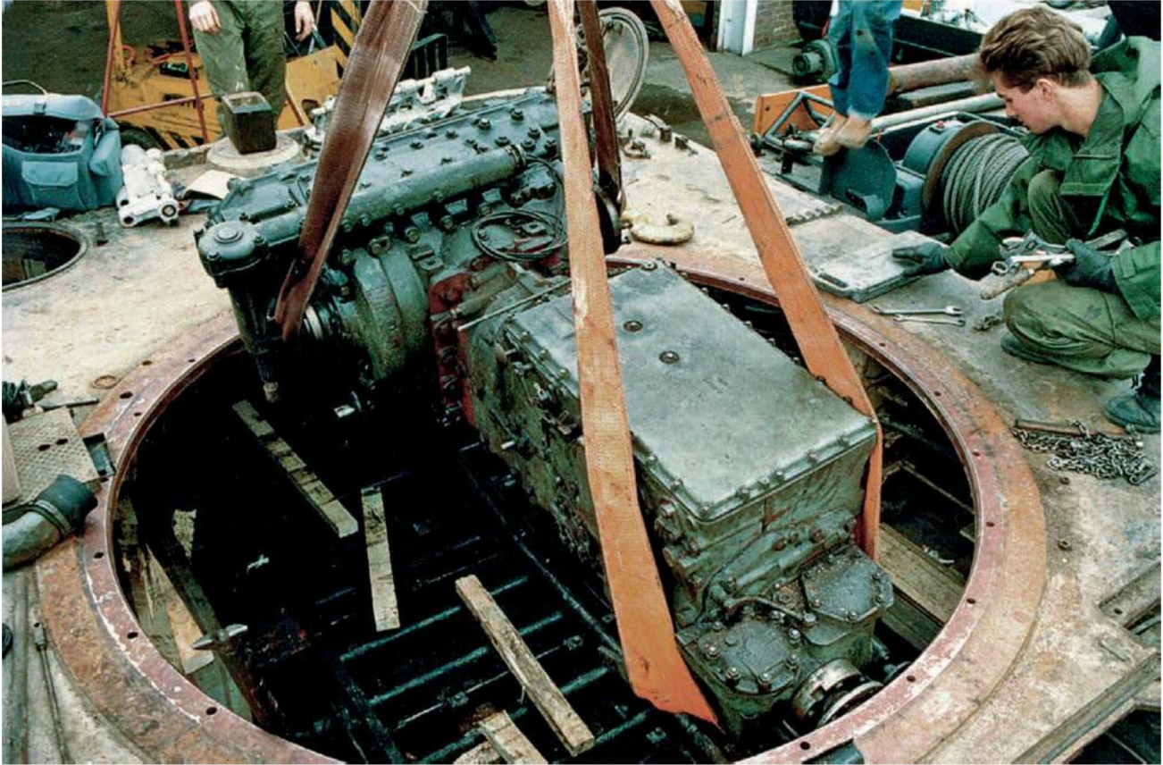
This photograph shows the transmission and steering unit coming out through the turretless hull of the Tiger E tank, belonging to the collection of the Tank Museum located at Bovington, England. At the bottom of the vehicle's hull can be seen some of the tank's torsion bars. Tank Museum, Bovington
