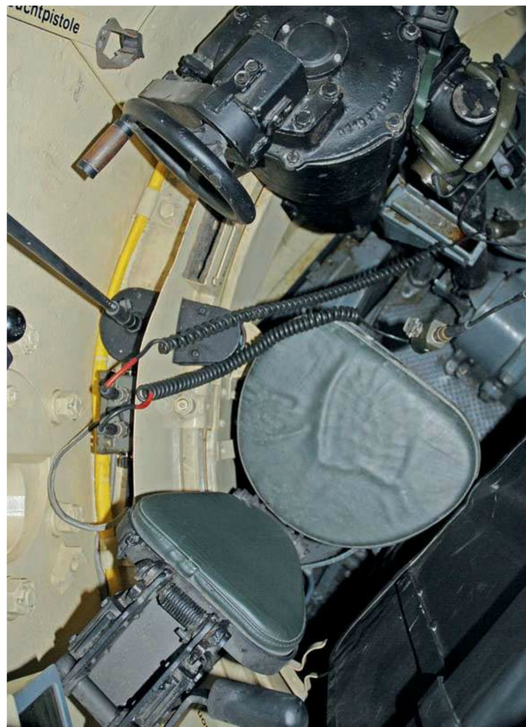
Visible looking down through the tank commander's hatch on a Tiger E tank is the commander's lower seat position. The upper seat folds down and acts as a backrest while the commander sits on the lower seat. To the upper right-hand side of the picture is his manually operated hand-wheel for turning the turret. Tank Museum, Bovington
