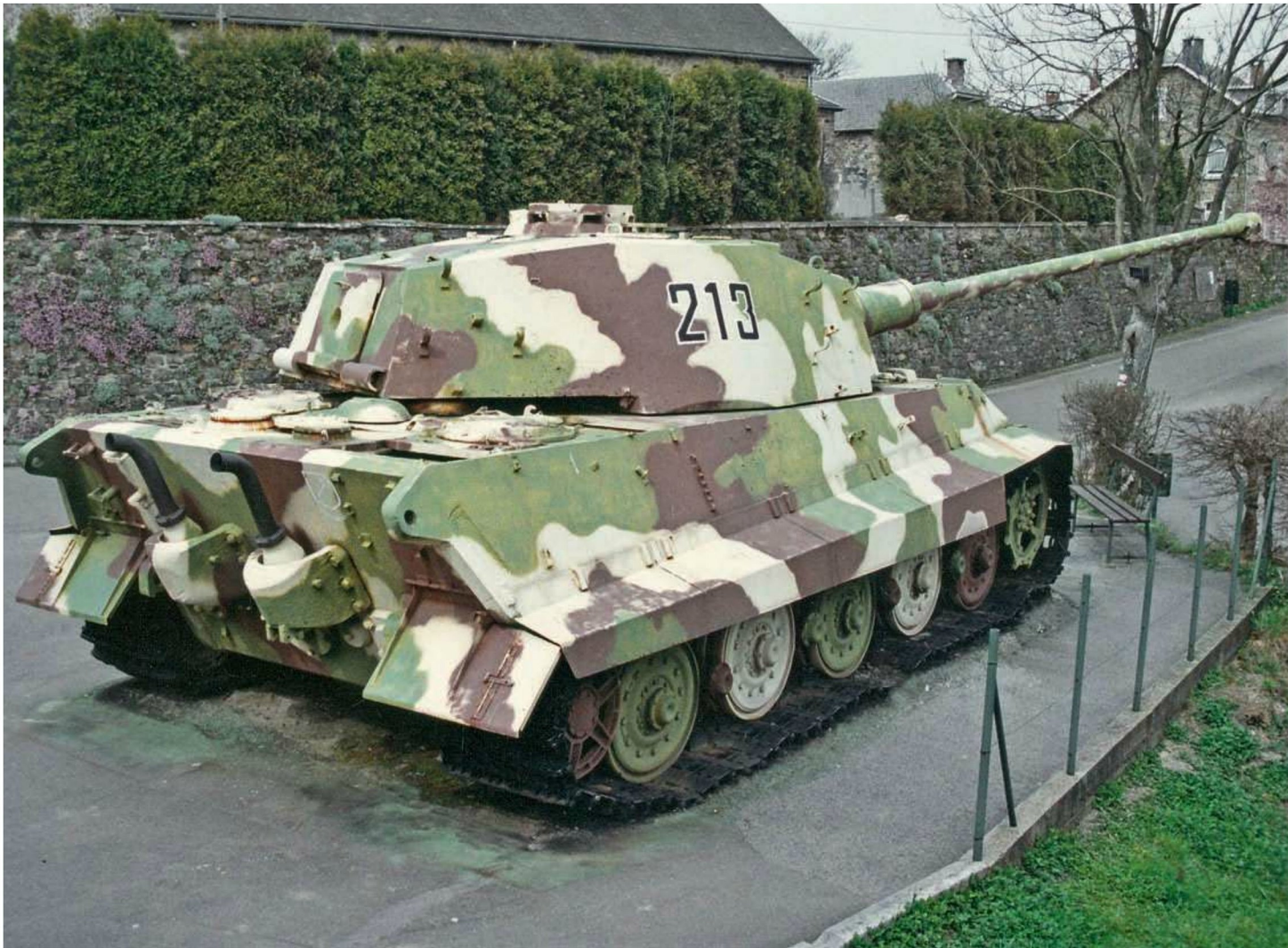
A Tiger B tank shows the long overhang of the rear turret bustle, which not only acted as a counterweight for the long and heavy main gun, but as additional storage space for main gun rounds. This particular example lacks the typical external storage features seen on wartime vehicles. It does feature the typical twin curved engine exhaust pipes on the rear hull plate. Andreas Kirchoff
