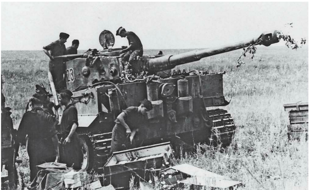
To fill certain main gun ammunition storage bins on the Tiger E tank, the crew had to rotate their turret to a rearward position, as is visible in this picture. This is not something normally done in the heat of combat, but it will often take place during lulls in action. Although a dangerous practice, crews on all sides often carried extra ammunition in extemporized stowage locations around the fighting compartment to avoid running out. Patton Museum
