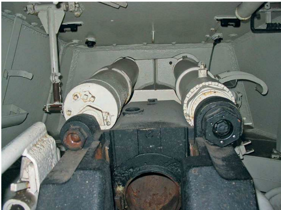
Located above the gun housing and barrel of an 8.8cm main gun, inside the turret of a Tiger B tank, are the two long cylinders that comprise the tank's recoil system. A recoil system is a mechanism designed to absorb the energy of recoil gradually and so avoid violent movement of the gun mount. Frank Schulz
