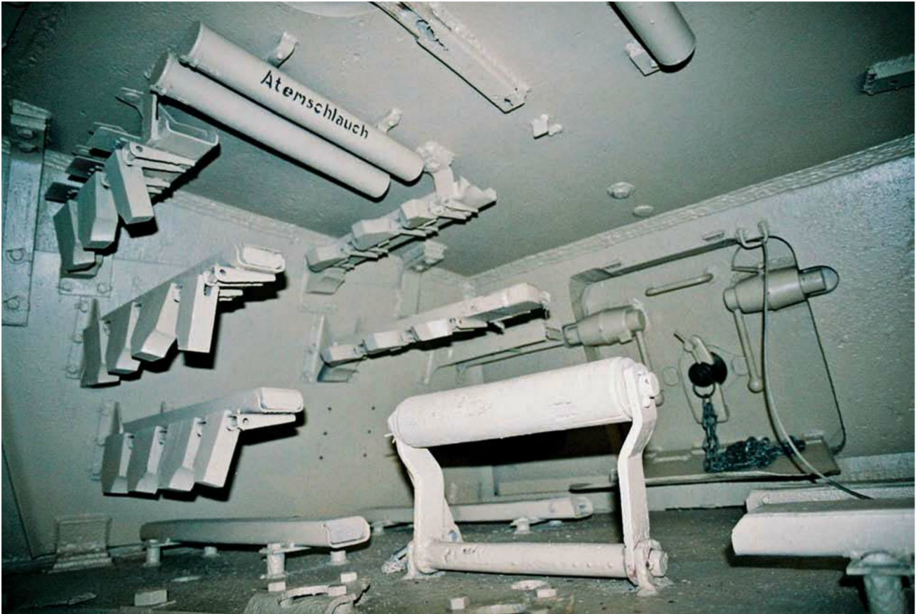
Looking backward and upward from the gunner's position on an Tiger B tank, some of the horizontal racks that held main gun rounds are visible in the turret bustle of the vehicle, as is the fold-down roller used by the vehicle's loader to assist him in manhandling the rounds into the breech of the 8.8cm main gun. Michael Green
