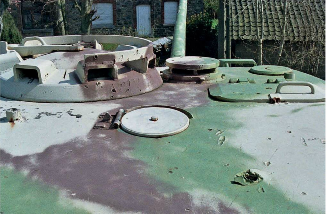
A picture from the rear of a Tiger B tank turret shows the tank commander's cupola, the loader's hatch, and the upper portion of the electrically powered ventilation turret fan. The smaller feature on the turret centerline is a port through which the loader disposed of spent main gun cartridge cases. Andreas Kirchoff
