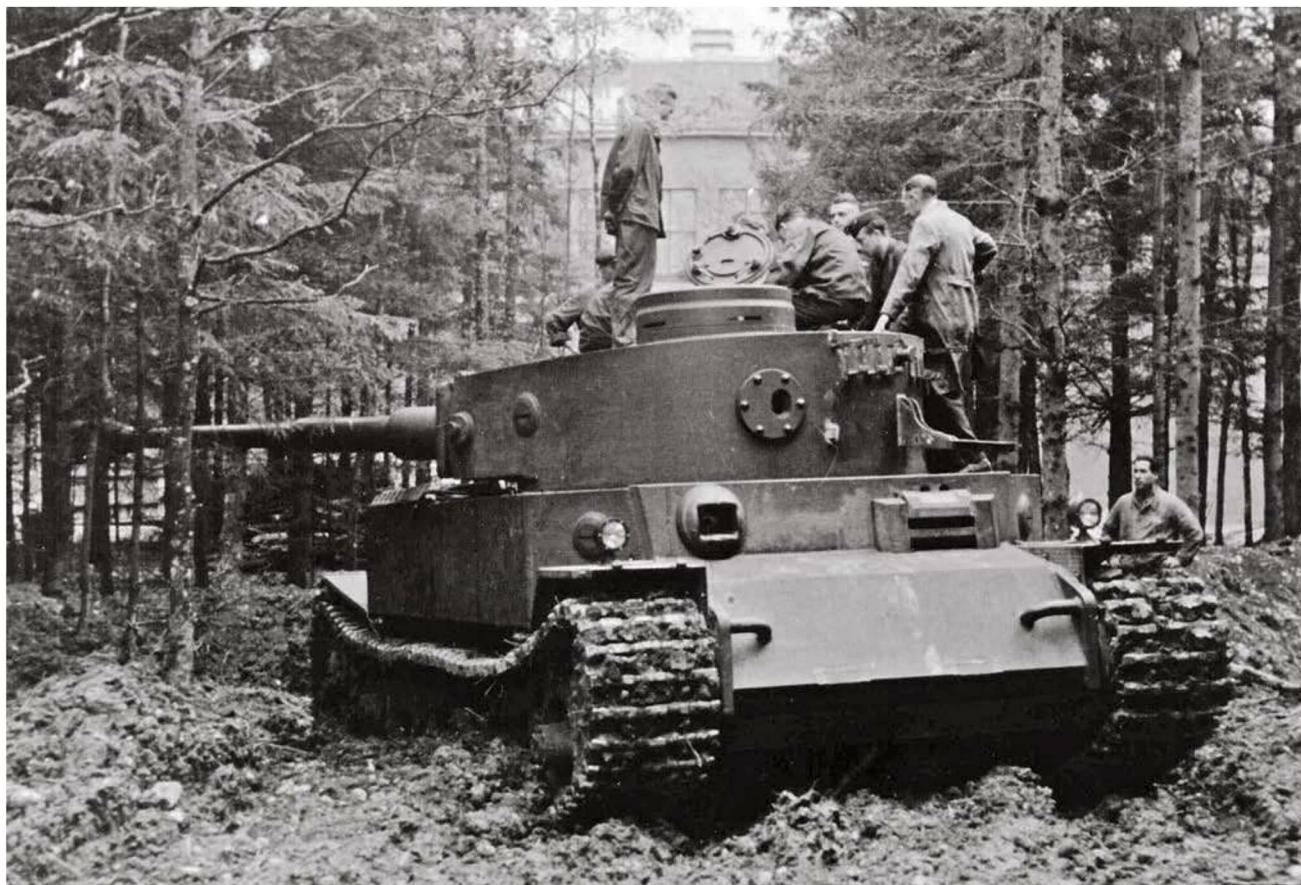
The Porsche-designed chassis for the German army's heavy tank competition appears on a forest trail during mobility testing. Dr. Ferdinand Porsche loved to innovate and came up with some very interesting concepts for his vehicle, including a gasoline-electric drivetrain. However, the rush to field a heavy tank left little time to work the bugs out of his untested concepts. Patton Museum
