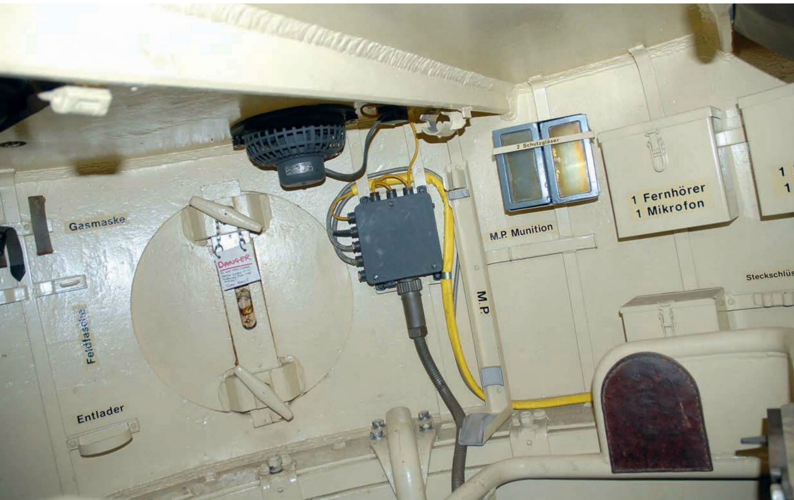
Looking rearward from the gunner's position on a Tiger E tank, the loader's escape hatch is visible. Overhead is the bottom portion of an electrically powered ventilation fan, with the upper portion projecting out over the top of the turret roof under an armored housing. Tank Museum, Bovington
