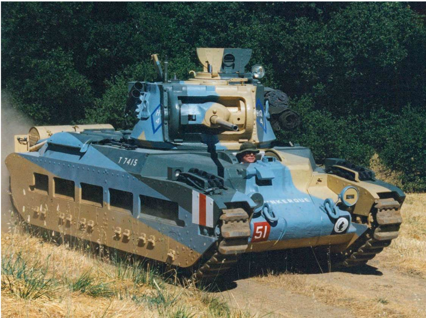
The British Matilda II infantry support tank armed with a 40mm main gun featured armor protection up to three inches thick. The thickness of the tank's armor made it immune to almost all the German army tank and antitank guns in the battle for France in the summer of 1940. Michael Green
