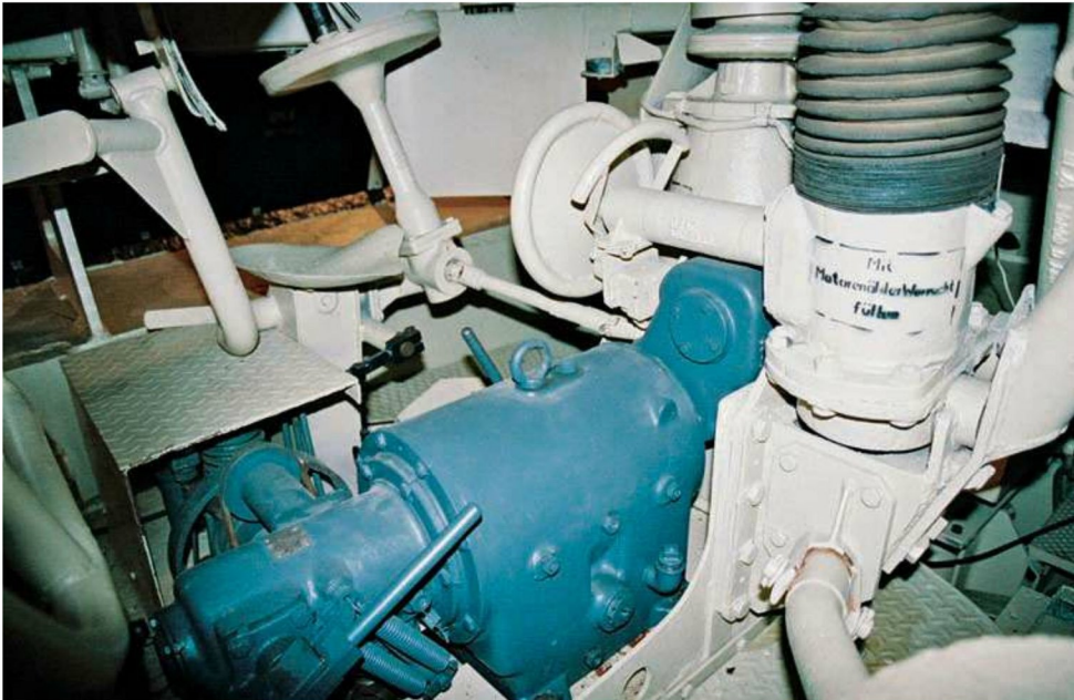
On the bottom of the turret basket floor of a Tiger B tank (painted in blue) is the vehicle's hydraulic turret traversing pump. Also visible is the gunner's elevation hand-wheel, with the firing handle located directly behind it and the gunner's traversing hand-wheel. Behind the gunner's seat, under the diamond plate sheet metal box, is the vehicle's air compressor (also painted in blue). Michael Green
