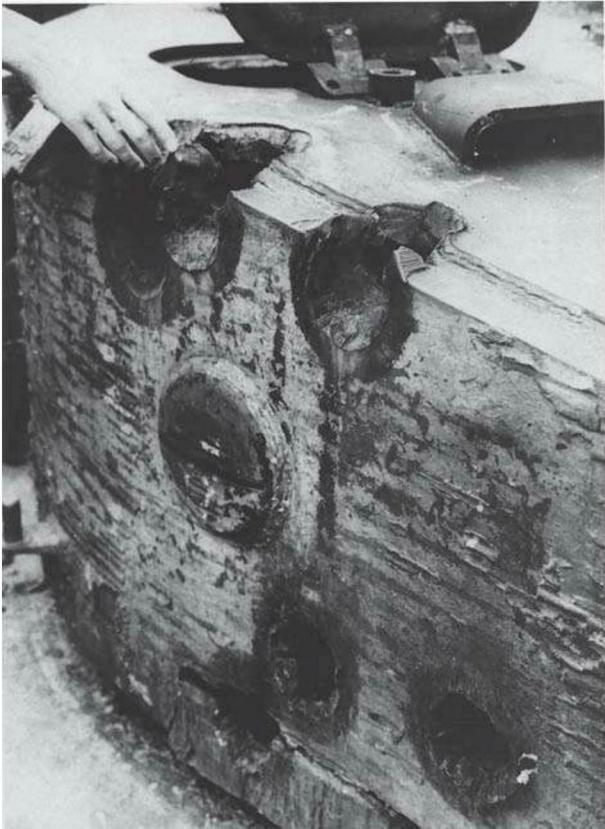
The turret wall of a Tiger E tank, on the loader's side of the tank, has taken numerous large-caliber hits from AP projectiles. The strikes on the upper portion of the tank's turret buckled the turret roof plate, while the lowest hit on the turret wall fractured the armor along a horizontal seam. Patton Museum
