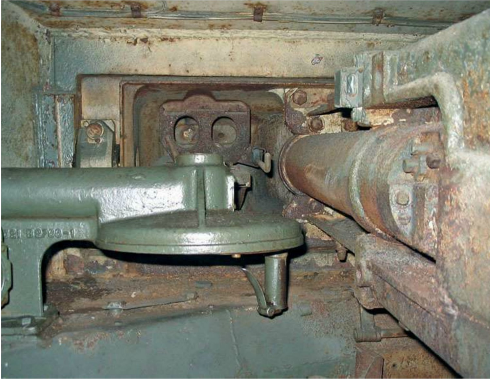
The Tiger E power traverse did not always offer enough control for good shooting accuracy, so once near the target, the gunner often refined his aim with the hand-wheel visible in the foreground. He could turn it as he looked out through the gun shield with his optical sights (missing in this vehicle although the bracket for mounting them remains). The gun mount is at the right in this view. Frank Schulz
