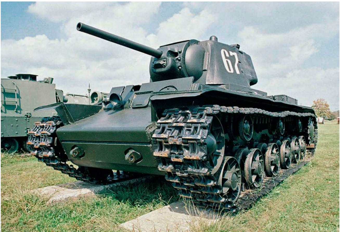
The Red Army KV-1 heavy tank mounted the same 76.2mm main gun as found on the T34/76 medium tank and boasted much thicker armor that made it even harder to kill by German tank and antitank guns. Only the German 88mm anti-aircraft gun had a chance of penetrating the KV-1's thick armor hide. Michael Green
