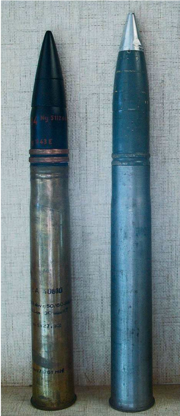
On the left of this picture is an 8.8cm Pzgr 39 AP round fired from the 8.8cm main gun on the Tiger E tank. On the right is a Sprenggranate (Sprgr) HE fragmentation round for the same gun, intended for engaging thinly armored or nonarmored targets. Unlike the Pzgr 39 AP projectile, the HE projectile has an adjustable fuse on its tip. Michael Green
