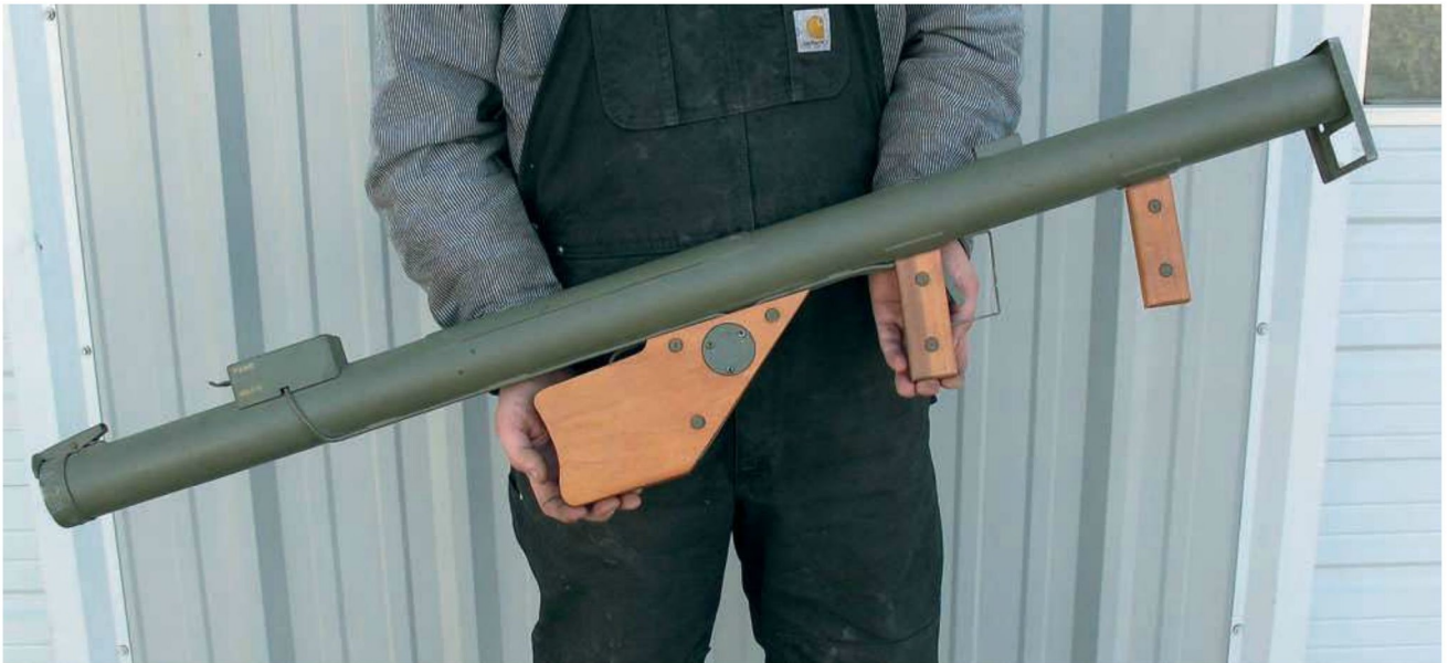
The American M1 2.36-inch Bazooka, pictured here, was a rocket-firing weapon, with a small shaped charge warhead that gave the average infantryman at least a chance of destroying enemy armored vehicles, Tiger tanks being a little iffy. The problem was that to be effective, a soldier had to be at close range to the intended target, which left him vulnerable to enemy counter fire. Michael Green
