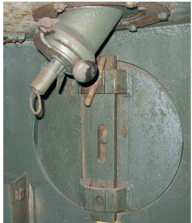
This picture shows a Krupp/Henschel turret roof. Visible on the roof of the vehicle's turret is the small circular exterior opening, just behind the loader's hatch, for the small traversable breech-loading mortar attached to the turret roof of the tank. Also visible is the loader's front turret-mounted periscope and the upper portion of the turret exhaust ventilation fan. Patton Museum
