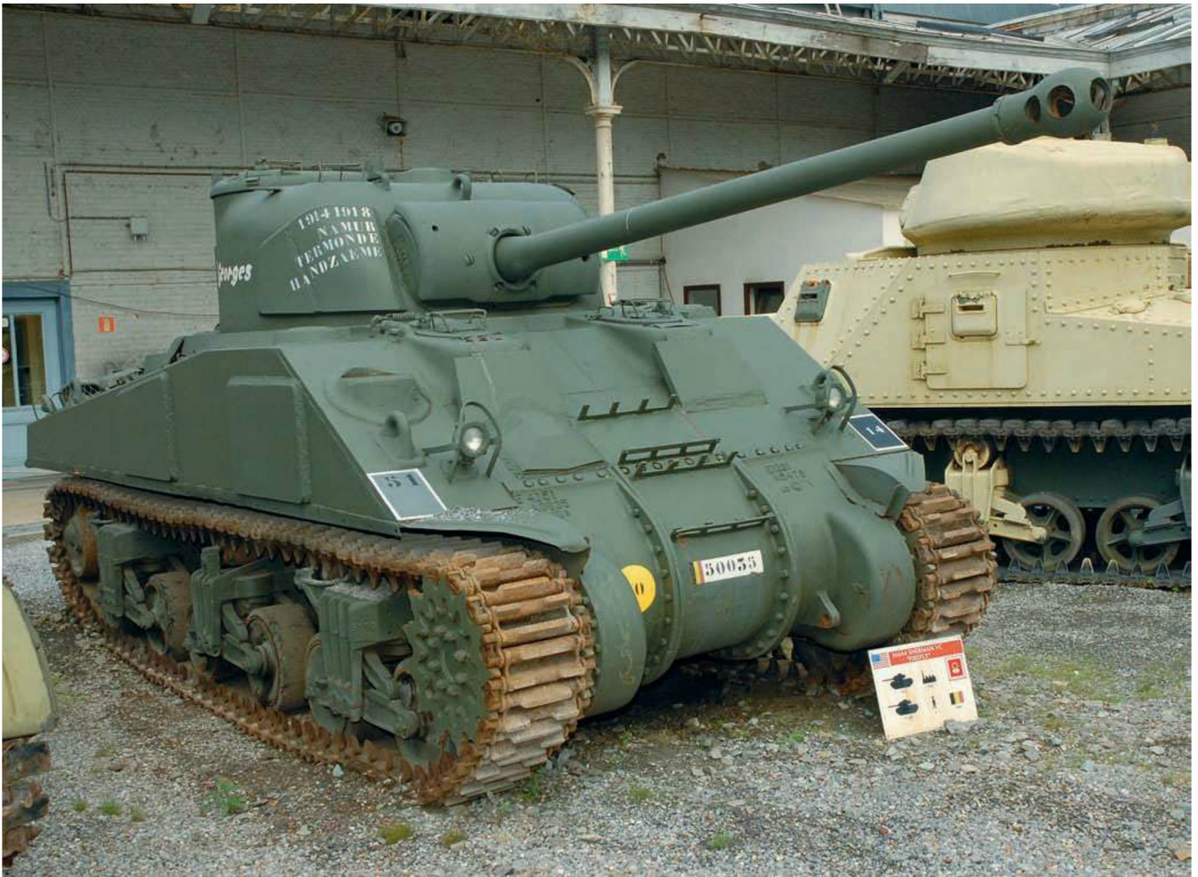
The only versions of the U.S. Army M4 Sherman medium tanks that mounted a main gun with sufficient penetrative powers to be able to defeat the thick armor on Tiger tanks proved to be those armed with the British army's tank gun version of their seventeen-pounder (76.2mm) antitank gun. An example of one of these tanks is on display at the Belgian Army Museum in Brussels. David Marian
