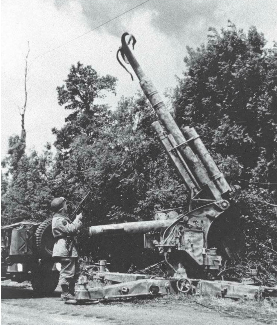
An American soldier looks at the destroyed remains of a German 8.8cm anti-aircraft gun at the side of a French road. The weapon fired a twenty-one-pound projectile to an effective ceiling of about 26,000 feet. A well-trained 8.8cm gun crew could manually load and fire up to fifteen rounds per minute. National Archives
