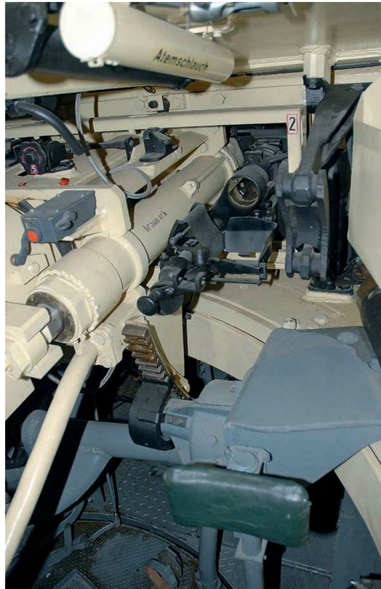
The mounting bracket for the coaxially mounted 7.92mm machine gun (not fitted in this picture) is visible on the loader's side of this Tiger E tank. Also visible is the elevating arc and elevating pinion for raising and lowering the tank's main gun, as well as the loader's seat. Tank Museum, Bovington
