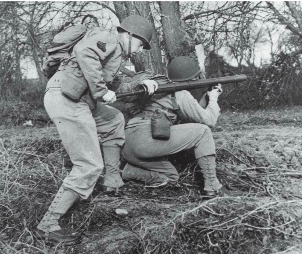
In this U.S. Army wartime training picture of a two-man bazooka team, the soldier in the rear is inserting the shaped charged-equipped rocket into the rear of the long metal tube that made up the weapon. With the rocket hooked up to the electrical firing system, the loader would tap the soldier holding the bazooka on the helmet to let him know that he could fire the weapon. National Archives
