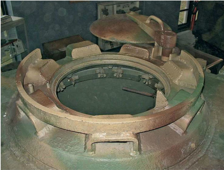
Beginning in July 1943, a new low-profile tank commander's cupola, as seen here, began appearing on Tiger E tanks with an attachment rail for a 7.92mm machine gun. This new cast armor cupola featured seven periscopes arrayed around its circumference that had external armored hoods. The hatch cover pivoted to open, and thus did not project above the tank. Frank Schulz
