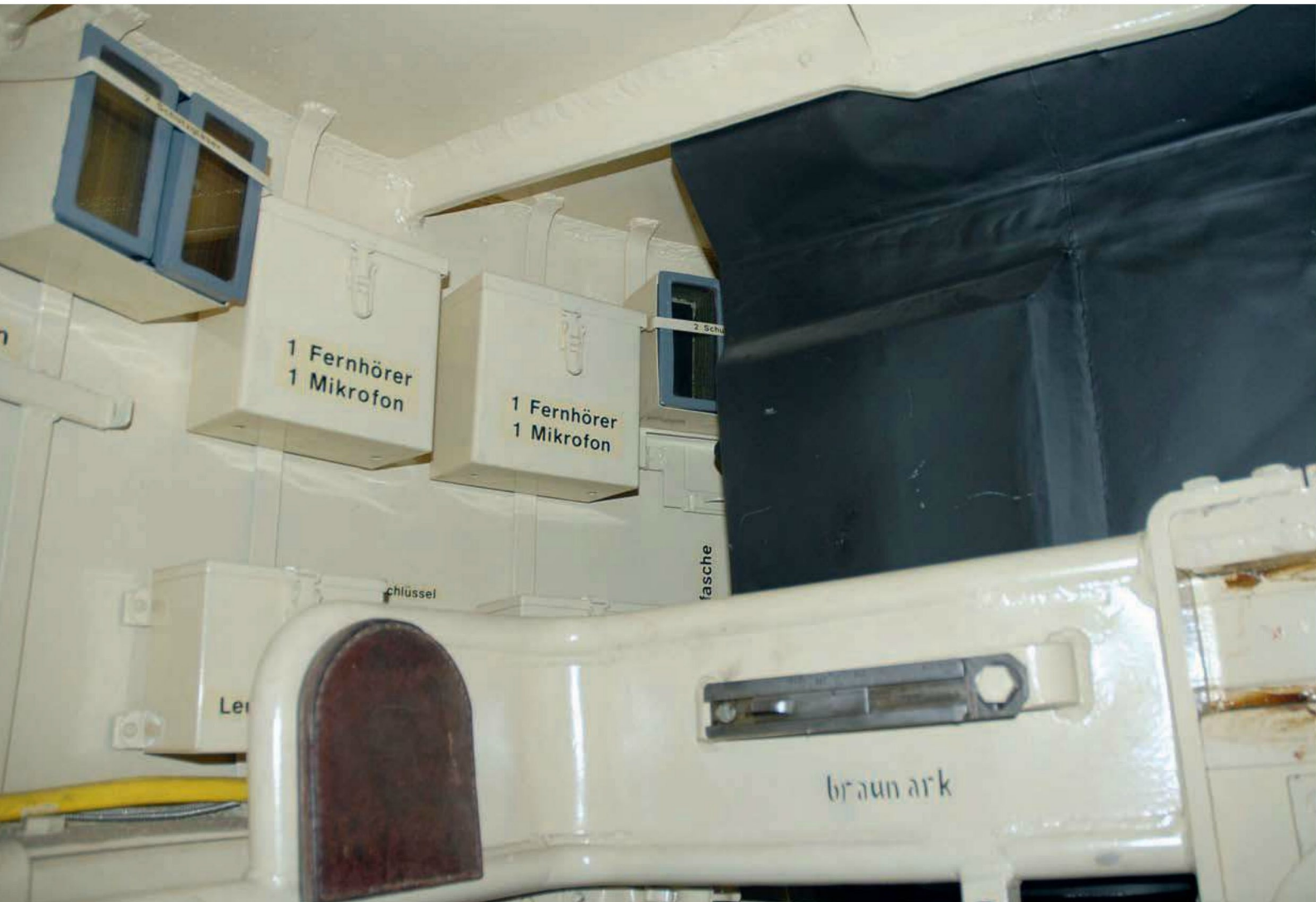
Taken from the loader's position (looking rearward) is this view of the right side of the recoil guard. Also visible is the sheet metal guard that protects the commander from any main gun back-blast when the breech opens. Visible at the rear portion of the recoil guard is a pad that the spent main gun cartridge cases strike on ejection from the main gun upon counter-recoil. Tank Museum, Bovington
