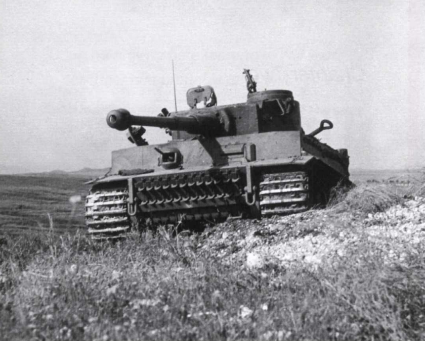
LEFT This photograph of Tiger 131 was taken on 22 April while shells landed nearby; the photographer is sheltering in a vacated German foxhole. Damage to the loader's hatch can be clearly seen and the towing cable appears to be loosened – perhaps ready for use. Note the absence of material on the front glacis plate. No one has yet started to remove items from the interior.
