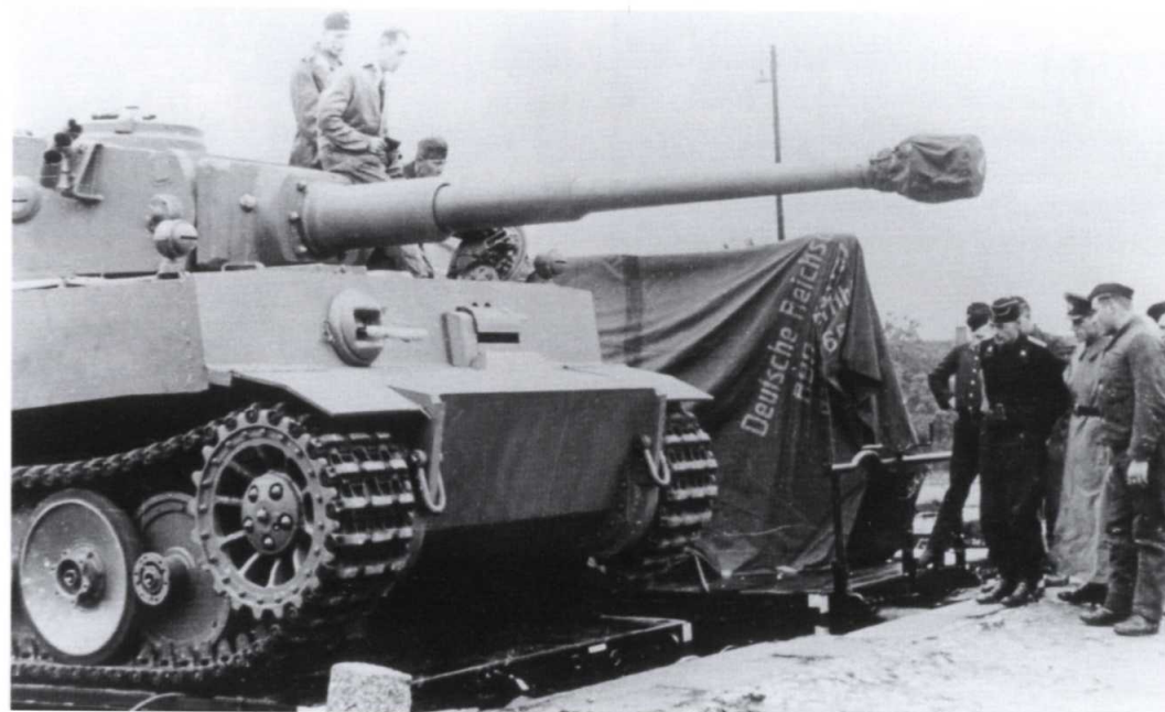
RIGHT This Tiger, being loaded onto a railway flat, has the narrower transport tracks fitted.
