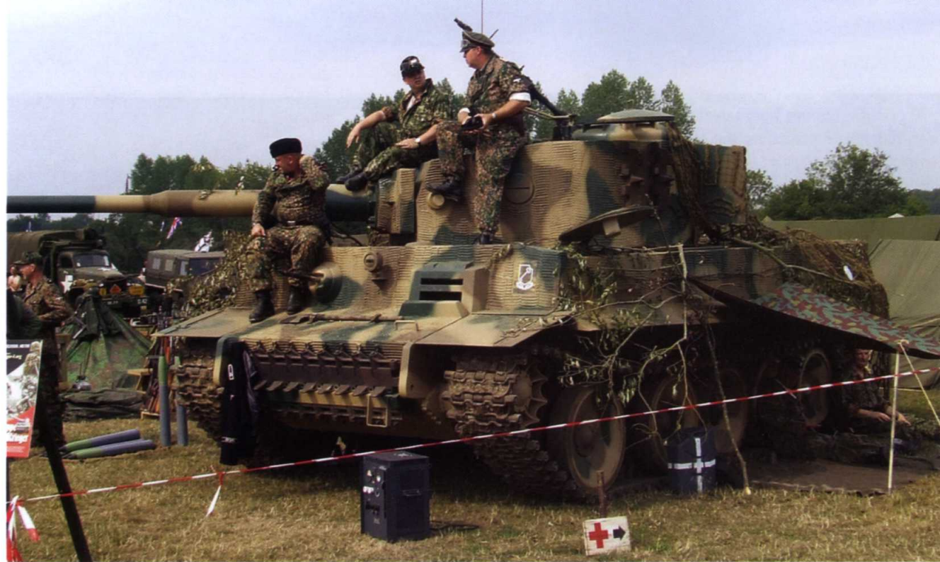
ABOVE AND BELOW A replica Tiger built on a T-54 chassis – perfect for re-enactors.
