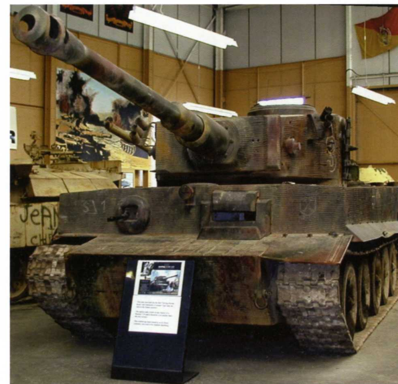
ABOVE A Tiger mock-up based on a T-34/85 chassis, made for the film Saving Private Ryan .
