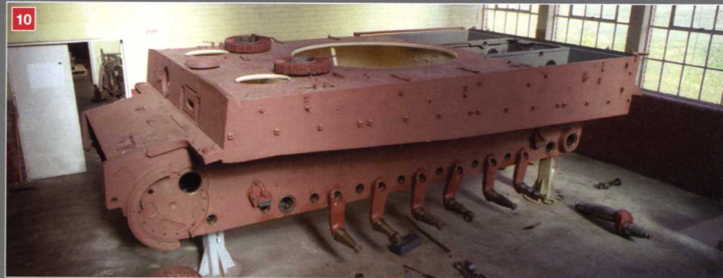
8 The hull stripped and shot-blasted.
