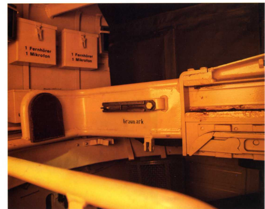
BELOW Looking back from the breech. The bar in the foreground stopped the loader from accidentally getting behind the recoiling breech when firing. The leather stop pad cushioned ejected empty propellant cases. The two boxes mounted on the turret wall contained a set of headphones and throat microphone. The black tin sheet on the far side of the breech was to protect the commander from any back-flash coming from the breech opening after firing.
