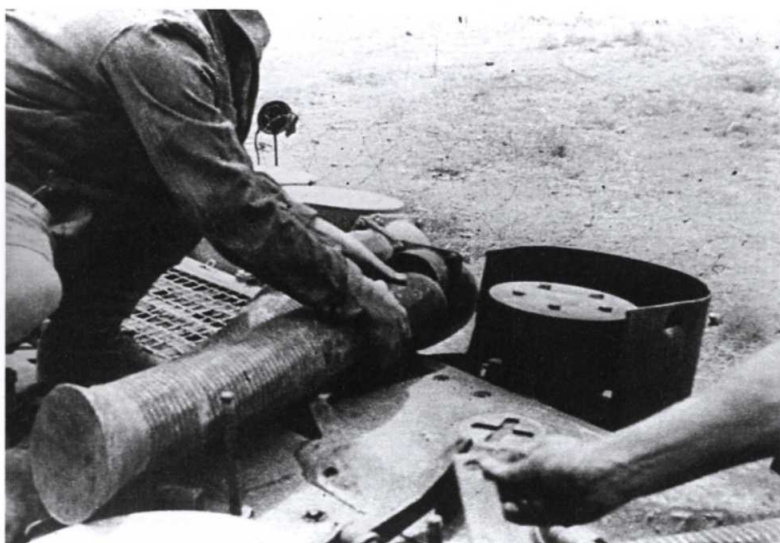
BELOW Fitting the Feifel air filters.
