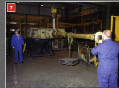
7 Removal of the gun mantlet.
