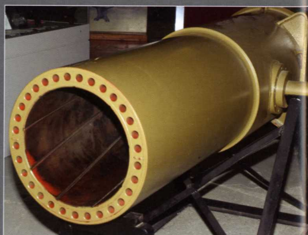
BELOW The mortar tube from the Sturmmörser . Marked as 'R19', 'Piece 19', the rifling inside the barrel to impart spin to the round can be seen.
