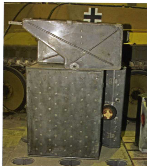
RIGHT The petrol tanks ready for refitting in the side panniers.
