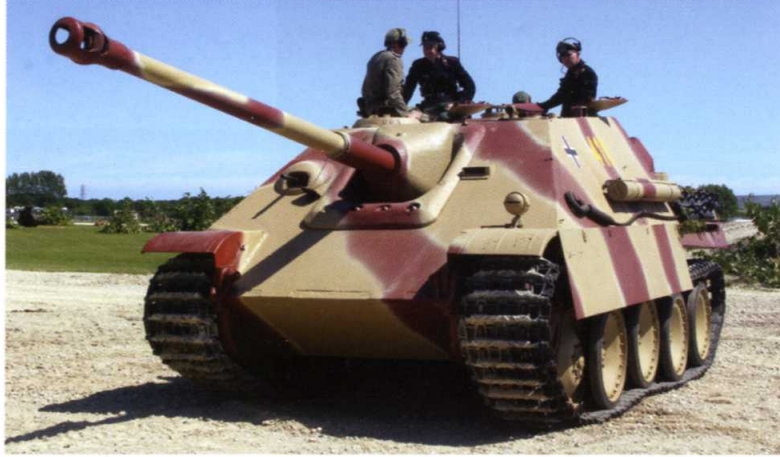
ABOVE The SdKfz Military Vehicle Foundation's Jagdpanther SdKfz 173 at Tankfest. This camouflage scheme was introduced during the Second World War as a paint-saving measure. A third of the red oxide primer was left uncovered.
