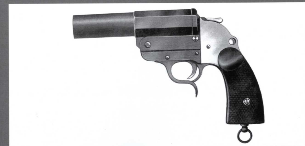
LEFT The Leuchtpistole or 2.7cm flare pistol. Firing a single cartridge it was mainly for communications, but it could also be used for launching grenades.
