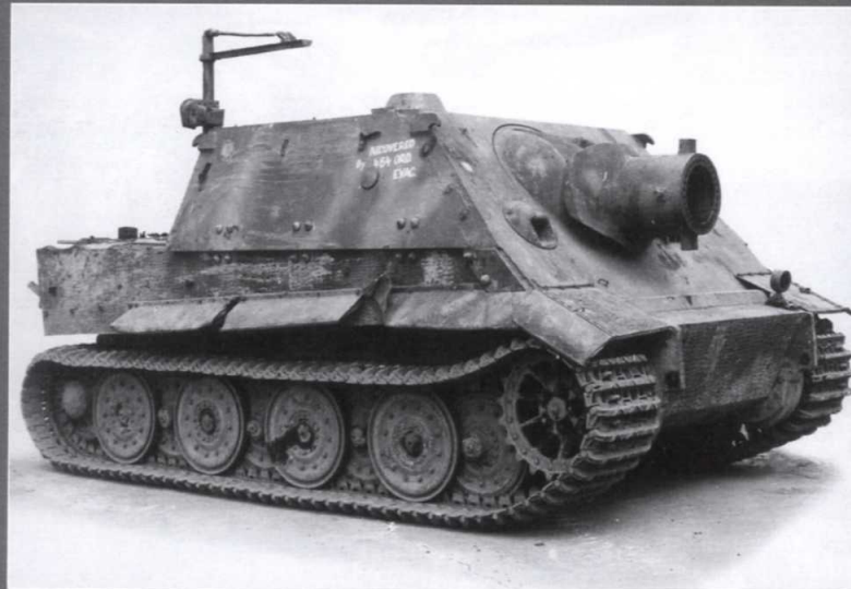
ABOVE The Sturmmörser Tiger. This captured example is fitted with a 38cm RW61 rocket-assisted mortar and shows the jib for manoeuvring the massive rounds that it fired. Also shown is the Zimmerit coating on the hull, evidence of the vehicle's conversion from a Zimmerit -coated gun tank.
