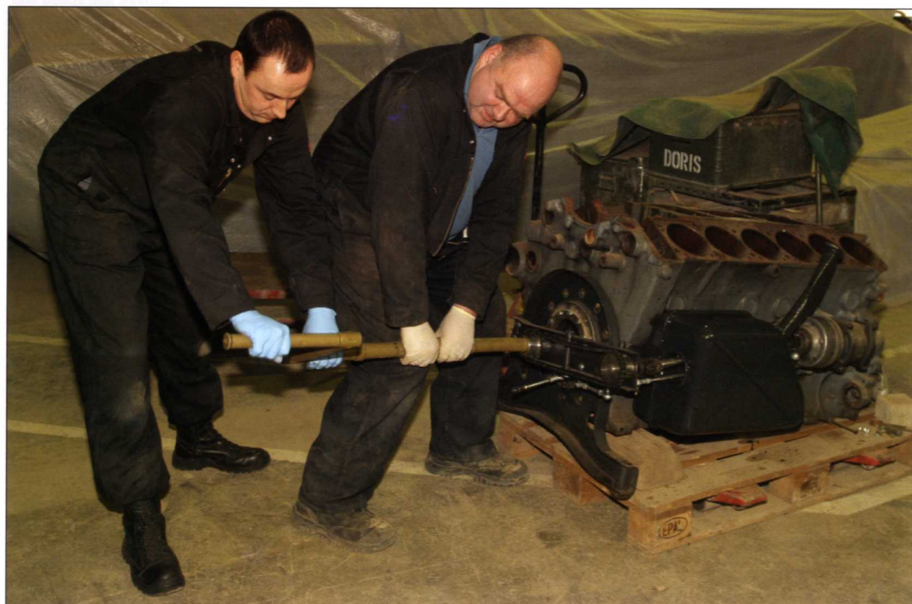
BELOW How it would work – the starting handle would fit through the rear wall of the engine compartment and engage gearing.
