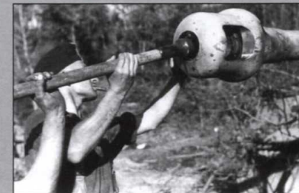
LEFT After firing the gun required cleaning. Light oil was poured onto the brush and the five rods screwed together to remove burnt residues from inside the gun. If left, they would erode the barrel, thereby shortening its life and accuracy.
