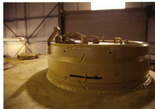
ABOVE The commander's cupola. The top rim had two small tubes welded in place to hold a canvas sun shield, an item rarely used.
