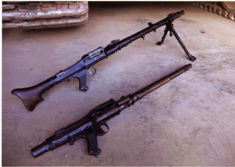
ABOVE The armoured barrelled MG34 for tanks (right) is next to the standard issue weapon.
