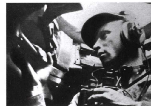
LEFT A Tiger commander looks out through the vision blocks in his cupola, binoculars to hand. He wears headphones and a throat microphone. As a system it had the advantage when in use of not transmitting background noise.
