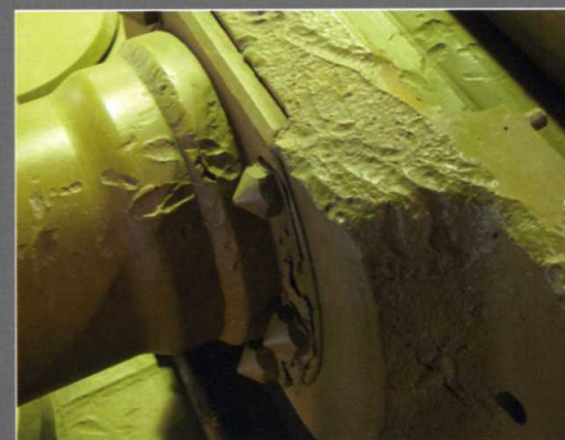
ABOVE Scarring from shell damage around the mantlet.
