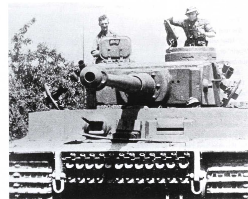
BELOW The crew of Tiger 131 in Tunisia. Note the welded front step and hand grip, and that only two smoke dischargers are present on the left turret bank.
