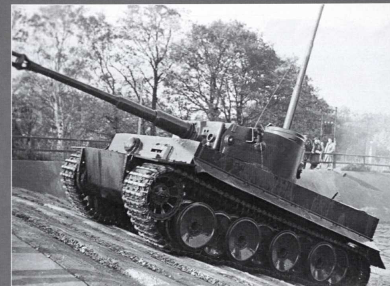
BELOW The Tiger emerges from the water tank. The domed MG34 cover can be clearly seen on the front plate.
