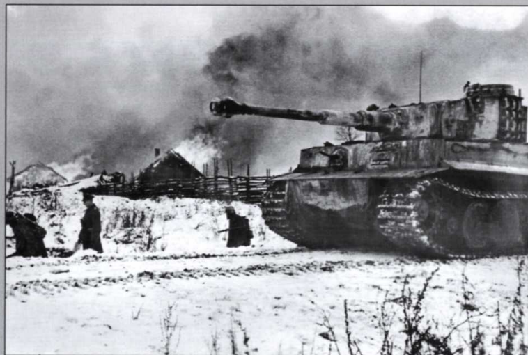
LEFT A Tiger with a whitewash camouflage scheme passes a burning Russian village on the Eastern Front. The front road wheel has been removed, a crew modification to prevent the build-up of earth or snow and the potential loss of a track. (Ullsteinbild/TopFoto 109475)
