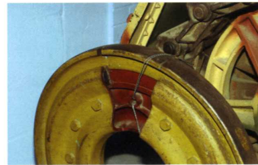
ABOVE Here is an example of a sectioned steel-rimmed road wheel. The rubber is the small black domed section under the central circular ridge. It was sandwiched and held in place between the outer rim and inner wheel section to act as a cushion by the circle of bolts. Belatedly the German authorities pursued the compatibility of parts, with this wheel type fitting the Tiger I and II and Panther series.
