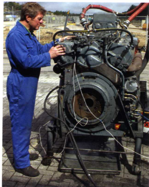
RIGHT The Maybach HL230 is run up on a test stand before refitting to the vehicle.
