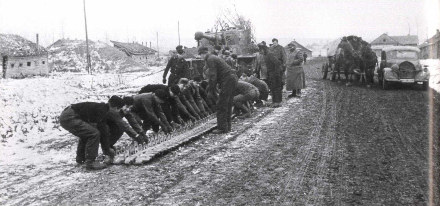
ABOVE 'Eins, Zwei, DREI!' Track is shifted by hand to straighten it ready for replacing on a Tiger in a chilly looking Russian village.
