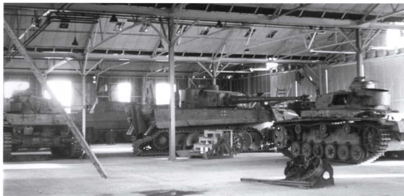
BELOW The Tiger in the sheds at Chobham while under inspection by the Department of Tank Design. Surrounded by other captured German vehicles (a Pz IV, a Pz III, and in the background, a mocked-up Panther), the Tiger has had the front drive sprocket removed, the track is broken and the rear engine deck has been raised.
