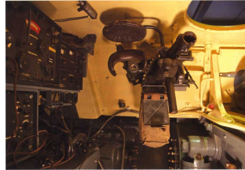
LEFT The bow machine-gun position with MG34 in place. The head cap was supposed to assist the firer in manoeuvring the gun; the sight, the KZF 2, sits under the rubber brow pad to the left of the gun.
