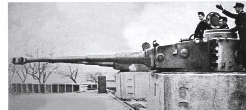
ABOVE Gunnery training was in redundant tank turrets installed on concrete mounts. The range was on the Baltic coast with the guns firing out to sea.
