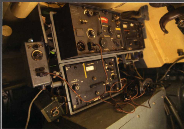
ABOVE The radios installed to the left of the bow machine-gunner's position.
