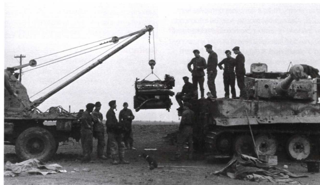
RIGHT The replacement of an engine in the field was never an easy task. Here is a Kfz 100 recovery with the standard 3-ton crane. The dog looks a little bored with it all.
