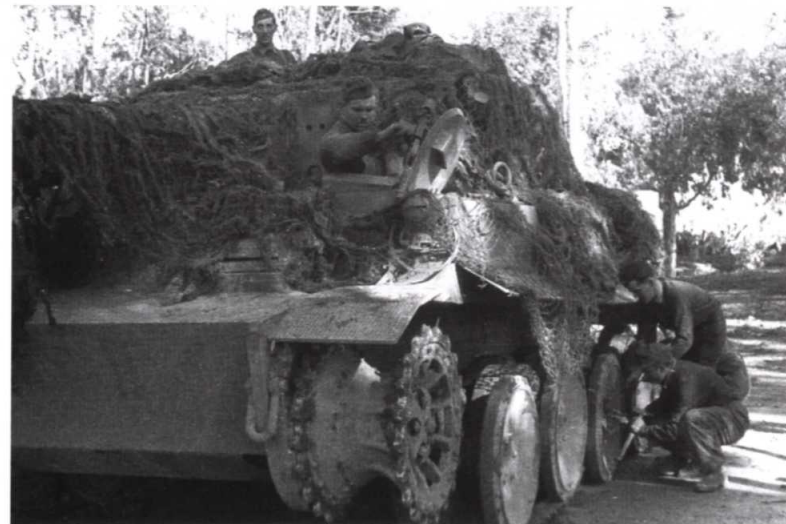
ABOVE 'Eins, Zwei, DREI!' Track is shifted by hand to straighten it ready for replacing on a Tiger in a chilly looking Russian village.
