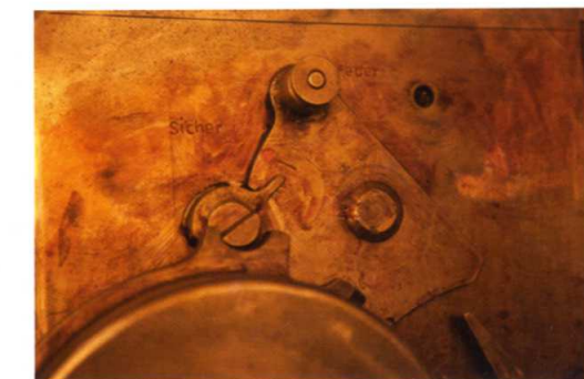
LEFT The safety and fire lock for the loader on the side of the breech. The gun could not be fired until the loader had set the lock to 'fire'.
