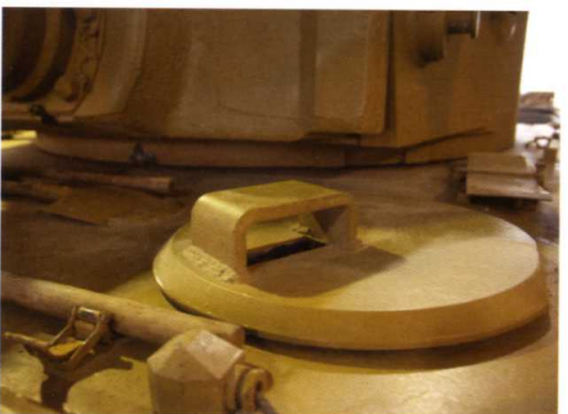
BELOW The driver's hatch closed. The stowed plate on the hull deck behind the hatch was used to seal an engine air intake during deep wading.
