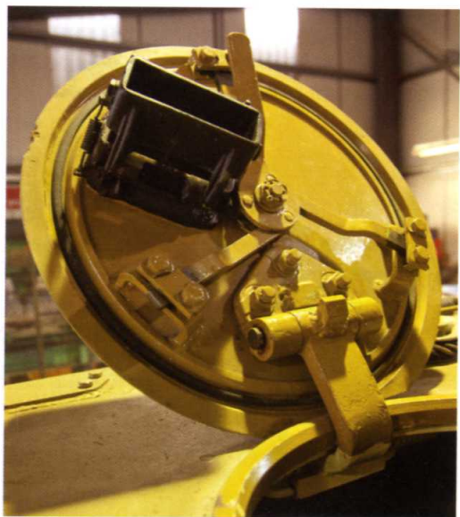
BELOW The driver's hatch closed. The stowed plate on the hull deck behind the hatch was used to seal an engine air intake during deep wading.
