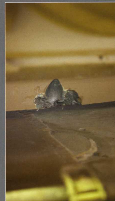
ABOVE Scarring from shell damage around the mantlet.
