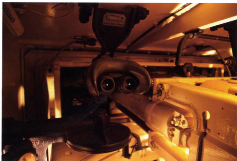
ABOVE Looking forward from the loader's position. The hand wheel (to the right of the eye pad) gives fine adjustment to the traverse. On the bracket above the sight a notice warns that the sight must be secured in position.
