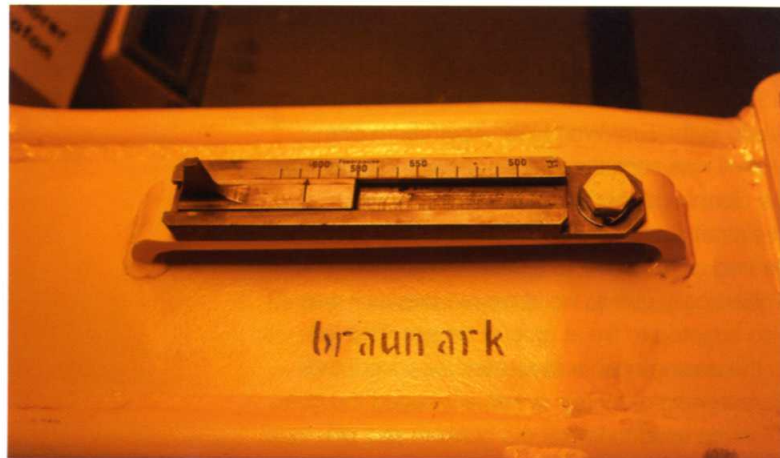
ABOVE The stencilled Braun Ark was a reminder of the fluid the gun hydraulics contained – a mixture of brown buffer fluid ( Bremsflüssigkeit braun ) and Arctic fluid ( Bremsflüssigkeit Arktisch ). The gun could recoil back to 620mm, but a marker on this gauge at 580mm warned 'Feuerpause' or 'Stop Firing'.
