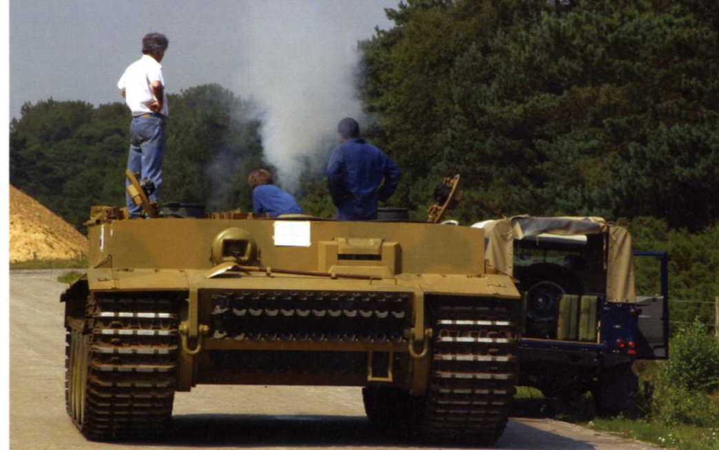
LEFT A test-track run for the engine in the hull. A connecting rod has just smashed through the engine block.
