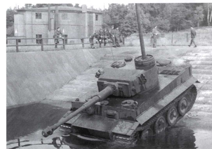
BELOW The trial at Haustenbeck near Sennelager. Here the Tiger is fitted with a snorkel in the commander's cupola.
