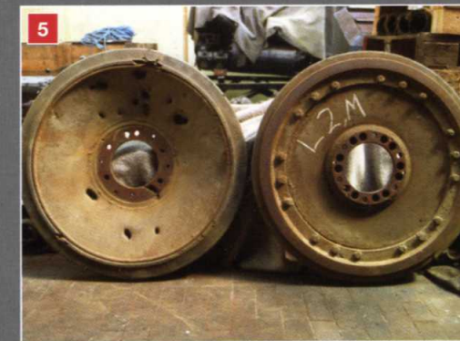
5 Removal of the road wheels. Here, battle damage can be clearly seen.
