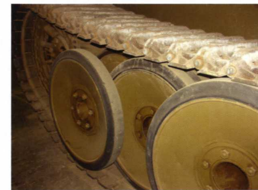
LEFT Correct track adjustment.
