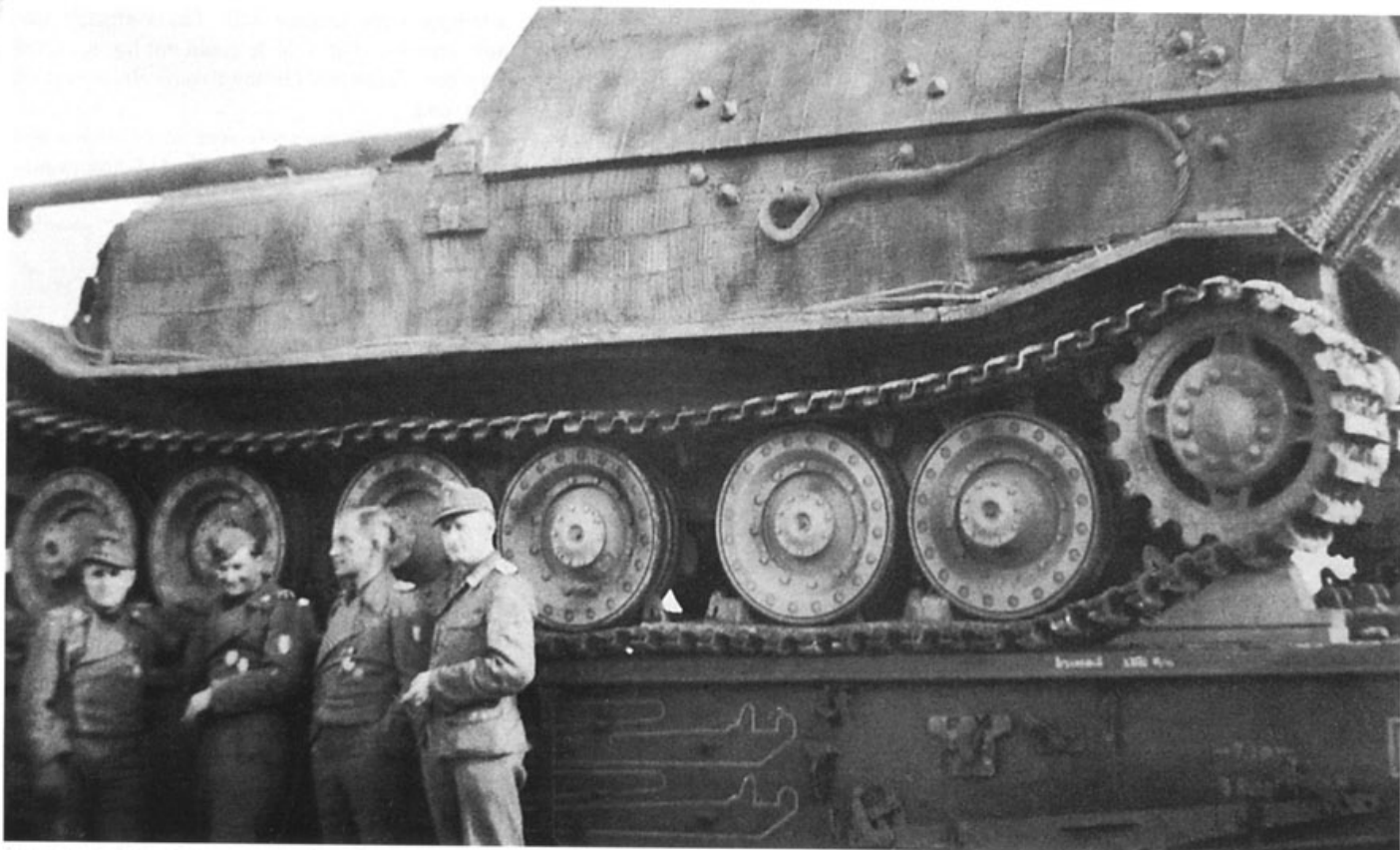
„Ferdinand“ z 1. kompanii 653. schwere Panzerjäger Abteilung na platformie Ssym w drodze na front włoski, luty 1944 roku. Pojazd jest pokryty Zimmeritem. A “Ferdinand” SP gun of the 1st Company 653rd schwere Panzerjäger Abteilung on Ssym railway flatcar, February 1944. Note vehicle is covered Zimmerit coating. [ASKM]
